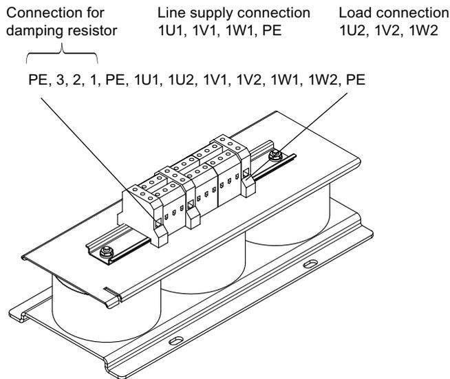
Figure 2-45 HFD line reactor 16 kW
