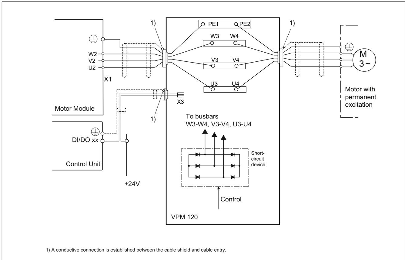
Figure 9-8 Connection example for Voltage Protection Module VPM 120
