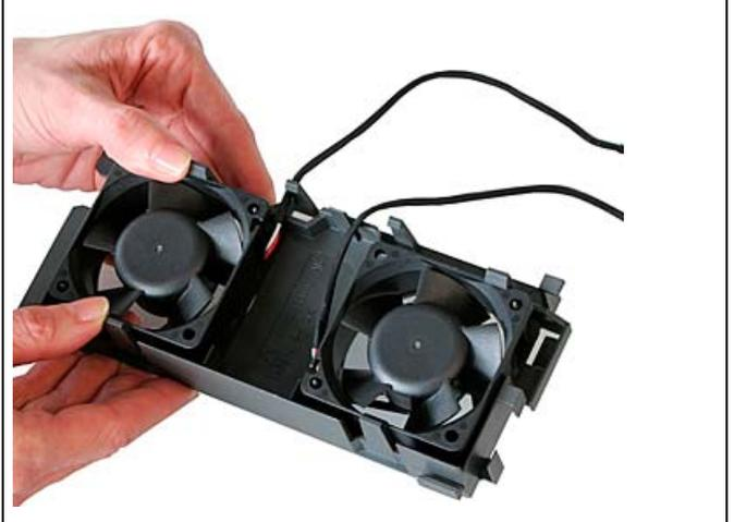
Slightly push the fan holder apart and pull out the fan
