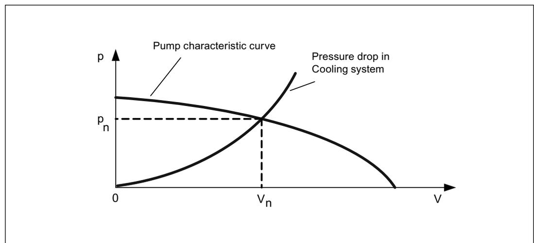
Figure 12-1 Pump characteristic curve
