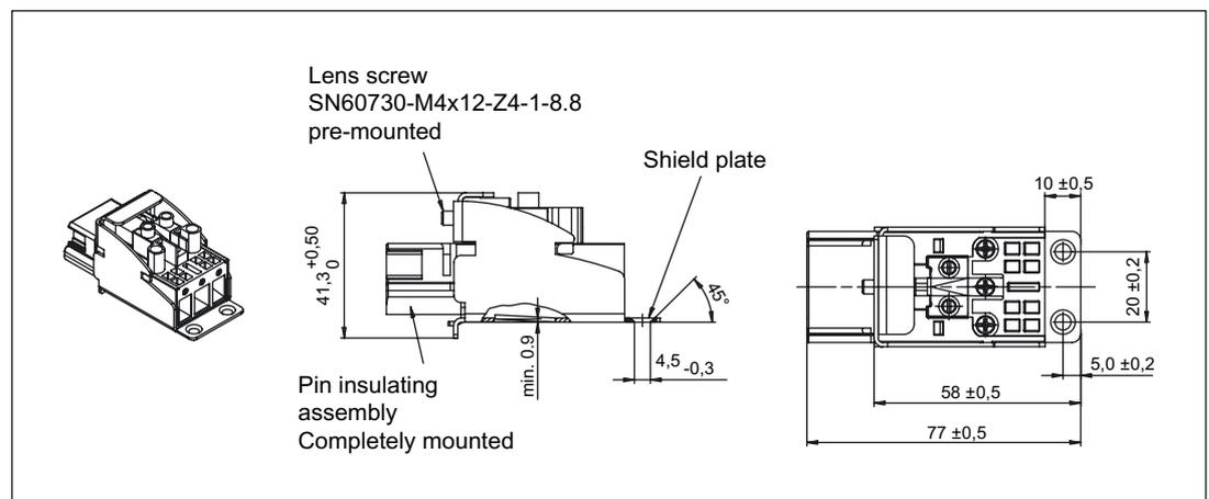
Figure 11-26 Dimensions: Power connector
