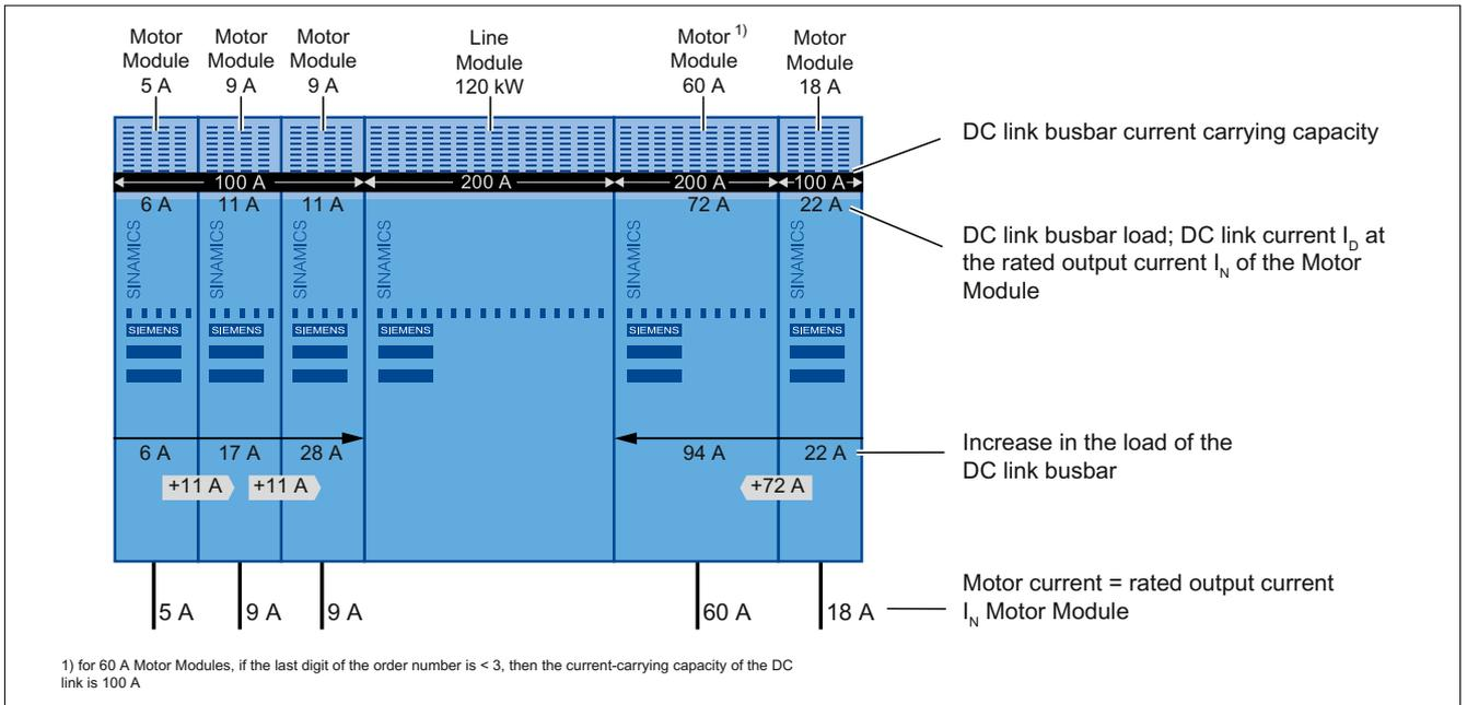
Figure 11-8 Infeed from left and right (center infeed)
