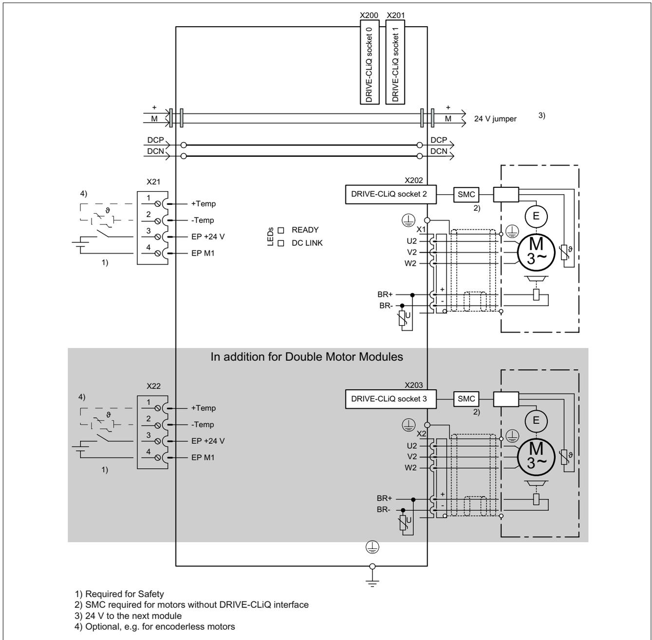
Figure 5-21 Connection example of Motor Modules 3 A to 30 A and Double Motor Modules 3 A to 18 A
