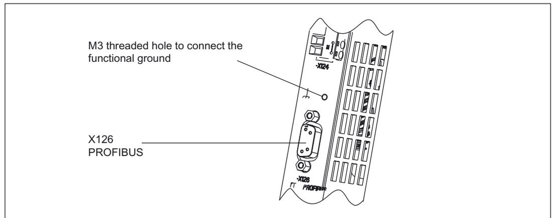
Figure 11-16 Functional ground connection for PROFIBUS
