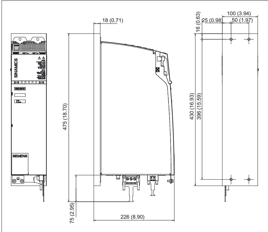
Figure 3-76 Dimension drawing of Basic Line Module with cold plate (20 kW), all dimensions in mm and (inches)
