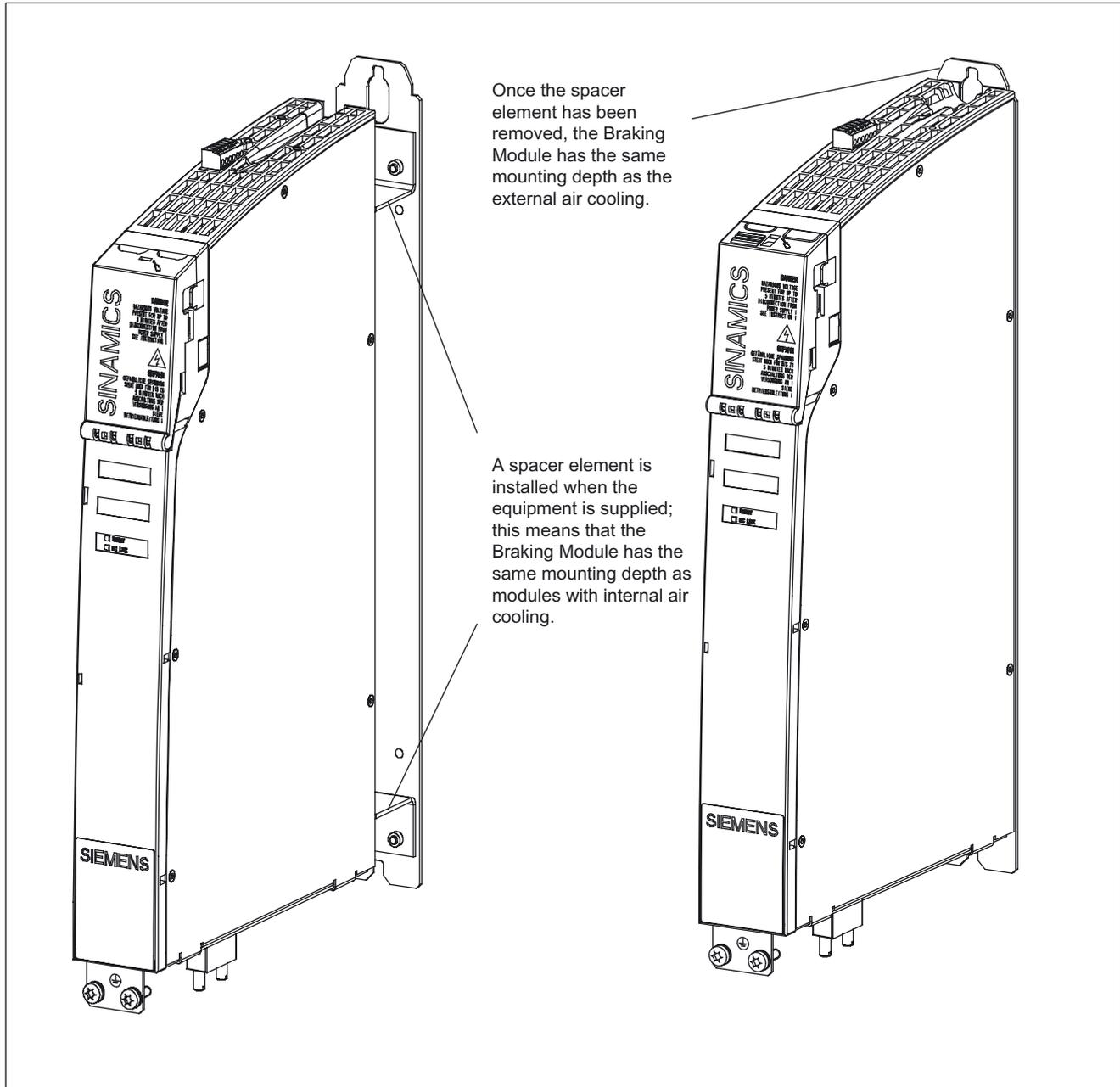
Figure 8-4 Methods of installing Braking Modules with/without spacer elements
