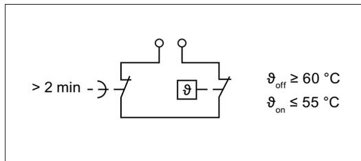
Figure 9-10 Signaling contact X3 of the Voltage Protection Module
