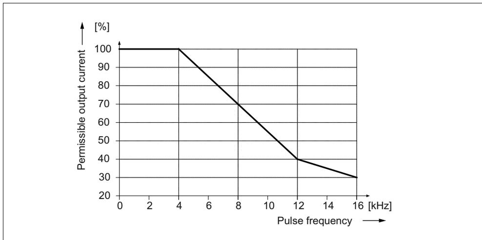
Figure 5-77 Output current as a function of the pulse frequency (applies from order number 6SL312x-1TE32-0AA4)
