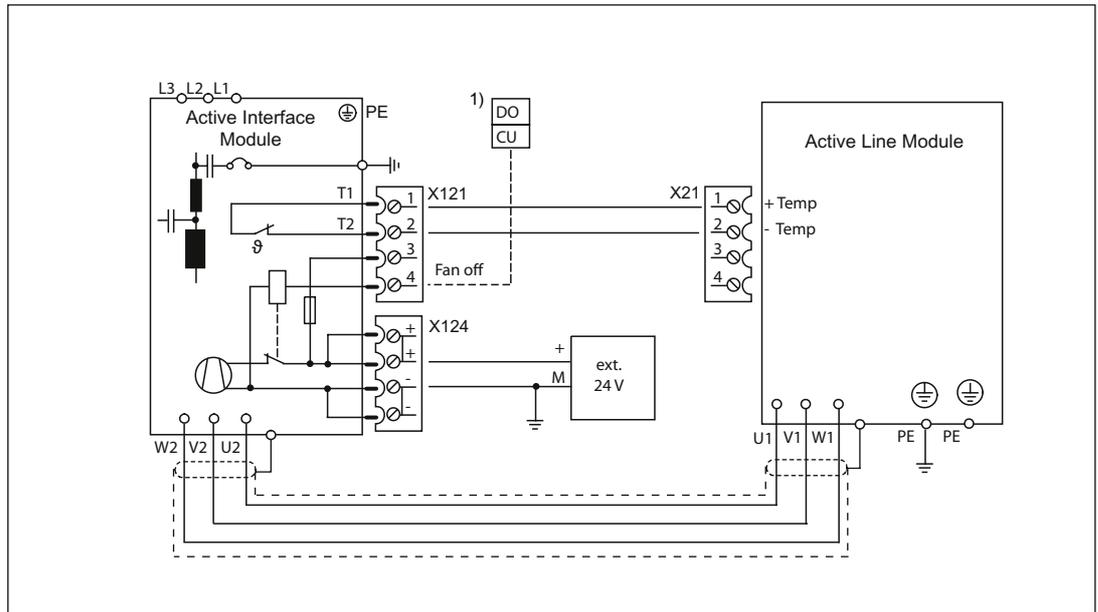
Figure 2-34 Connection example: Active Interface Module
