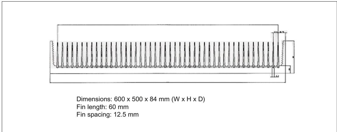
Figure 11-30 Example of an air heat sink
