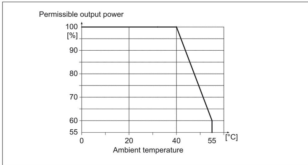
Figure 3-99 Output power as a function of the ambient temperature
