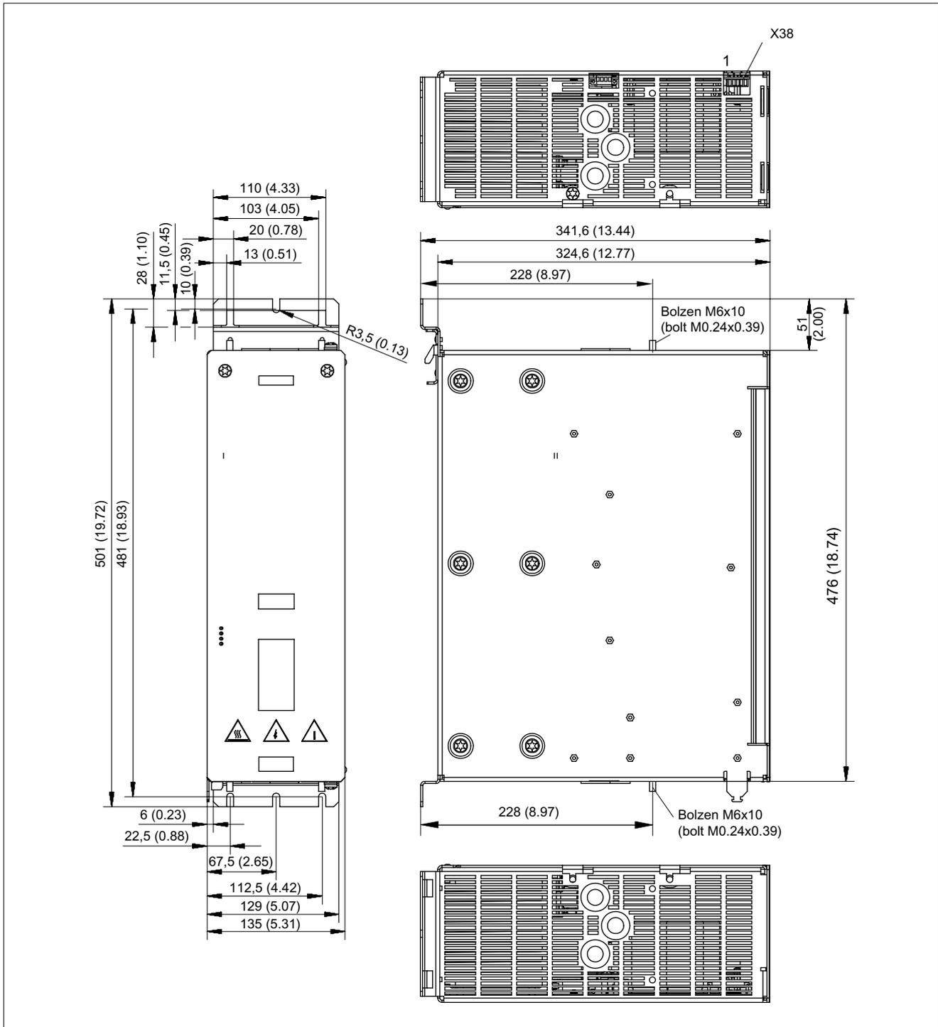
Figure 3-70 Dimension diagram of MASTERDRIVES braking unit, all data in mm and (inches)
