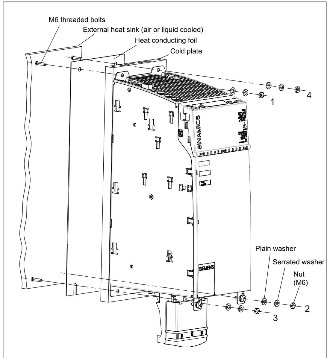
Figure 3-34 Installation of a cold plate power unit with an external heat sink and heat-conducting foil
