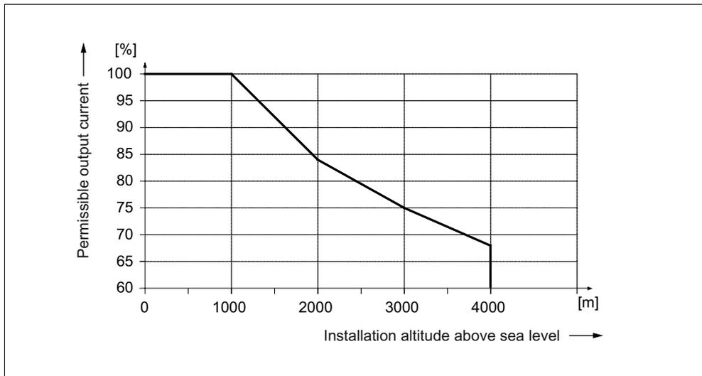
Figure 5-43 Output current as a function of the installation altitude
