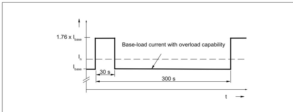
Figure 5-57 Duty cycle with 30 s overload with a duty cycle duration of 300 s
