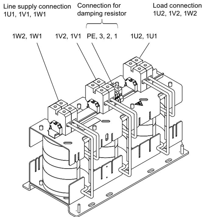
Figure 2-49 HFD line reactor 120 kW
