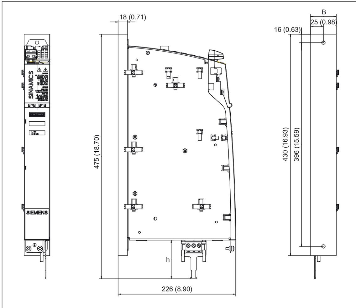
Figure 3-116 Dimension drawing of Smart Line Module with cold plate (5 kW and 10 kW), all dimensions in mm and (inches)
