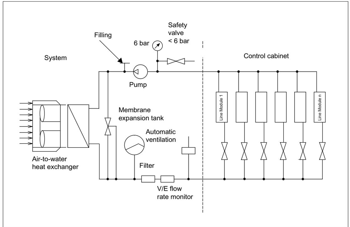
Figure 12-5 Air-to-water heat exchanger
