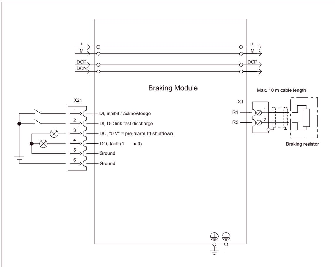
Figure 8-2 Example connection of Braking Module
