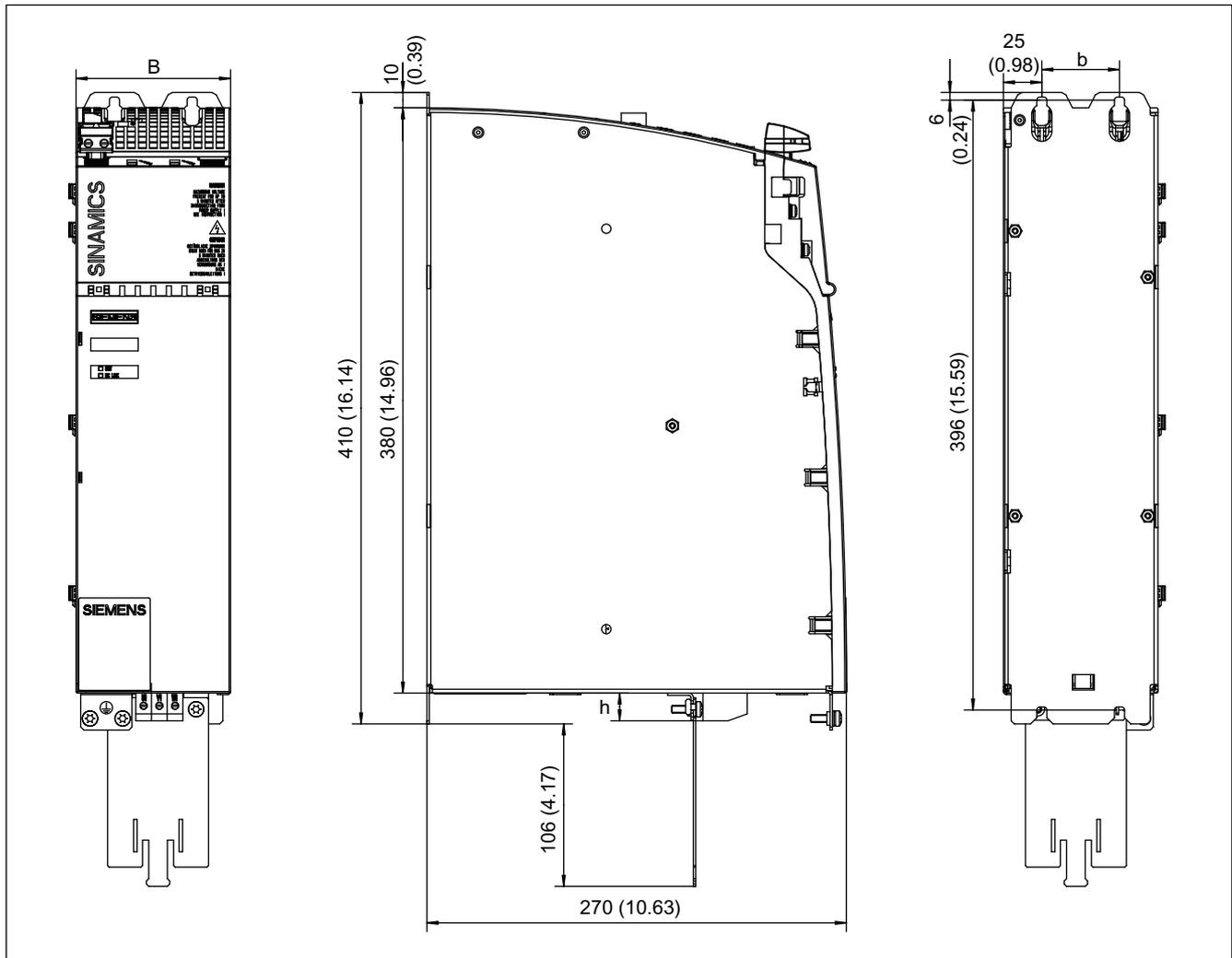
Figure 3-3 Dimension drawing of Active Line Module 16 kW with internal air cooling, all data in mm and (inches)
