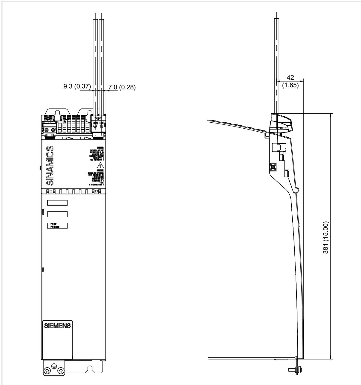
Figure 10-21 Dimension drawing of 100 mm component with DC link rectifier adapter for 0.5 mm<sup>2</sup> to 10 mm<sup>2</sup>, all dimensions in mm and (inch)
