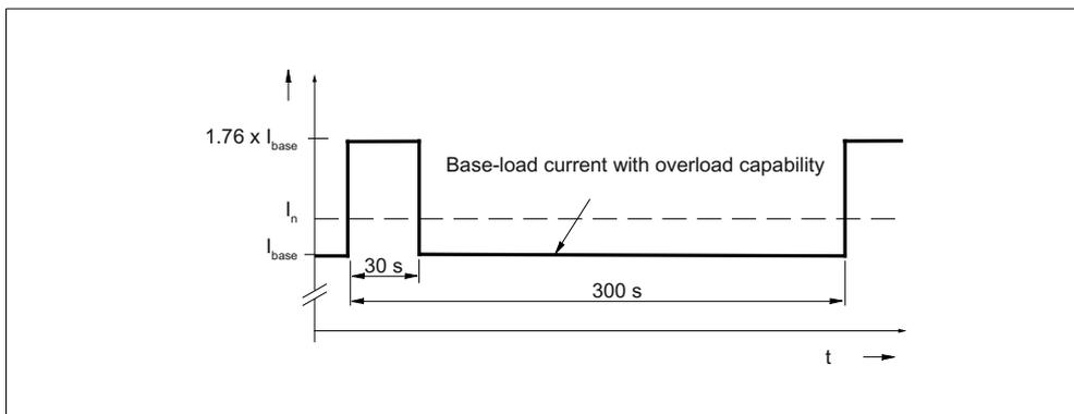
Figure 5-13 Duty cycle with 30 s overload with a duty cycle duration of 300 s
