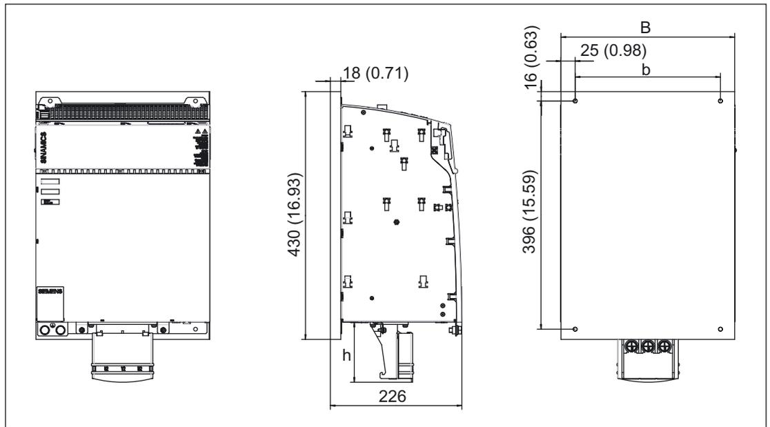
Figure 5-51 Dimension drawing of Motor Module with cold plate 132 A and 200 A, all dimensions in mm and (inches)
