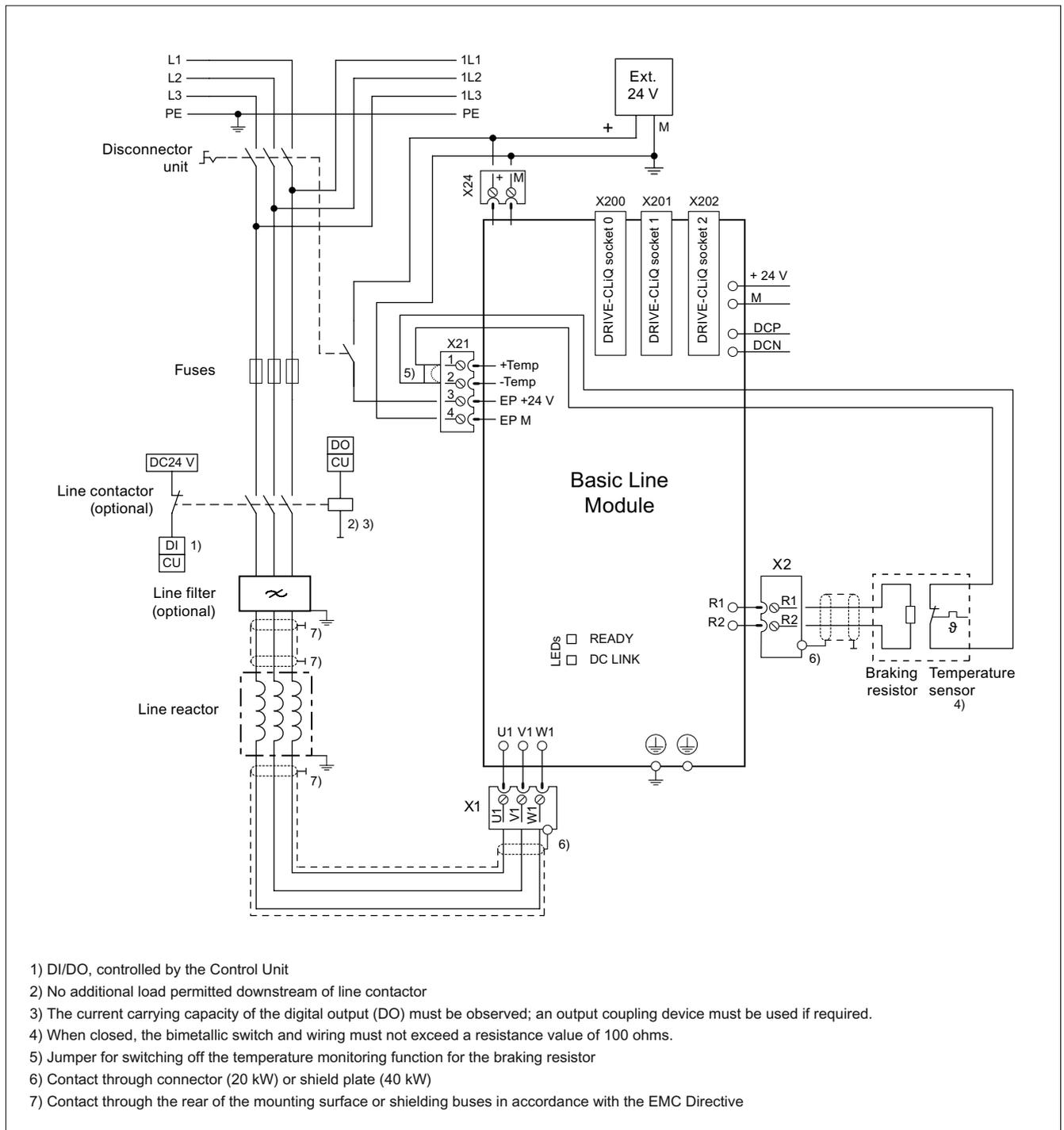
Figure 3-53 Connection example: Basic Line Module (20 kW and 40 kW)
