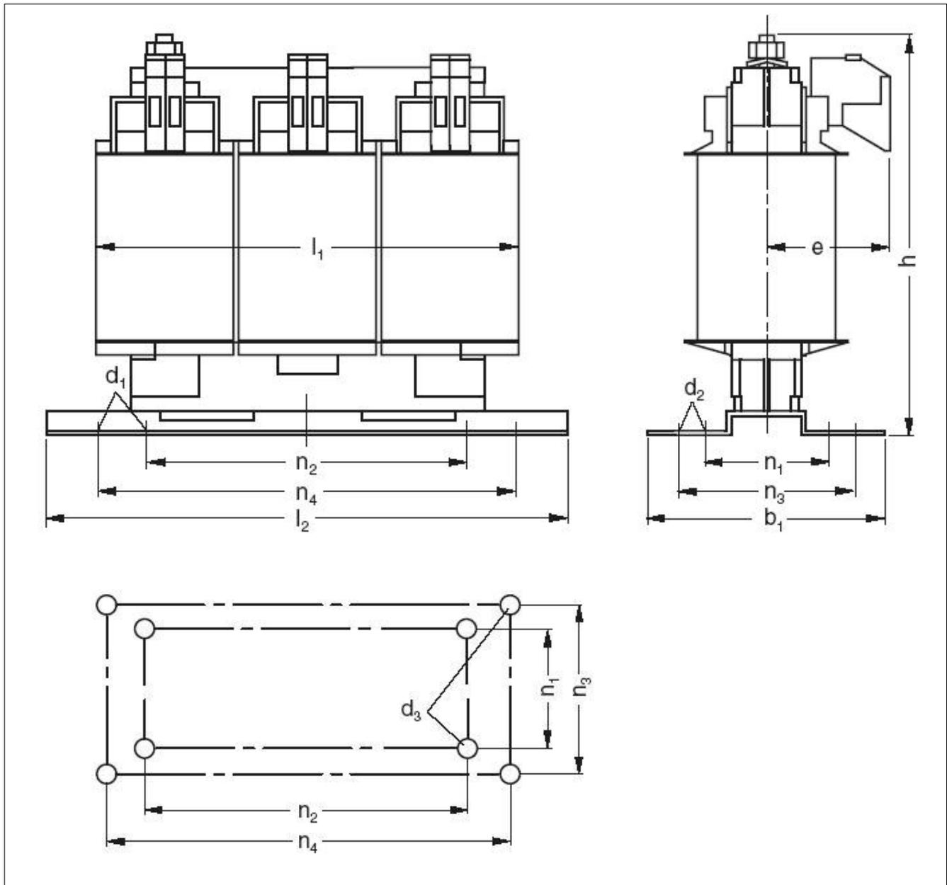
Figure 9-3 Dimension drawing and mounting hole of motor reactor 9 A (6SL3000-2BE21-0AA0)
