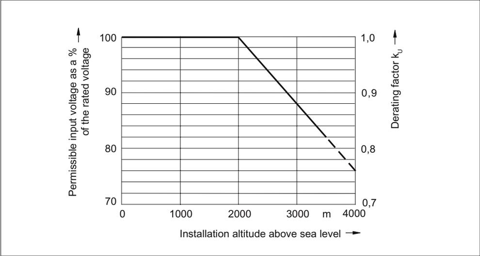
Figure 3-86 Voltage derating as a function of the installation altitude
