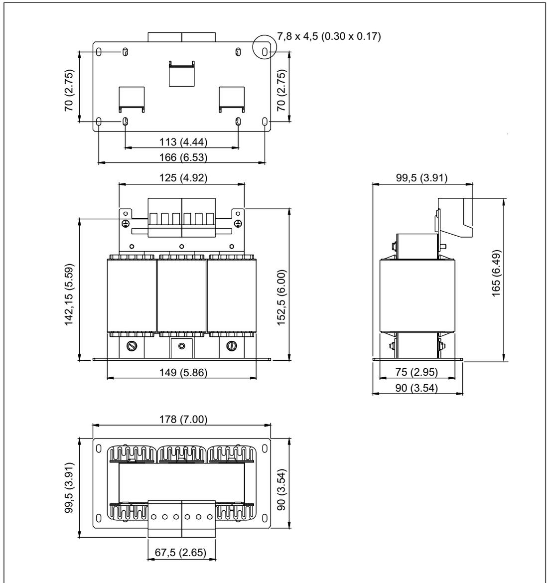
Figure 2-66 Dimension drawing of line reactor for Basic Line Module 20 kW, all dimensions in mm and (inches)
