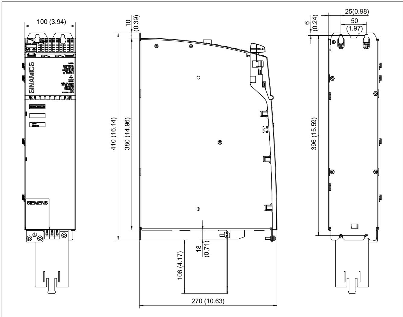
Figure 3-96 Dimension drawing of Smart Line Module with internal air cooling (16 kW), all dimensions in mm and (inches)
