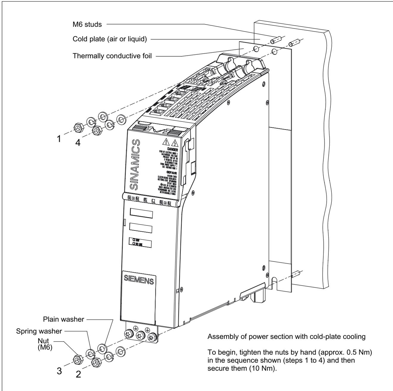
Figure 6-9 Installation: Motor Module Booksize Compact with cold plate
