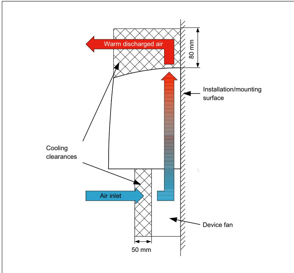
Figure 11-35 Cooling clearances for 300 mm components with mounted equipment fan
