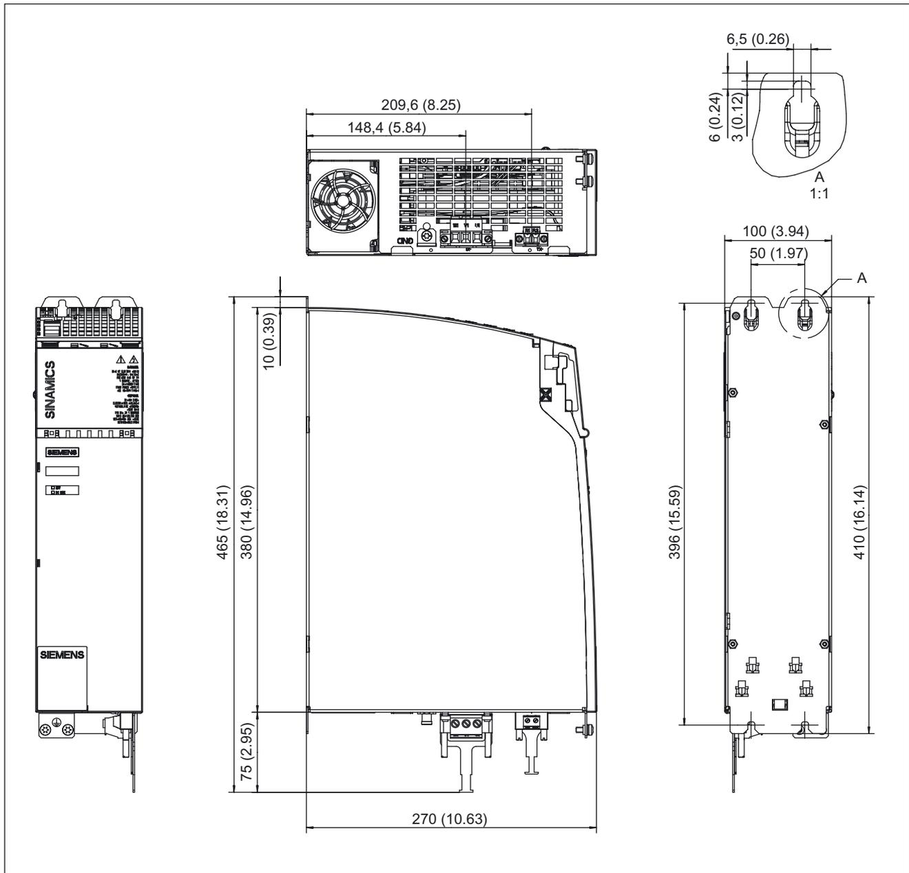
Figure 3-55 Dimension drawing of Basic Line Module 20 kW with internal air cooling, all dimensions in mm and (inches)
