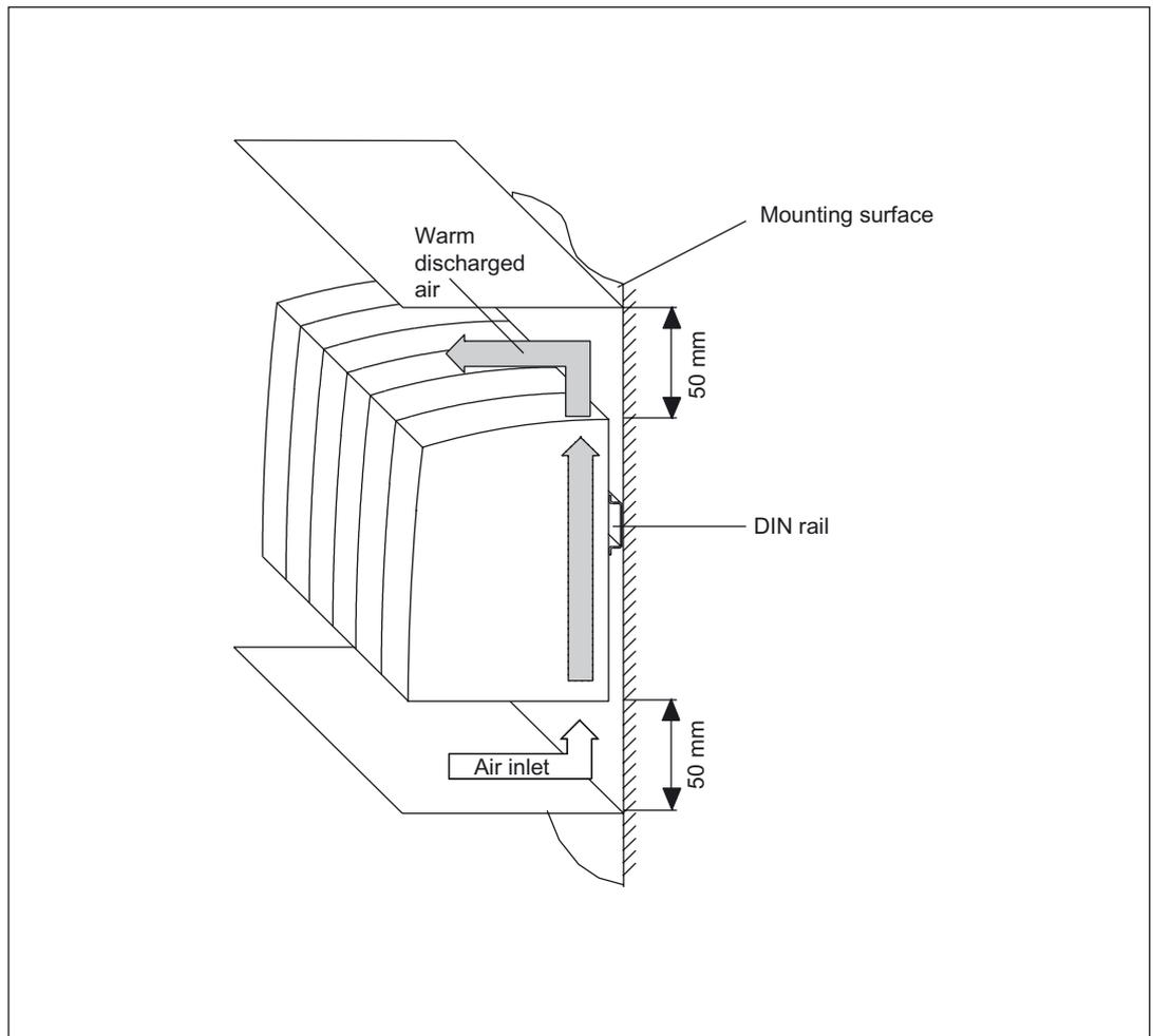
Figure 11-36 Cooling clearances, rail-mounted modules (e.g. VSM, SMC, TM, DMC)
