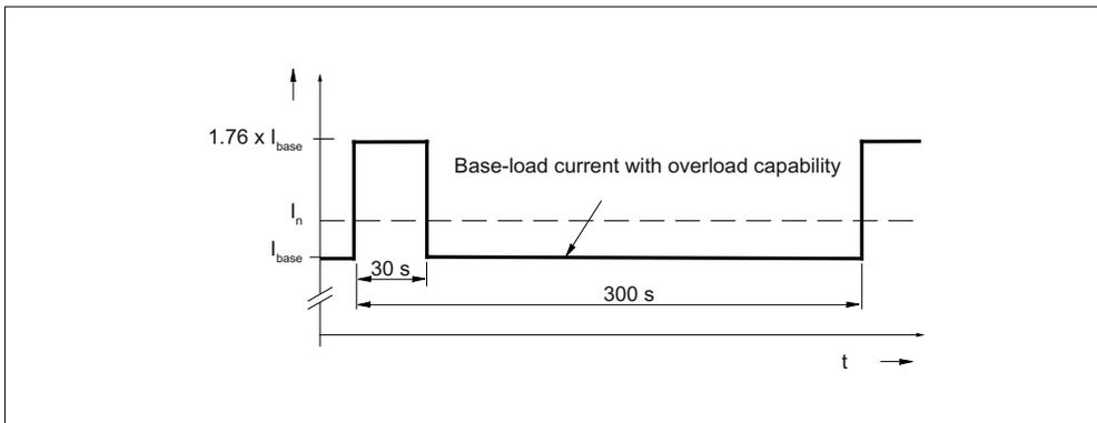
Figure 5-72 Duty cycle with 30 s overload with a duty cycle duration of 300 s
