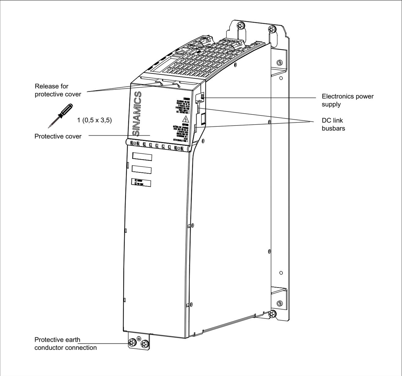
Figure 8-8 Interface description of the capacitor module
