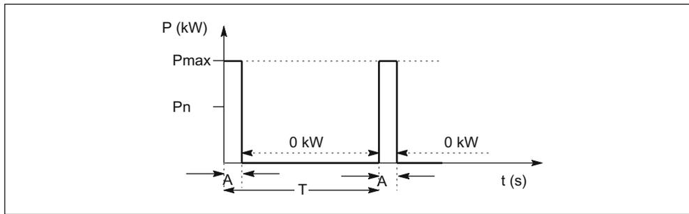
Figure 8-7 Duty cycle for braking resistors
