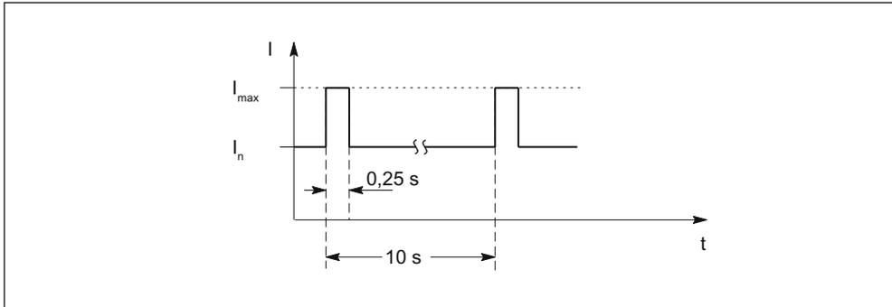
Figure 5-53 Duty cycle with initial load (for servo drives)
