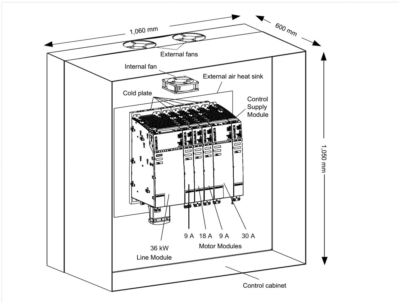
Figure 11-28 Example: cabinet setup with powers actions, cold plate, and external air heat sink
