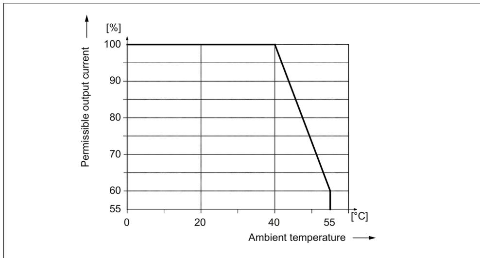
Figure 5-40 Output current as a function of the ambient temperature
