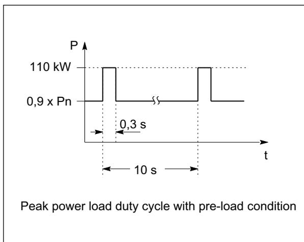
Figure 3-10 Rated duty cycle of 55 kW Active Line Modules with Active Interface Module
