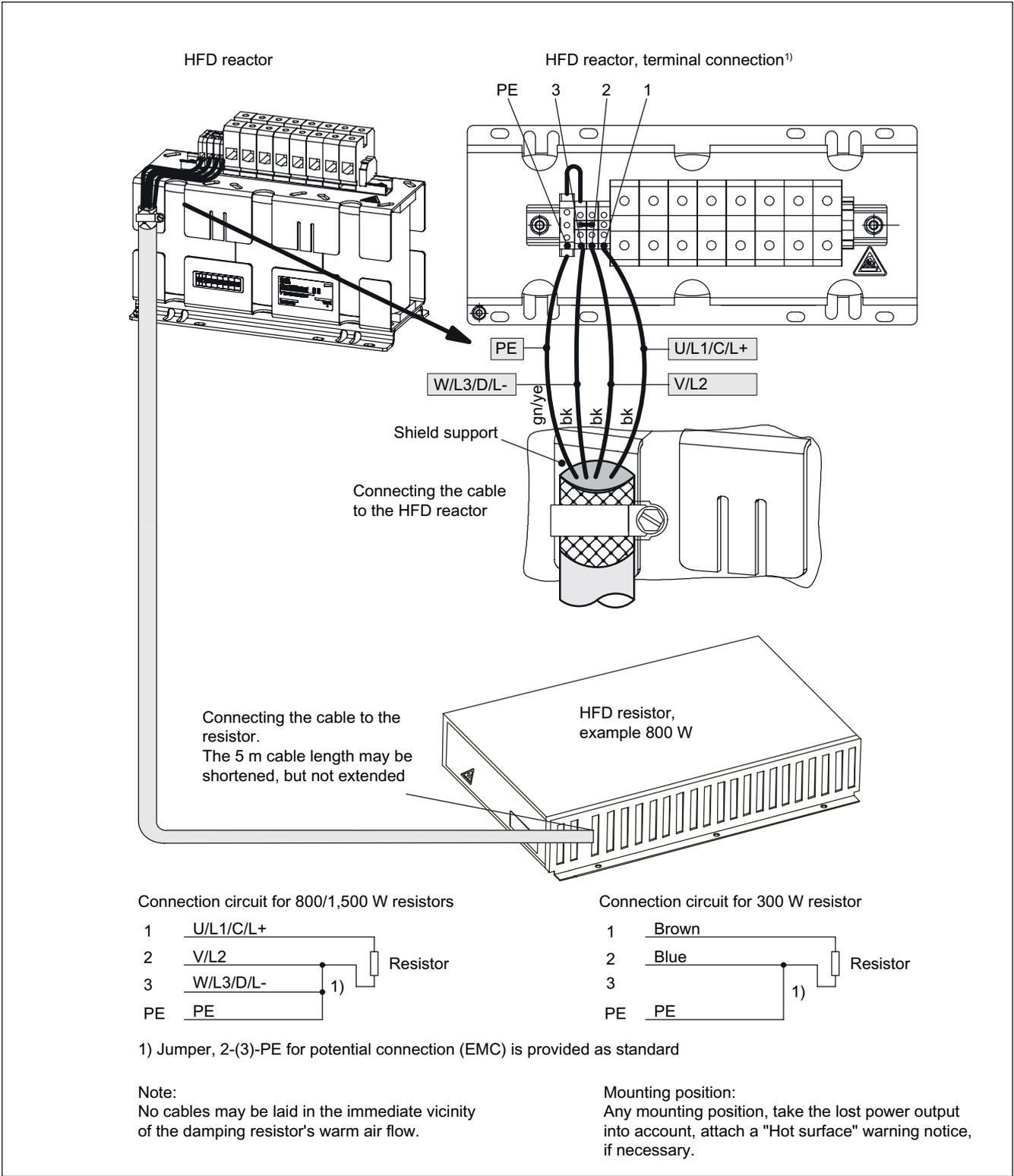
Figure 2-58 Wiring the HFD line reactor with a damping resistor
