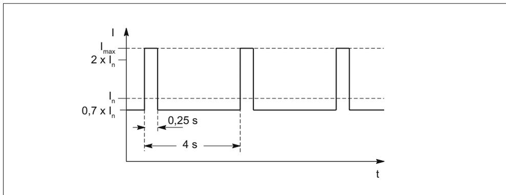
Figure 6-14 Peak current duty cycle with initial load
