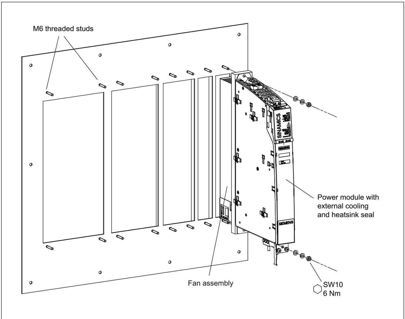
Figure 3-105 Example: Installation of the Power Module with external air cooling
