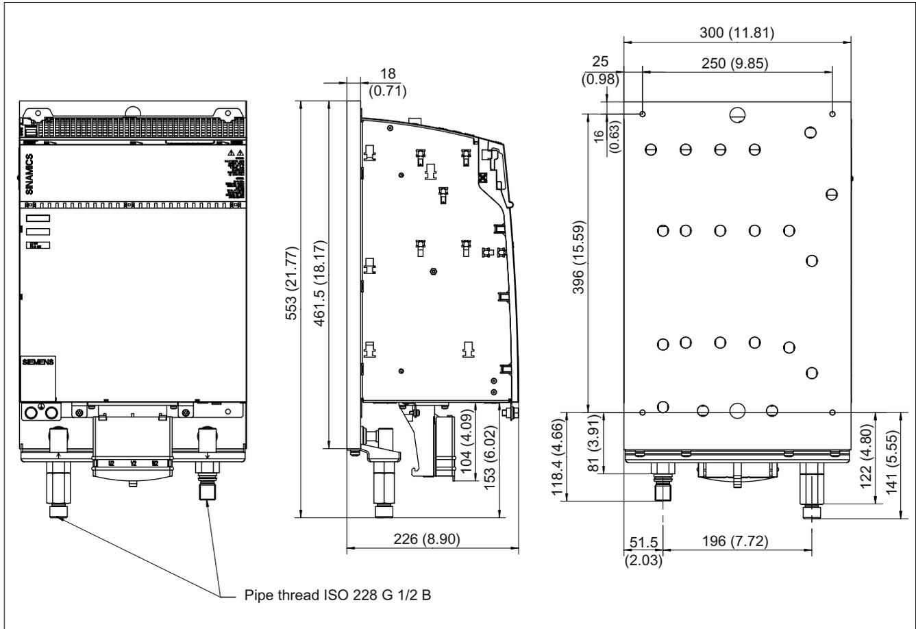
Figure 5-66 Dimension drawing of Motor Module Liquid Cooled (200 A), all dimensions in mm and (inches)
