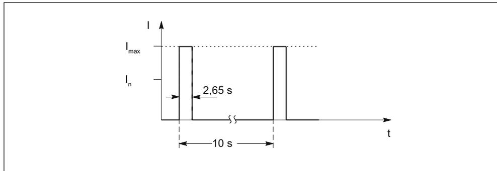
Figure 5-35 Duty cycle without initial load (for servo drives)
