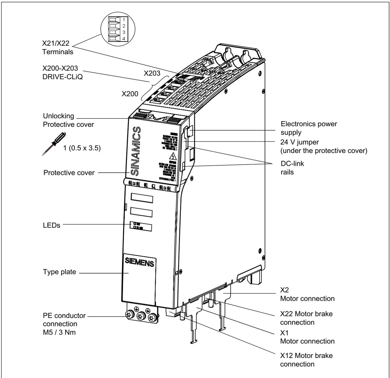
Figure 6-3 Example: Double Motor Module Booksize Compact format 2 x 1.7 A, 2 x 3 A, 2 x 5 A
