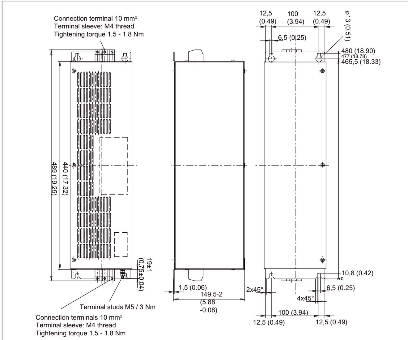
Figure 2-17 Dimension drawing of Wideband Line Filter 16 kW for Active Lines Modules, all dimensions in mm and (inches)
