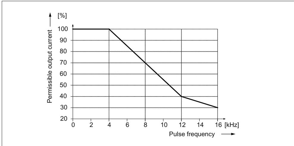
Figure 5-42 Output current as a function of the pulse frequency for 200 A Motor Modules (applies from order number 6SL312x-1TE32-0AA4)
