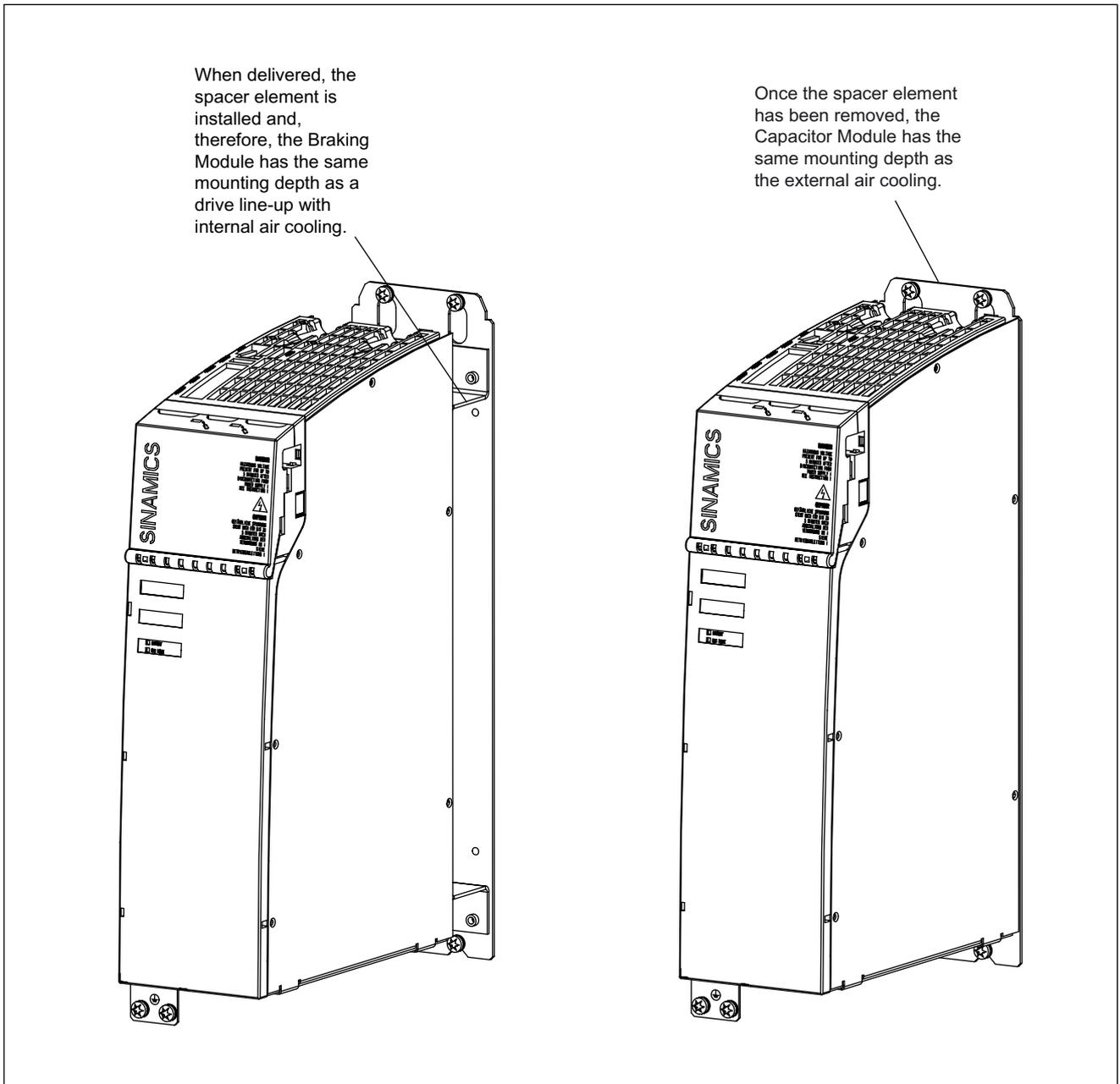
Figure 8-10 Installing a Capacitor Module with/without spacer elements
