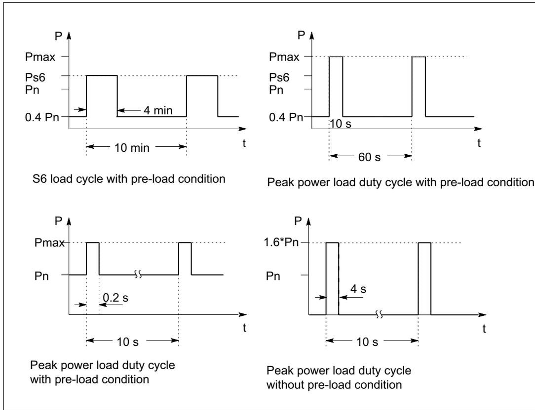
Figure 3-98 Rated duty cycles of Smart Line Modules
