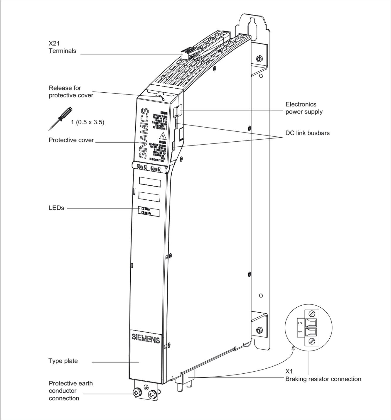
Figure 8-1 Interface description of Braking Module
