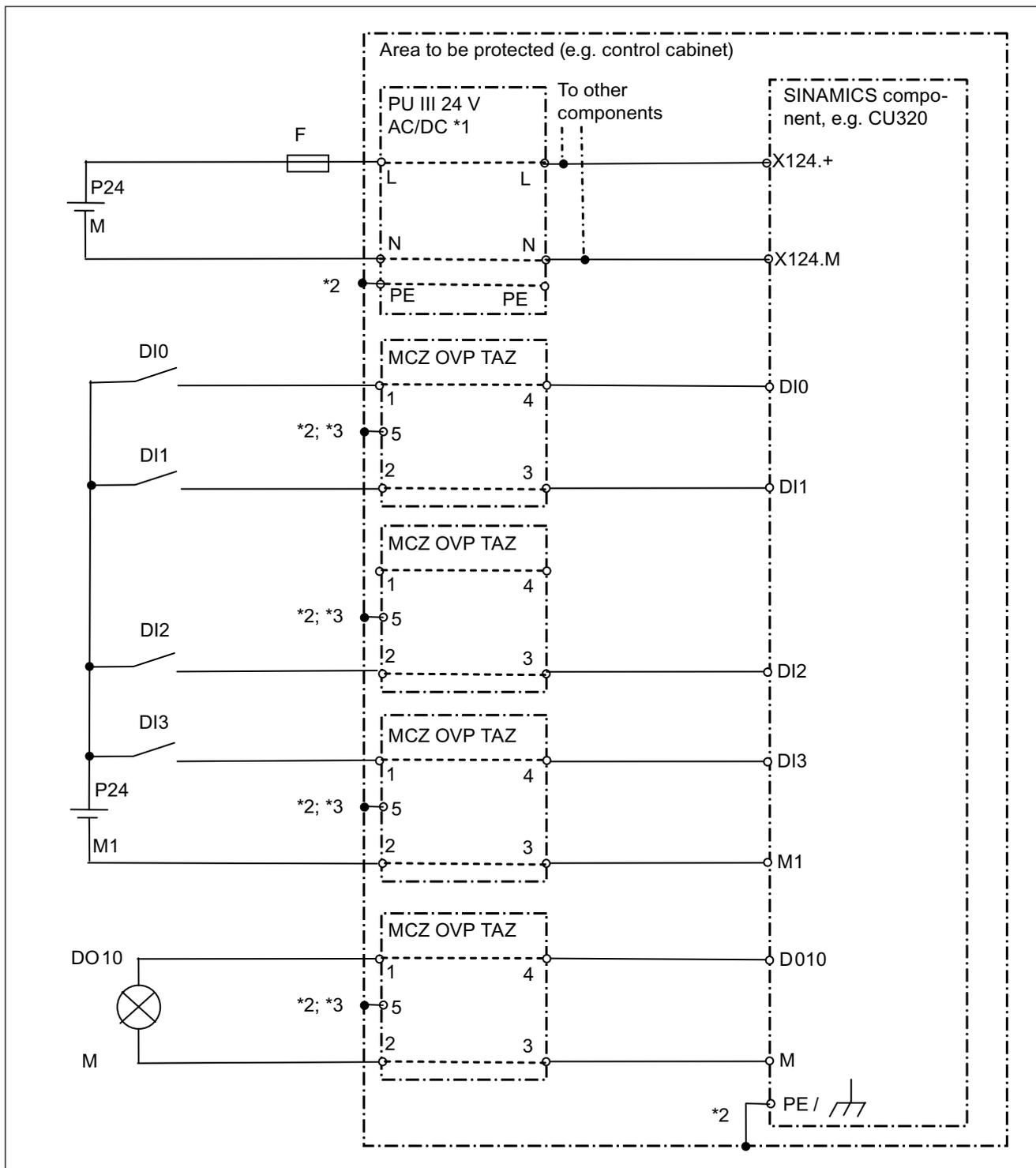
Figure 11-6 Connection example: Overvoltage protection components from Weidmüller to SINAMICS components
