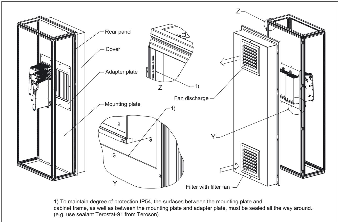
Figure 5-33 Example 2: installation in cabinet with mounting plate
