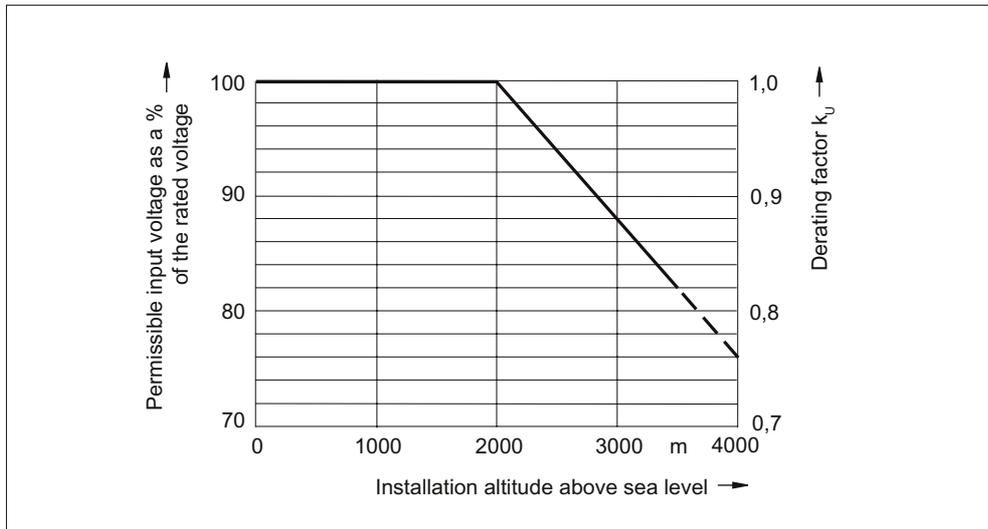
Figure 3-64 Voltage derating as a function of the installation altitude
