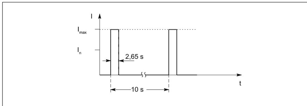
Figure 5-69 Duty cycle without initial load (for servo drives)
