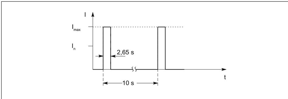
Figure 5-10 Duty cycle without initial load (for servo drives)
