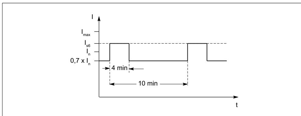
Figure 5-70 S6 duty cycle with initial load with a duty cycle duration of 600 s (for servo drives)
