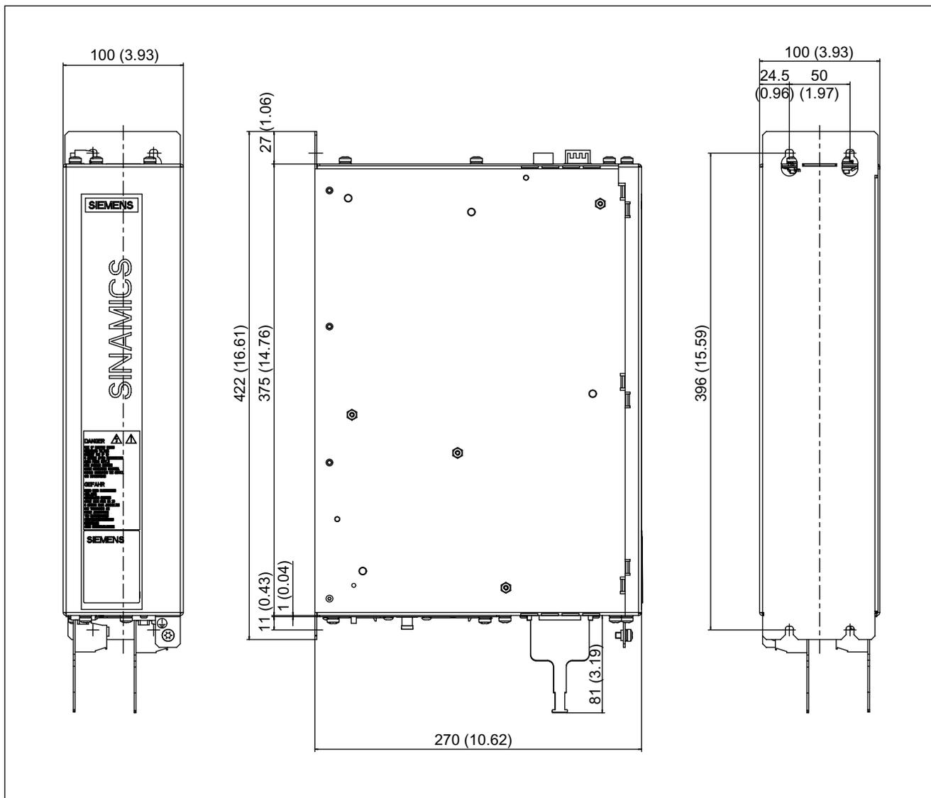
Figure 2-35 Dimension drawing of Active Interface Module 16 kW, all dimensions in mm and (inches)
