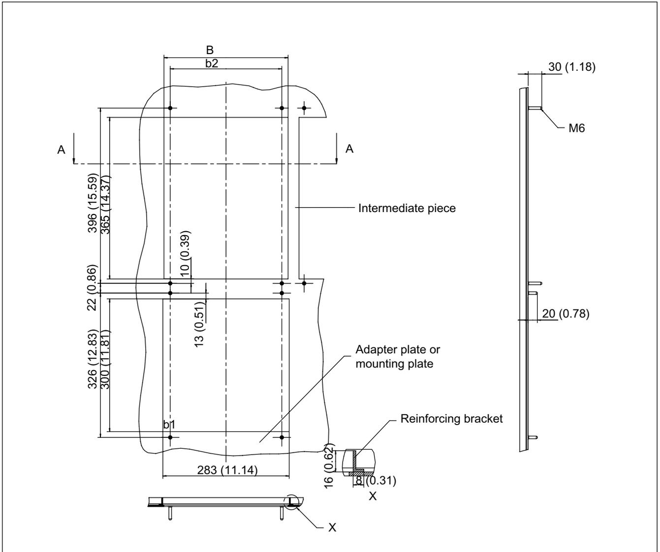
Figure 5-30 Installation openings for the power unit with external air cooling, 300 mm
