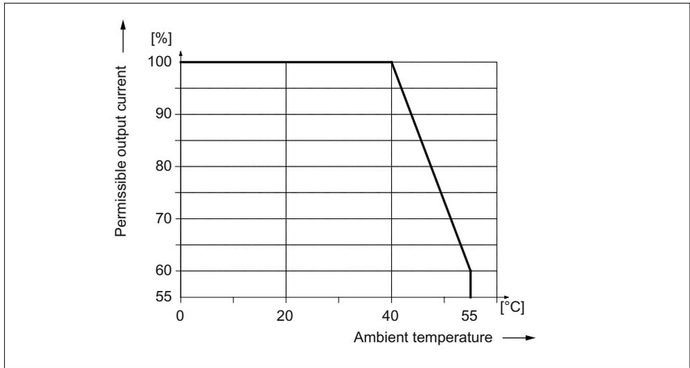
Figure 5-59 Output current as a function of the ambient temperature
