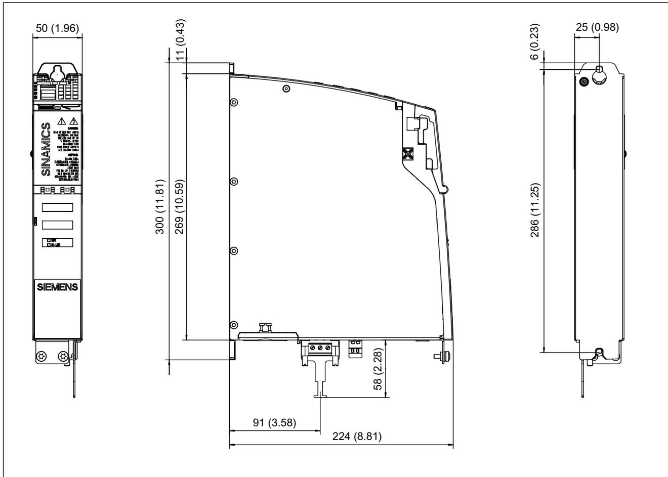
Figure 6-5 Dimension drawing of Motor Module in booksize compact format 3 A, 5 A, and 9 A, all dimensions in mm and (inches)
