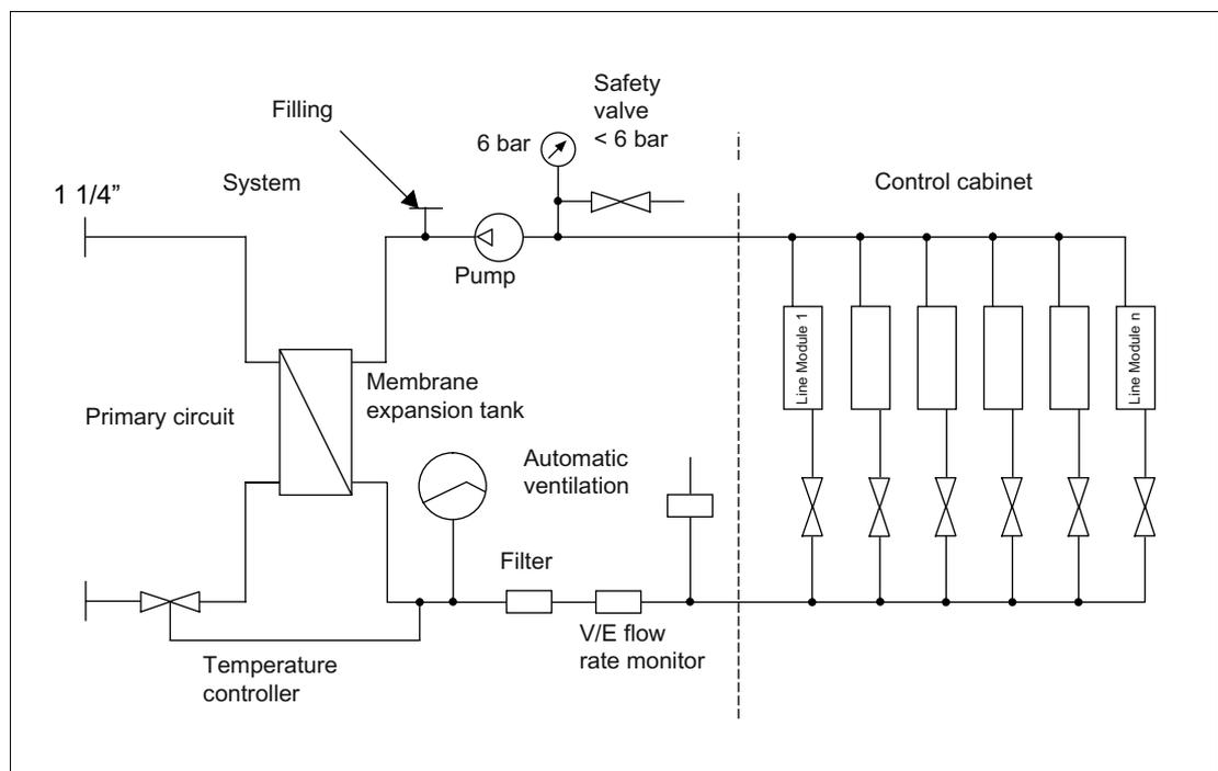
Figure 12-4 Water-to-water heat exchanger
