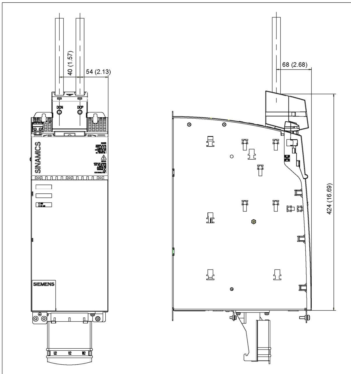
Figure 10-22 Dimension drawing of 150 mm component with DC link rectifier adapter for 35 mm<sup>2</sup> to 95 mm<sup>2</sup>, all dimensions in mm and (inch)
