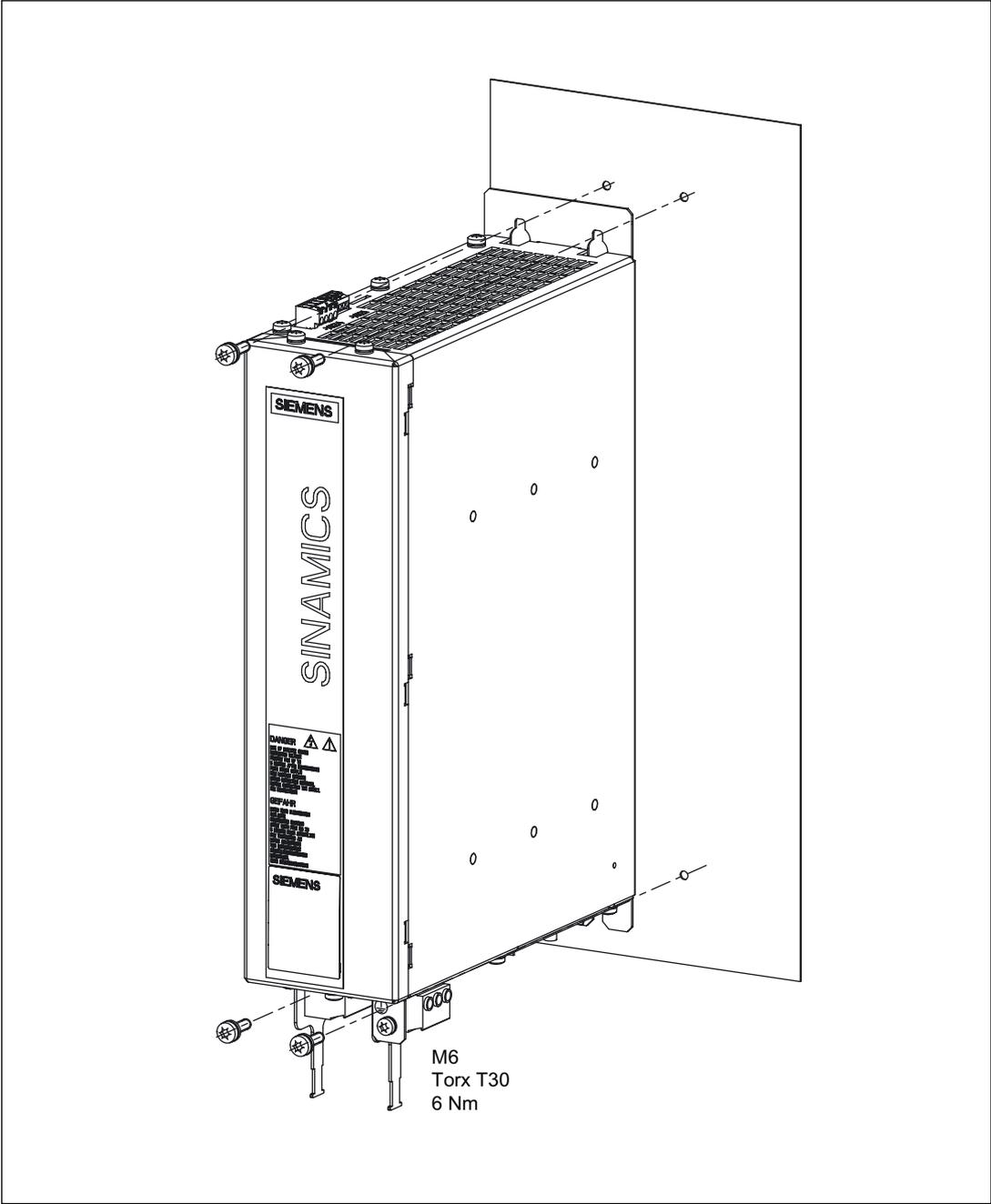
Figure 2-39 Mounting: Active Interface Module 16 kW
