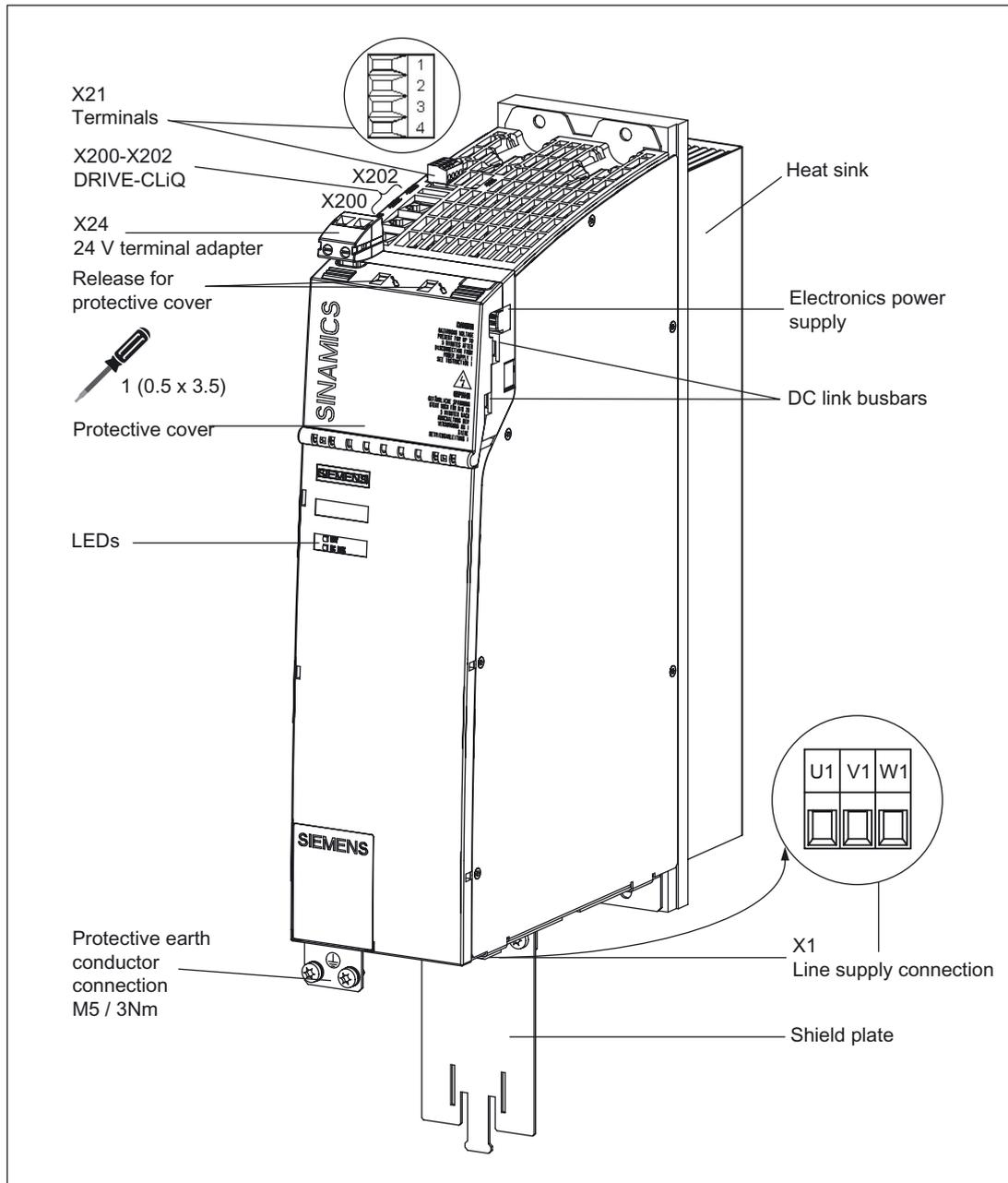
Figure 3-14 Active Line Module with external air cooling (example: 16 kW)
