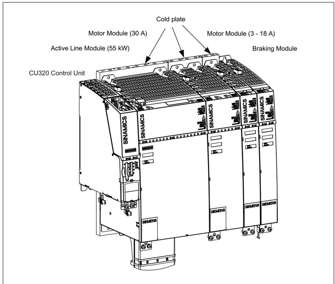
Figure 11-10 Example of a drive line-up with cold plate
