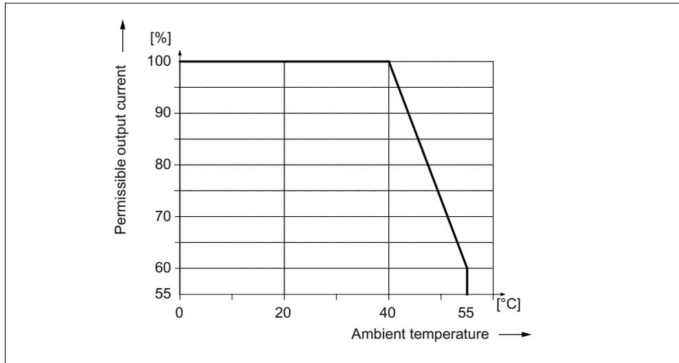
Figure 5-74 Output current as a function of the ambient temperature
