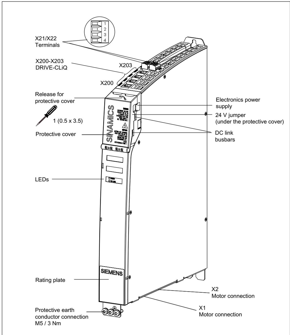
Figure 5-1 Example: Double Motor Module Booksize format with internal air cooling (2 x 3 A)
