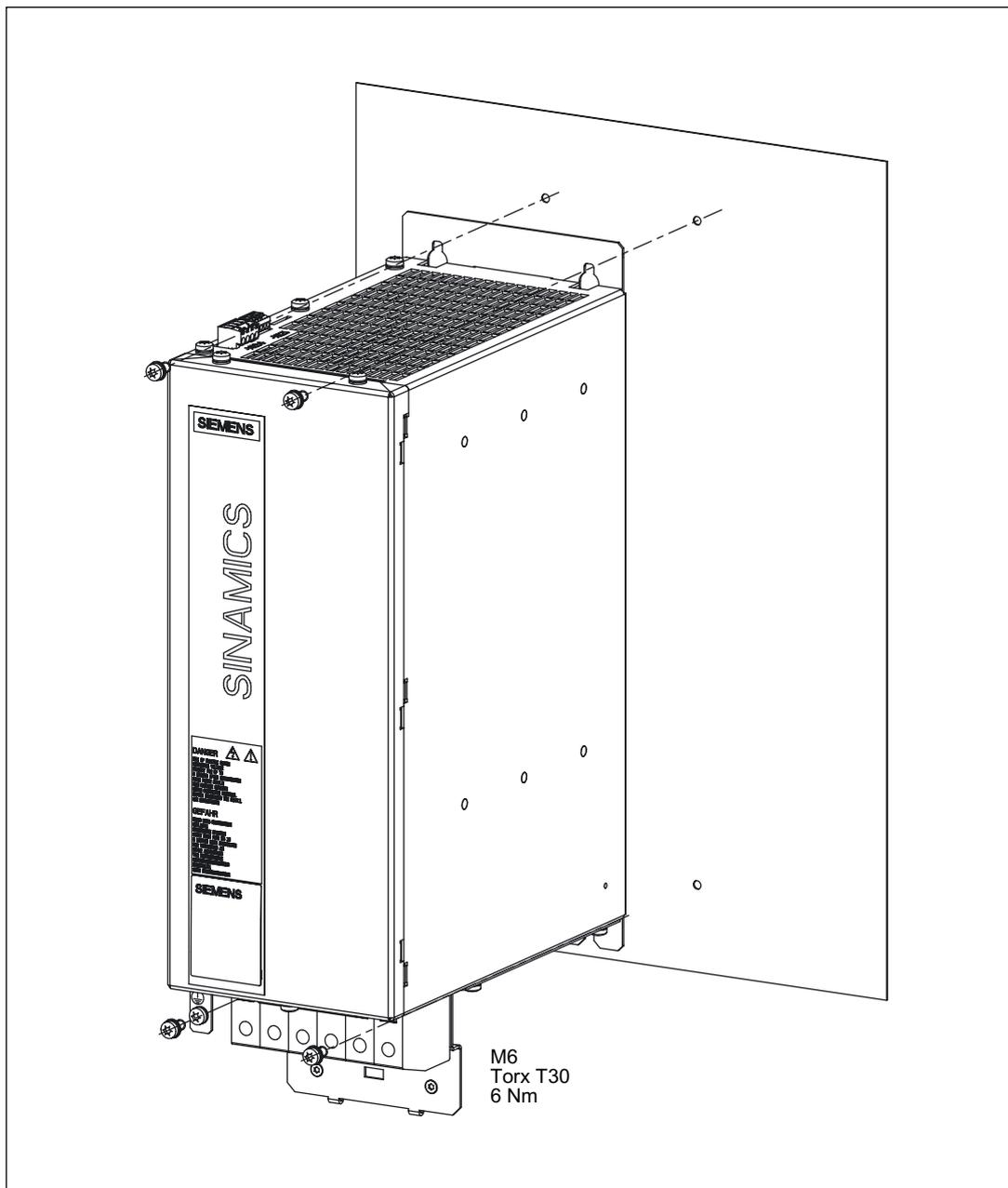
Figure 2-40 Mounting: Active Interface Module 36 kW
