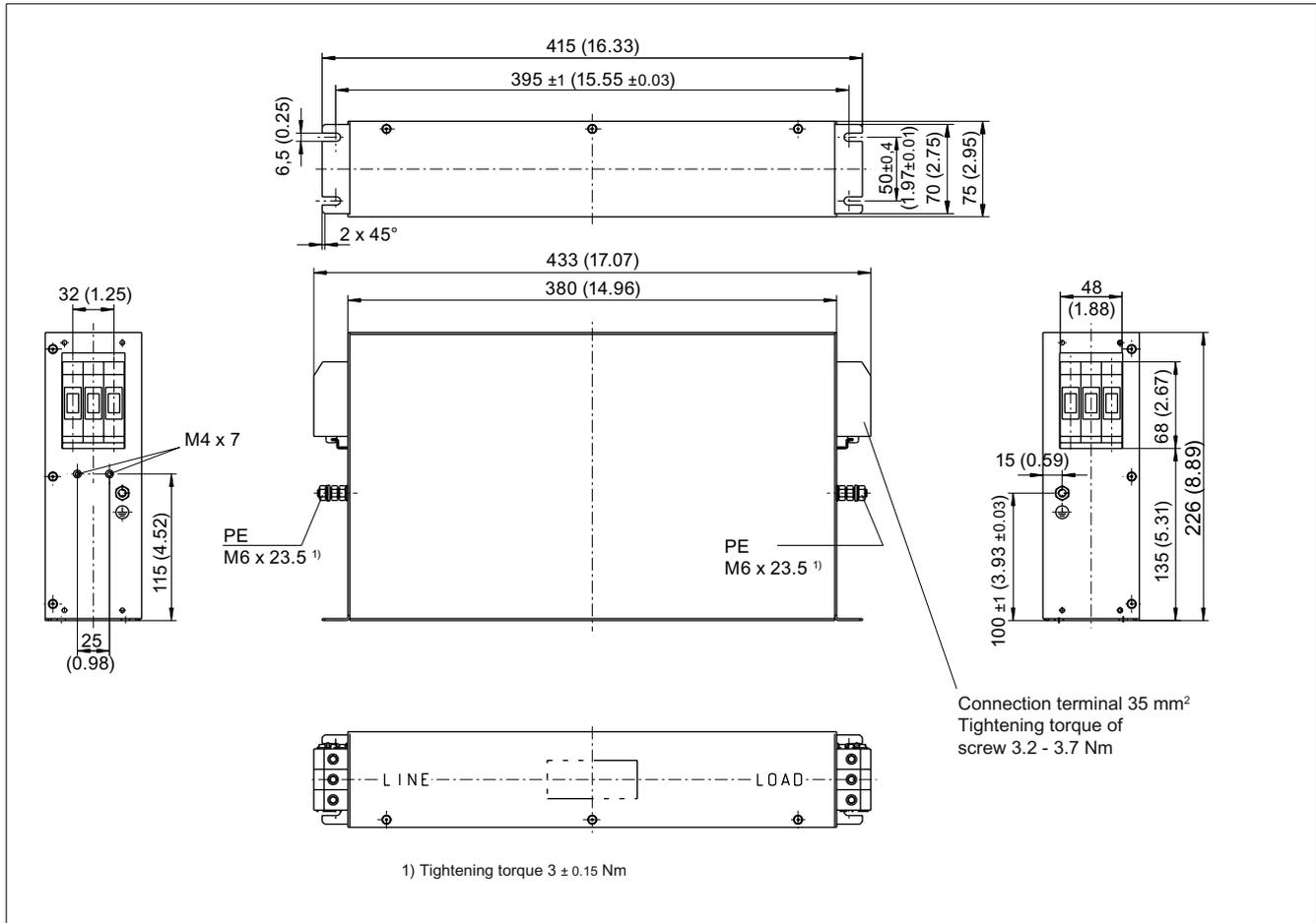
Figure 2-13 Dimension drawing of Basic Line Filter 36 kW, order number 6SL3000-0BE23-6DA1, all dimensions in mm and (inches)
