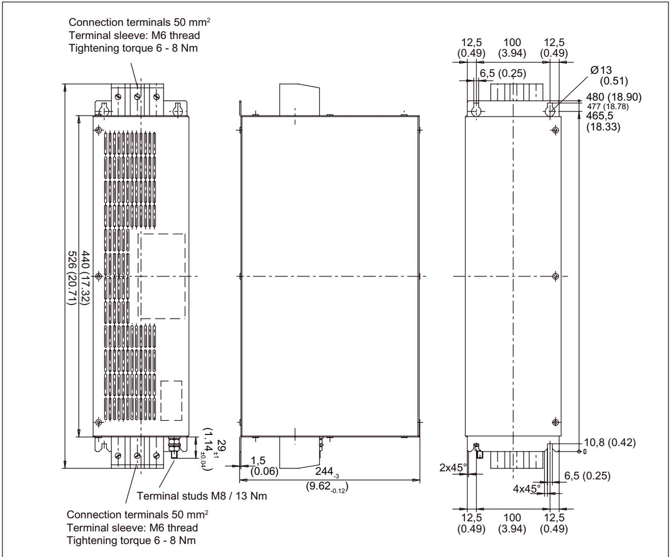
Figure 2-18 Dimension drawing of Wideband Line Filter 36 kW for Active Lines Modules, all dimensions in mm and (inches)
