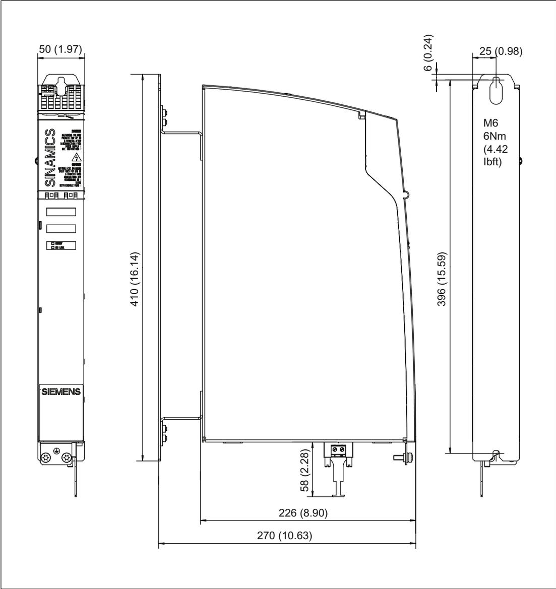
Figure 8-3 Dimension drawing of Braking Module, all dimensions in mm and (inches)
