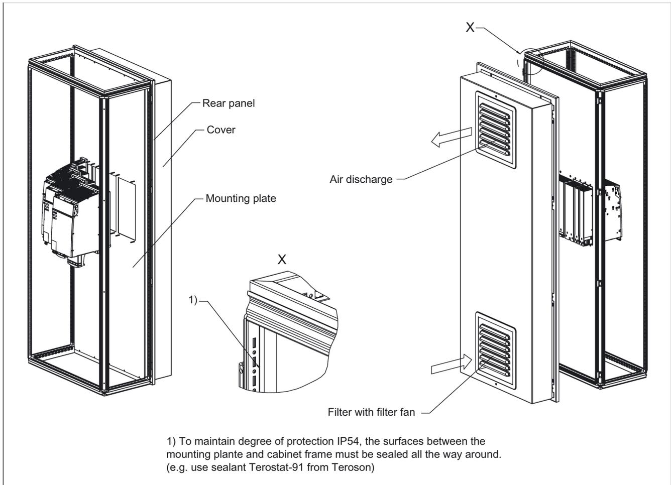
Figure 3-108 Example 1: installation in cabinet with mounting plate
