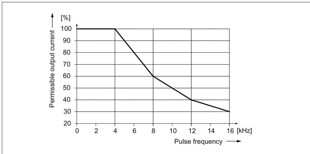
Figure 5-16 Output current as a function of the pulse frequency
