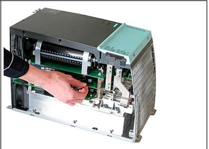
Pull the first fan cable by pressing it slightly
