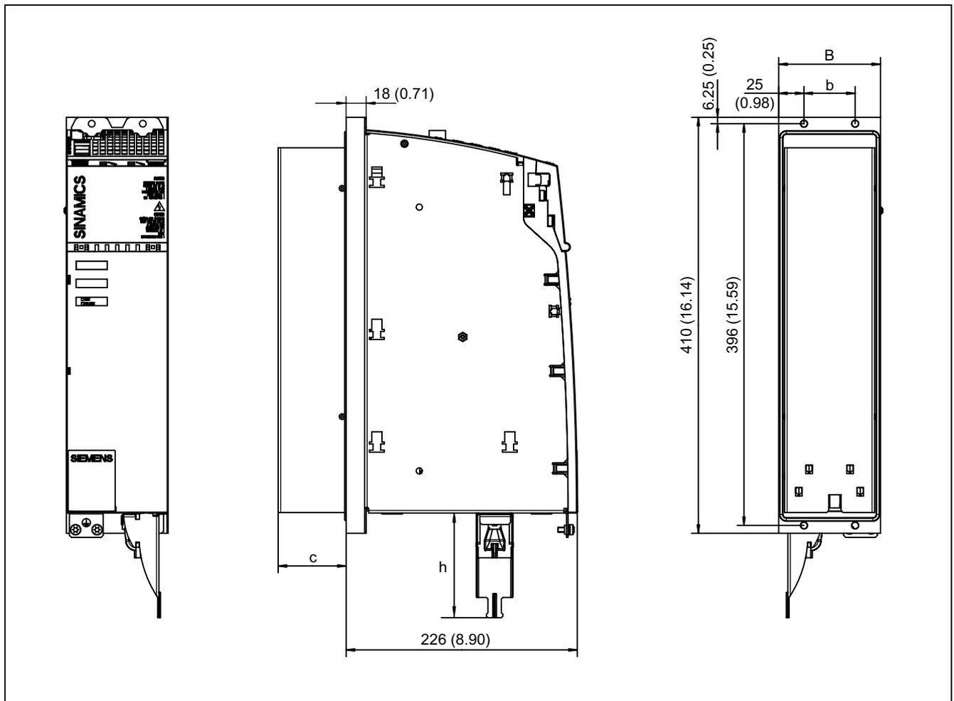
Figure 5-24 Dimension drawing of Motor Modules with external air cooling 30 A and 2 x 18 A, all dimensions in mm and (inches)
