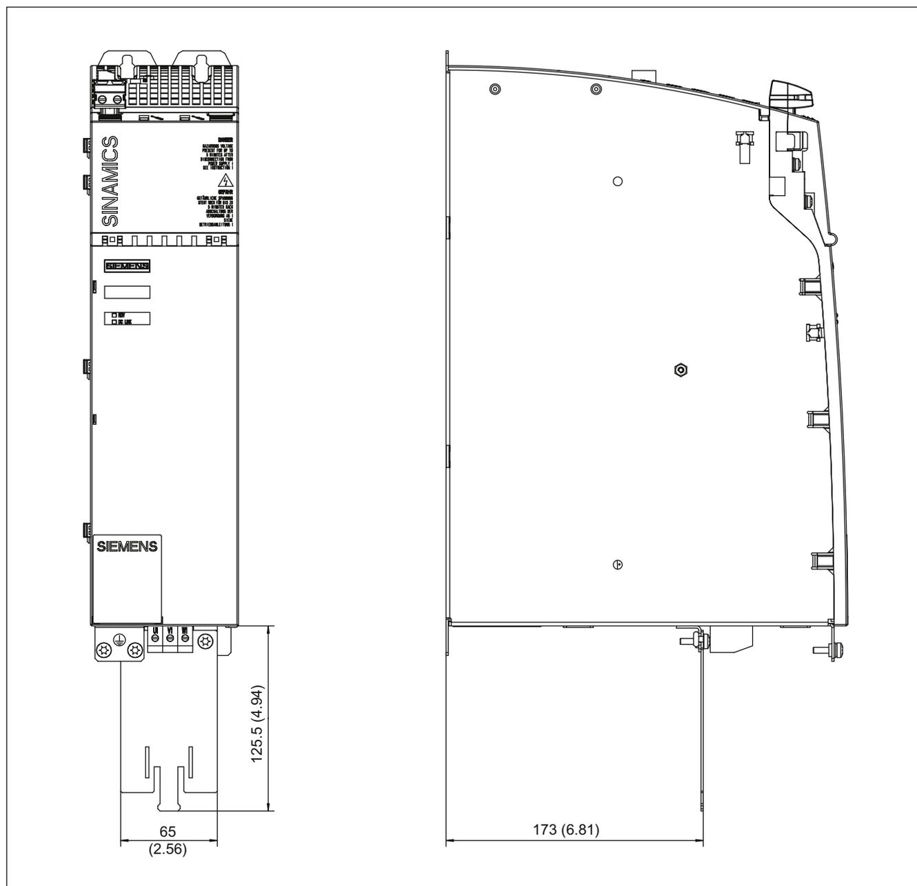
Figure 10-5 Dimension drawing of shield connecting plate on a 100 mm component with internal air cooling, all dimensions in mm and (inches)
