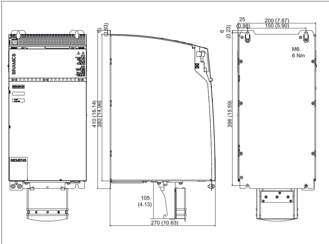
Figure 3-57 Dimension drawing of Basic Line Module 100 kW with internal air cooling, all dimensions in mm and (inches)
