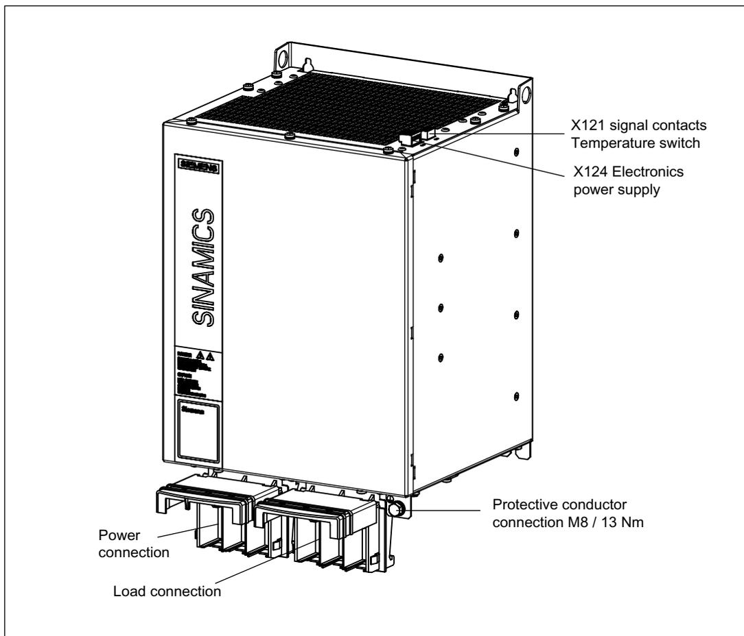
Figure 2-33 Interface description: Active Interface Module (80 kW and 120 kW)
