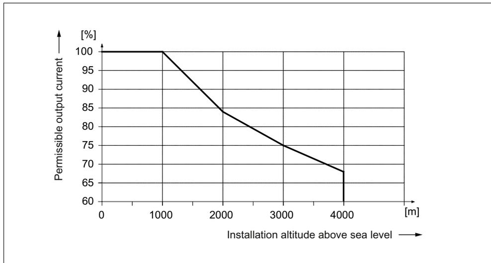
Figure 5-62 Output current as a function of the installation altitude
