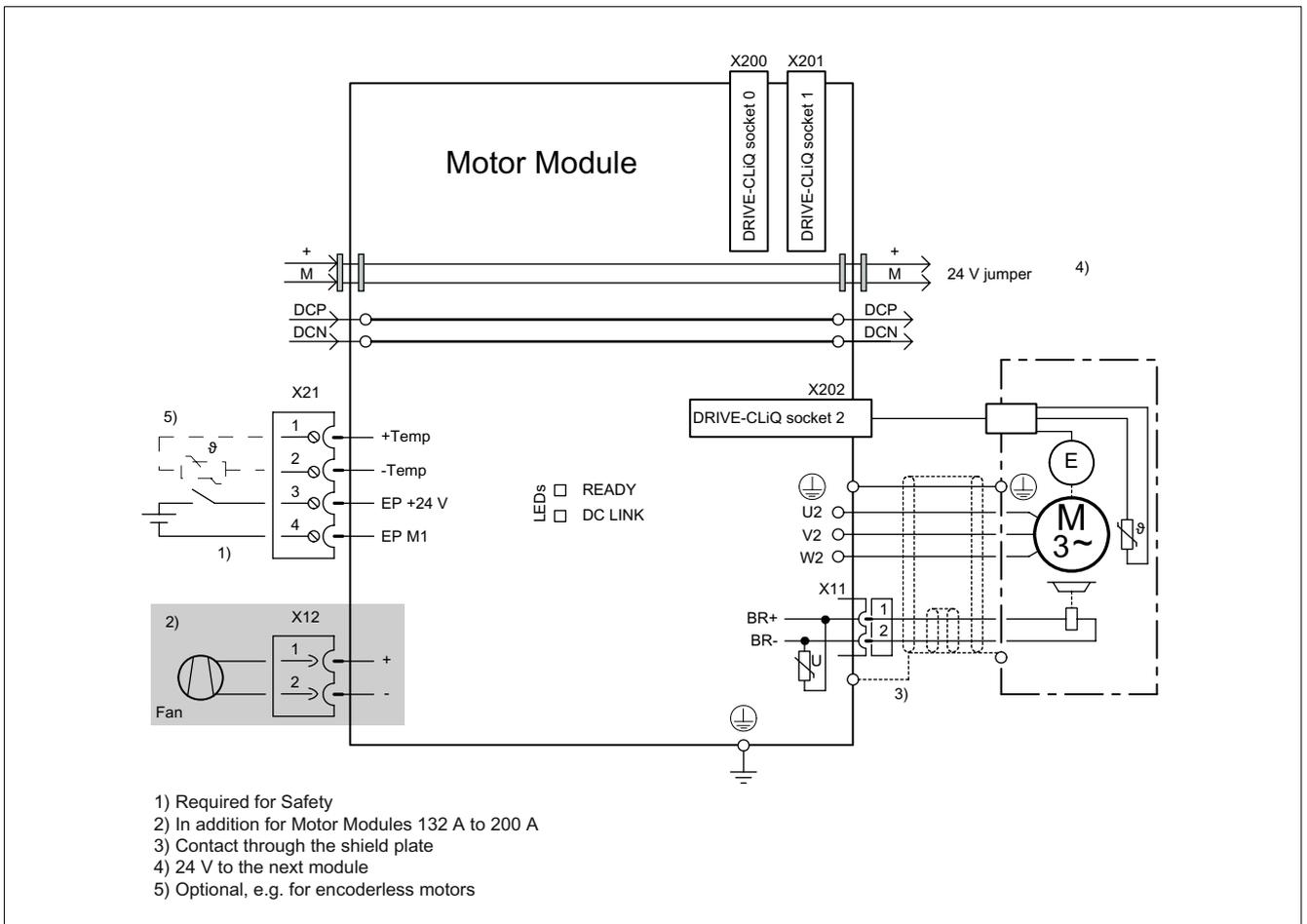
Figure 5-22 Example connection of Single Motor Modules 45 A to 200 A
