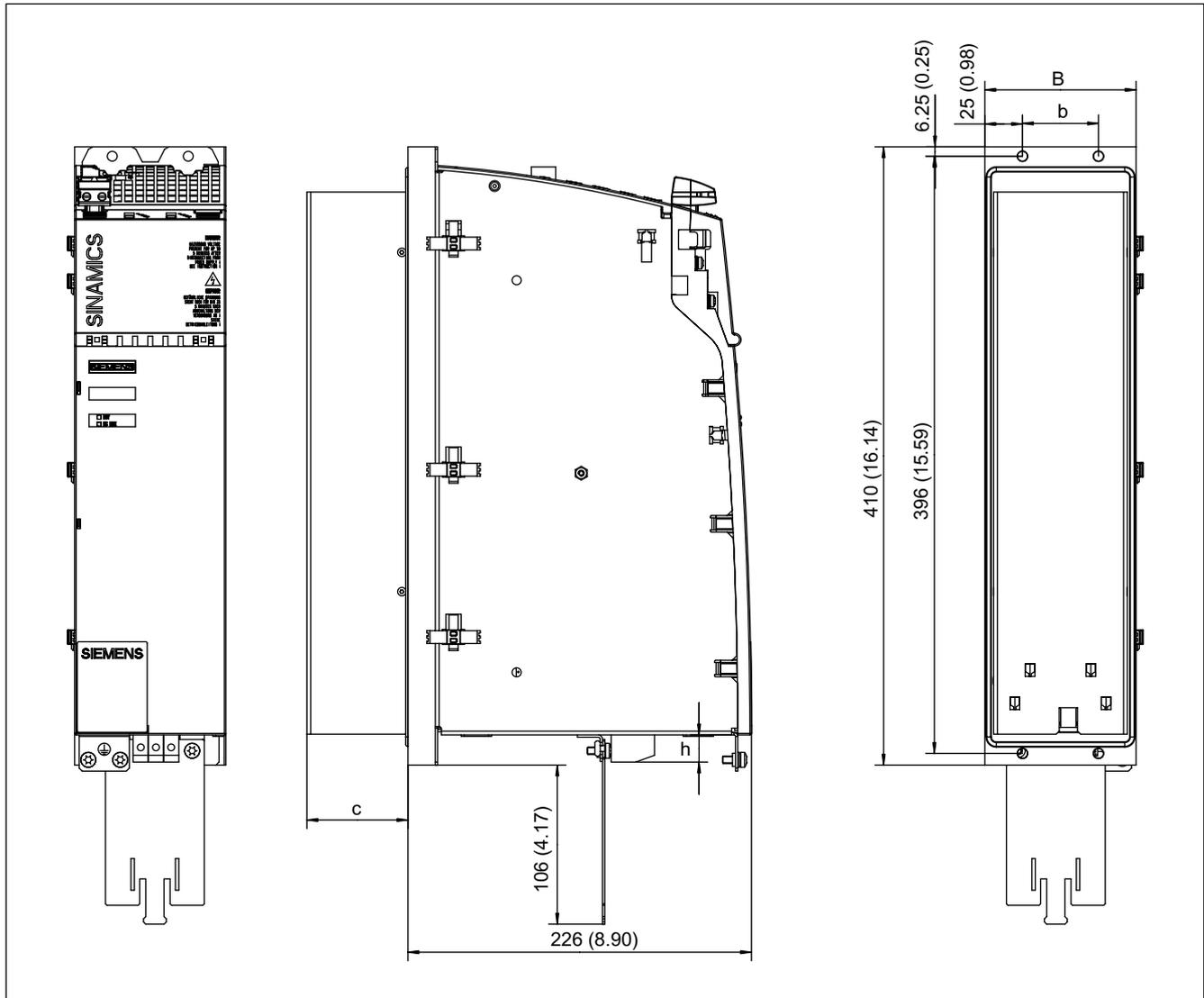
Figure 3-16 Dimension drawing of Active Line Module 16 kW with external air cooling, all data in mm and (inches)
