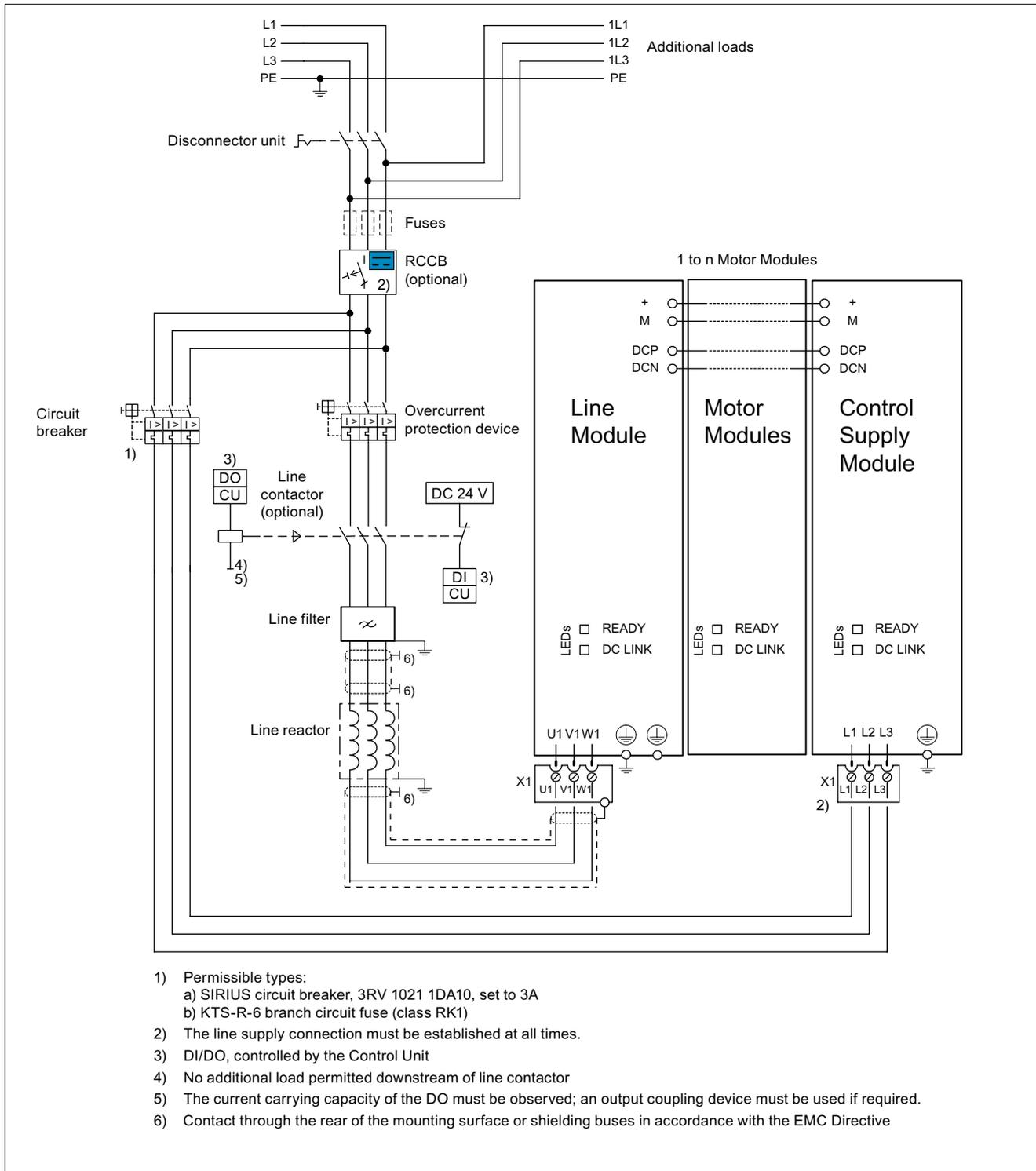
Figure 8-12 Example connection of Control Supply Module
