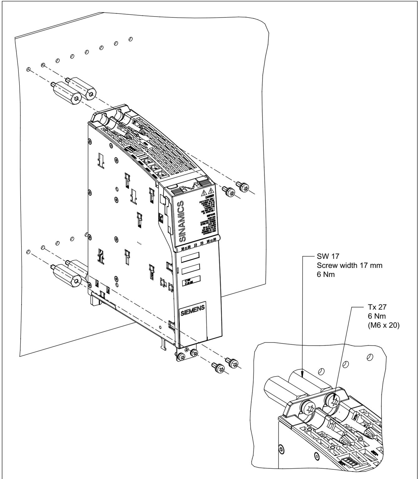
Figure 10-34 Installation of the spacing bolts on a booksize compact format component (example: Motor Module booksize compact, 18 A)
