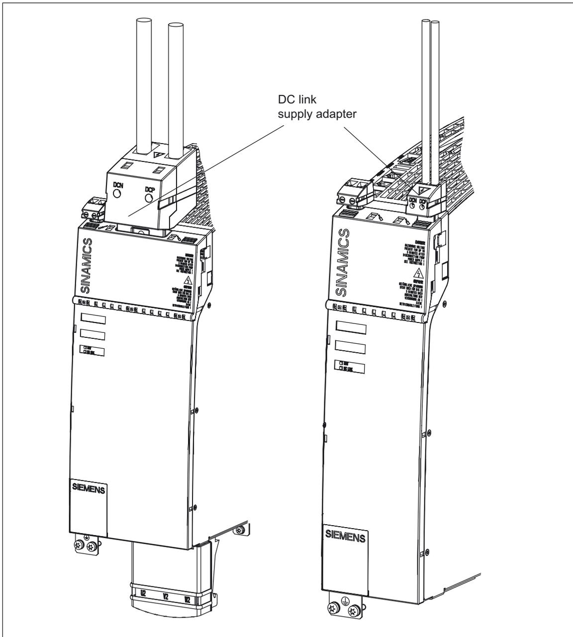
Figure 10-20 150 mm components with DC link rectifier adapter for 35 mm<sup>2</sup> to 95 mm<sup>2</sup> and 100 mm components with DC link rectifier adapter for 0.5 mm<sup>2</sup> to 10 mm<sup>2</sup>
