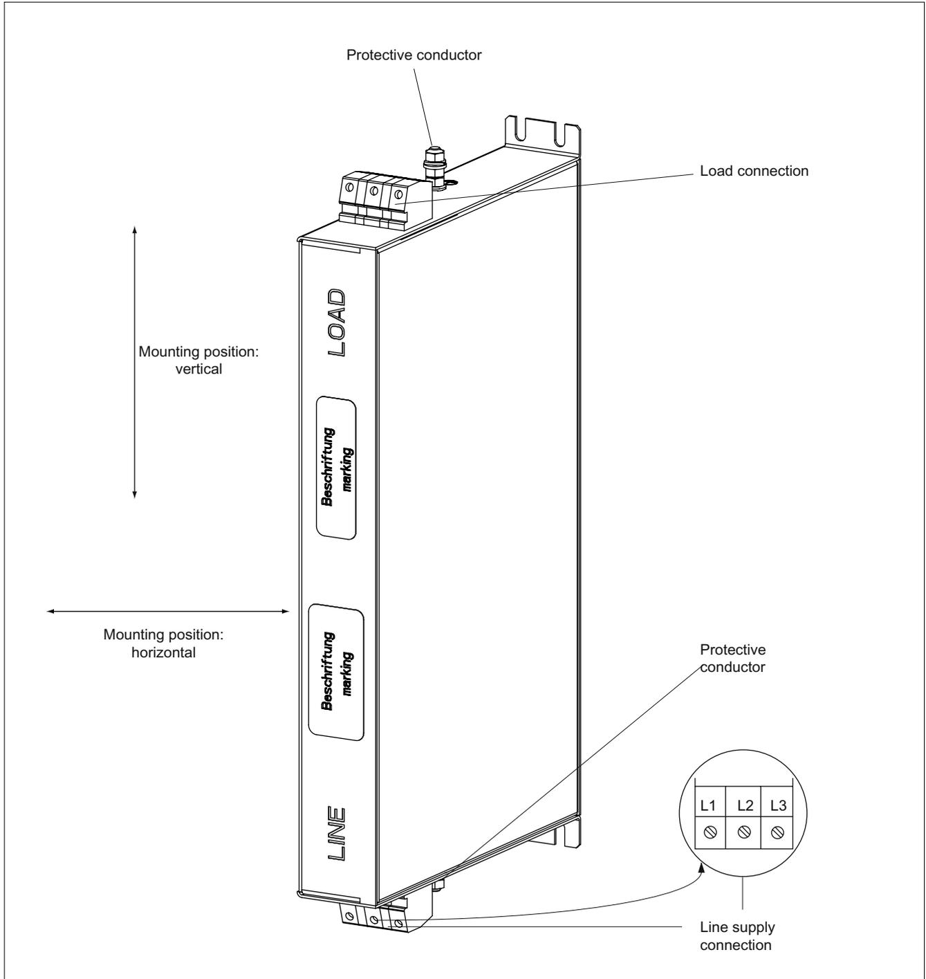
Figure 2-8 Basic Line Filter for Active Line Modules with Active Interface Module 16 kW
