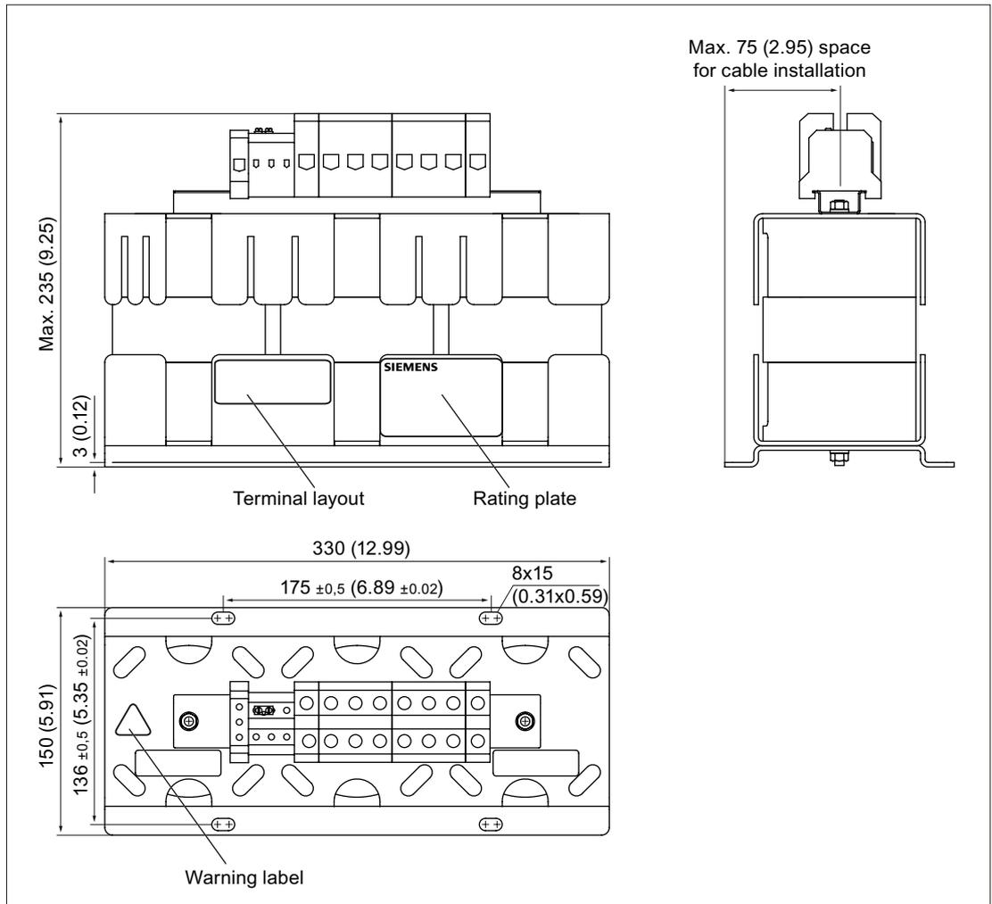
Figure 2-51 Dimension drawing of HFD line reactor 36 kW, all dimensions in mm and (inches)
