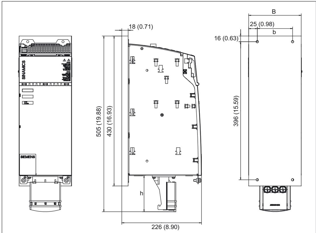
Figure 5-50 Dimension drawing of Motor Module with cold plate 45 A, 60 A, and 85 A, all dimensions in mm and (inches)
