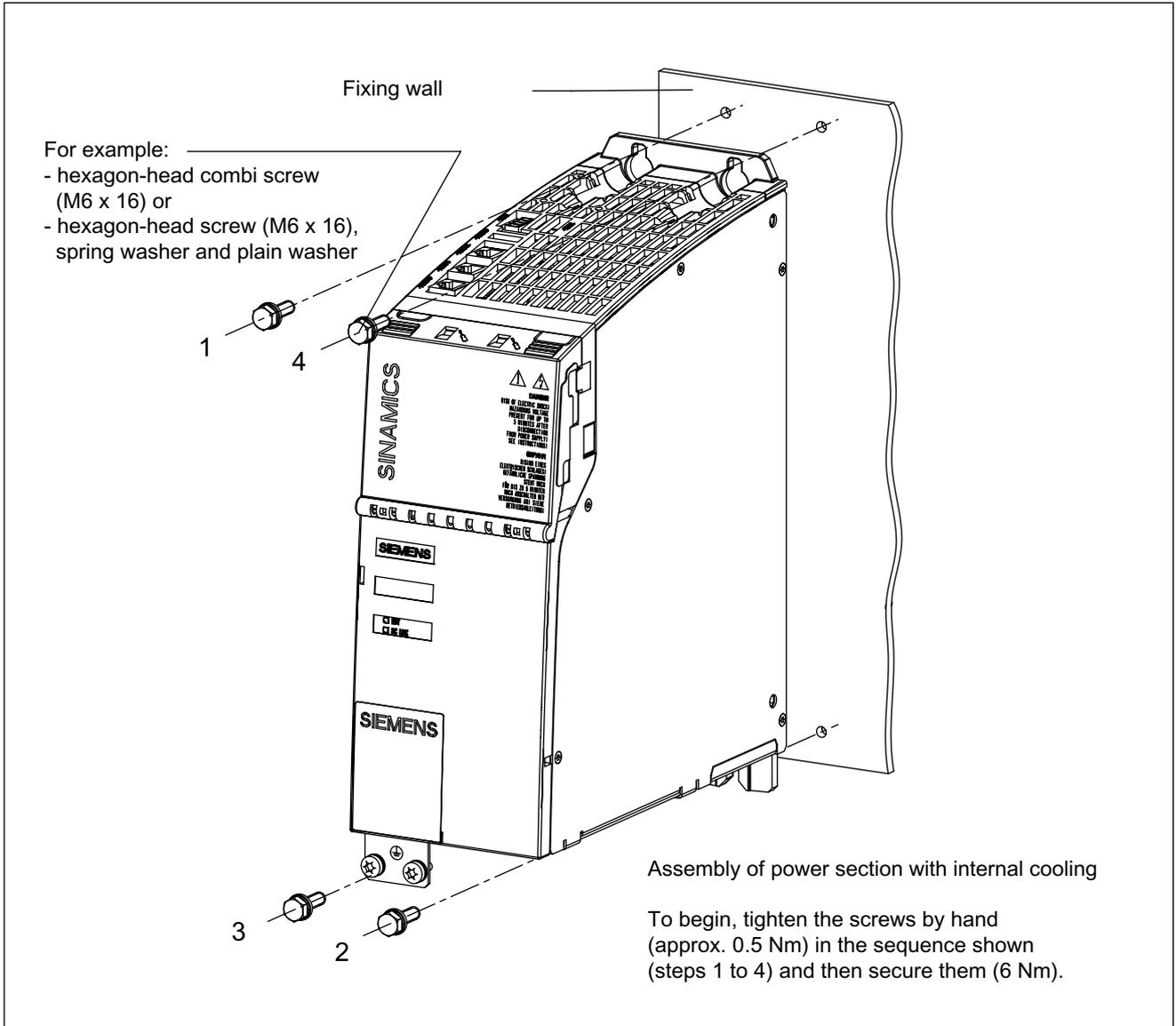
Figure 4-4 Installation: Smart Line Module Booksize Compact 16 kW with internal cooling
