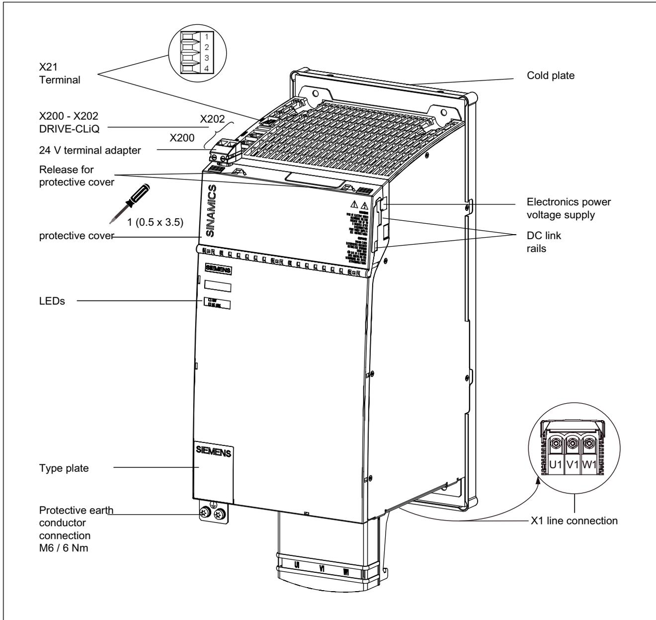
Figure 3-73 Basic Line Module with cold plate (100 kW)
