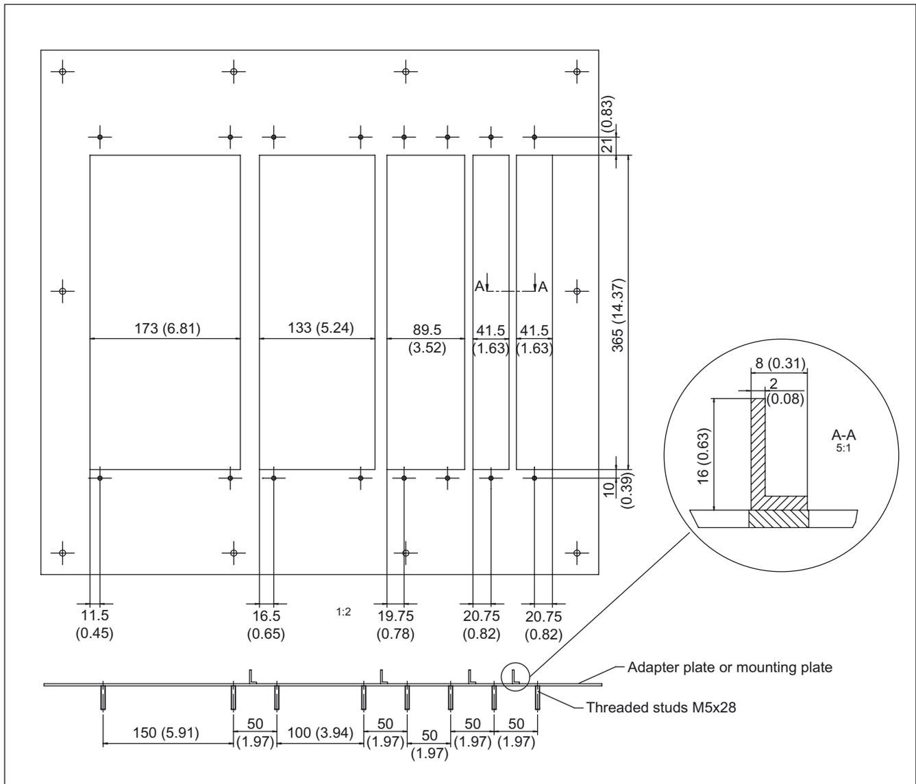
Figure 5-31 Example: mounting plate with a drive line-up
