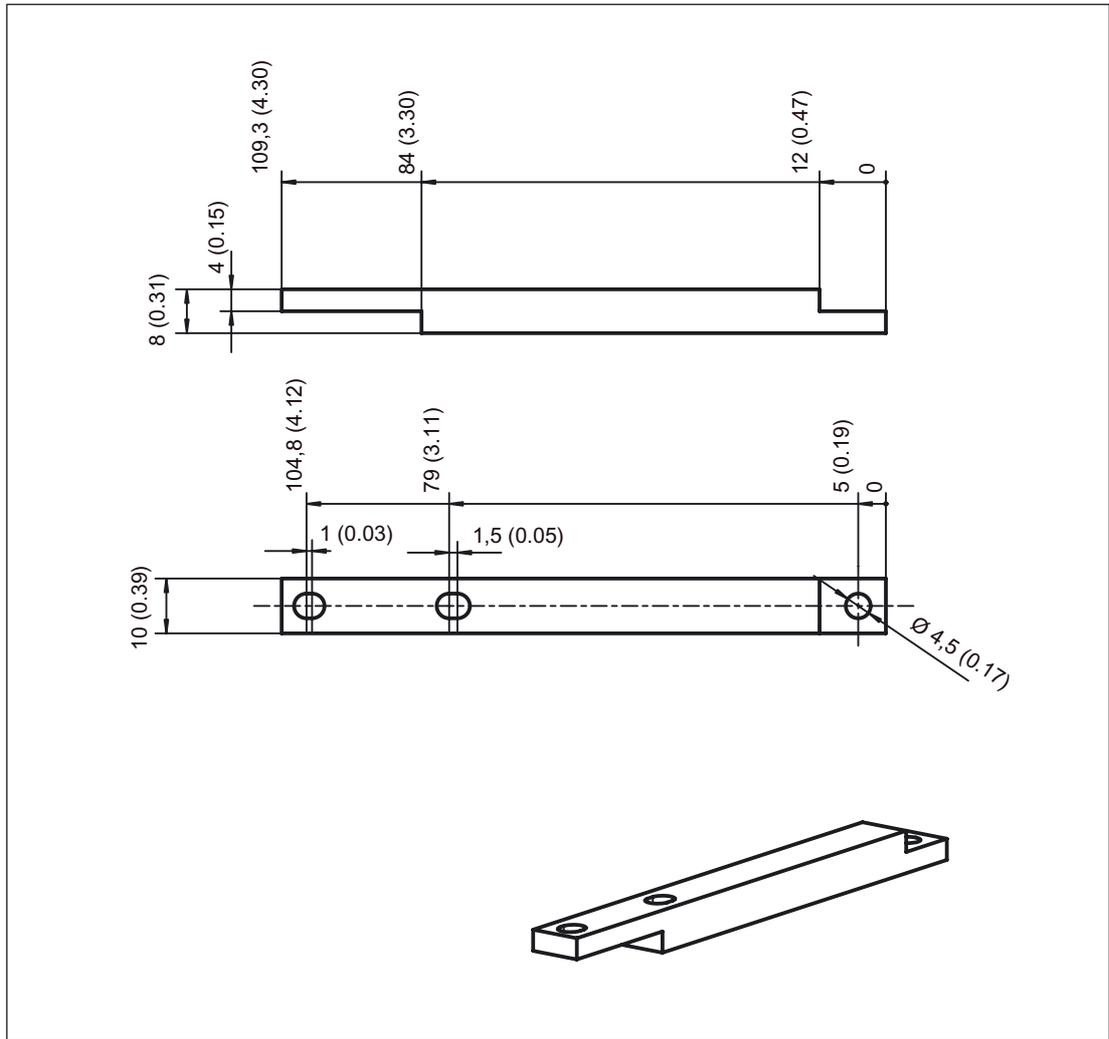
Figure 10-26 Dimension drawing of reinforced DC-link busbar 100 mm, all dimensions in mm and (inches)
