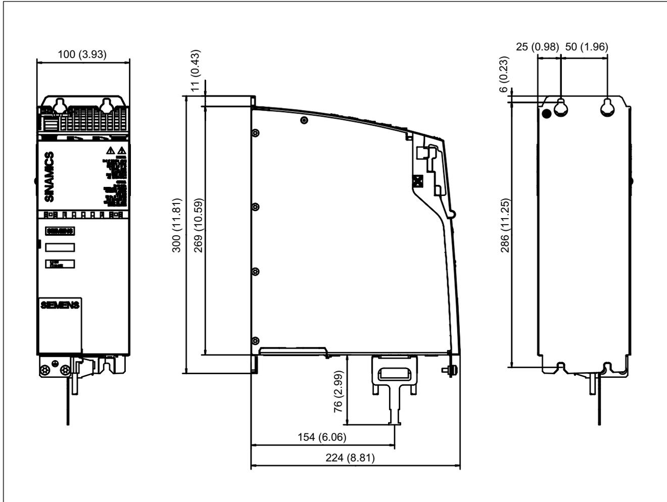
Figure 4-3 Dimension drawing Smart Line Module Booksize Compact format (16 kW), all dimensions in mm and (inches)
