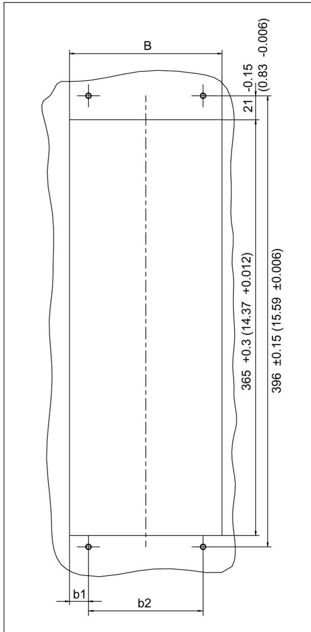
Figure 3-19 Installation openings for the power unit with external air cooling, 50 mm to 200 mm
