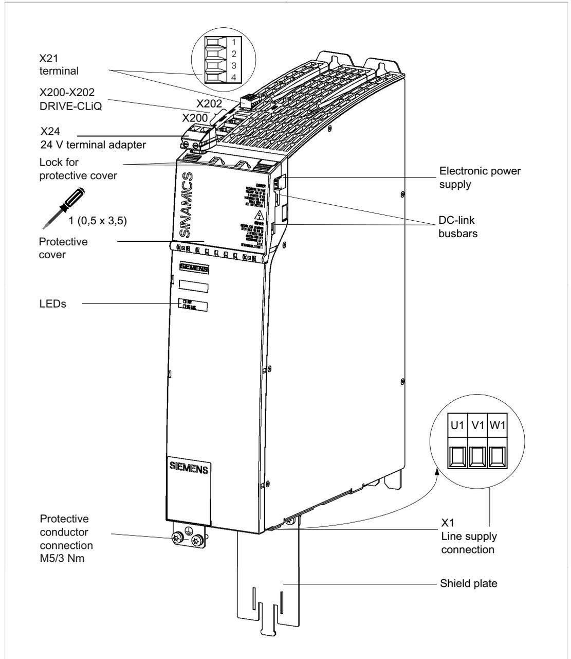
Figure 3-91 Smart Line Module with internal air cooling (16 kW)
