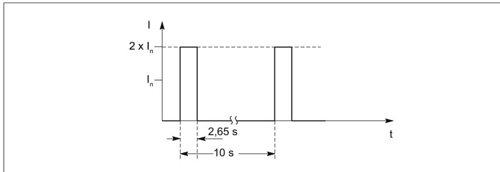
Figure 6-11 Duty cycle without initial load
