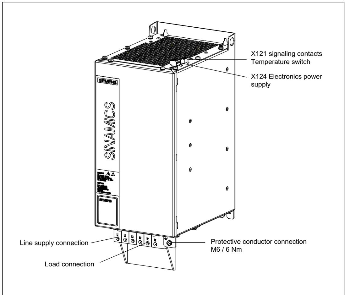
Figure 2-32 Interface description: Active Interface Module 55 kW
