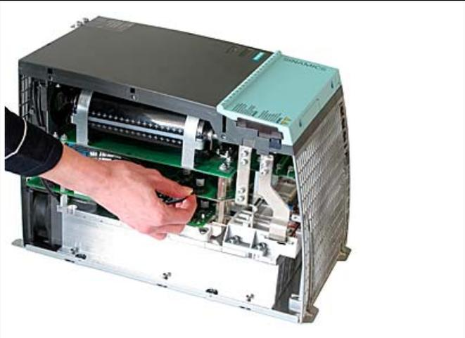
Pull the first fan cable by pressing it slightly
