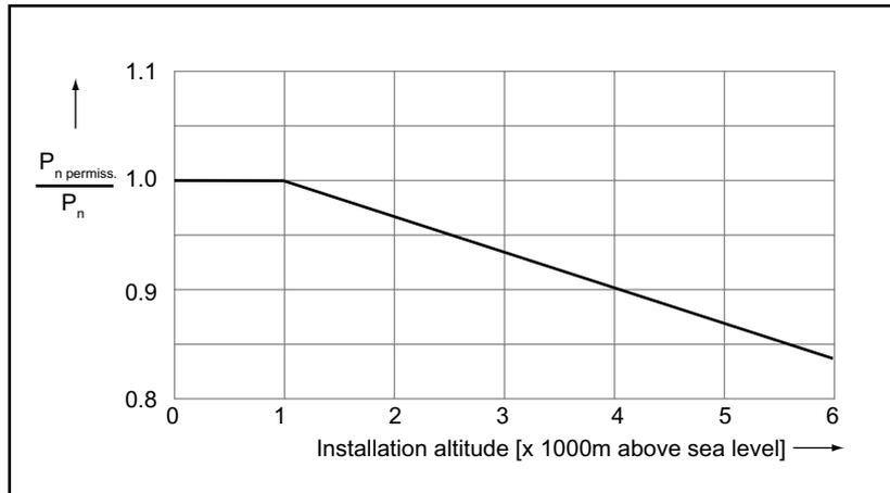
Figure 2-77 Load characteristics in relation to the installation altitude
