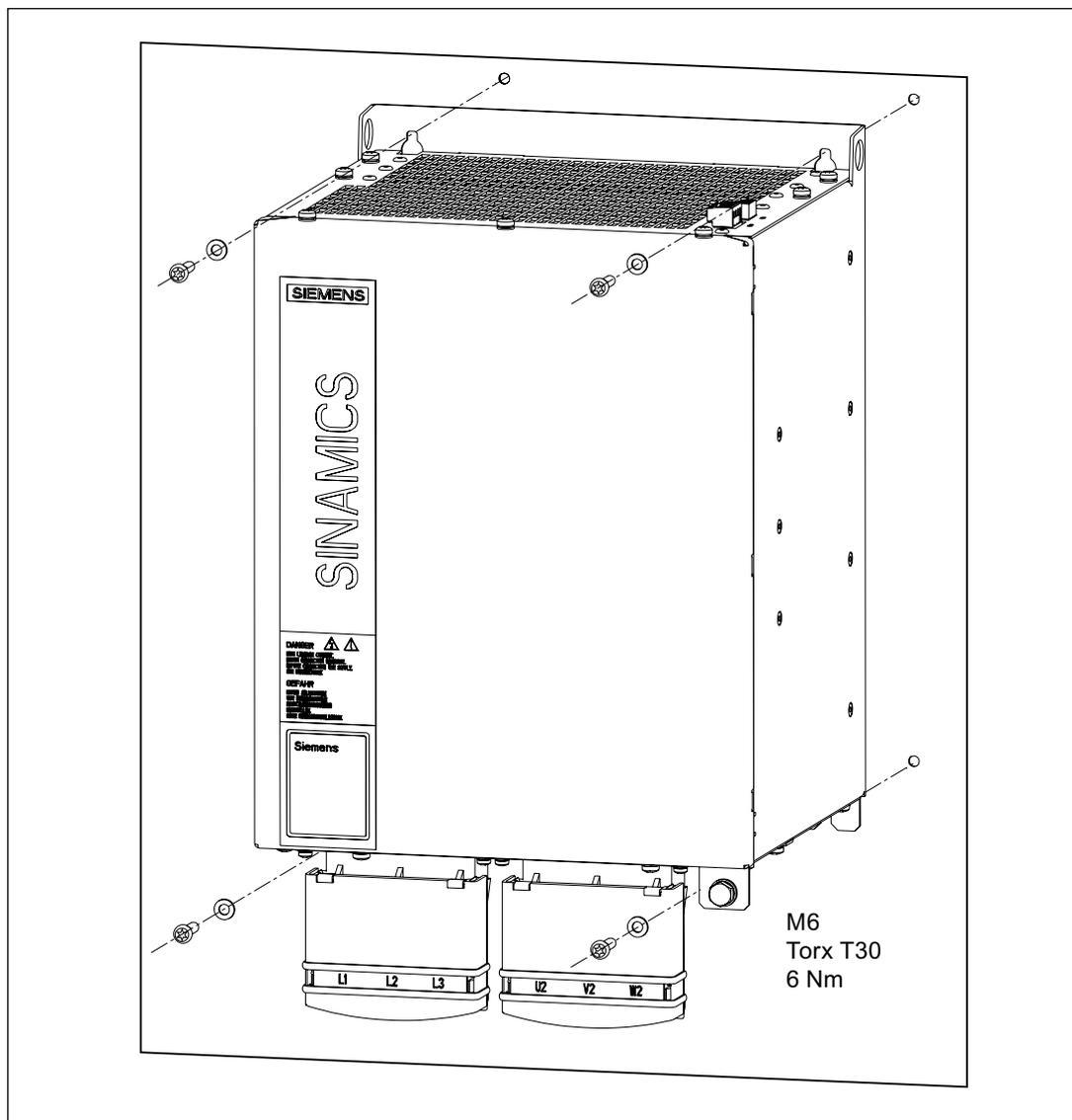
Figure 2-41 Mounting: Active Interface Module 55 kW
