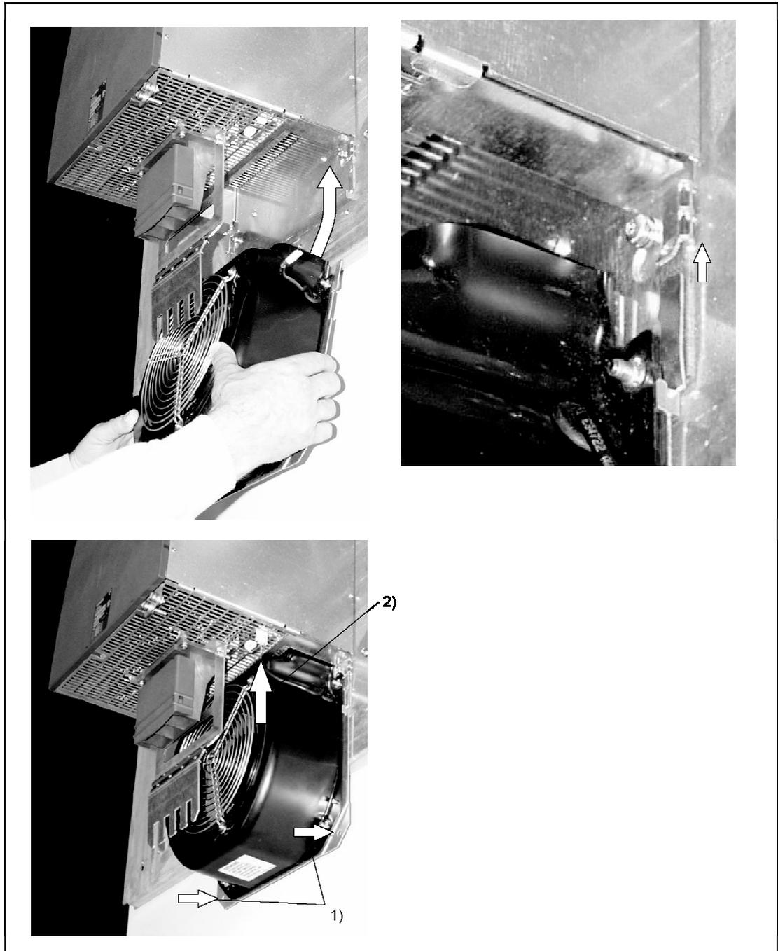
Figure 3-7 Installing the fan for 300 mm modules
