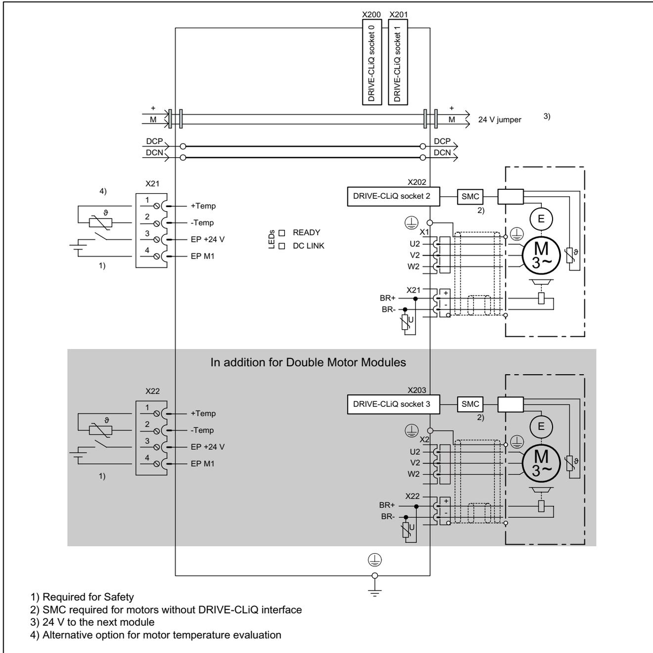
Figure 6-4 Connection example: Single Motor Module Booksize Compact 3 A to 18 A and Double Motor Module Booksize Compact 1.7 A to 5 A
