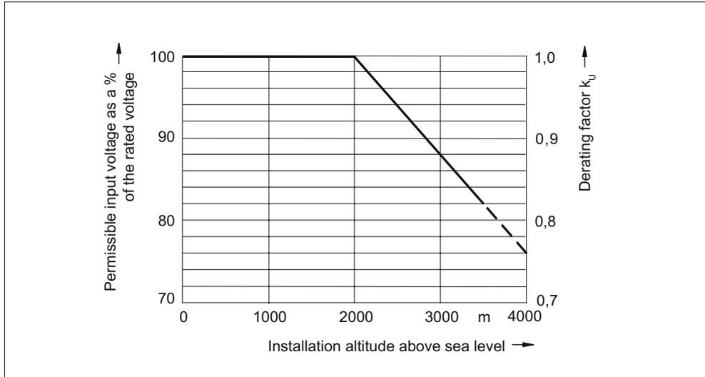
Figure 3-40 Voltage derating as a function of the installation altitude
