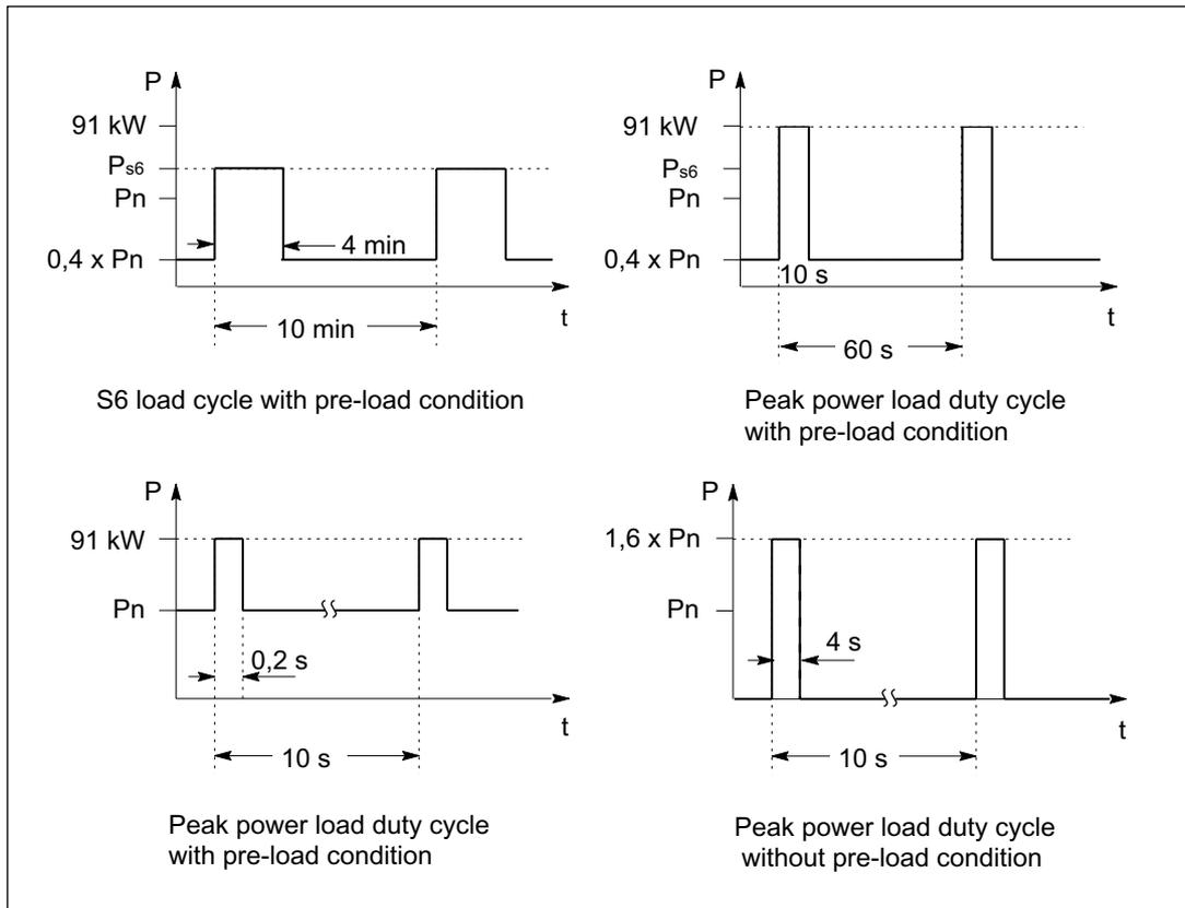
Figure 3-9 Rated duty cycles of 55 kW Active Line Modules with Active Interface Module
