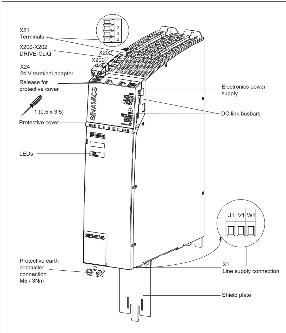
Figure 3-1 Active Line Module with internal air cooling (example: 16 kW)
