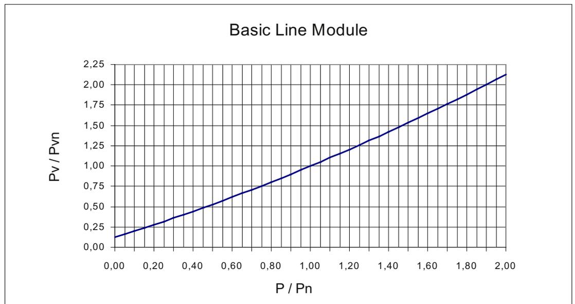
Figure 11-39 Losses in the partial load range for Basic Line Modules
