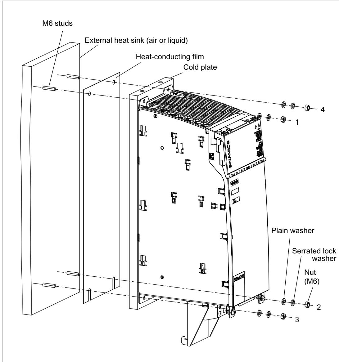
Figure 3-79 Installation of Basic Line Module 40 kW with external heat sink and heat-conducting film
