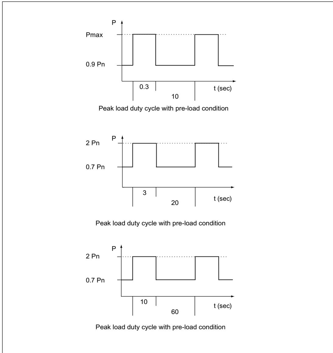
Figure 3-81 Rated duty cycles of 20 kW and 40 kW Basic Line Modules
