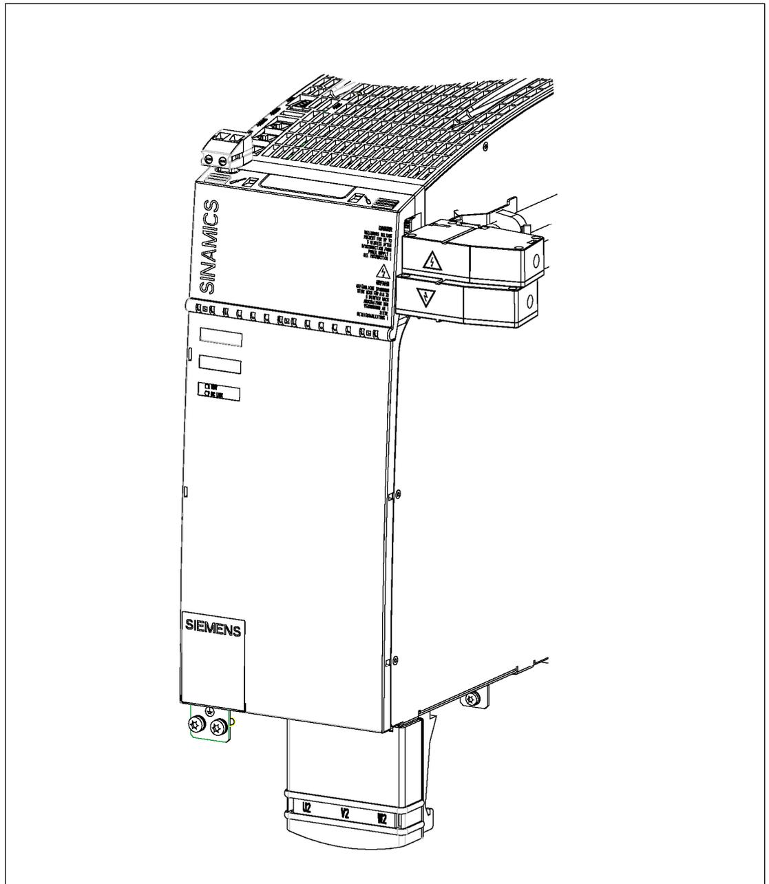
Figure 10-23 150 mm components with DC link adapter for two-row configuration 35 mm<sup>2</sup> to 95 mm<sup>2</sup>
