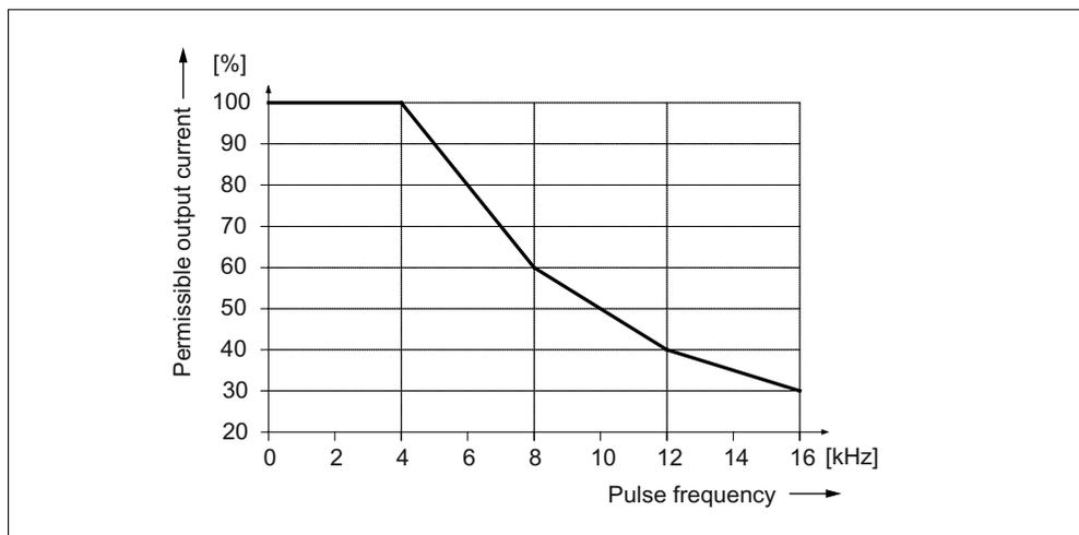
Figure 5-41 Output current as a function of the pulse frequency
