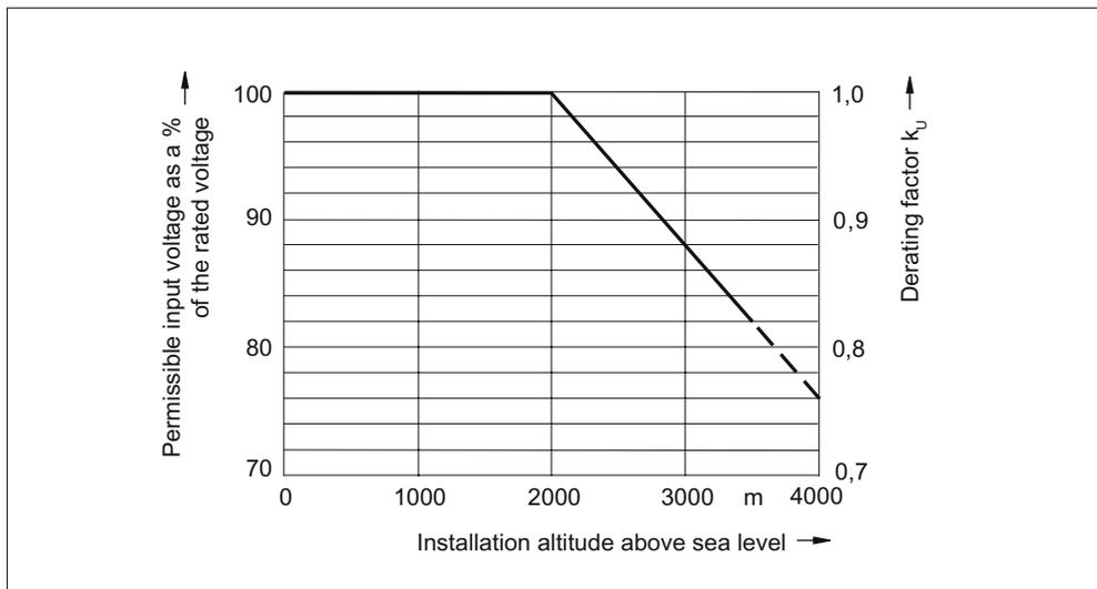
Figure 3-49 Voltage derating as a function of the installation altitude
