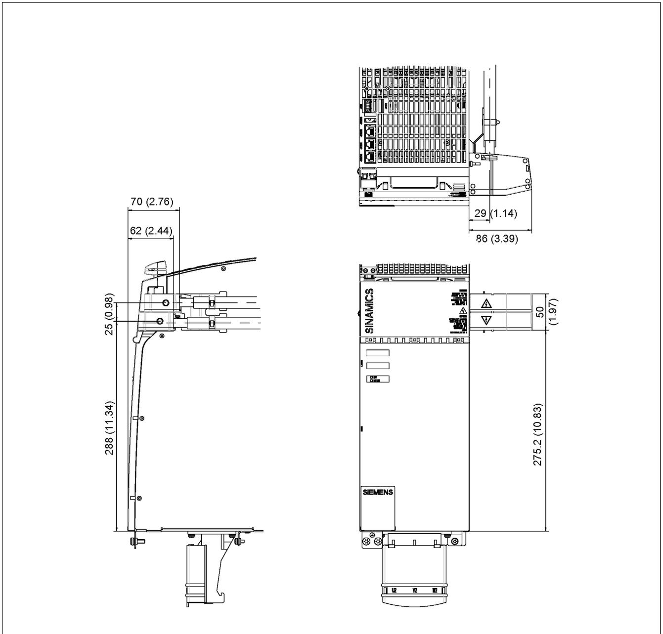
Figure 10-24 Dimension drawing of 150 mm component with DC link rectifier adapter for 35 mm<sup>2</sup> to 95 mm<sup>2</sup>, all dimensions in mm and (inches)
