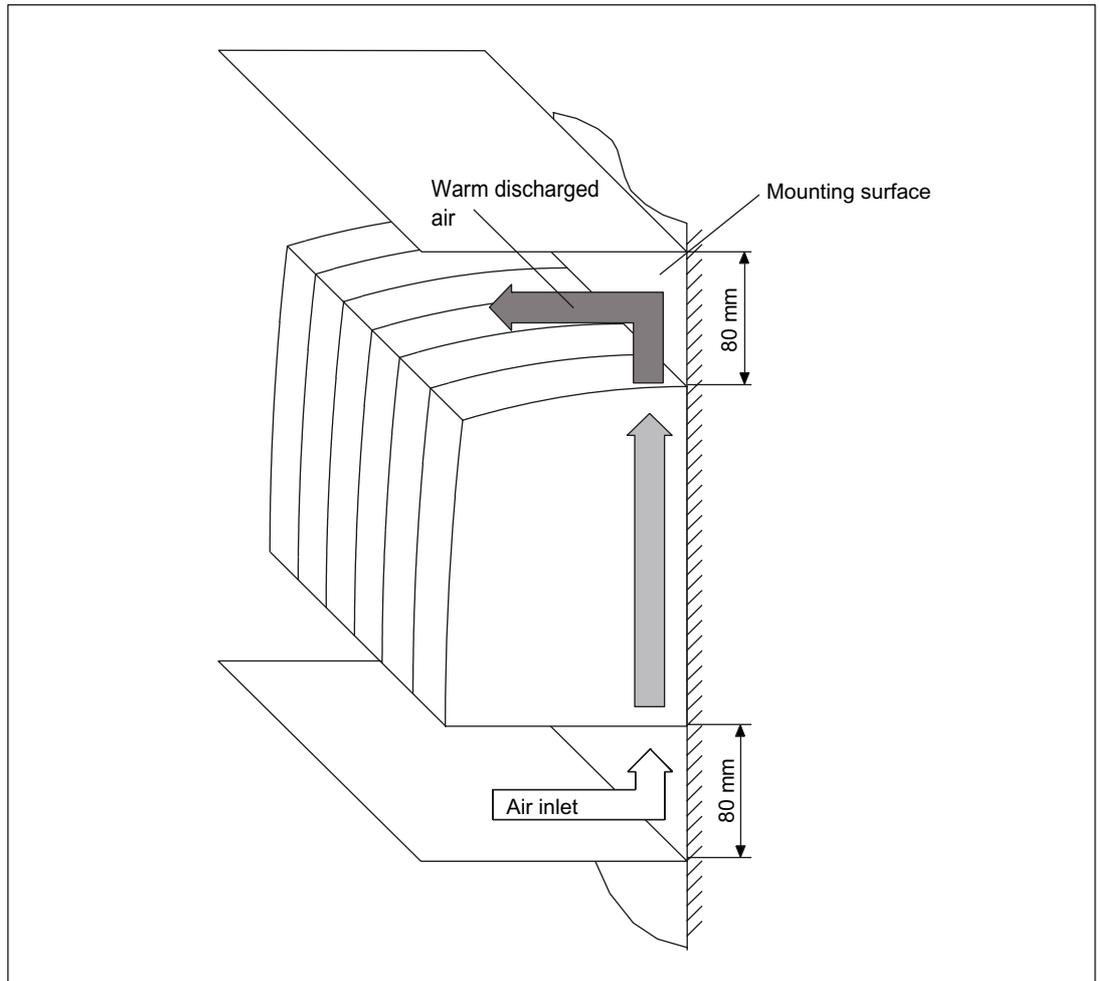
Figure 11-32 Clearances for booksize drive line-up with internal air cooling
