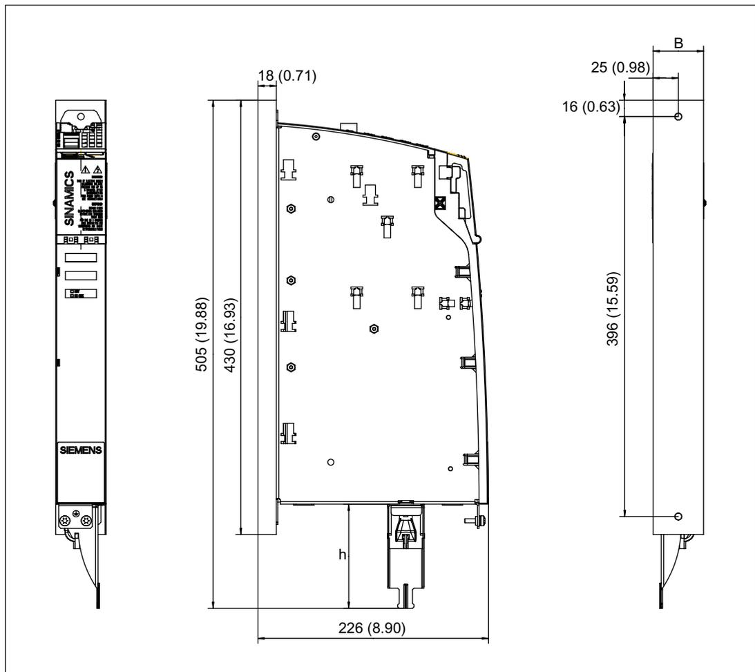
Figure 5-48 Dimension drawing of Motor Module with cold plate 3 A to 18 A and 2 x 3 A to 2 x 9 A, all dimensions in mm and (inches)
