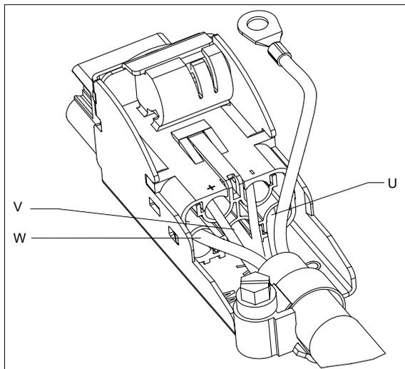
Figure 11-21 Crimp version motor connection plug with locking mechanism
