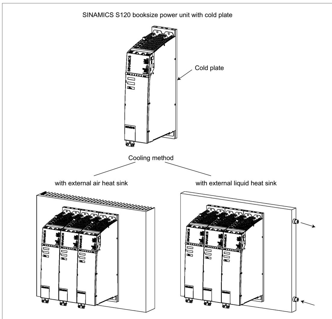
Figure 11-27 Overview of cold plate cooling methods
