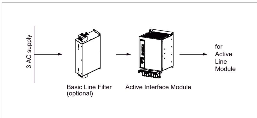
Figure 2-2 Overview: line connection with Active Interface Module
