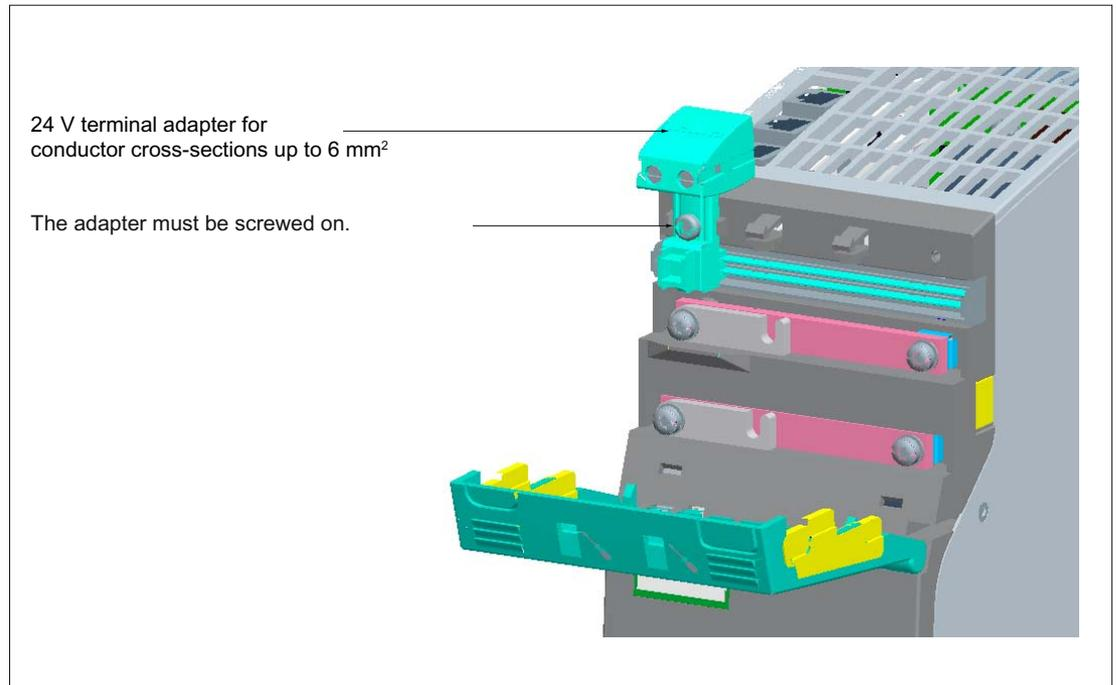
Figure 7-2 24 V terminal adapter
