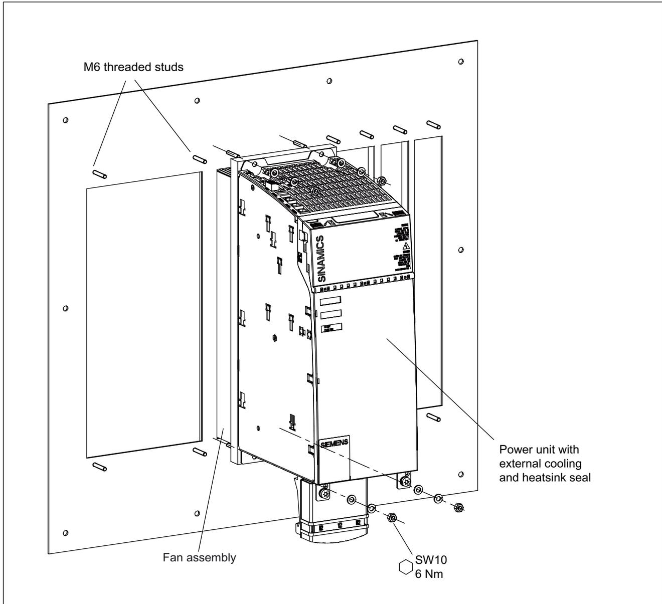
Figure 3-18 Example: Installation of the power unit with external air cooling
