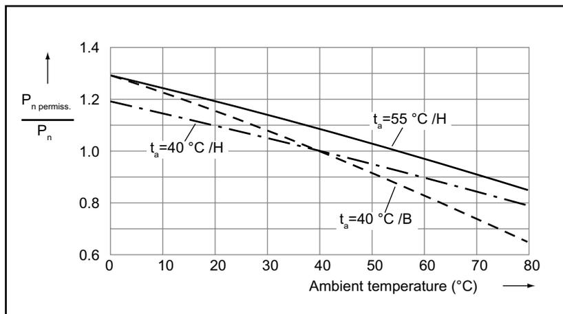
Figure 2-76 Load characteristics in relation to the ambient temperature
