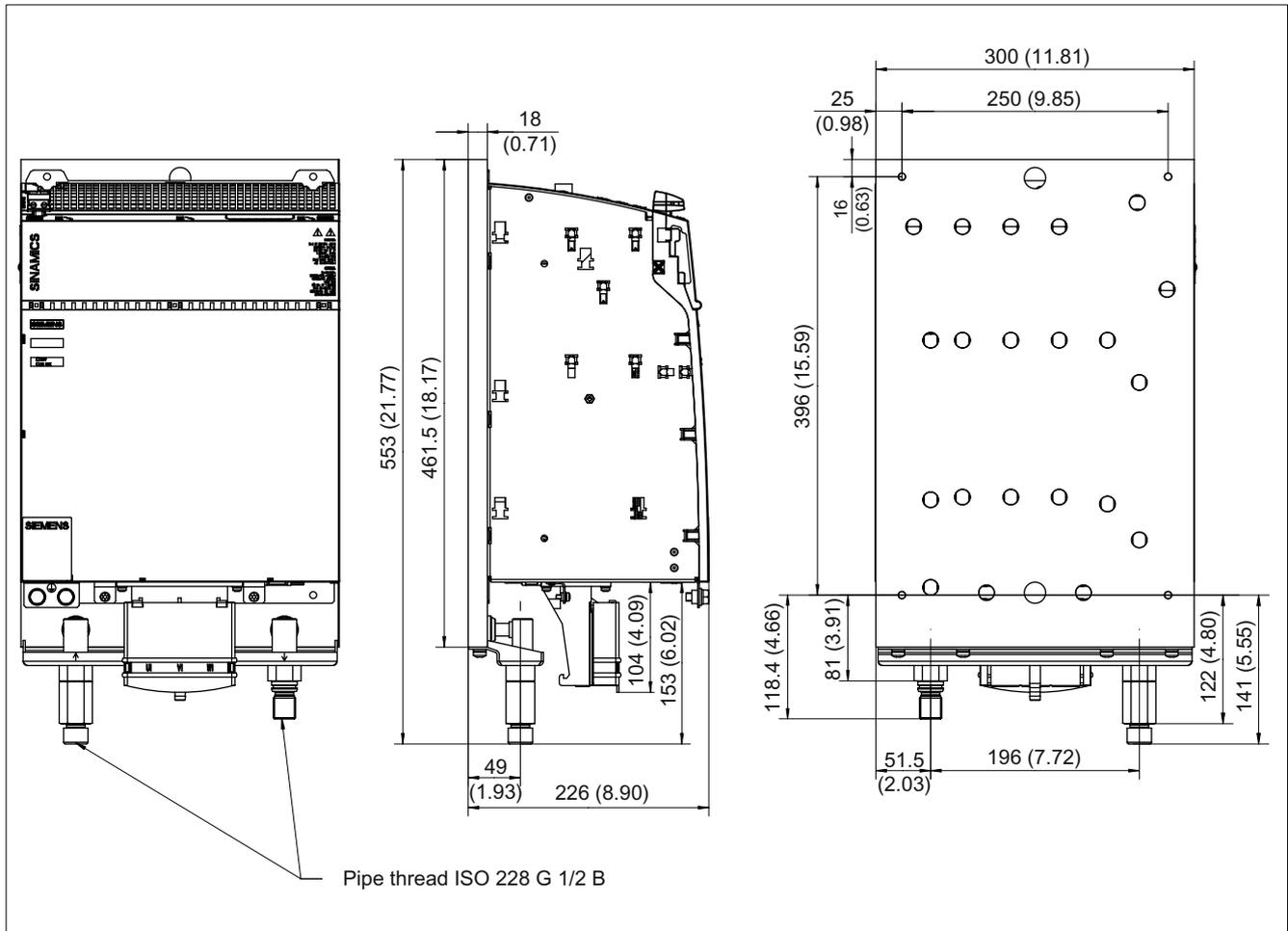
Figure 3-43 Dimension drawing of Active Line Module Liquid Cooled 120 kW, all dimensions in mm and (inches)
