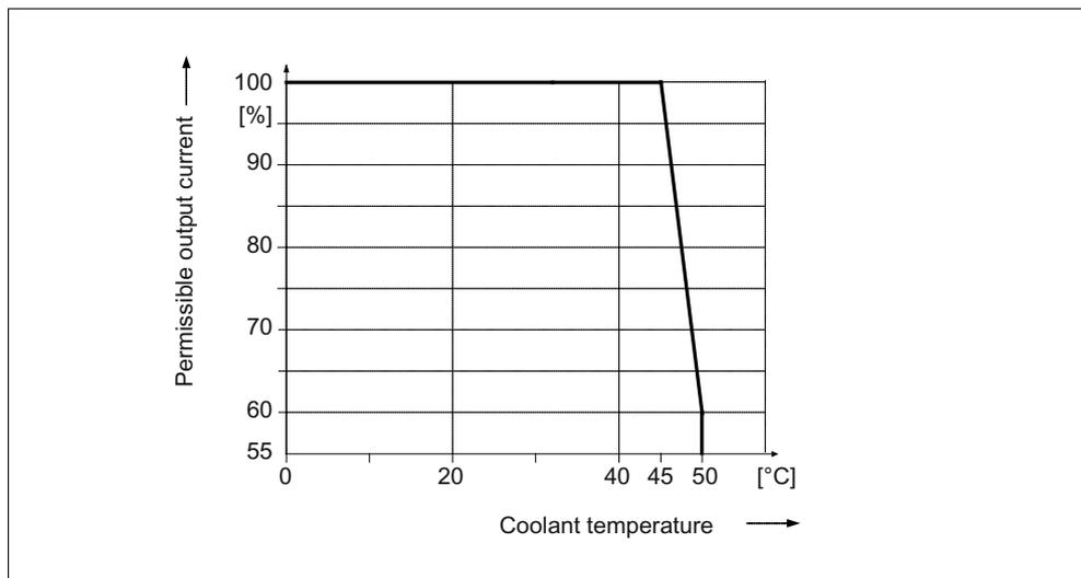
Figure 5-75 Output current as a function of the coolant temperature
