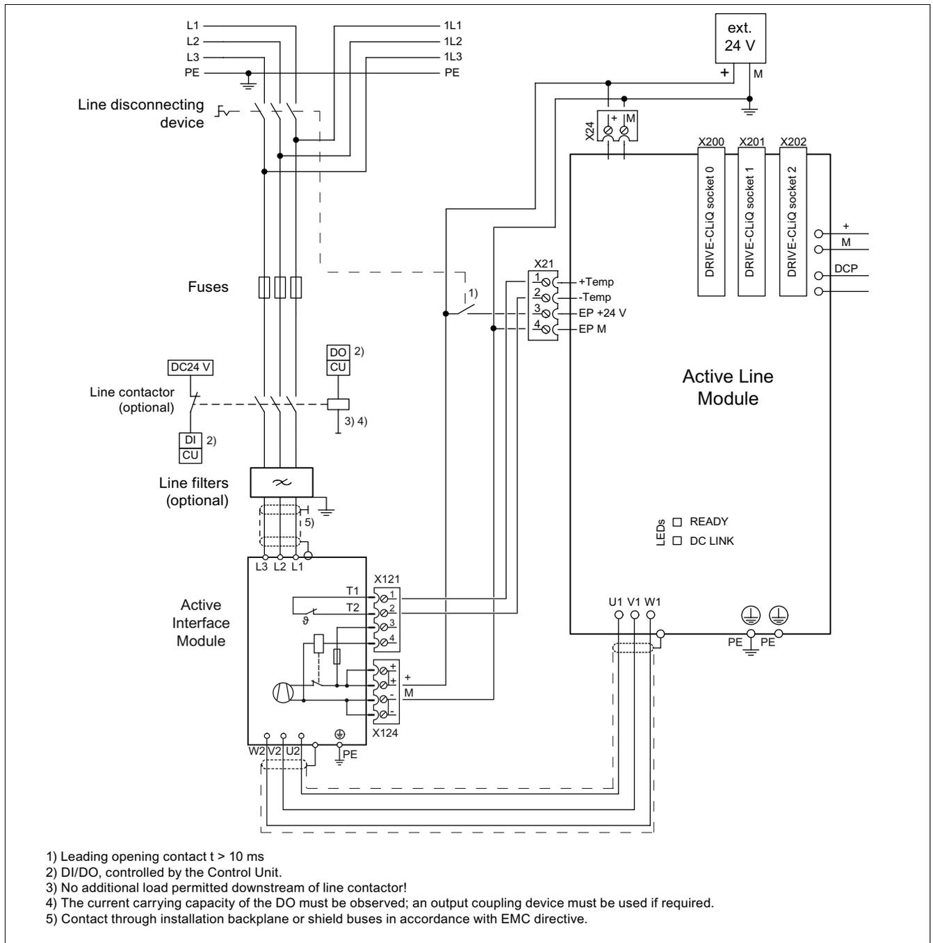
Figure 3-15 Example connection of Active Line Module
