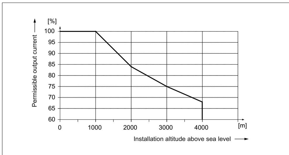
Figure 3-120 Output current as a function of the installation altitude
