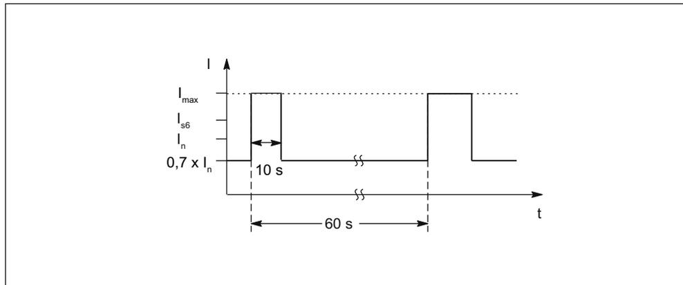
Figure 5-56 S6 duty cycle with initial load with a duty cycle duration of 60 s (for servo drives)
