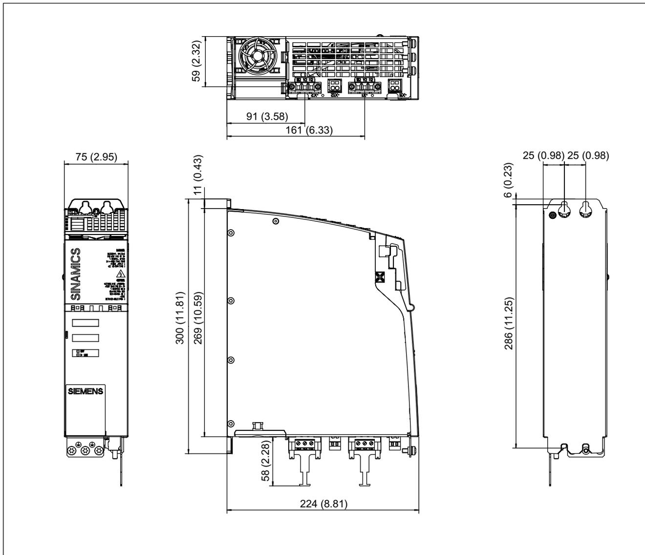
Figure 6-7 Dimension drawing of Double Motor Module in compact format 2 x 1.7 A, 2 x 3 A, and 2 x 5 A, all dimensions in mm and (inches)
