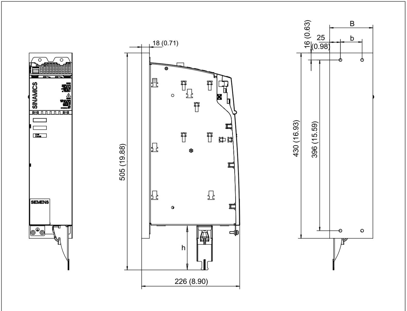
Figure 5-49 Dimension drawing of Motor Module with cold plate 30 A and 2 x 18 A, all dimensions in mm and (inches)
