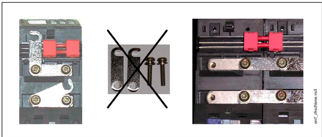
Figure 11-11 Removing the DC-link bridges
