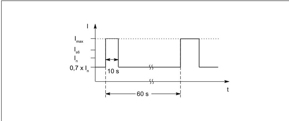
Figure 5-37 S6 duty cycle with initial load with a duty cycle duration of 60 s (for servo drives)
