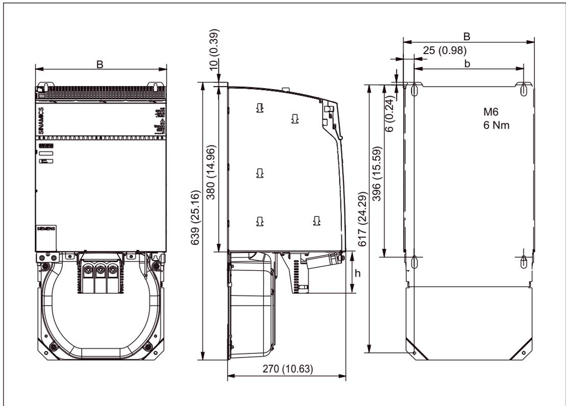
Figure 5-7 Dimension drawing of Motor Module in booksize format with internal air cooling 132 A and 200 A, all dimensions in mm and (inches)
