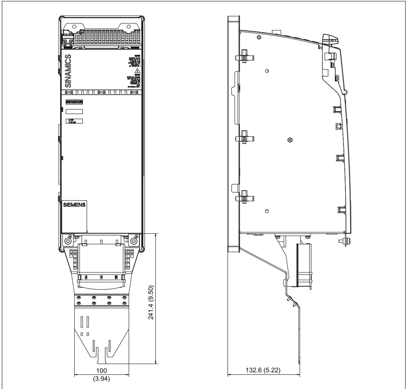
Figure 10-14 Dimension drawing of shield connecting plate on a 150 mm component with cold plate, all dimensions in mm and (inches)
