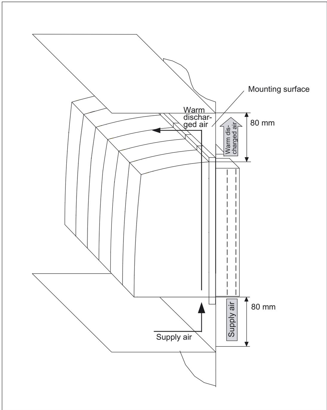
Figure 11-33 Clearances for booksize drive line-up with external air cooling
