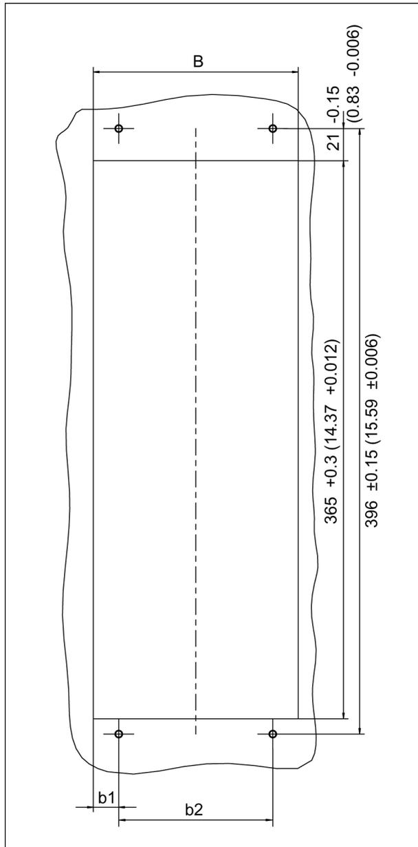
Figure 3-106 Installation openings for the Power Module with external air cooling (50 mm to 200 mm)
