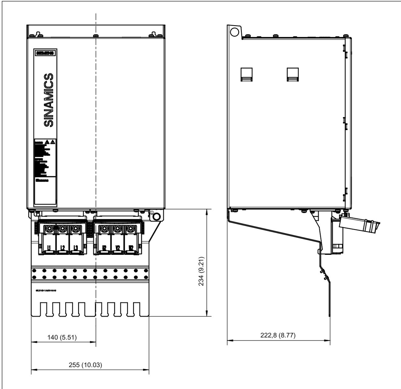
Figure 10-19 Dimension drawing of shield connecting plate on the 80 and 120 kW Active Interface Module, all dimensions in mm and (inches)
