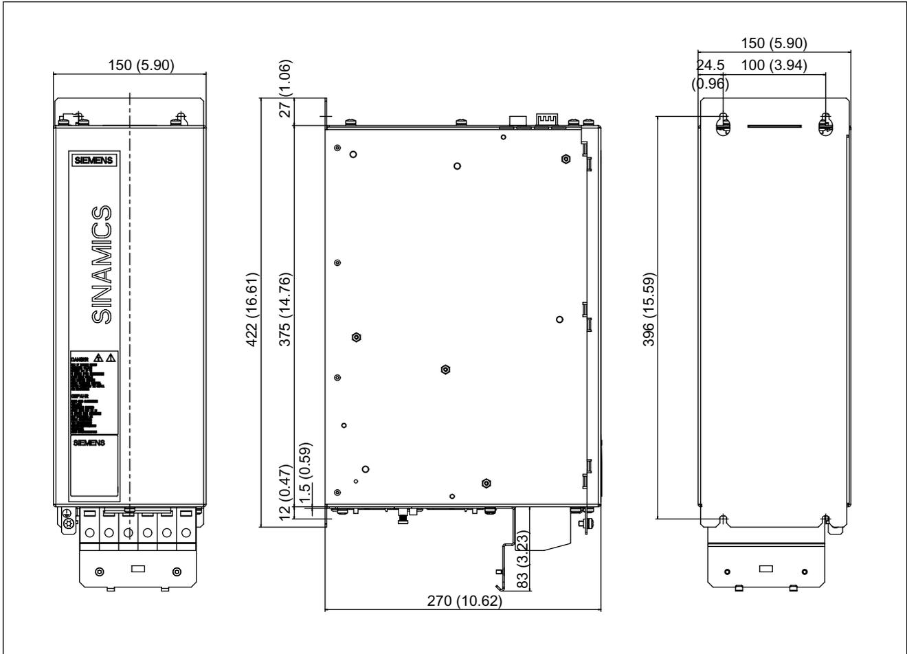
Figure 2-36 Dimension drawing of Active Interface Module 36 kW, all dimensions in mm and (inches)
