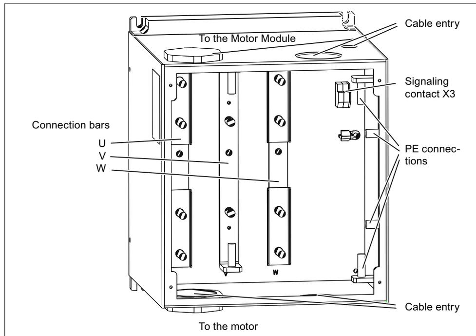
Figure 9-7 Voltage Protection Modules VPM 200 Dynamik (without cover)
