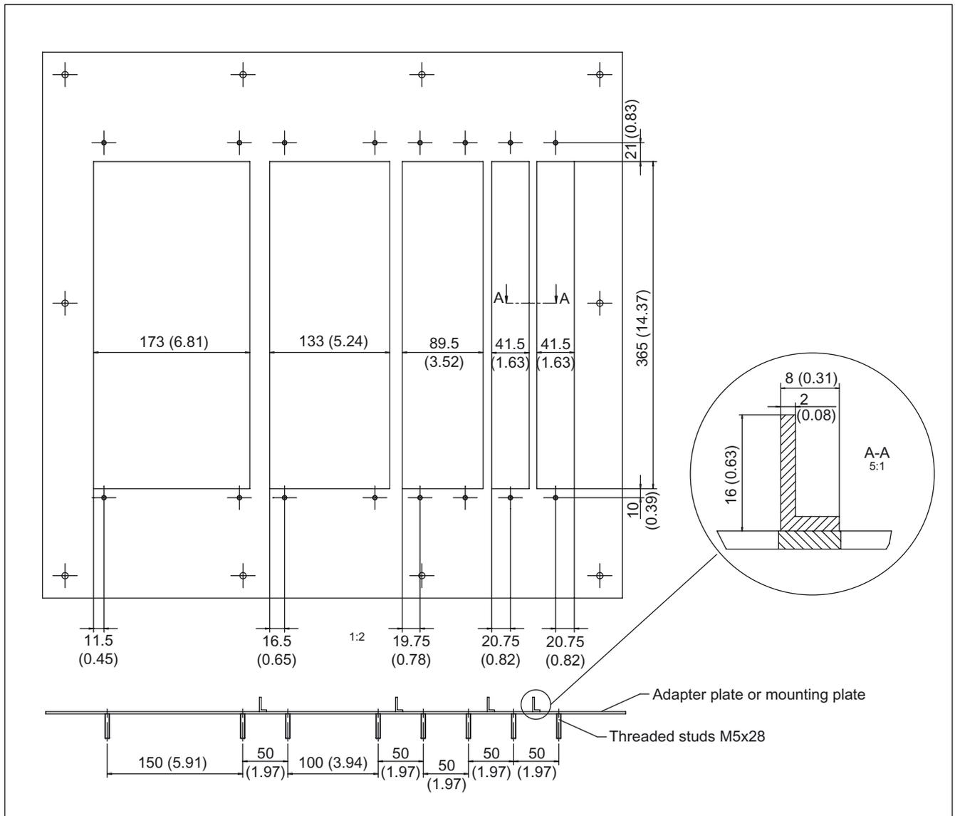
Figure 3-107 Example: mounting plate with a drive line-up
