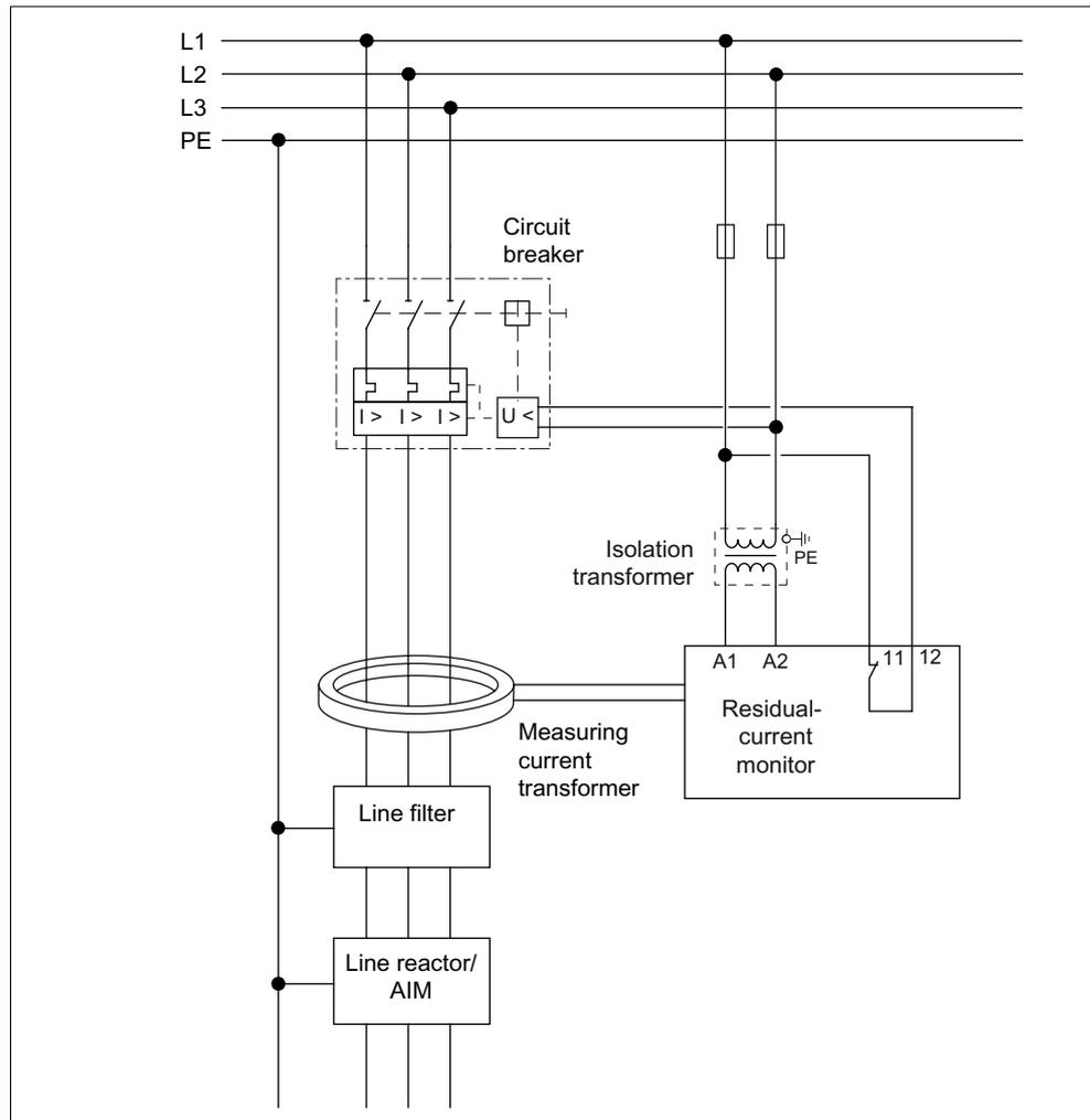
Figure 11-3 Connecting a residual-current monitor
