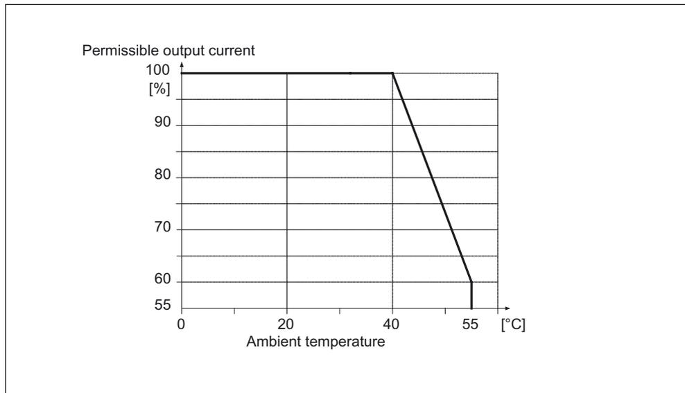
Figure 3-119 Output current as a function of the ambient temperature
