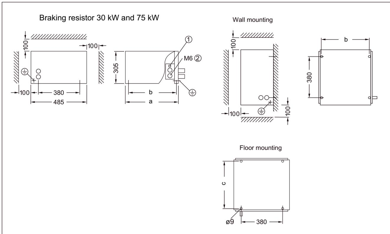
Figure 3-66 Dimension and installation drawing for braking resistor 30 kW and 75 kW, all dimensions in mm
