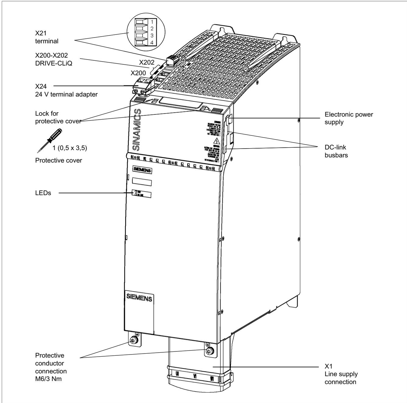
Figure 3-92 Smart Line Module with internal air cooling (36 kW)
