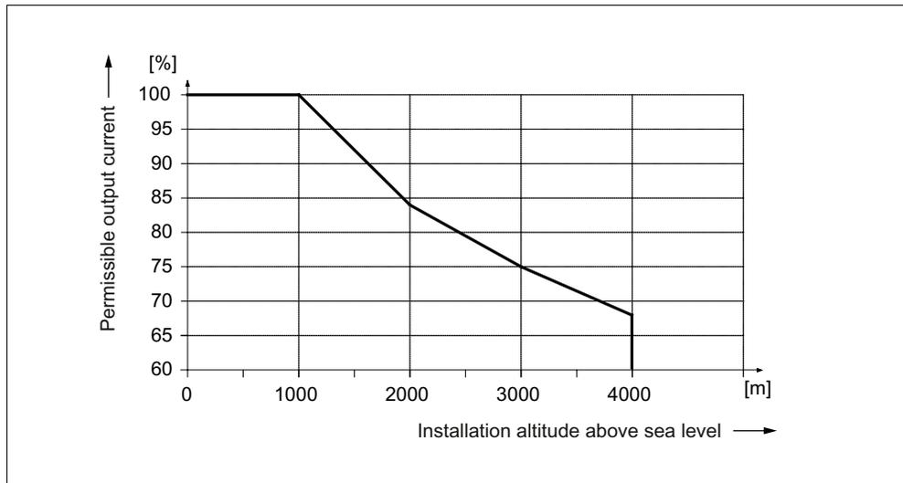
Figure 6-20 Output current as a function of the installation altitude
