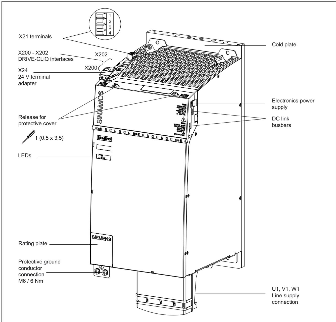
Figure 3-30 Active Line Module with cold plate (example: 55 kW)
