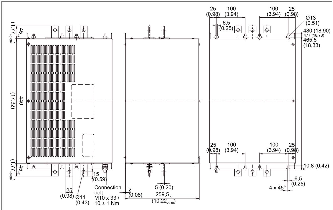
Figure 2-21 Dimension drawing of Wideband Line Filter 120 kW for Active Lines Modules, all dimensions in mm and (inches)
