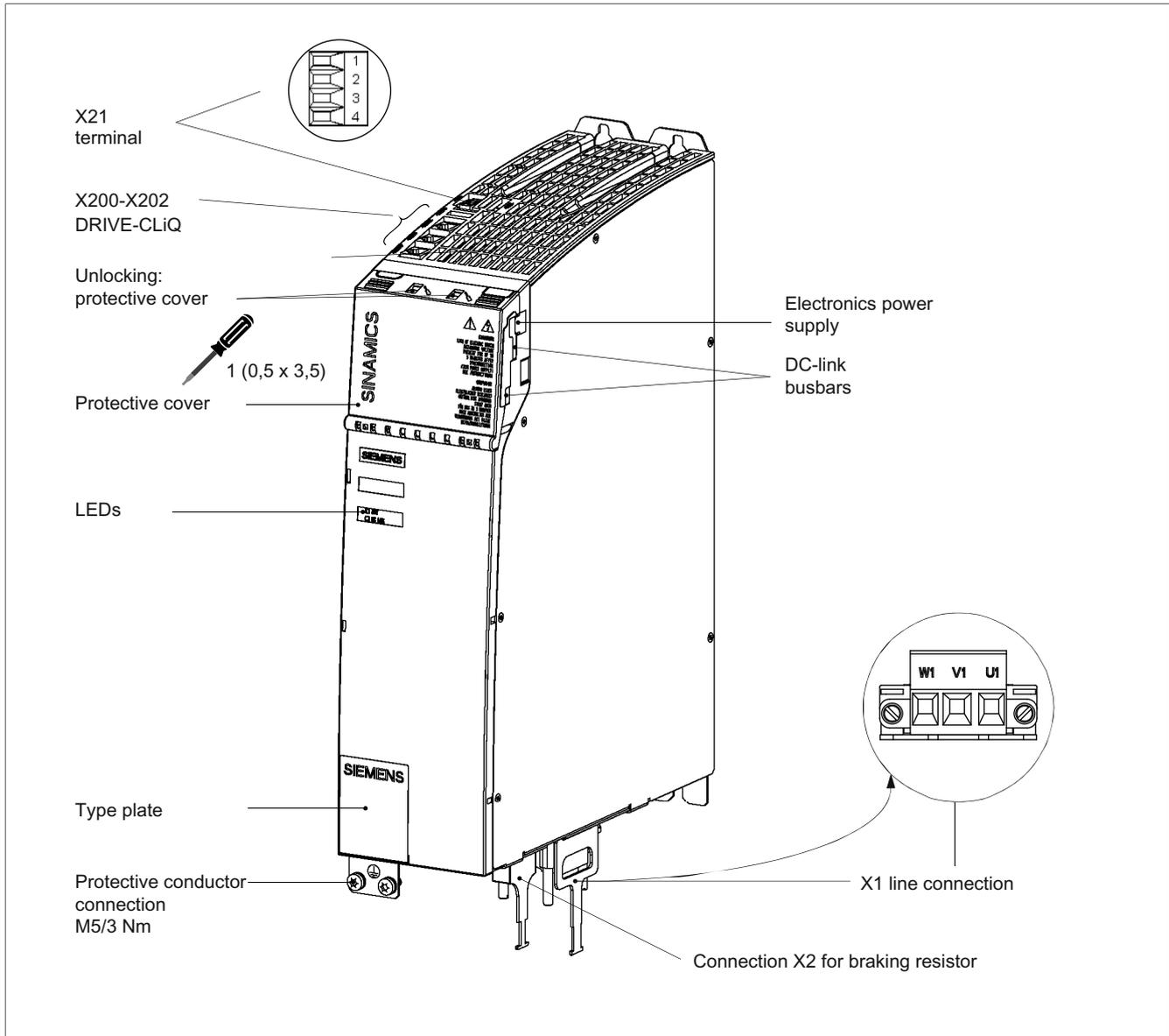
Figure 3-50 Basic Line Module with internal air cooling (20 kW)
