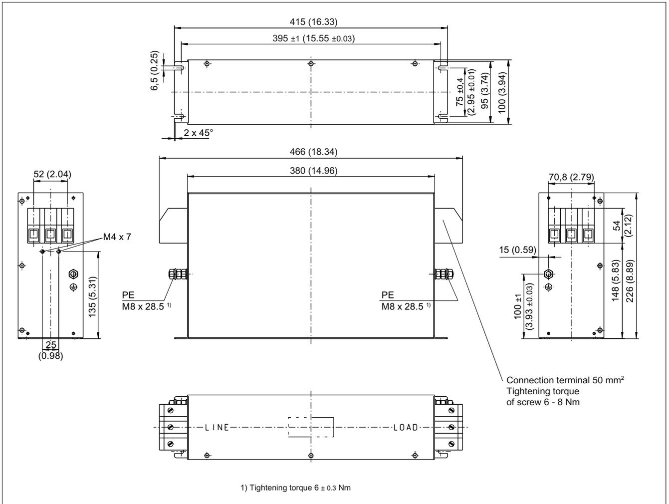
Figure 2-14 Dimension drawing of Basic Line Filter 55 kW, order number 6SL3000-0BE25-5DAx, all dimensions in mm and (inches)
