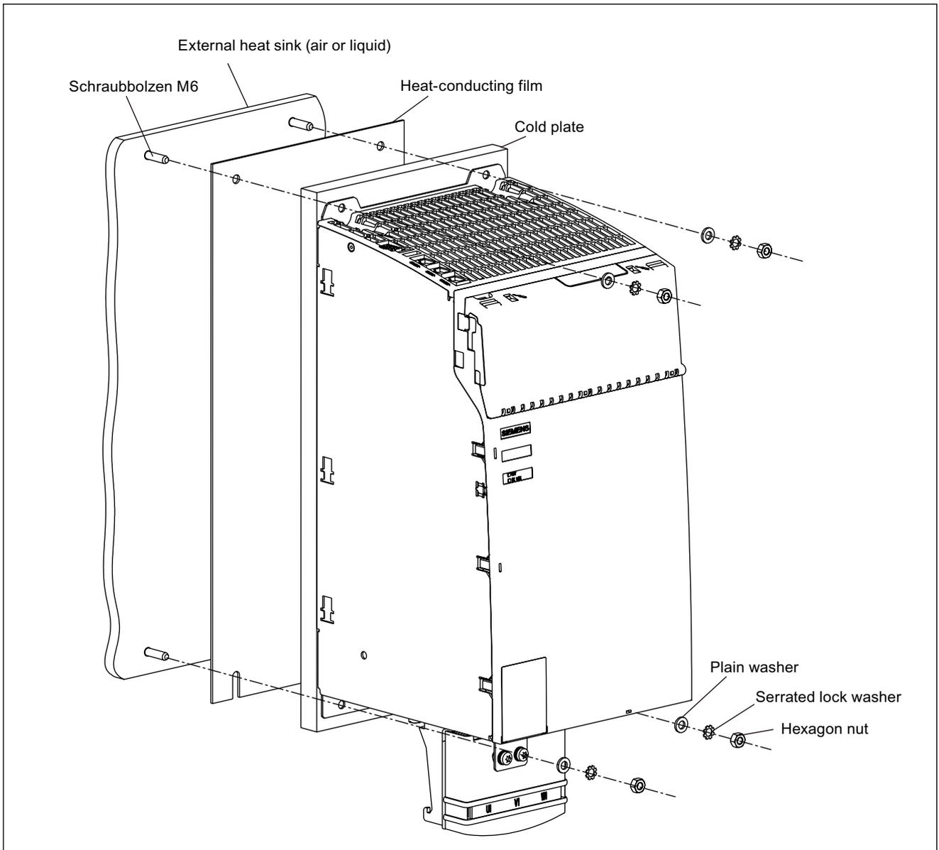
Figure 3-80 Installation of Basic Line Module 100 kW with external heat sink and heat-conducting film
