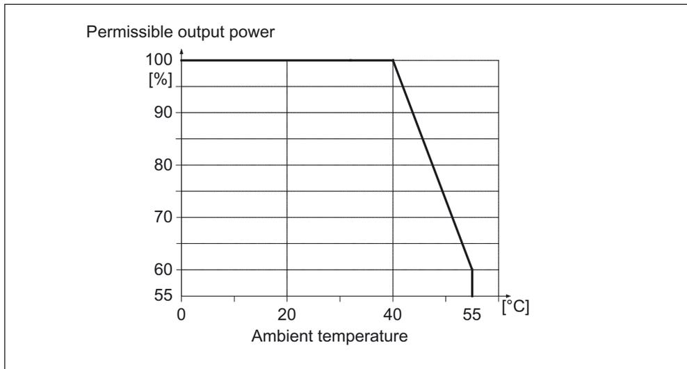
Figure 3-84 Output power as a function of the ambient temperature
