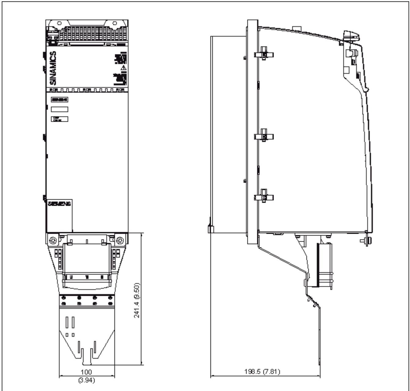
Figure 10-10 Dimension drawing of shield connecting plate on a 150 mm component with external air cooling, all dimensions in mm and (inches)
