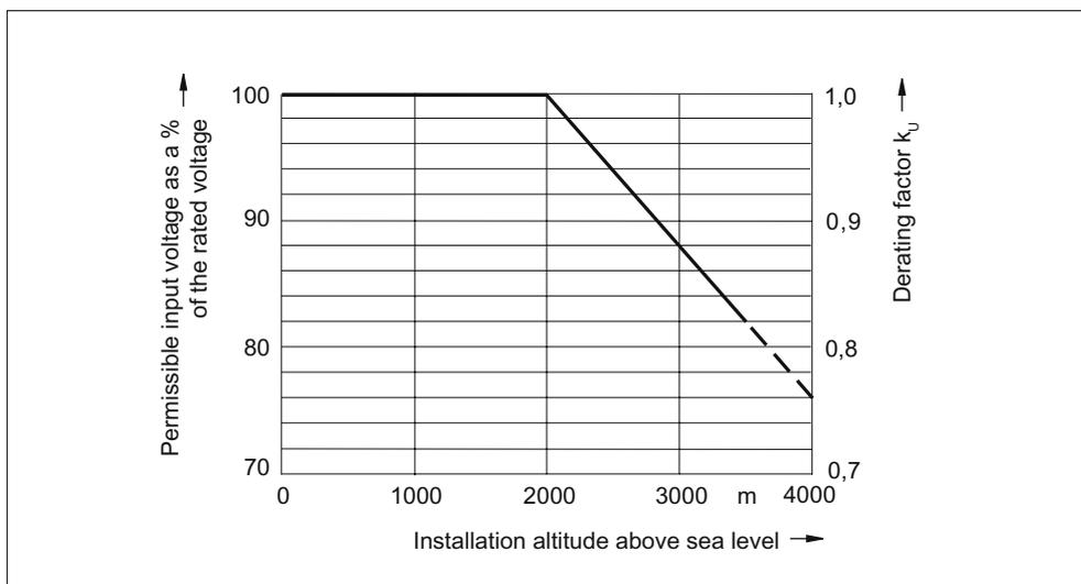
Figure 5-63 Voltage derating as a function of the installation altitude
