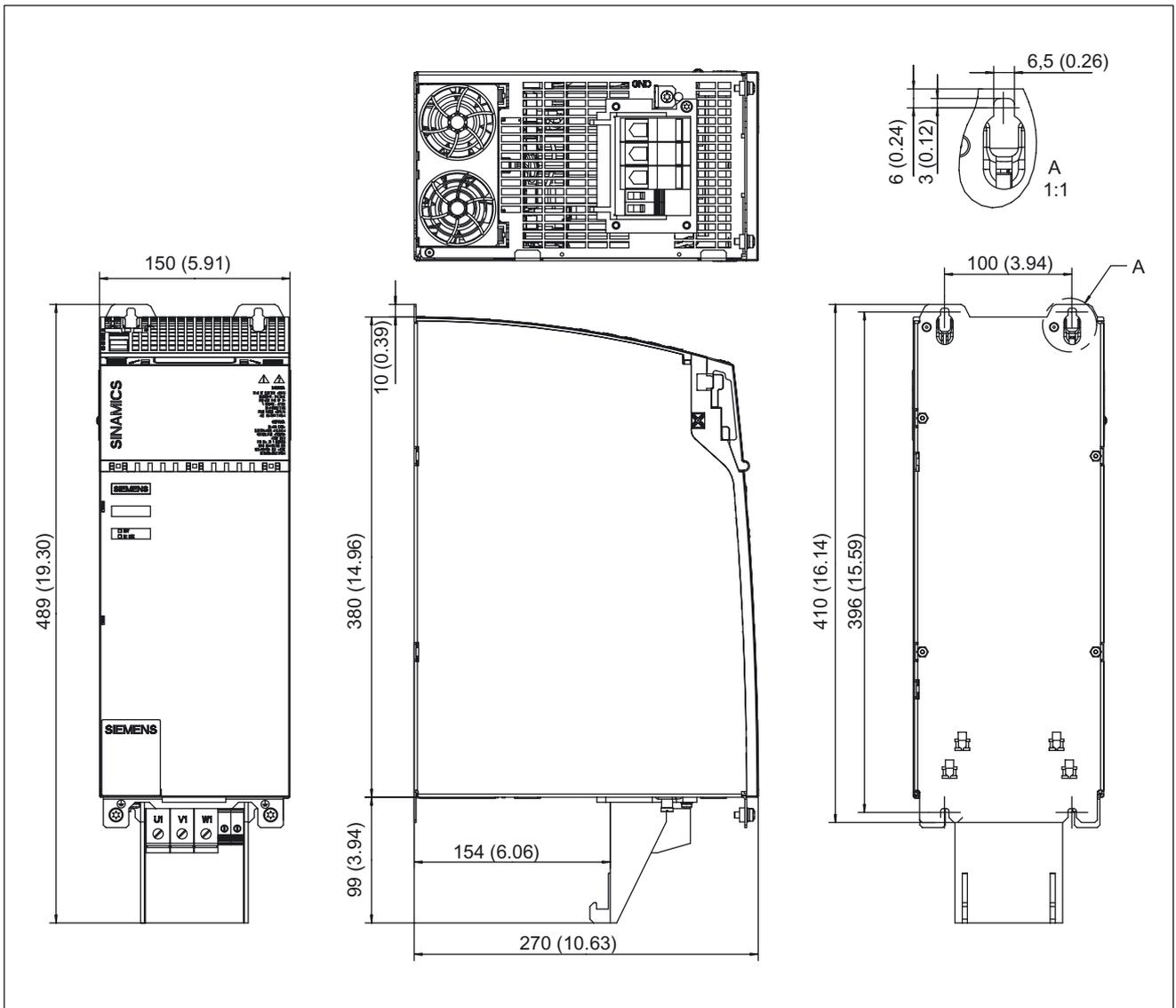
Figure 3-56 Dimension drawing of Basic Line Module 40 kW with internal air cooling, all dimensions in mm and (inches)
