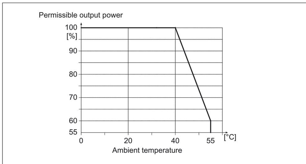
Figure 3-62 Output power as a function of the ambient temperature
