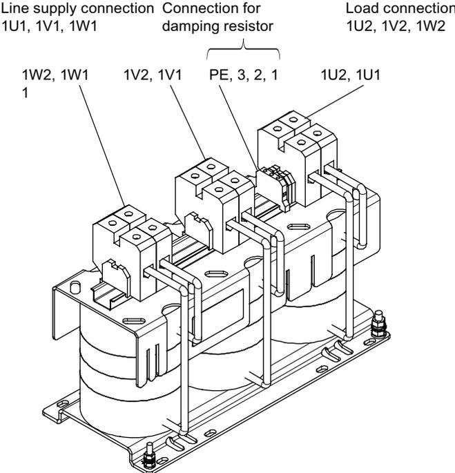
Figure 2-48 HFD line reactor 80 kW
