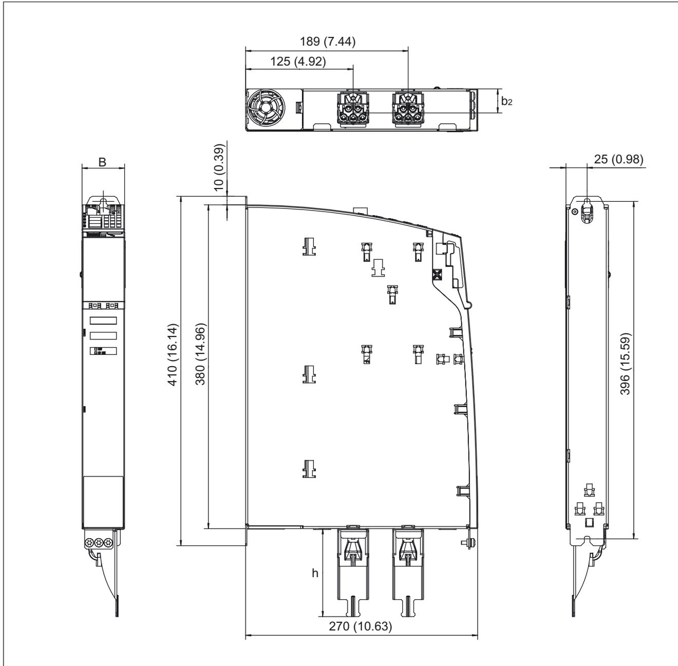
Figure 5-4 Dimension drawing of Motor Module in booksize format with internal air cooling 3 A to 18 A and 2 x 3 A to 2 x 9 A, all dimensions in mm and (inches)
