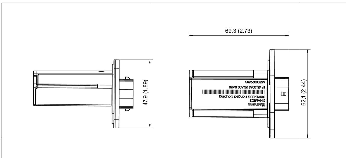
Figure 10-28 Dimension drawing of the DRIVE-CLiQ cabinet bushing, all dimensions in mm and (inches)
