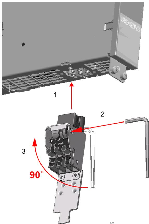
Figure 11-18 Installation example: Screw connector
