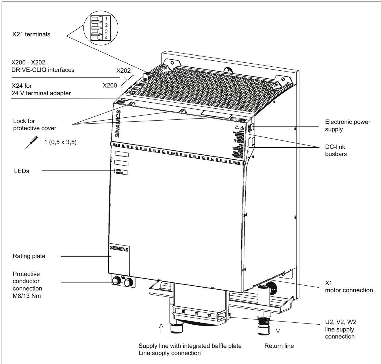
Figure 5-64 Motor Module Liquid Cooled (200 A)
