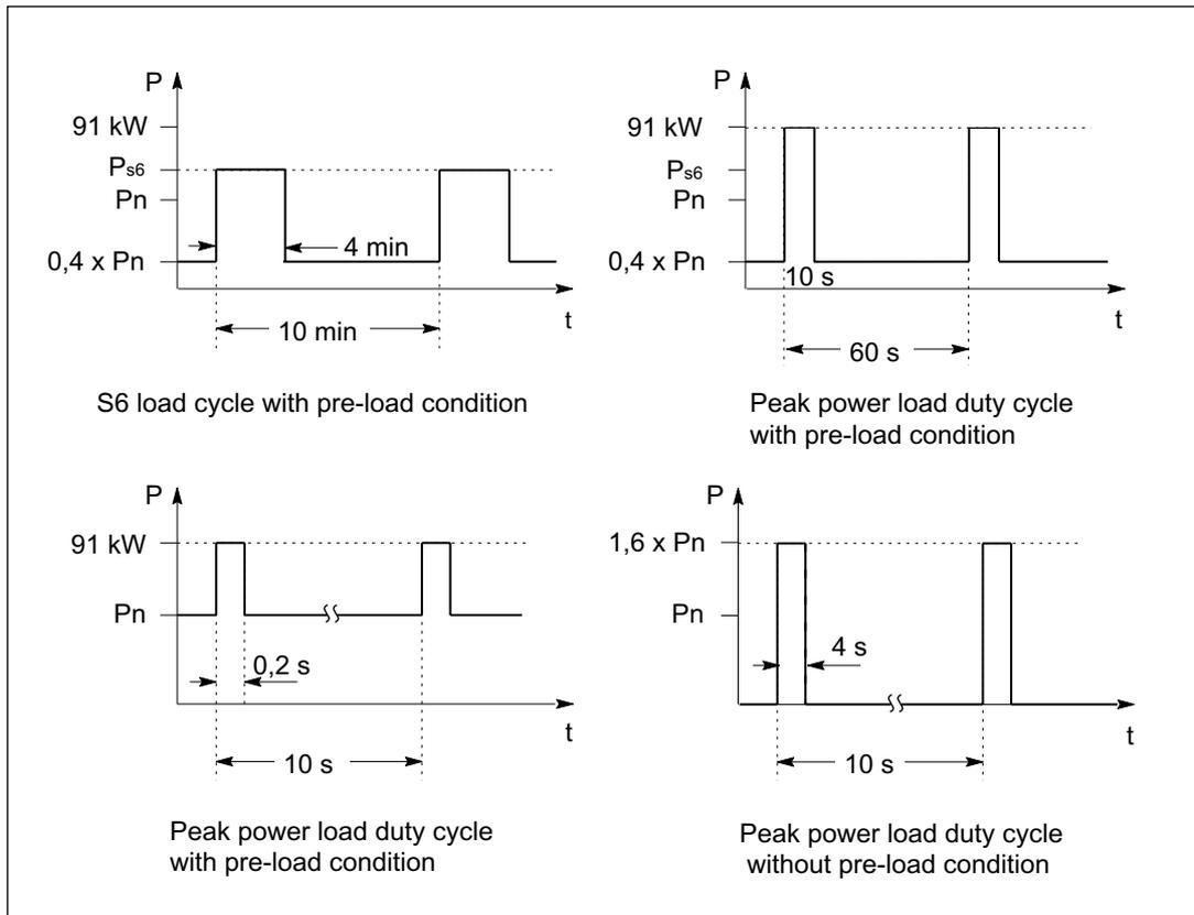
Figure 3-36 Rated duty cycles of 55 kW Active Line Modules with Active Interface Module
