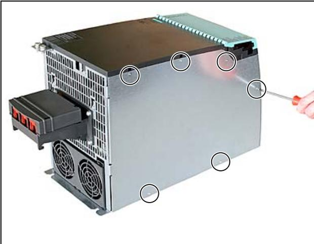
Open the right device cover by loosening the six marked screws
