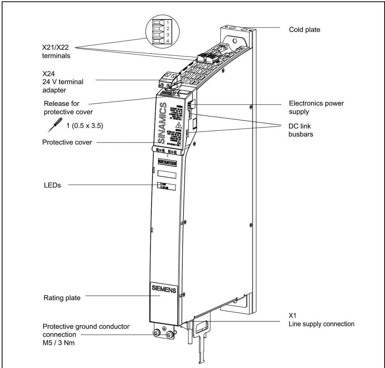
Figure 3-114 Smart line module with cold plate (10 kW)
