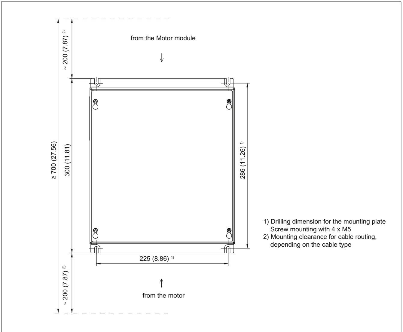
Figure 9-14 Mounting dimensions for a Voltage Protection Module VPM200
