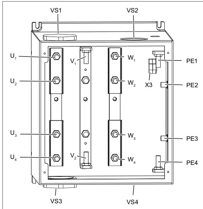
Figure 9-16 Terminals for Voltage Protection Module VPM 200 Dynamik
