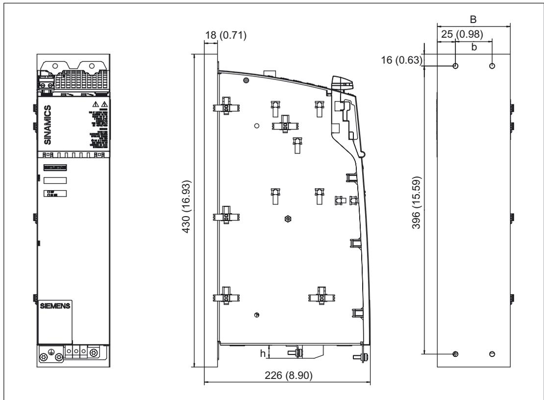
Figure 3-32 Dimension drawing of Active Line Module with cold plate (16 kW), all dimensions in mm and (inches)
