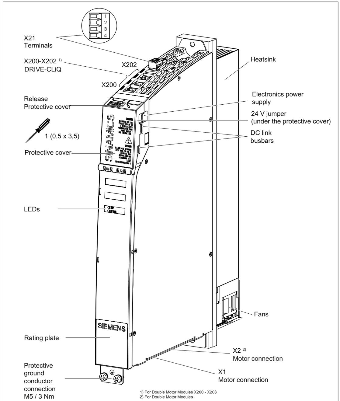
Figure 5-20 Example: Single Motor Module with external air cooling (5 A)
