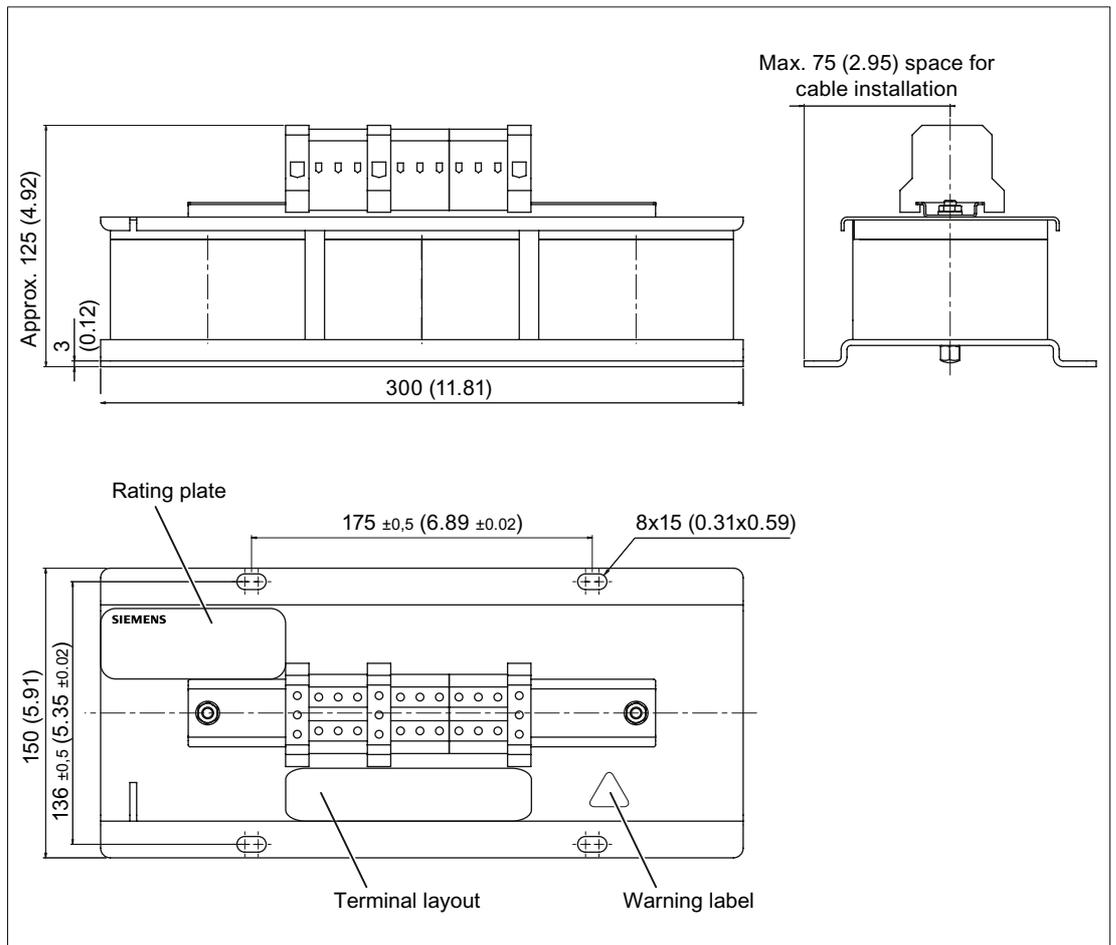
Figure 2-50 Dimension drawing of HFD line reactor 16 kW, all dimensions in mm and (inches)
