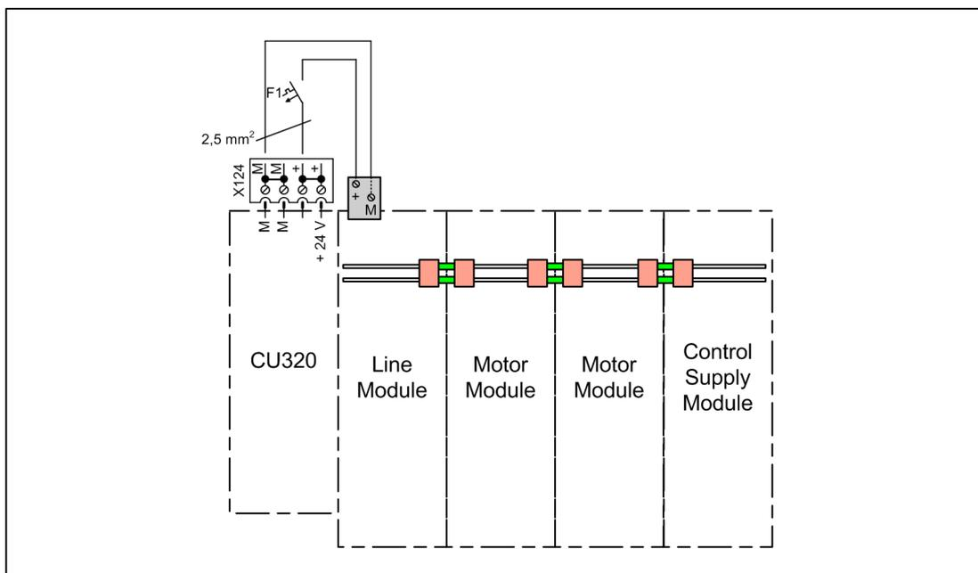
Figure 11-4 Example: 24 V supply with Control Supply Module
