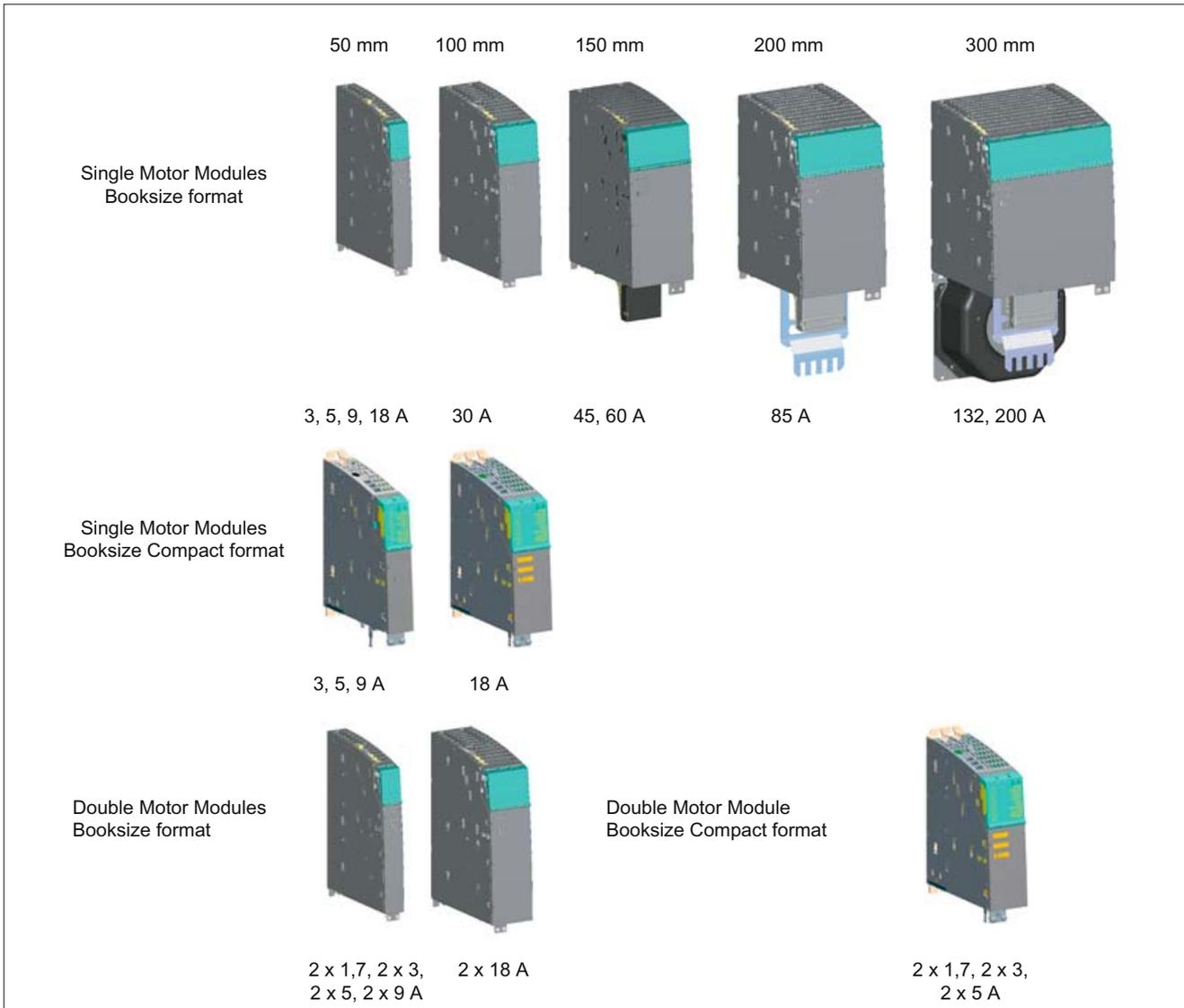
Figure 1-6 Overview of Motor Modules booksize (currents are continuous rms)
