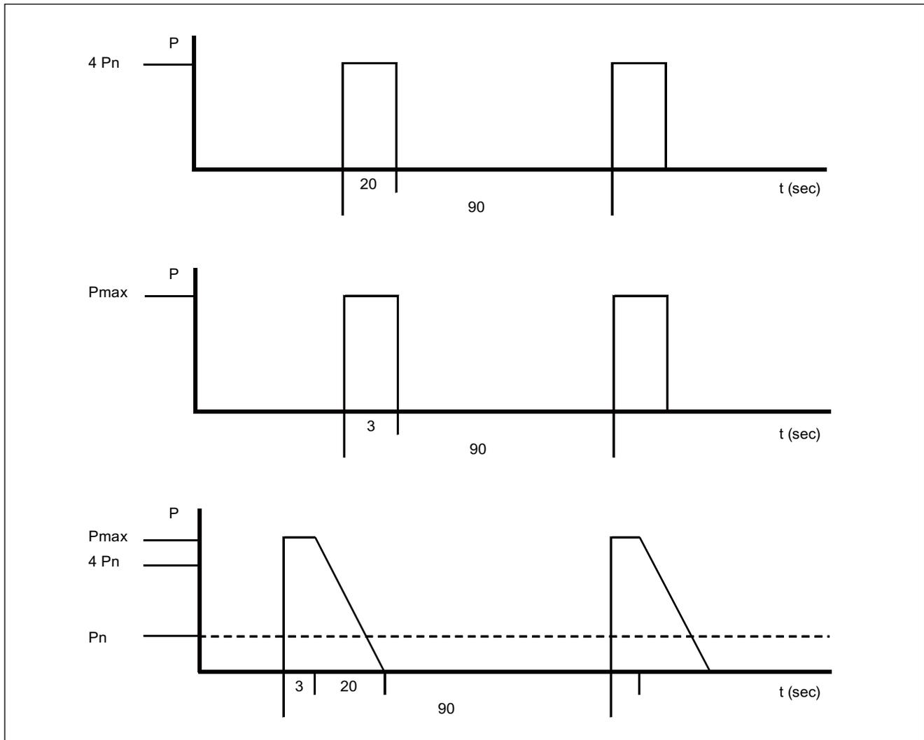
Figure 3-67 Braking duty cycles for braking resistors
