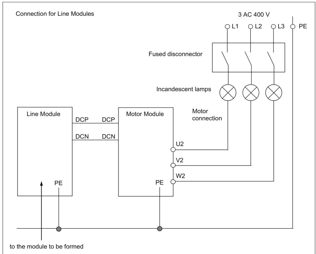
Figure 13-1 Forming circuit for Line Modules with incandescent lamps
