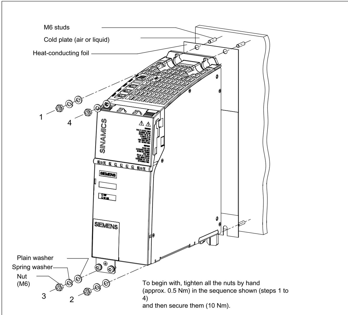
Figure 4-5 Installation: Smart Line Module Booksize Compact onto a cold plate
