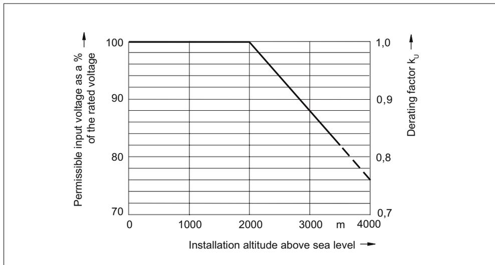
Figure 5-79 Voltage derating as a function of the installation altitude
