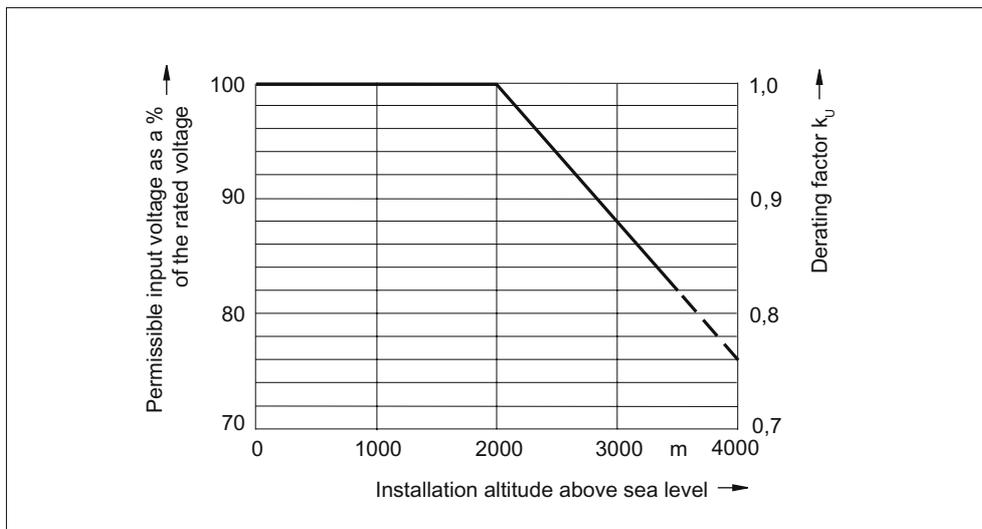
Figure 3-29 Voltage derating as a function of the installation altitude
