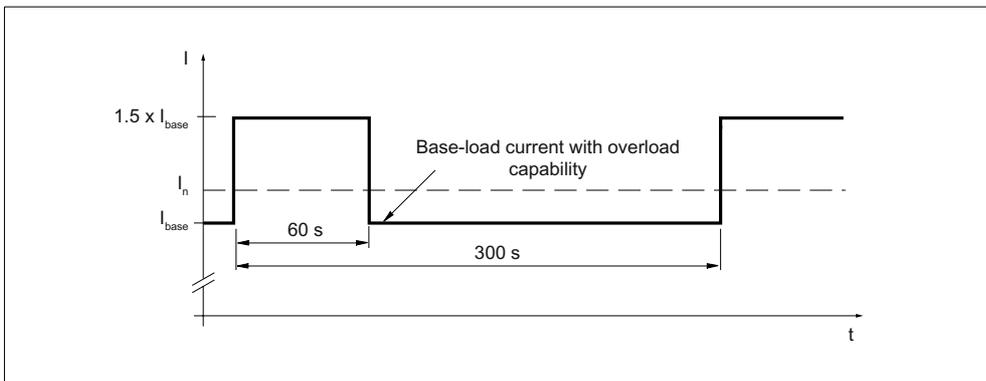
Figure 5-73 Duty cycle with 60 s overload with a duty cycle duration of 300 s
