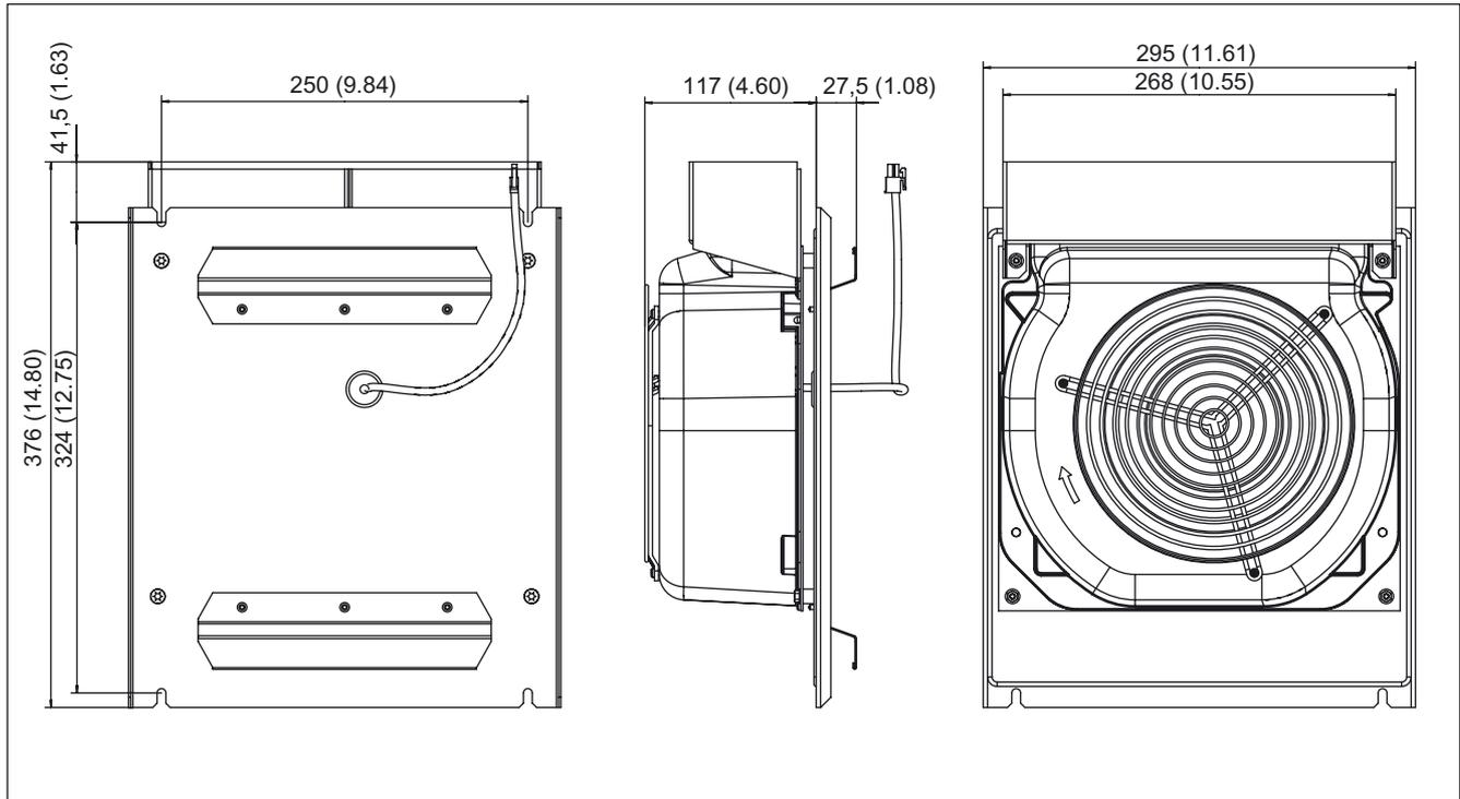
Figure 5-27 Dimension drawing of Fans for Motor Modules with external air cooling 132 A and 200 A, all dimensions in mm and (inches)
