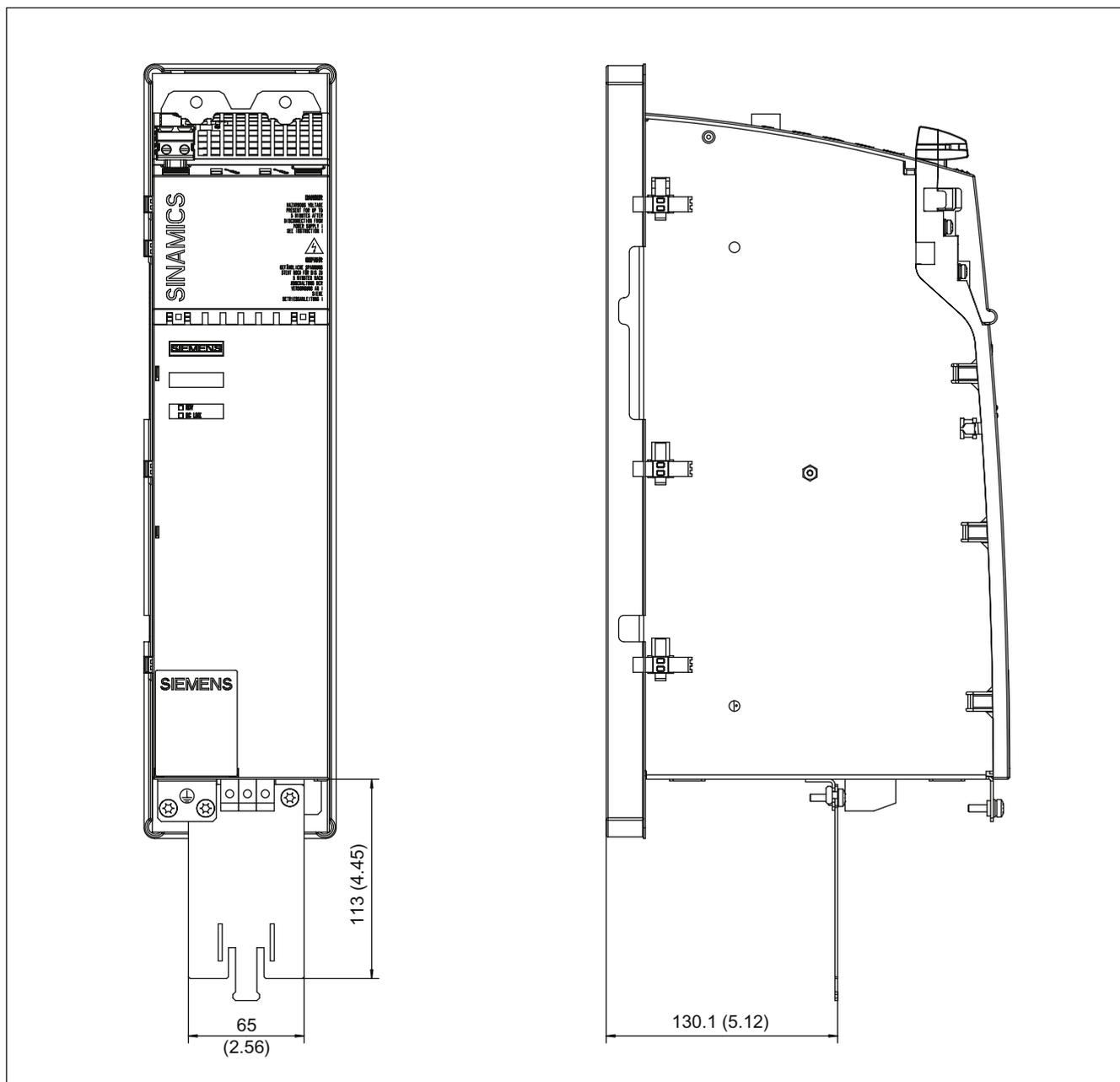
Figure 10-13 Dimension drawing of shield connecting plate on a 100 mm component with cold plate, all dimensions in mm and (inches)
