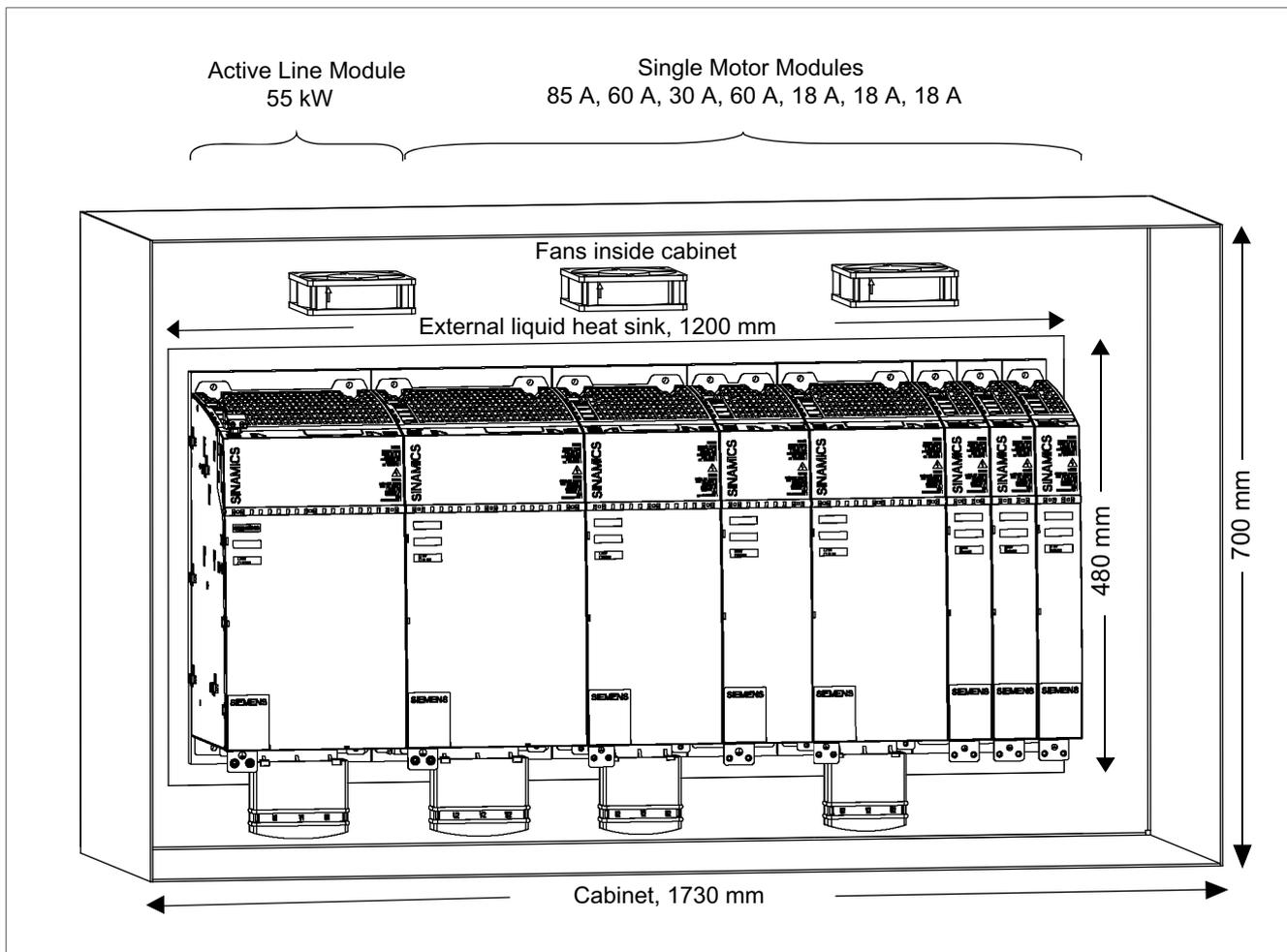
Figure 11-31 Example: cold plate drive line-up with external liquid cooling
