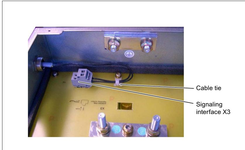
Figure 9-15 Connecting terminal X3 on the Voltage Protection Module (using the VPM 200 as an example)
