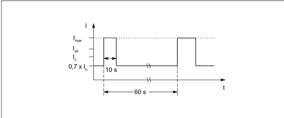
Figure 5-71 S6 duty cycle with initial load with a duty cycle duration of 60 s (for servo drives)
