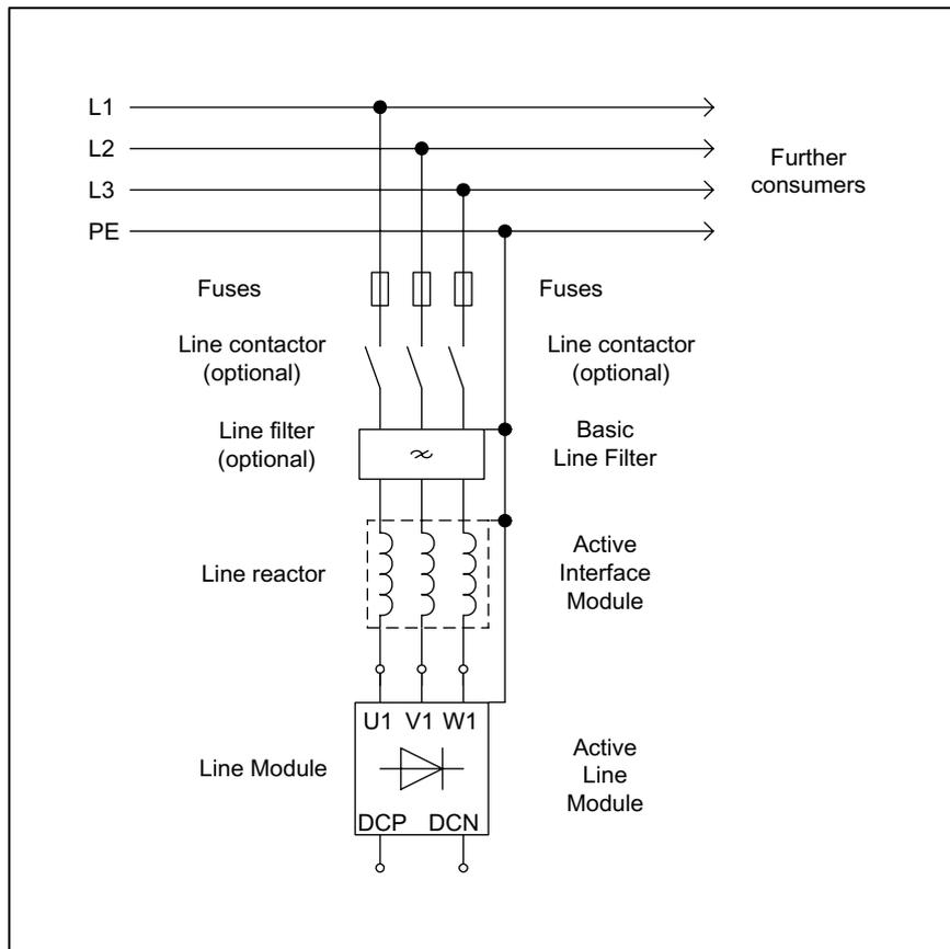
Figure 2-70 Direct operation on the line supply
