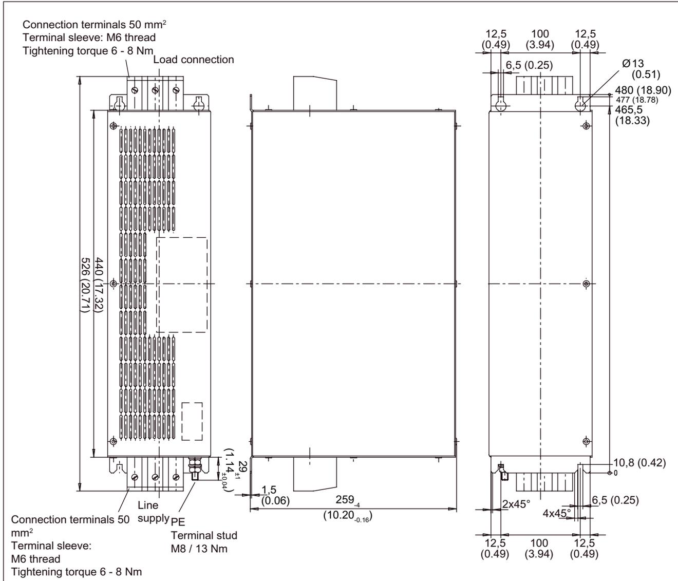
Figure 2-19 Dimension drawing of Wideband Line Filter 55 kW for Active Lines Modules, all dimensions in mm and (inches)
