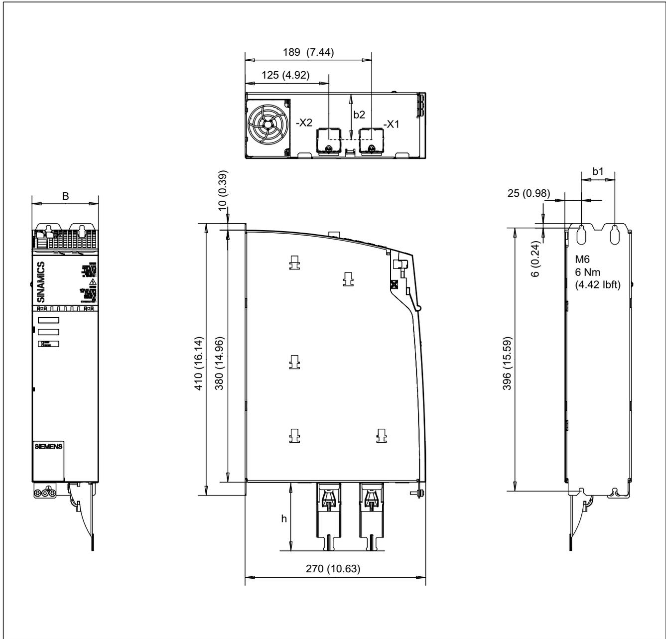
Figure 5-5 Dimension drawing of Motor Module in booksize format with internal air cooling 30 A and 2 x 18 A, all dimensions in mm and (inches)
