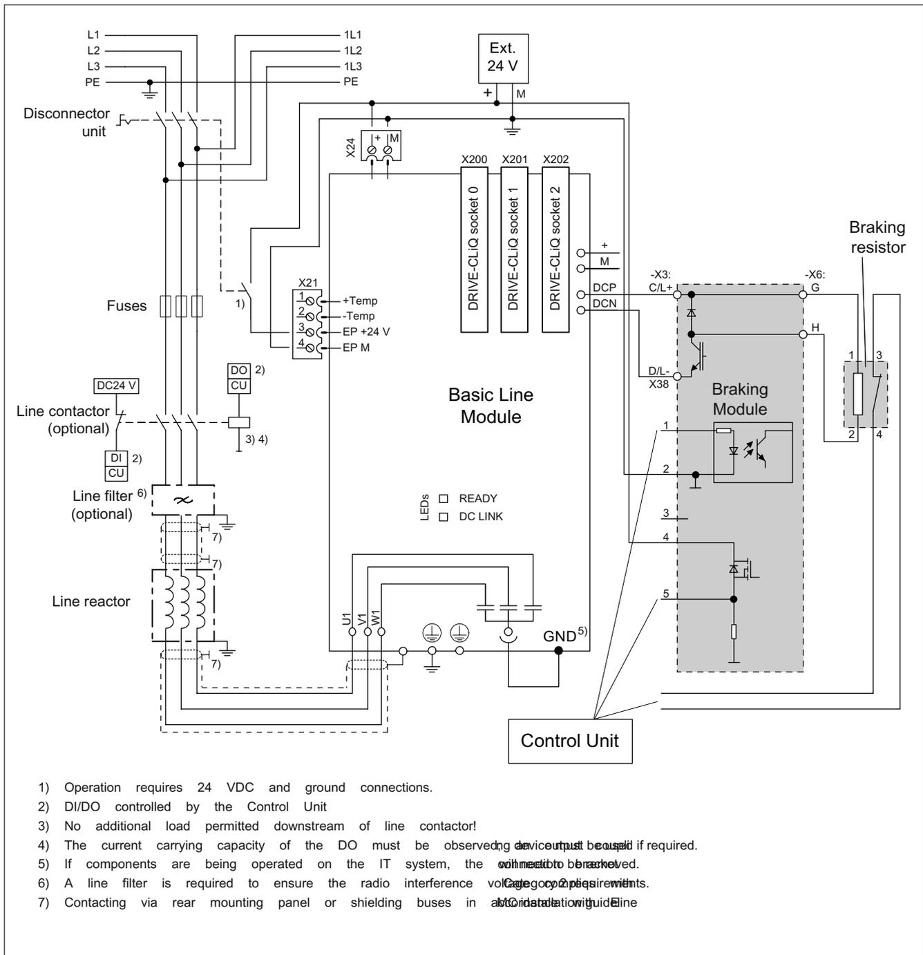
Figure 3-69 Connection example MASTERDRIVES braking module
