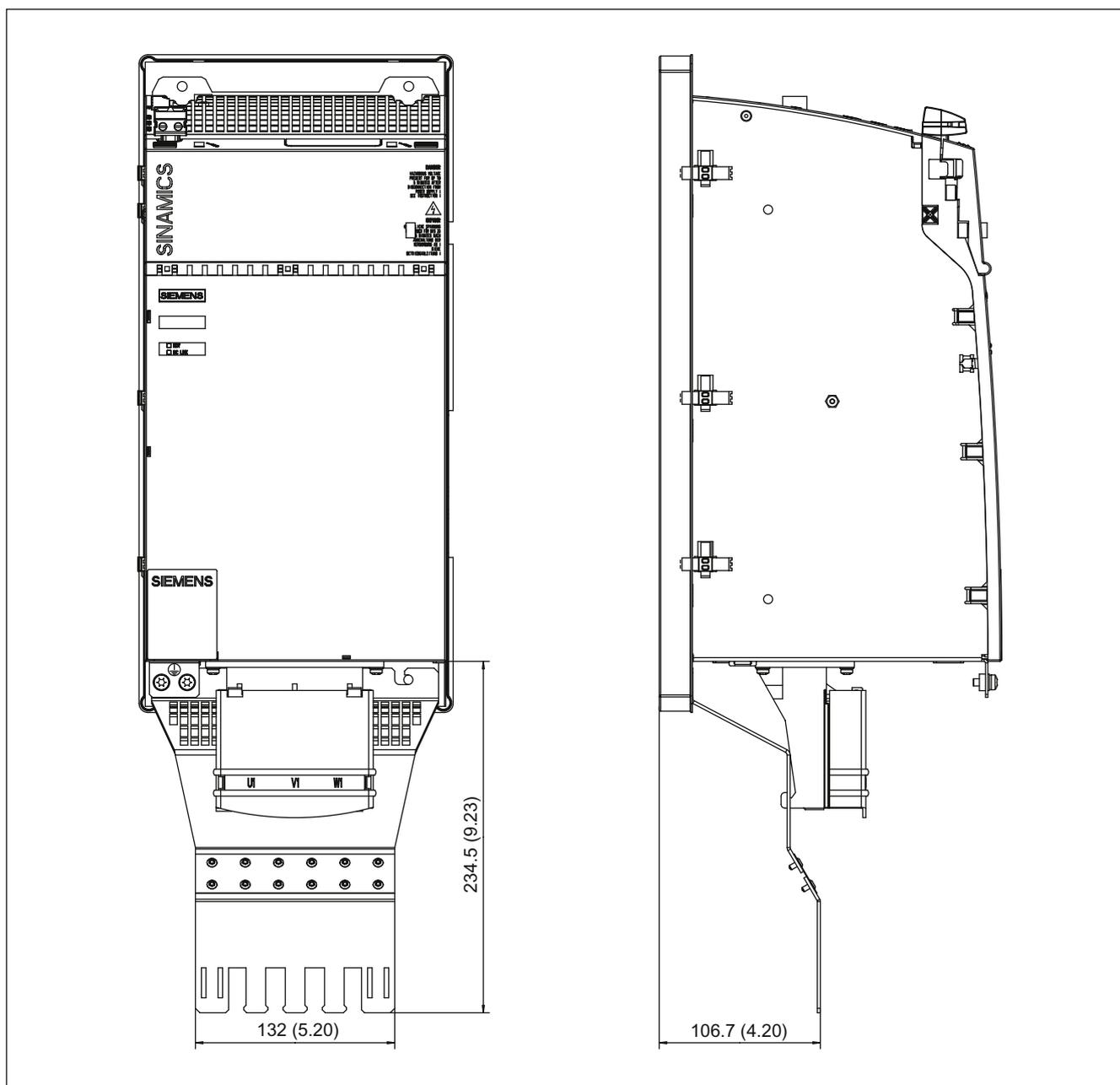
Figure 10-15 Dimension drawing of shield connecting plate on a 200 mm component with cold plate, all dimensions in mm and (inches)
