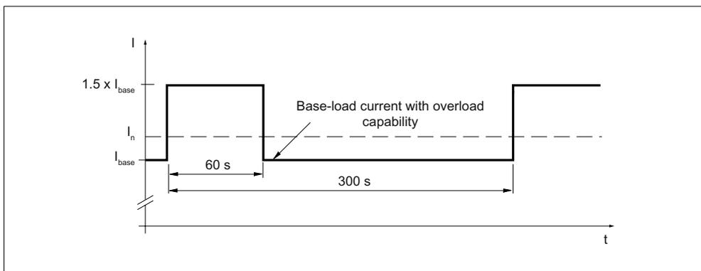
Figure 5-14 Duty cycle with 60 s overload with a duty cycle duration of 300 s
