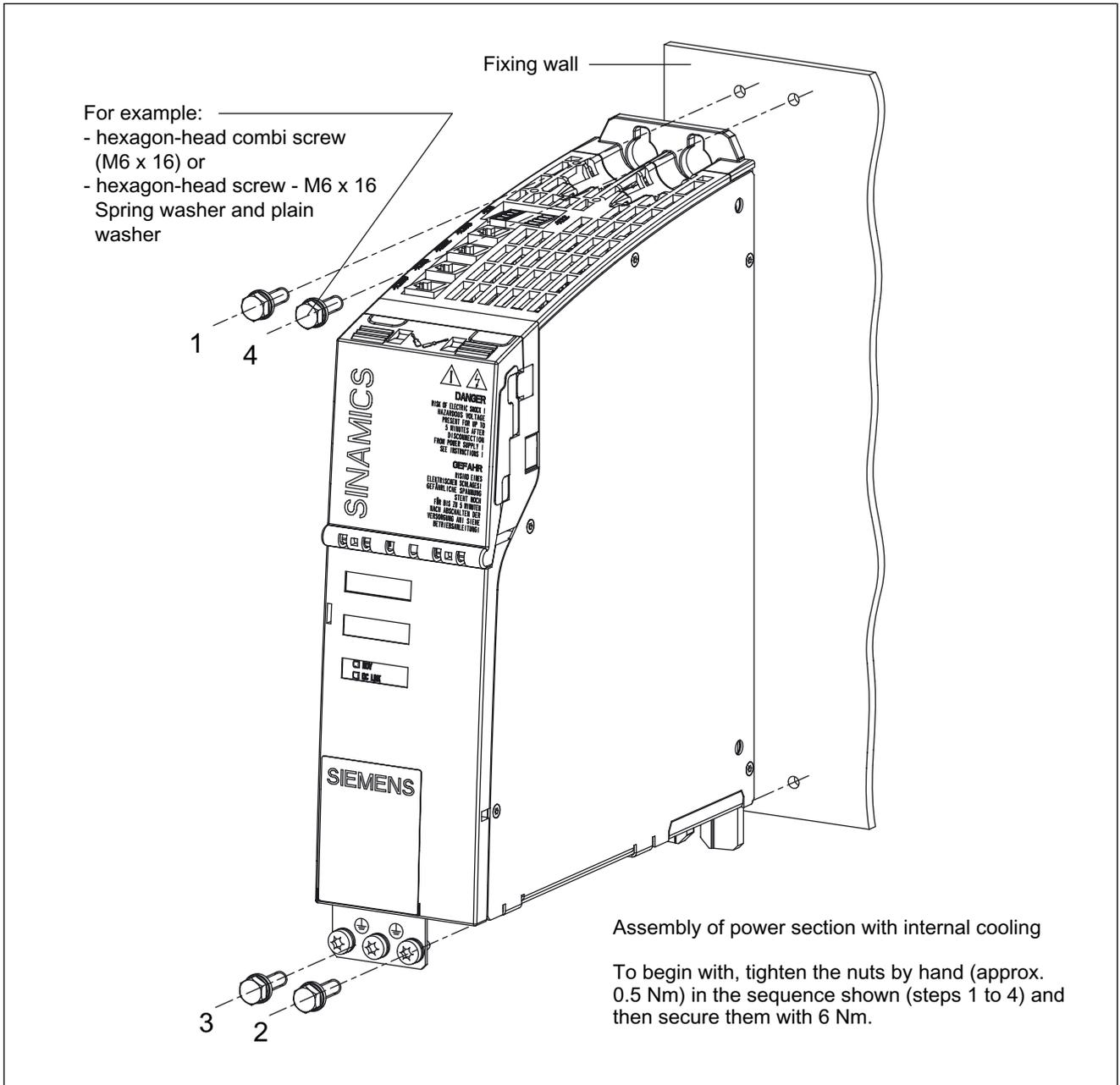
Figure 6-8 Installation: Motor Module Booksize Compact with internal air cooling
