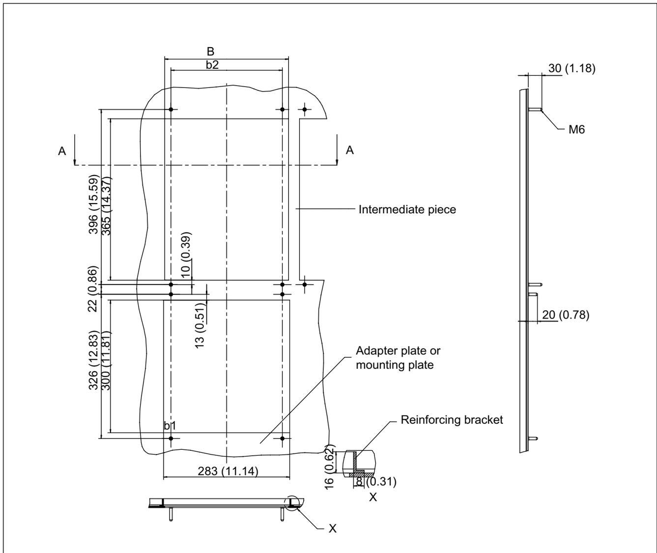
Figure 3-20 Installation openings for the power unit with external air cooling, 300 mm
