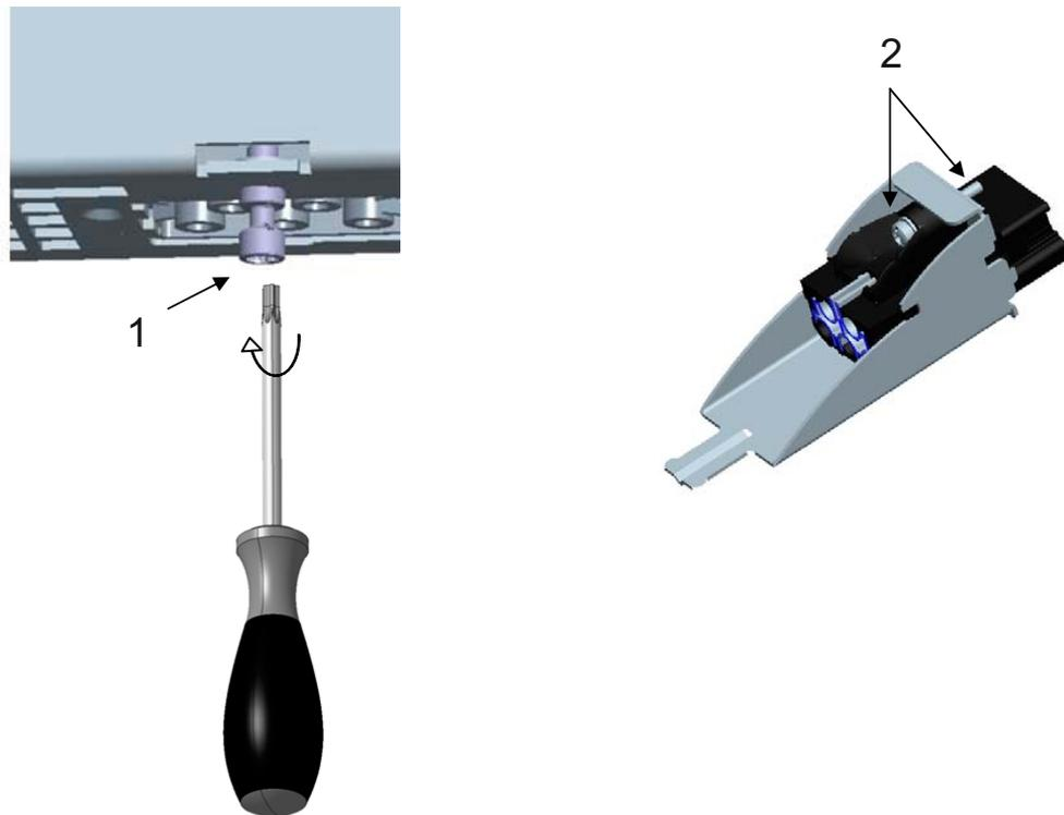
Figure 11-19 Installation of the motor connection plug with screwed joint
