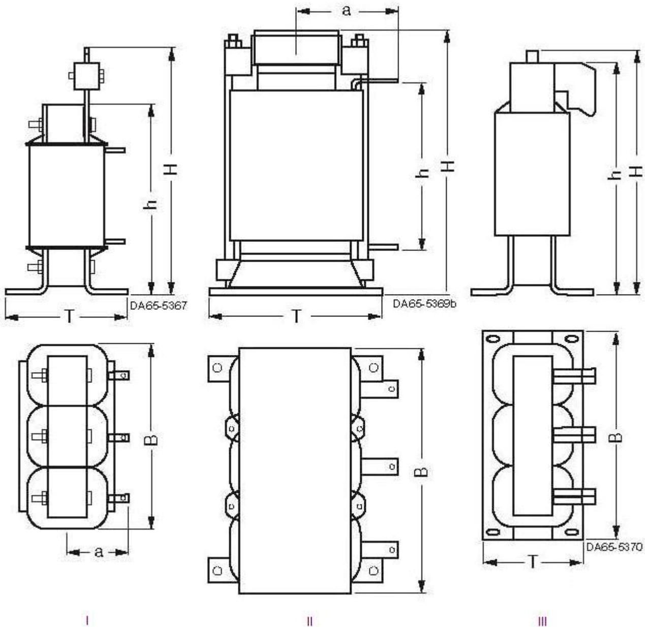
Figure 9-1 Dimension drawings of motor reactors
