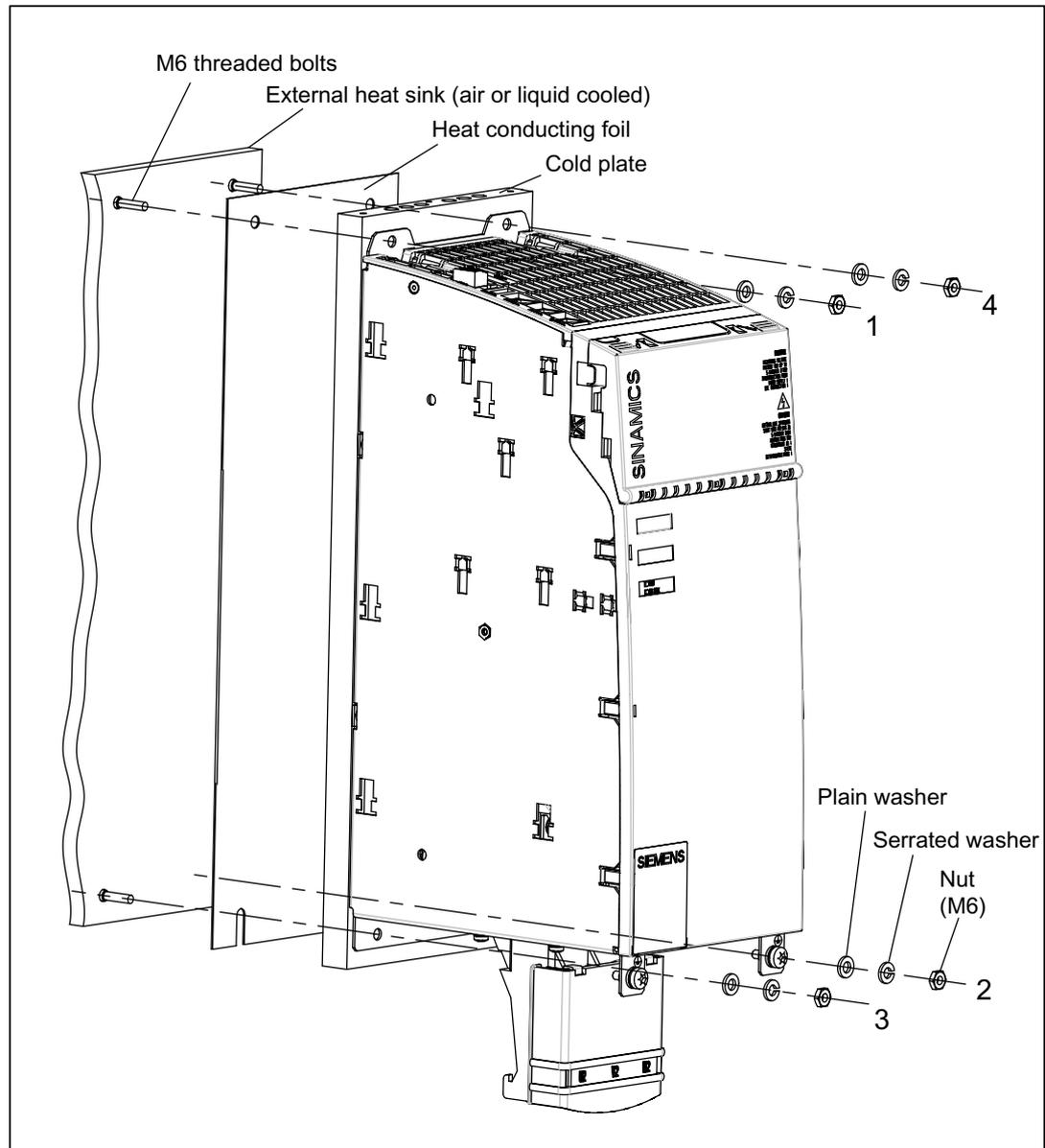
Figure 5-52 Installation of a cold plate power unit with an external heat sink and heat-conducting foil
