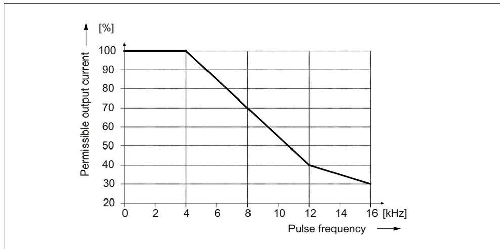
Figure 5-61 Output current as a function of the pulse frequency for 200 A Motor Modules (applies from order number 6SL312x-1TE32-0AA4)
