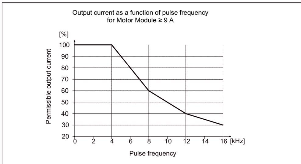
Figure 6-19 Output current as a function of the pulse frequency for the Motor Module  $\geq 9$  A
