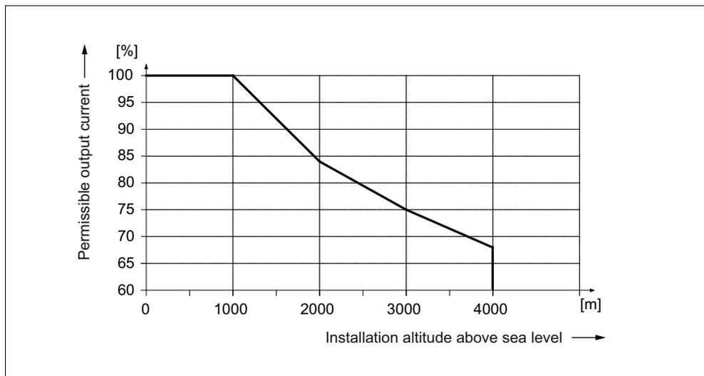
Figure 3-39 Output current as a function of the installation altitude
