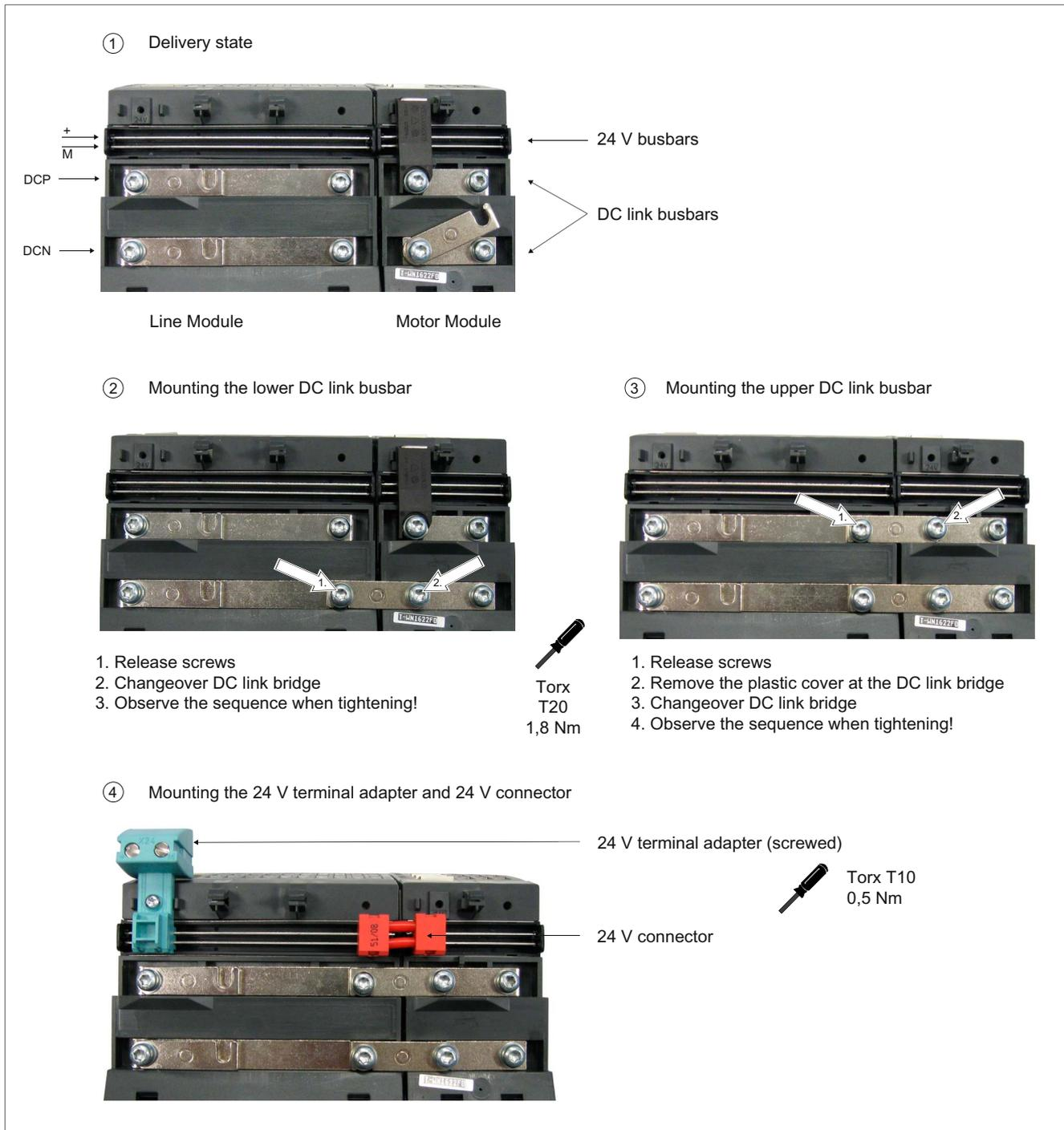
Figure 7-1 Connection of DC-link busbars and 24 V busbars
