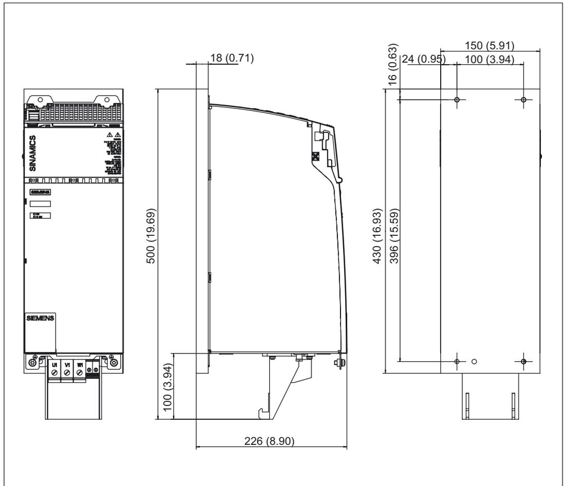
Figure 3-77 Dimension drawing of Basic Line Module with cold plate (40 kW), all dimensions in mm and (inches)
