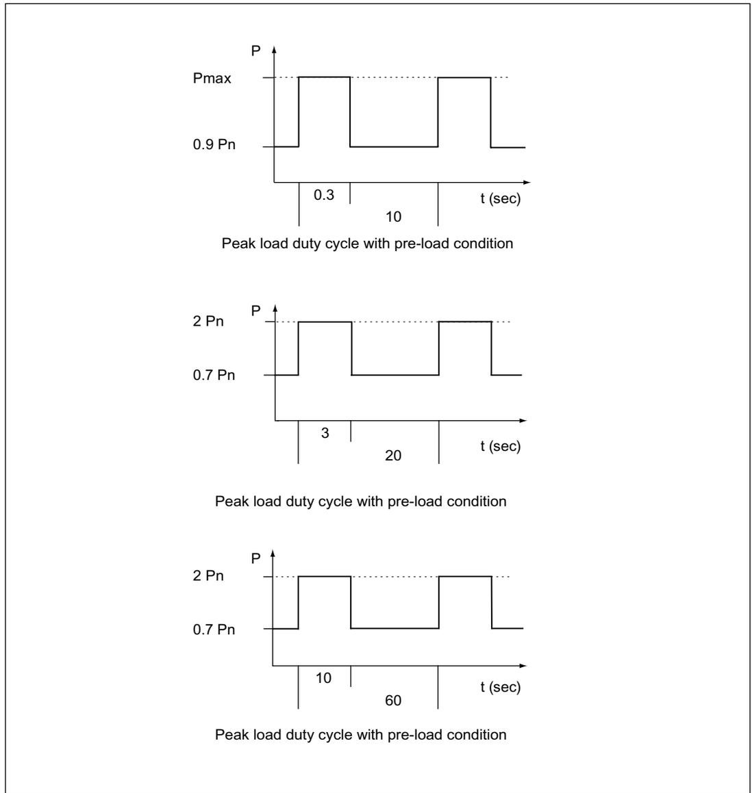
Figure 3-59 Rated duty cycles of 20 kW and 40 kW Basic Line Modules
