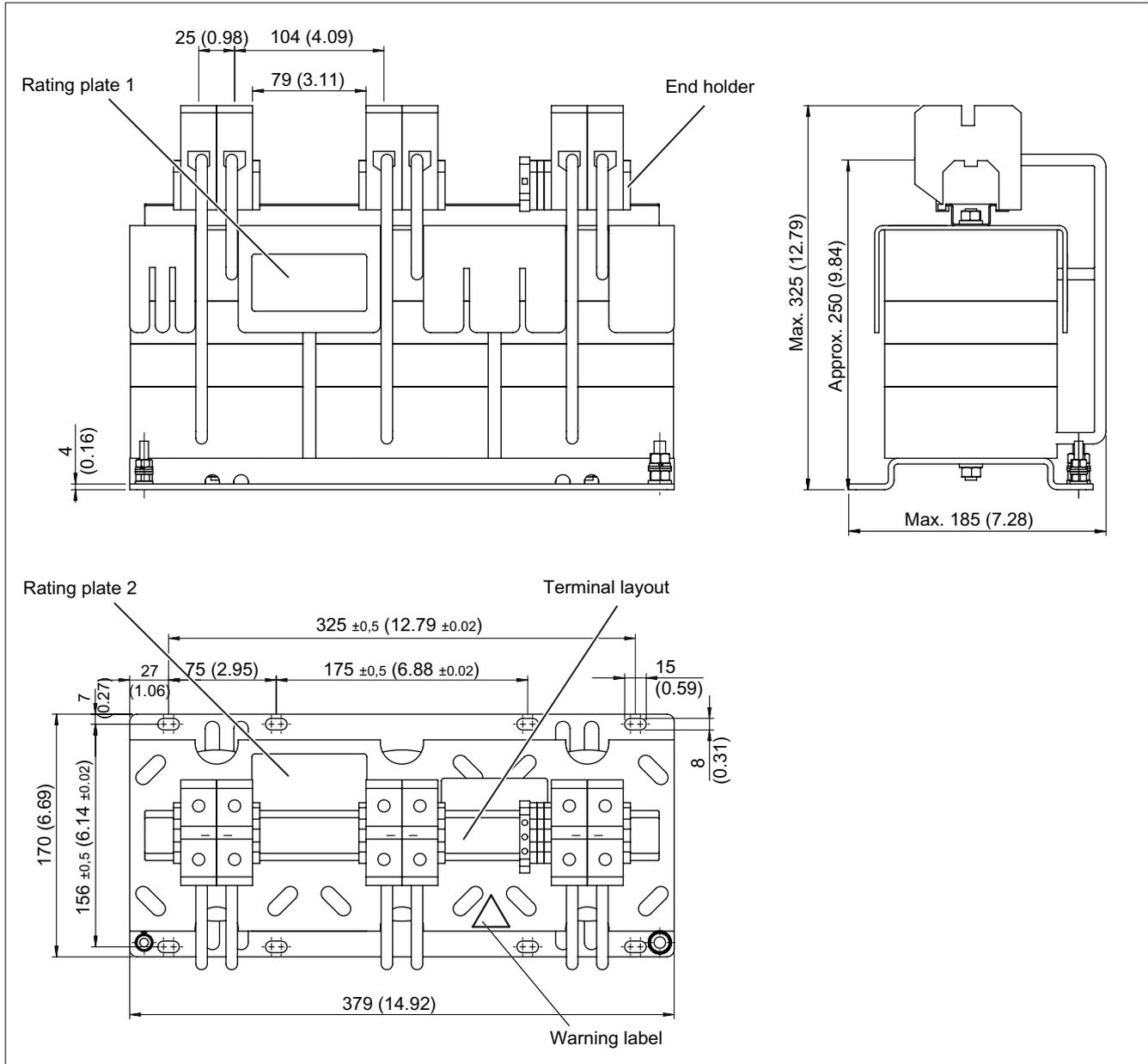
Figure 2-53 Dimension drawing of HFD line reactor 80 kW, all dimensions in mm and (inches)
