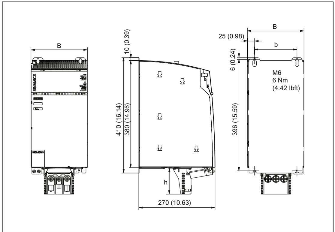
Figure 5-6 Dimension drawing of Motor Module in booksize format with internal air cooling 45 A to 85 A, all dimensions in mm and (inches)
