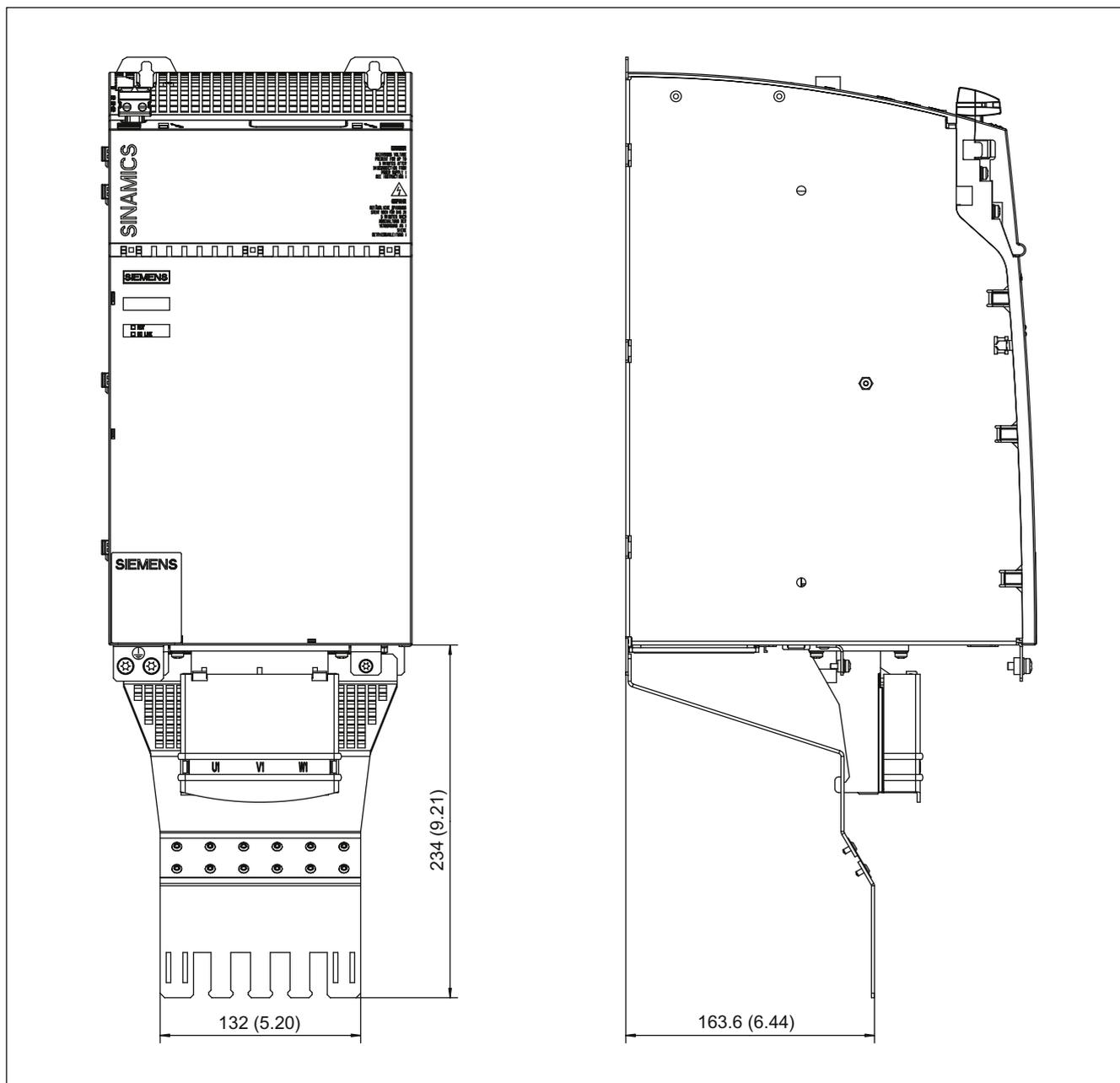
Figure 10-7 Dimension drawing of shield connecting plate on a 200 mm component with internal air cooling, all dimensions in mm and (inches)
