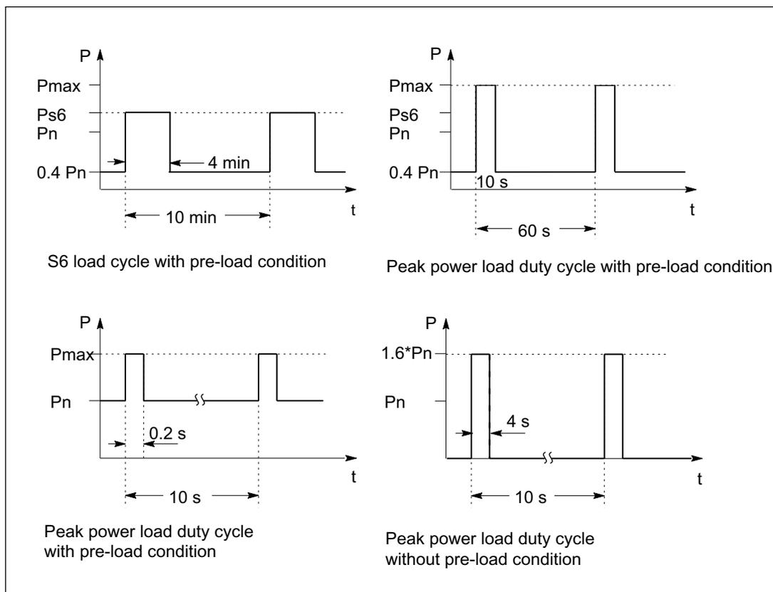
Figure 3-118 Rated duty cycles of Smart Line Modules
