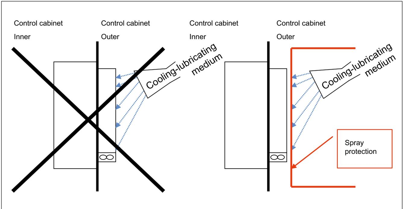
Figure 11-34 Spray protection for external cooling
