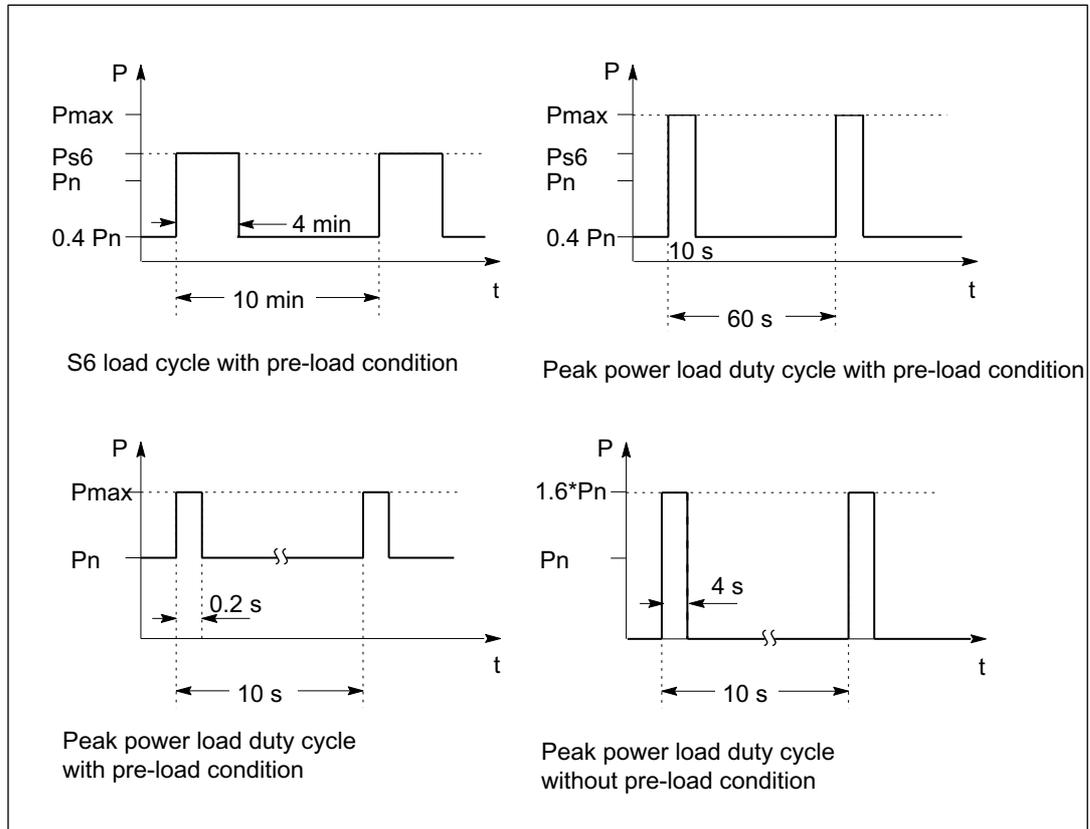
Figure 3-35 Rated duty cycles of Active Line Modules (**exception:** not applicable for 55 kW Active Line Module with Active Interface Module)
