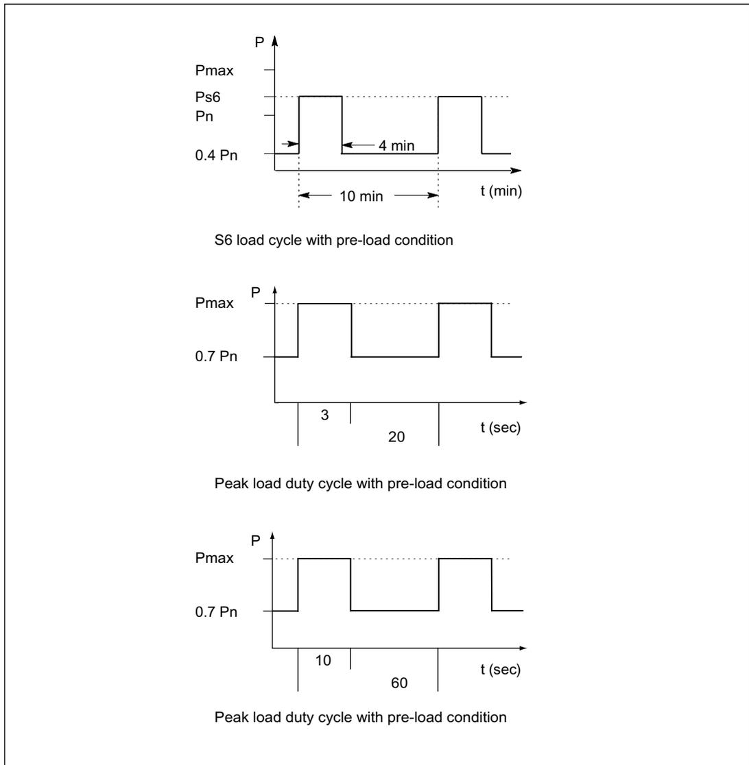
Figure 3-60 Rated duty cycles of 100 kW Basic Line Module
