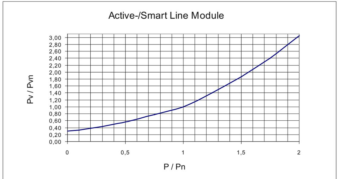
Figure 11-38 Losses in the partial load range for Active Line Modules and Smart Line Modules
