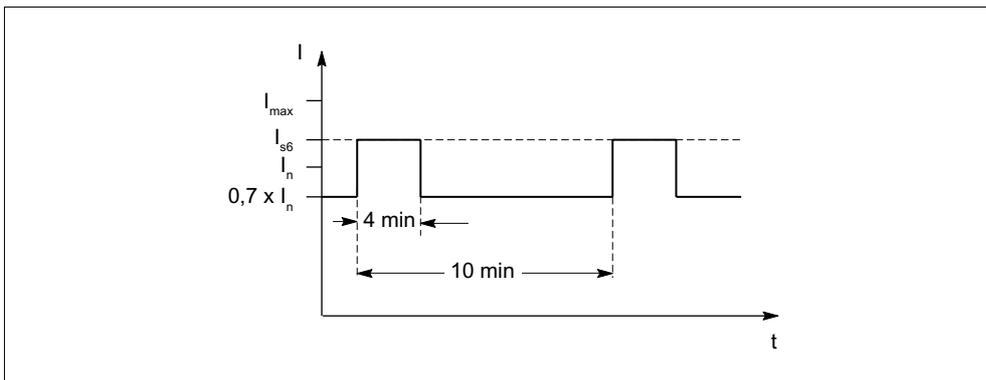
Figure 5-55 S6 duty cycle with initial load with a duty cycle duration of 600 s (for servo drives)
