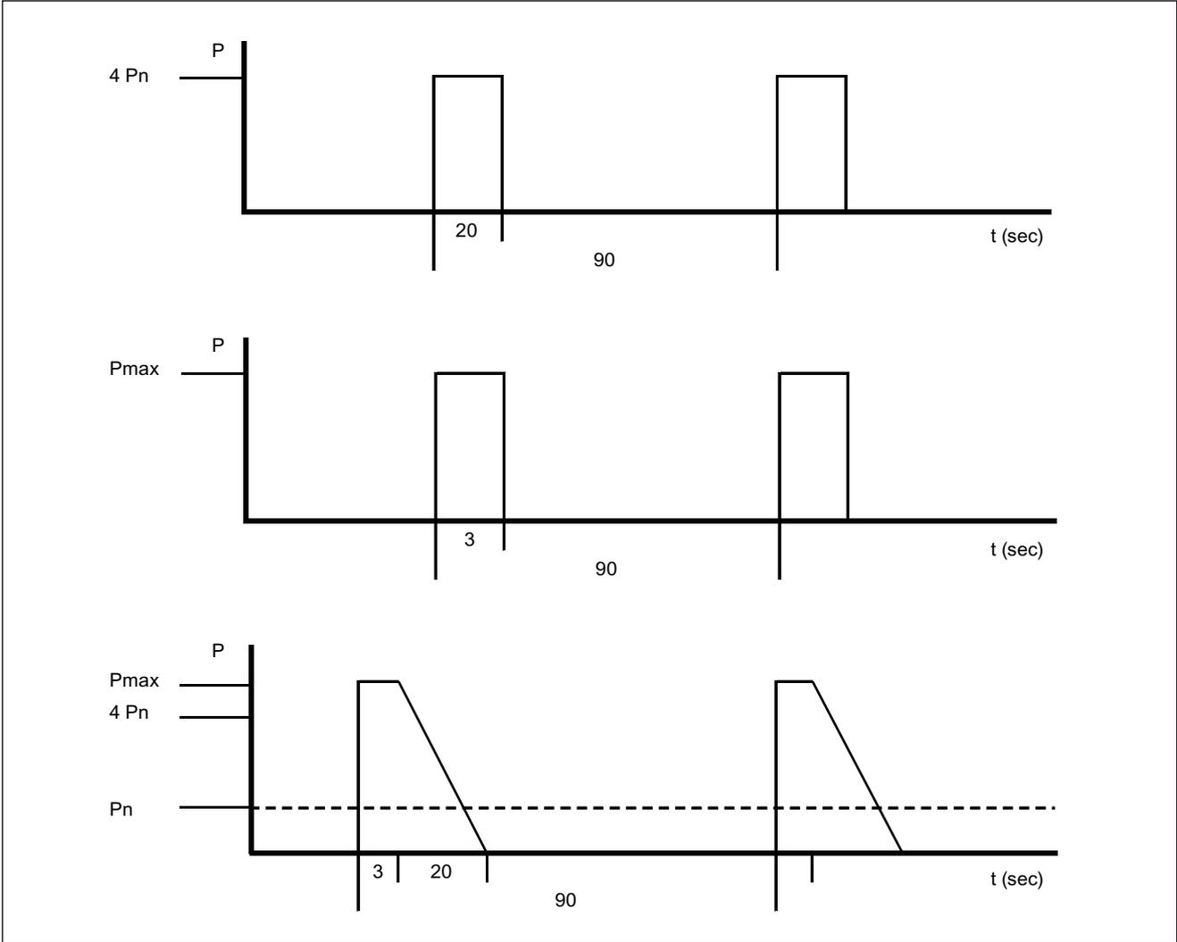
Figure 3-89 Braking duty cycles for braking resistors
