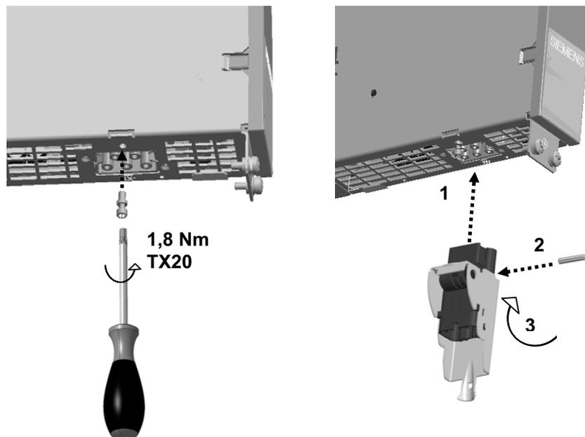
Figure 11-17 Installation example: Crimp plug
