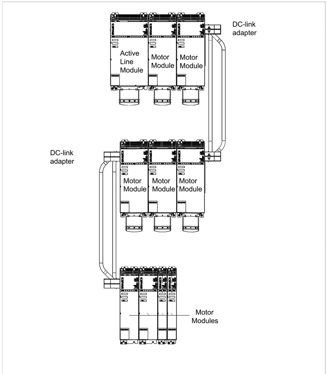
Figure 11-14 Example of a three-tier configuration with components between 50 and 200 mm wide
