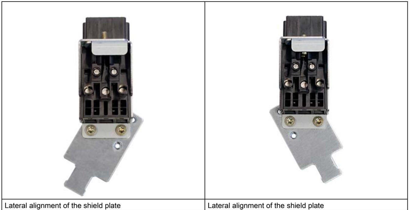
The shield plate supplied can be installed at a number of angles using the two (M4) screws provided (tightening torque 1.8 Nm).
