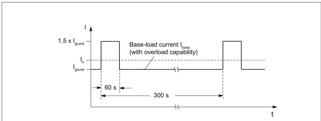
Figure 6-15 Duty cycle with 60 s overload with a duty cycle duration of 300 s
