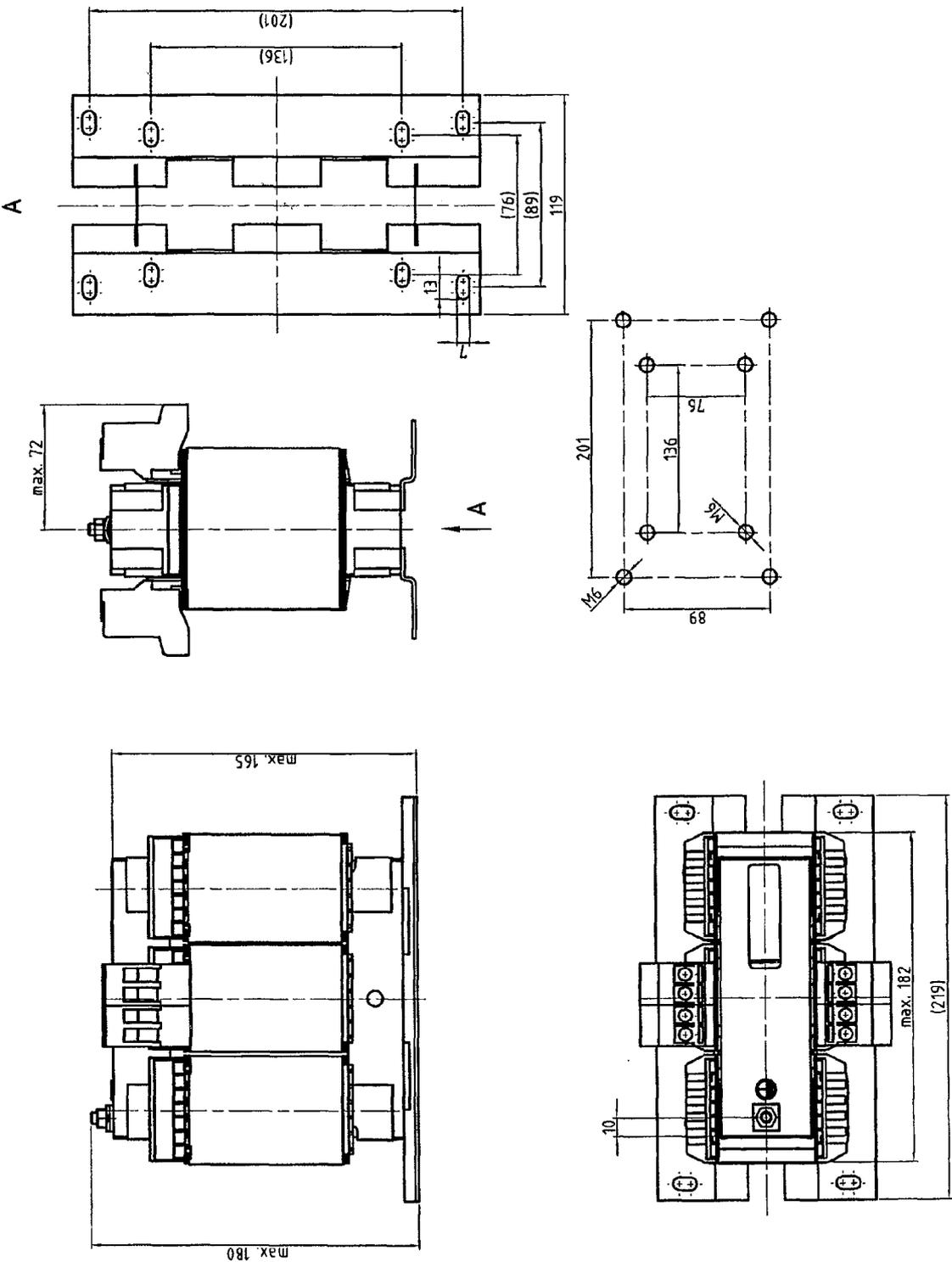
Figure 2-61 Dimension drawing of line reactor for the Smart Line Module 16 kW
