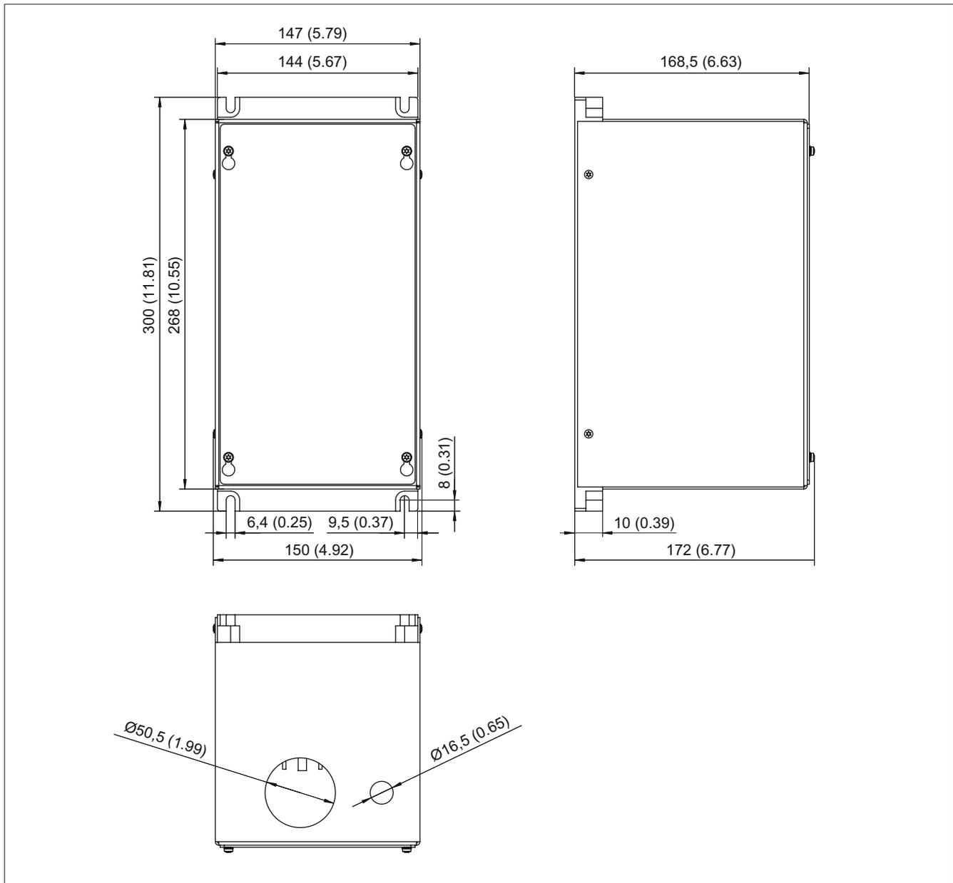
Figure 9-11 Dimension drawing of the Voltage Protection Module VPM120, all data in mm and (inches)
