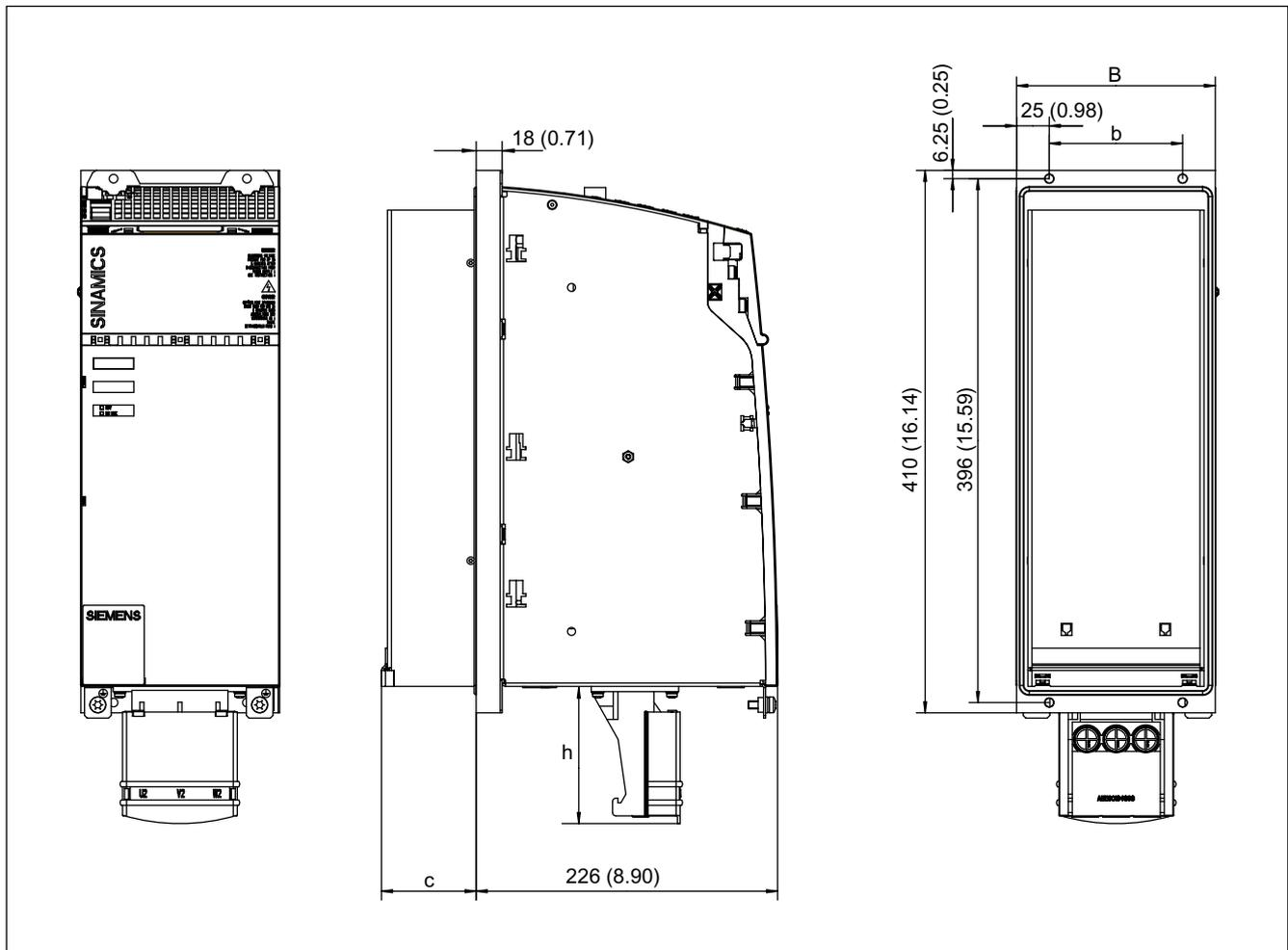
Figure 5-25 Dimension drawing of Motor Modules with external air cooling 45 A, 60 x 85 A, all dimensions in mm and (inches)
