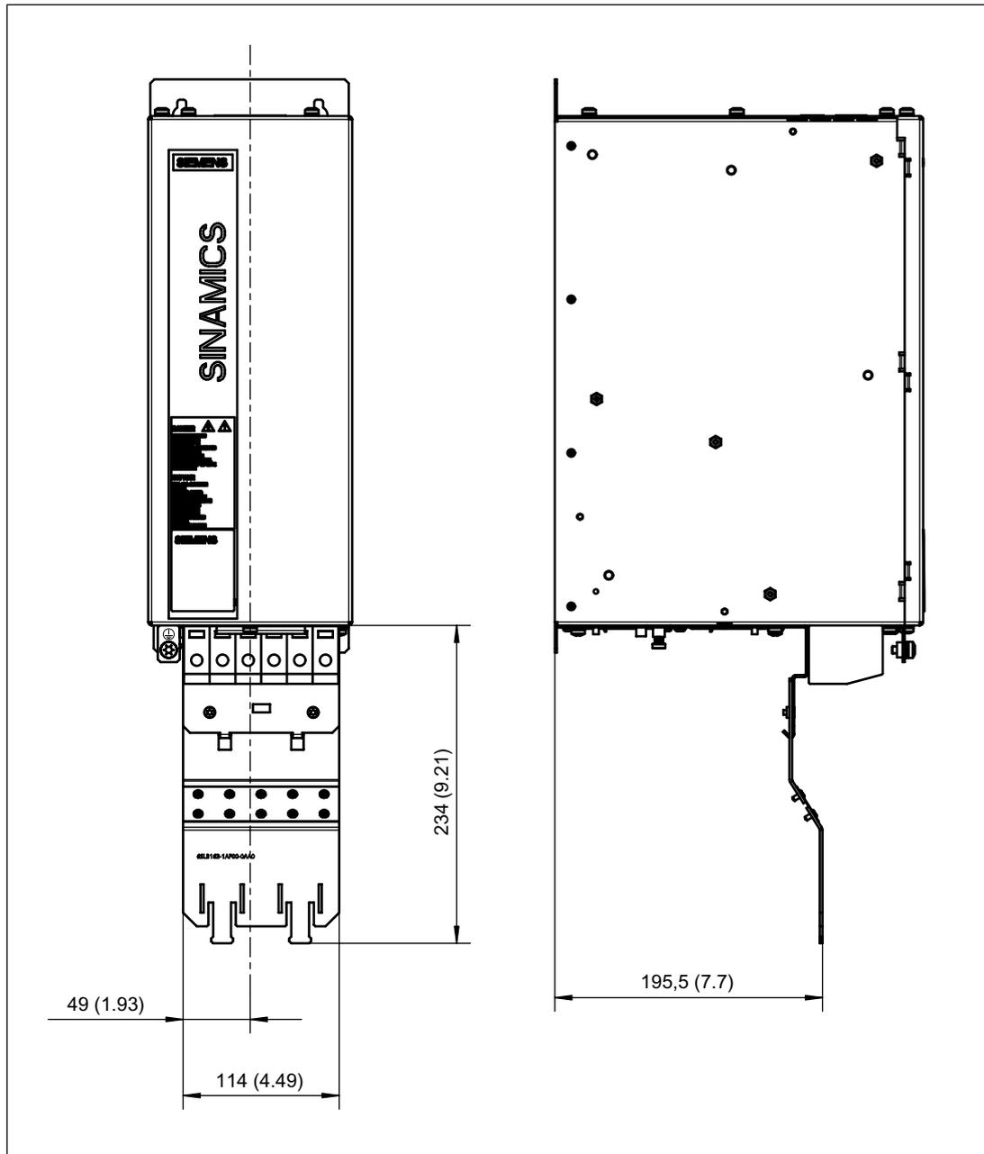
Figure 10-17 Dimension drawing of shield connecting plate on the 36 kW Active Interface Module, all dimensions in mm and (inches)
