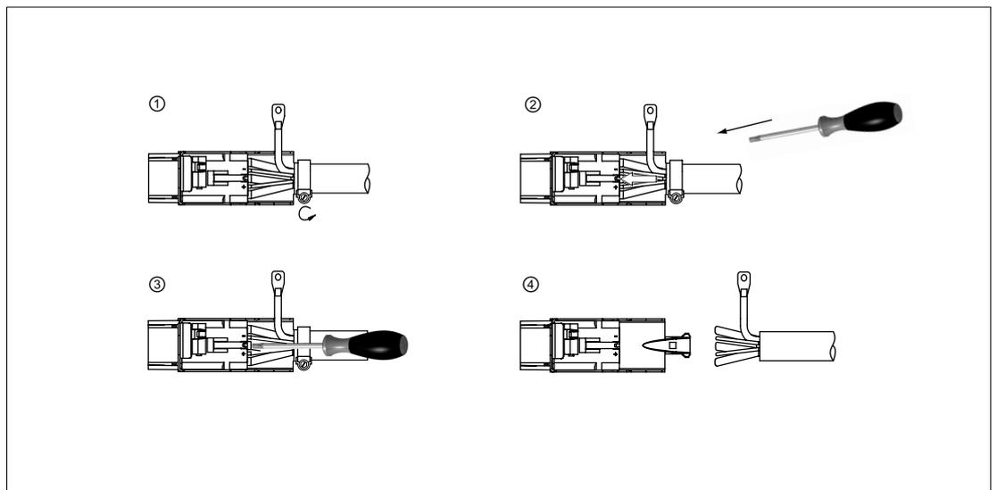
Figure 11-23 Removing the crimp plug with locking mechanism
