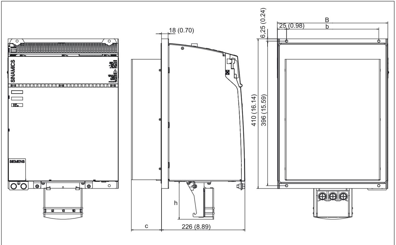
Figure 5-26 Dimension drawing of Motor Modules with external air cooling 132 A and 200 A, all dimensions in mm and (inches)
