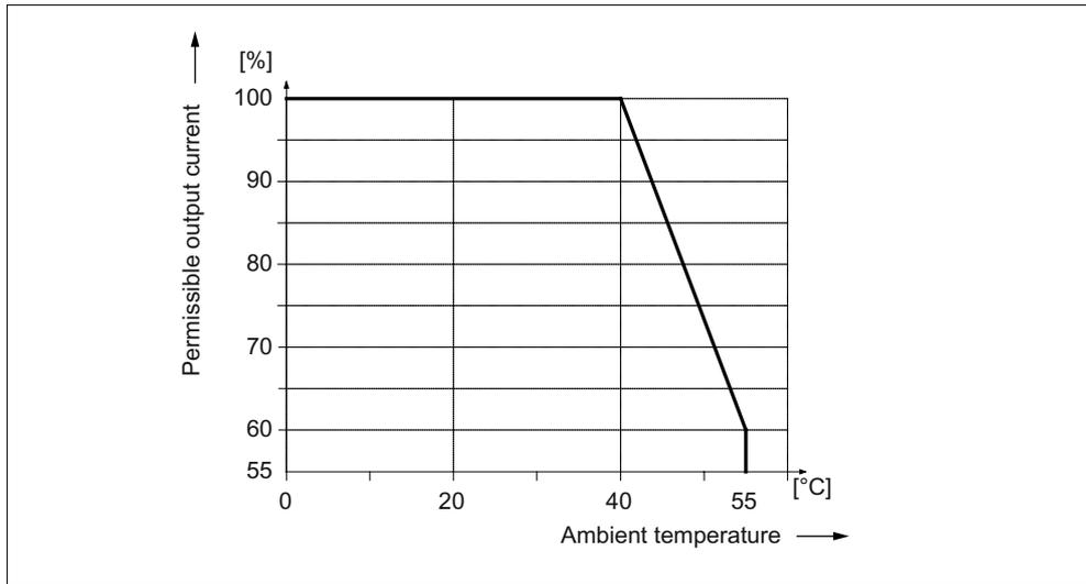
Figure 5-15 Output current as a function of the ambient temperature
