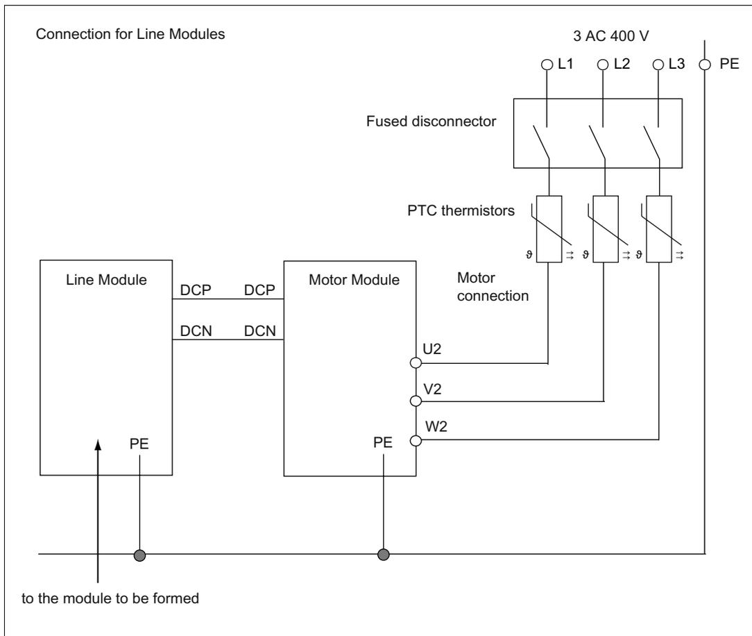
Figure 13-2 Forming circuit for Line Modules with PTC resistors
