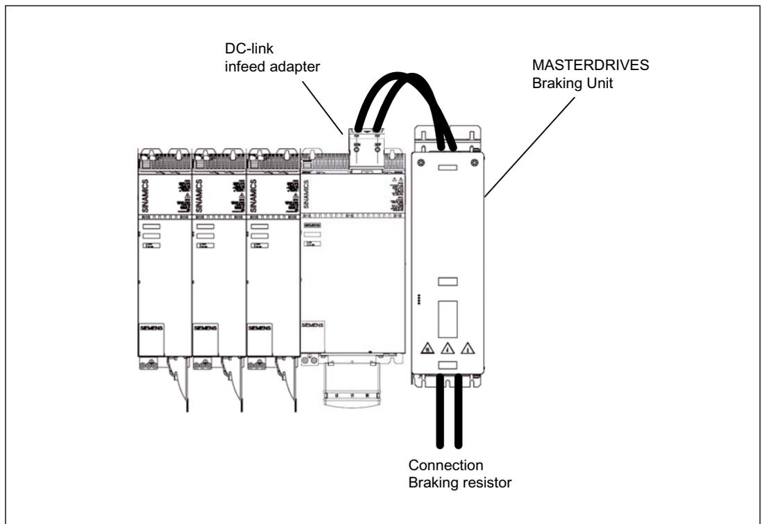
Figure 3-68 Connection of the MASTERDRIVES braking unit
