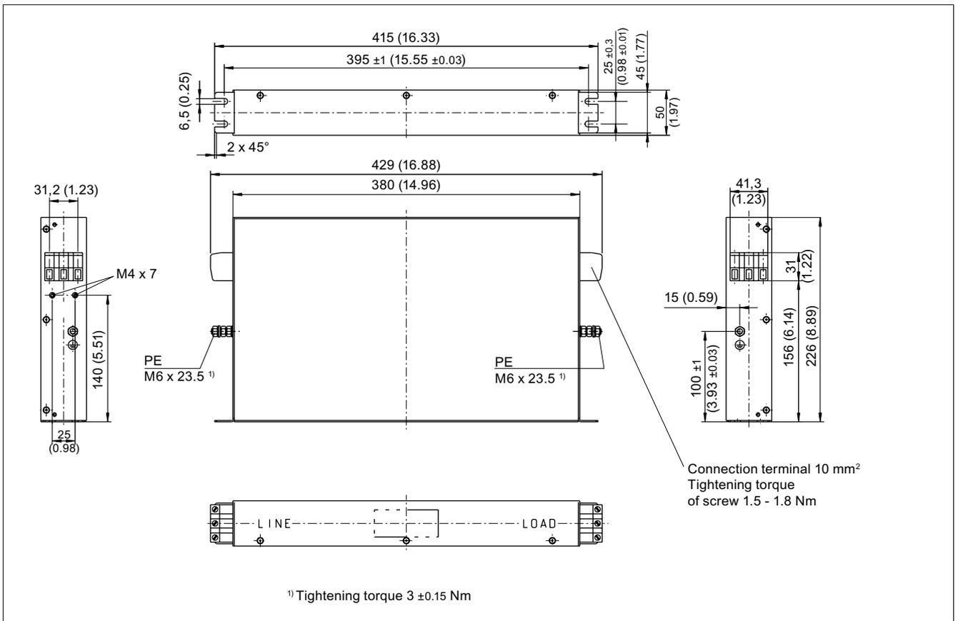
Figure 2-12 Dimension drawing of Basic Line Filter 16 kW, order number 6SL3000-0BE21-6DAx, all dimensions in mm and (inches)
