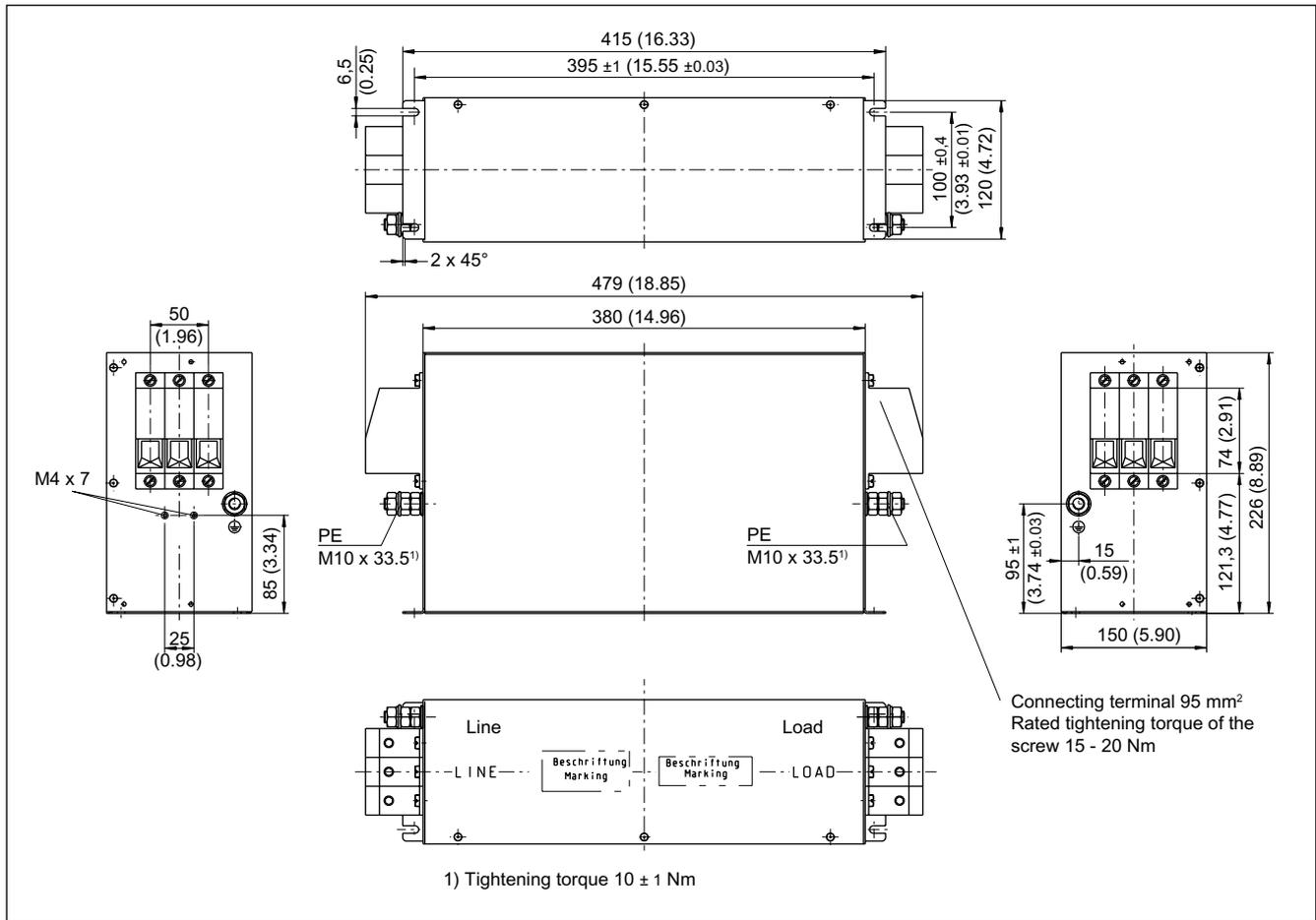
Figure 2-25 Dimension drawing of Basic Line Filter for Basic Line Modules 100 kW, order number 6SL3000-0BE31-2DAx, all dimensions in mm and (inches)
