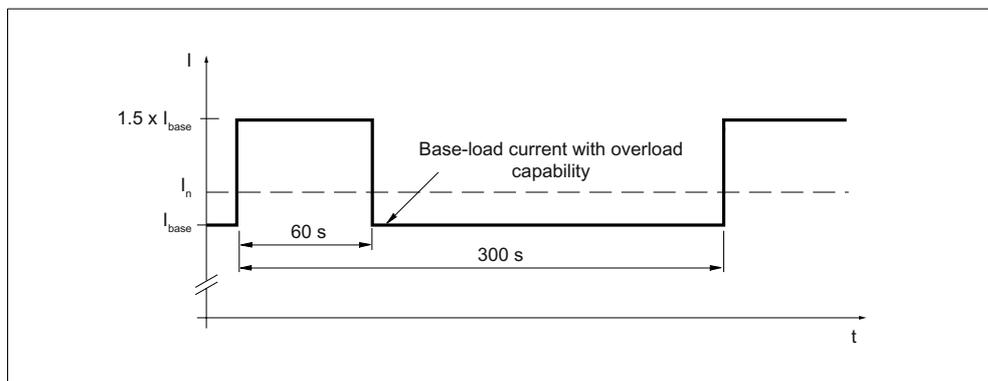
Figure 5-58 Duty cycle with 60 s overload with a duty cycle duration of 300 s
