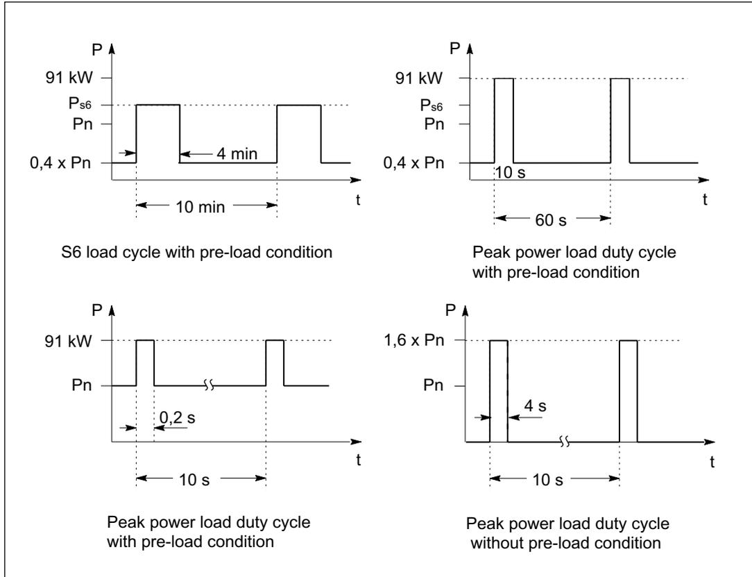
Figure 3-25 Rated duty cycles of 55 kW Active Line Modules with Active Interface Module
