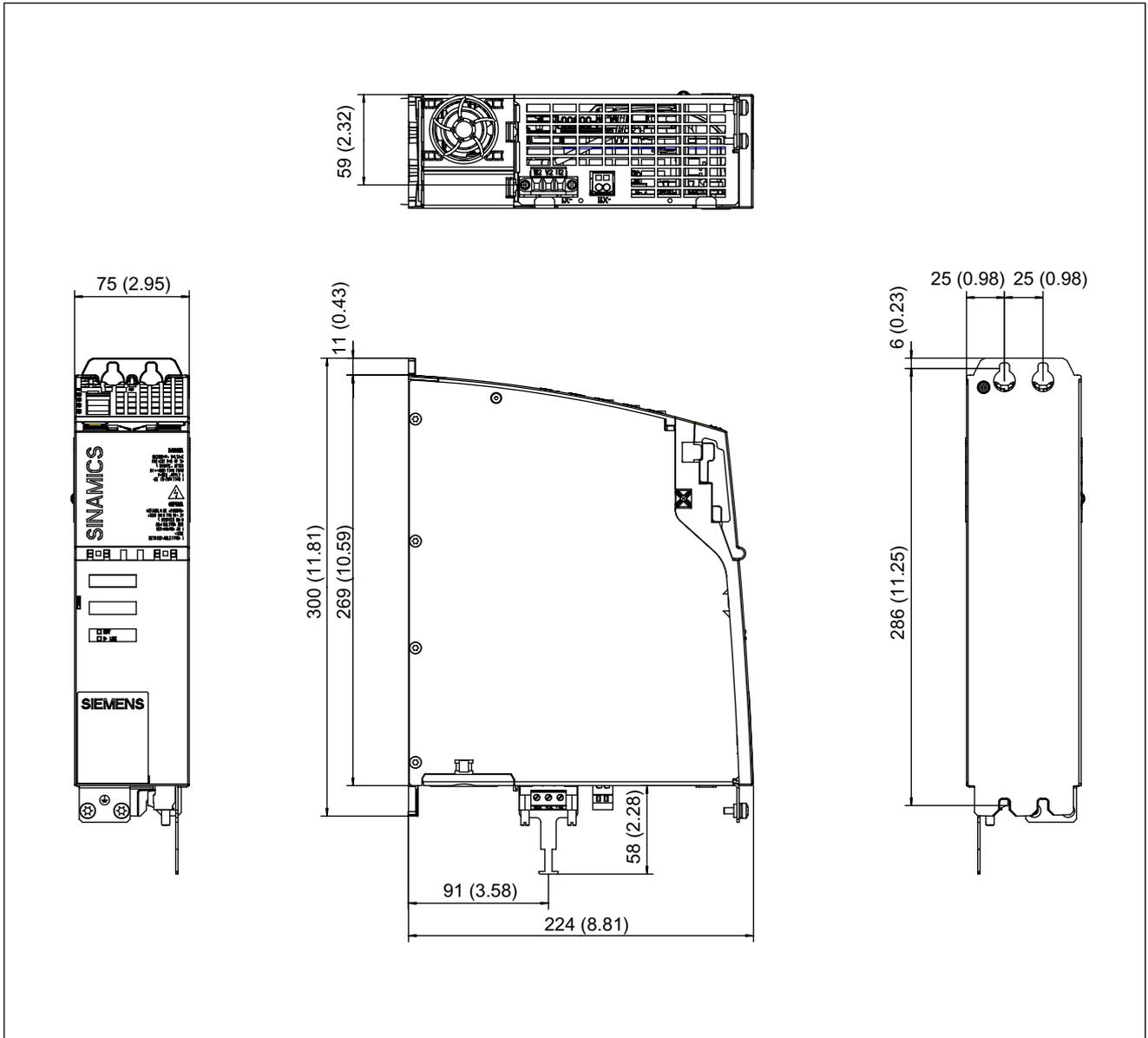
Figure 6-6 Dimension drawing of Motor Module in booksize compact format 18 A, all dimensions in mm and (inches)
