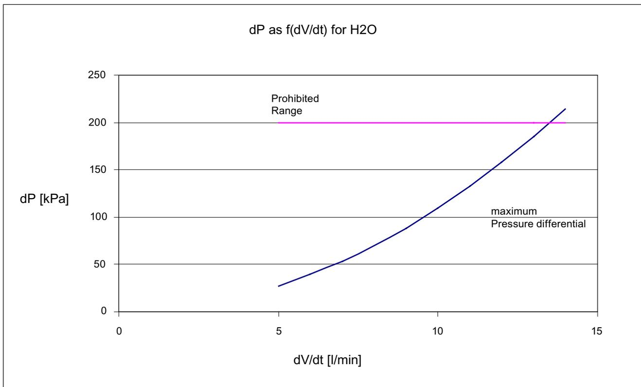
Figure 12-2 Pressure difference as a function of volumetric flow
