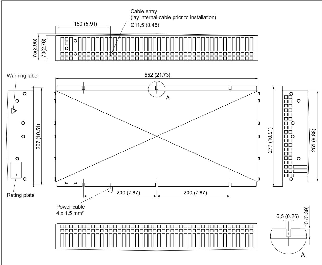
Figure 2-56 800 W damping resistor for HFD line reactors, all dimensions in mm and (inches)
