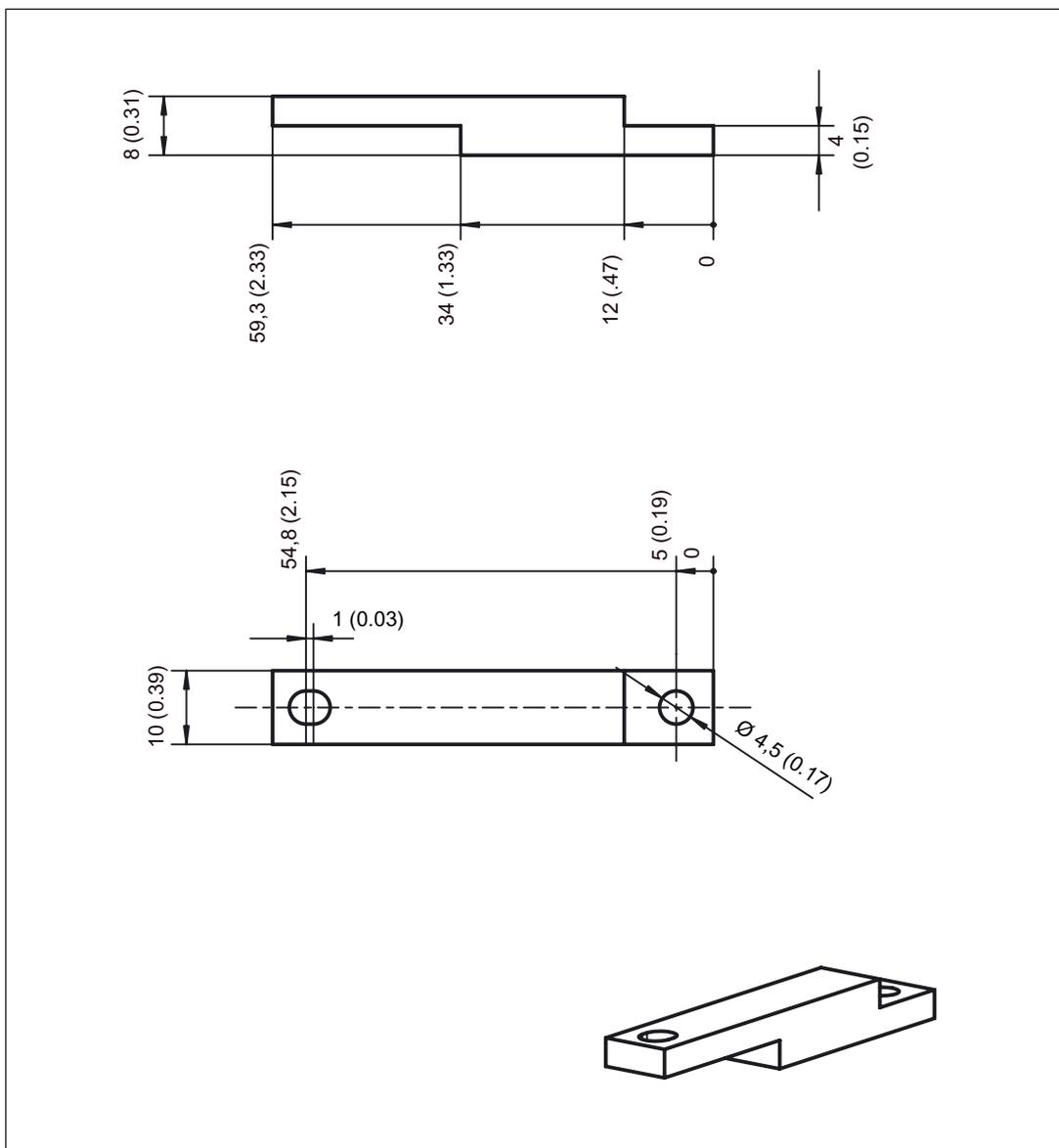
Figure 10-25 Dimension drawing of reinforced DC-link busbar 50 mm, all dimensions in mm and (inches)
