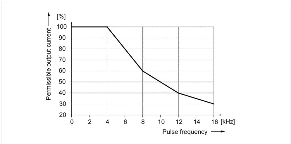
Figure 5-60 Output current as a function of the pulse frequency
