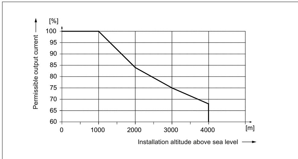
Figure 5-18 Output current as a function of the installation altitude
