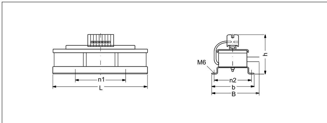
Figure 2-43 Dimension drawing of HF line reactor for Active Line Modules up to 55 kW
