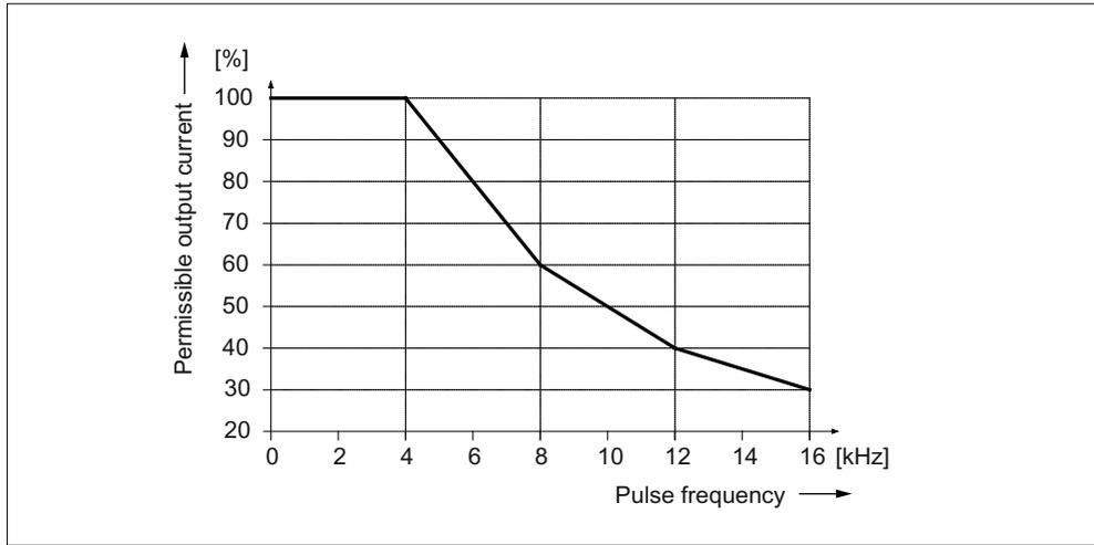
Figure 5-76 Output current as a function of the pulse frequency
