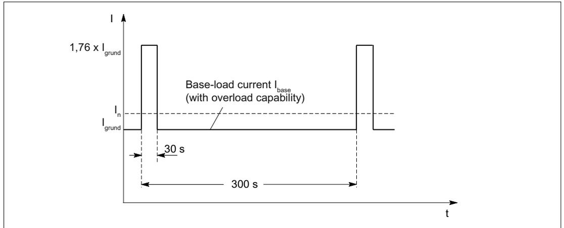
Figure 6-16 Duty cycle with 30 s overload with a duty cycle duration of 300 s
