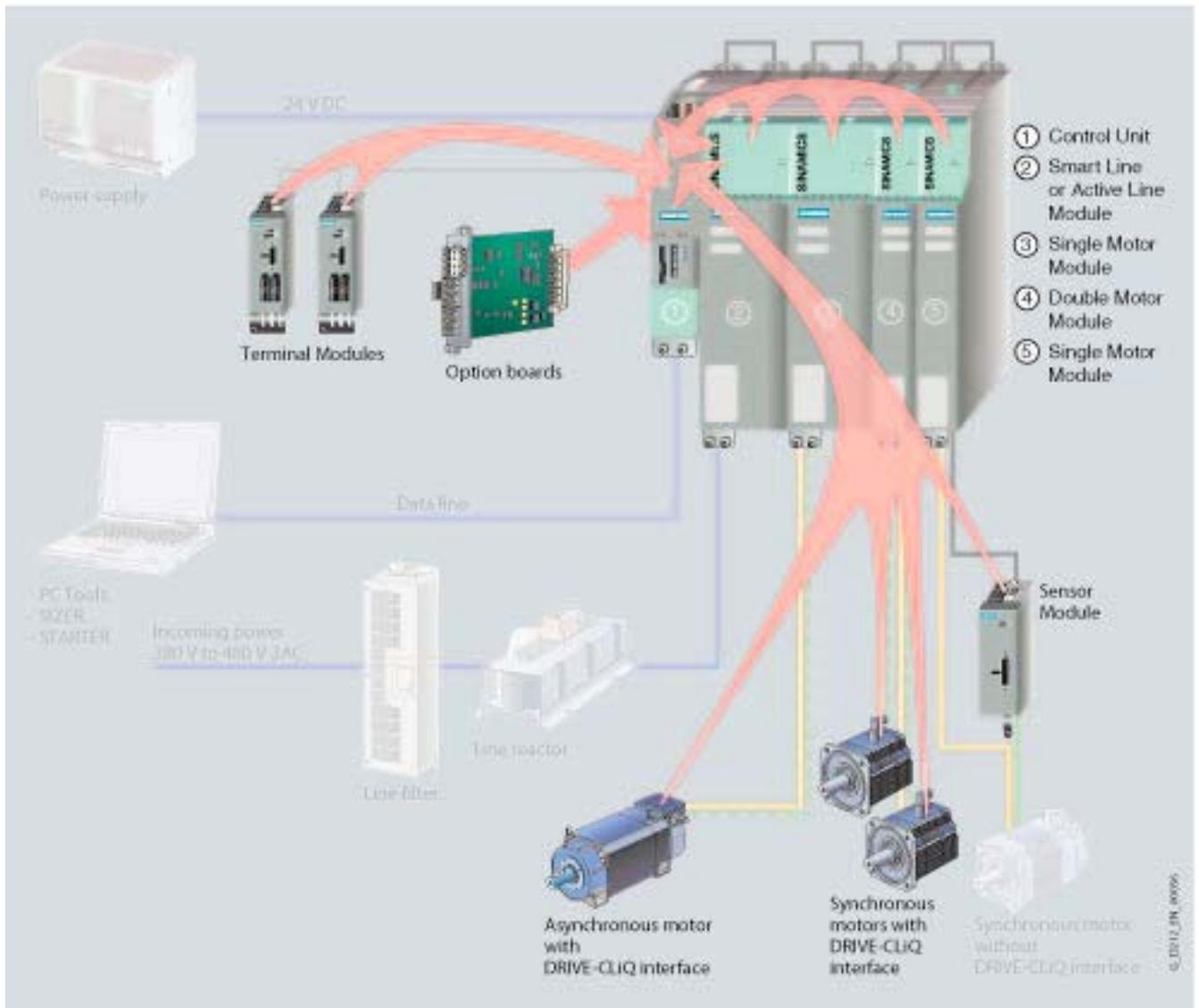
Figure 1-4 The electronic rating plate for SINAMICS S120
