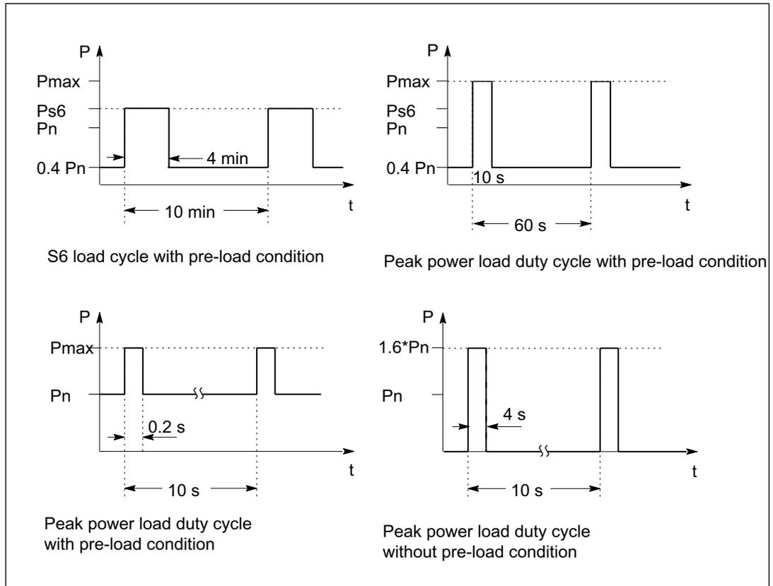
Figure 3-24 Rated duty cycles of Active Line Modules (**exception:** not applicable for 55 kW Active Line Module with Active Interface Module)
