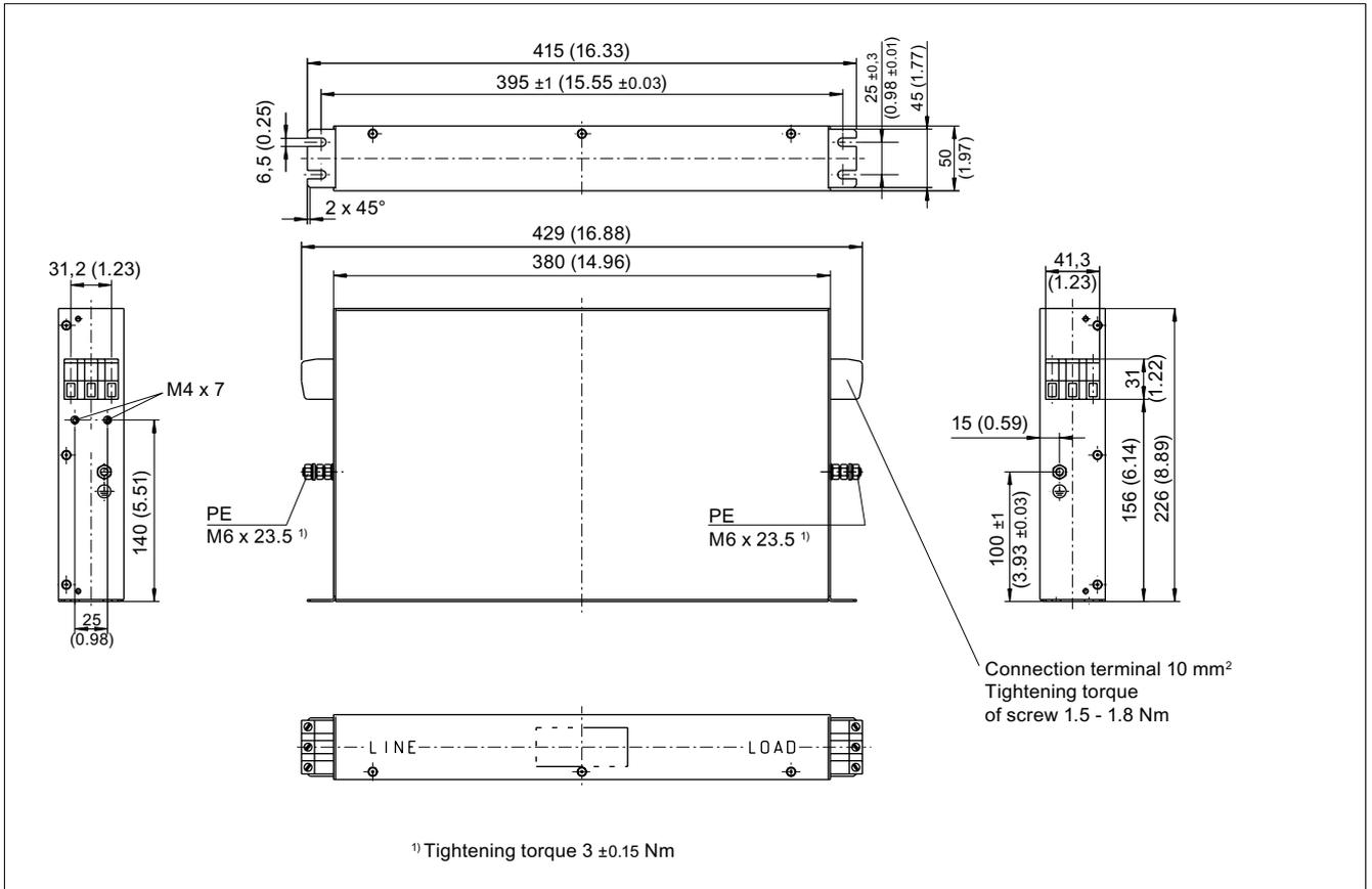
Figure 2-5 Dimension drawing of Basic Line Filter 16 kW, order number 6SL3000-0BE21-6DAx, all dimensions in mm and (inches)
