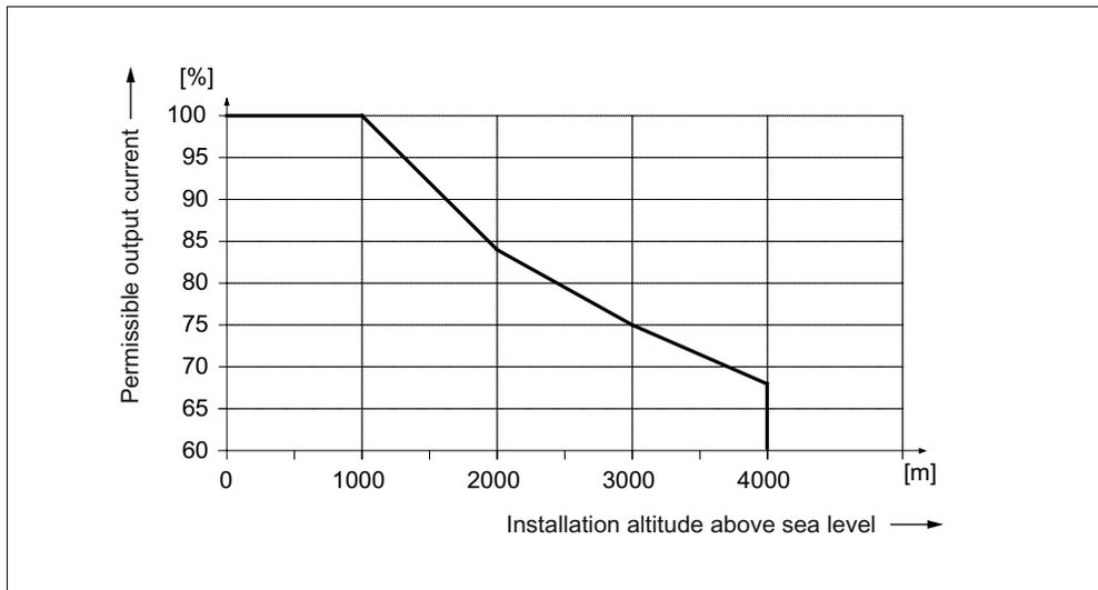
Figure 3-112 Output current as a function of the installation altitude
