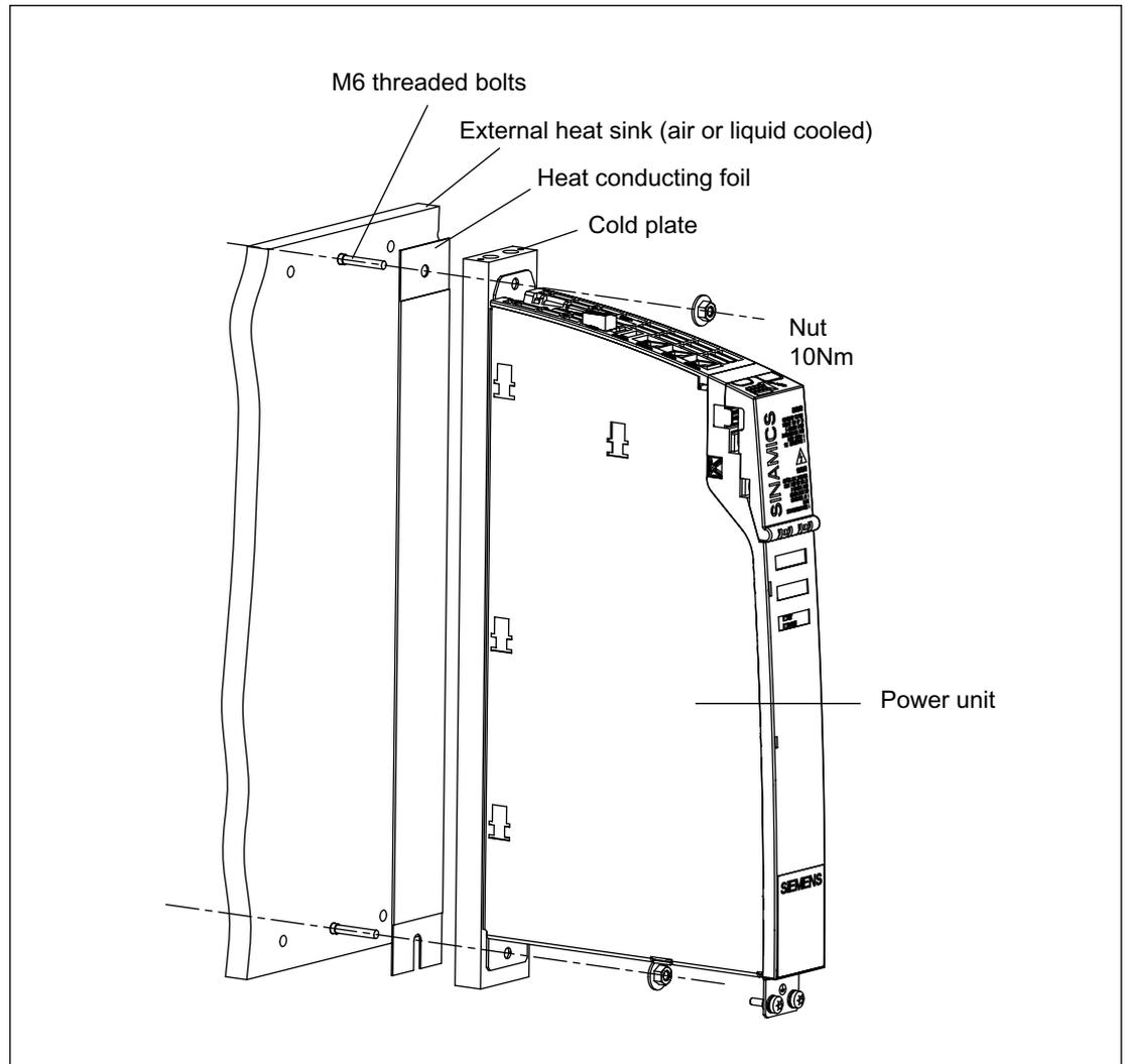
Figure 3-117 Installation of a cold-plate power unit with an external heat sink
