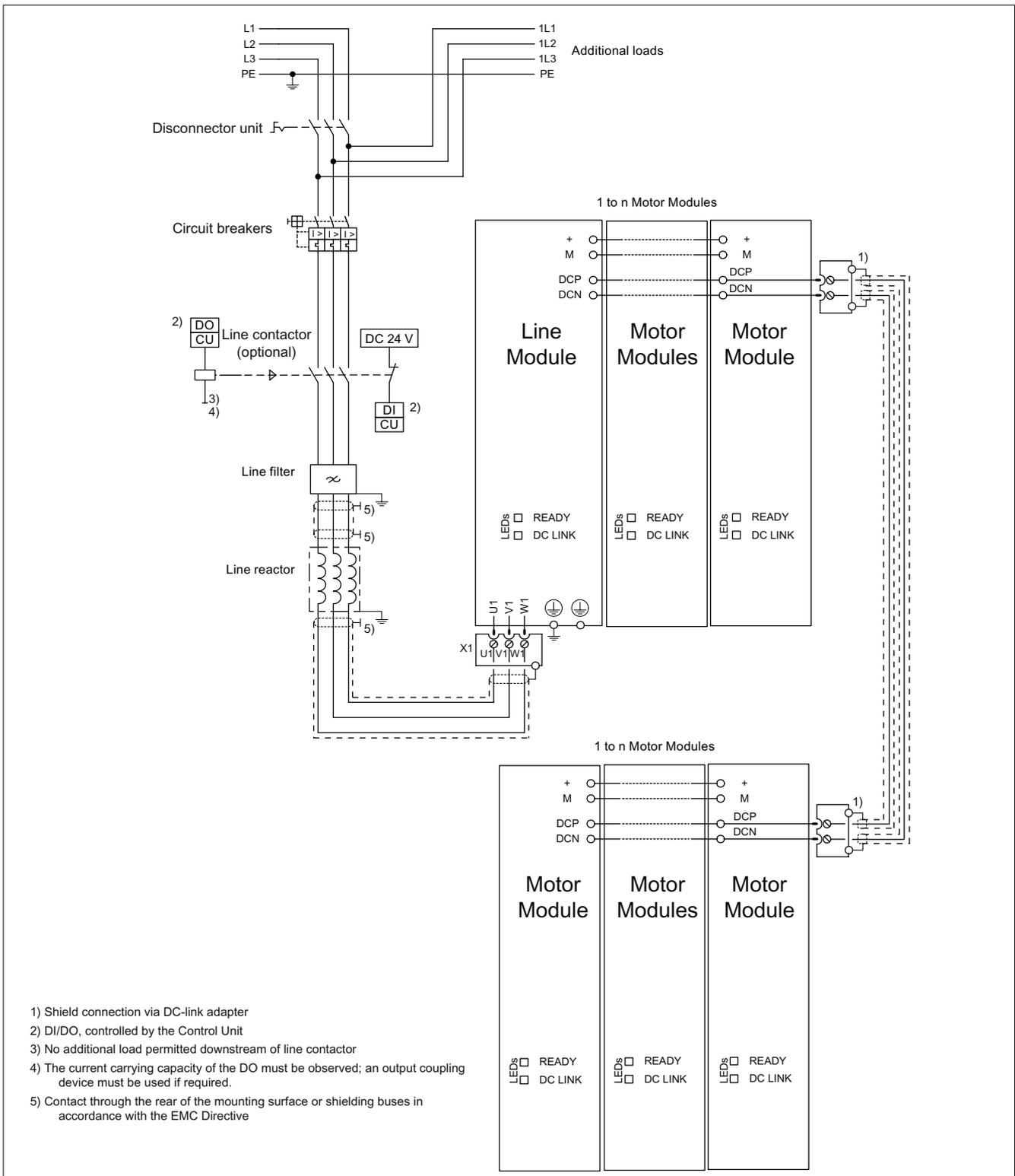
Figure 11-13 Connection example of a two-tier drive line-up
