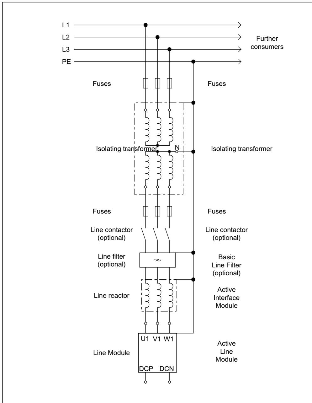
Figure 2-72 Isolating transformer
