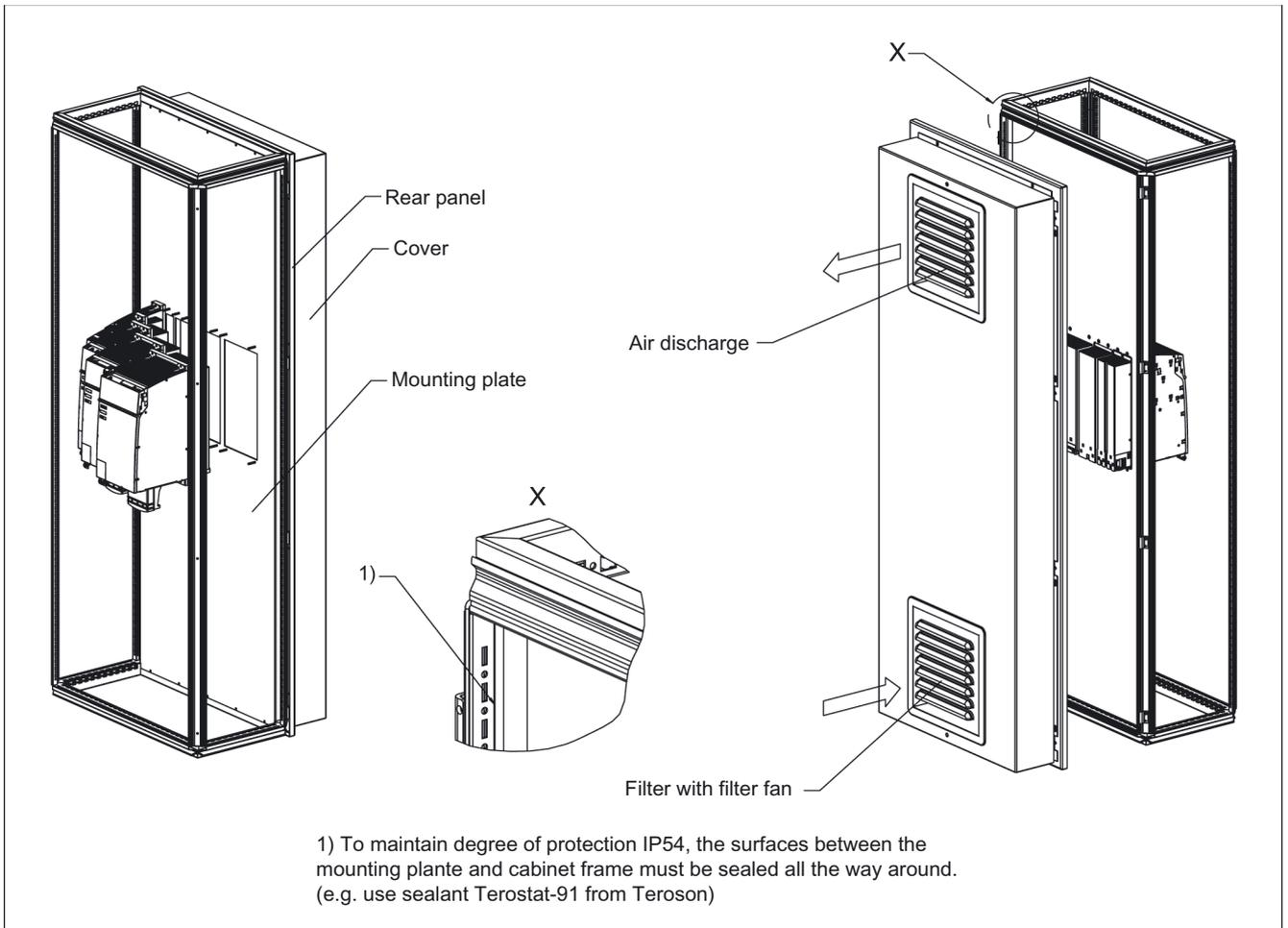
Figure 5-32 Example 1: installation in cabinet with mounting plate
