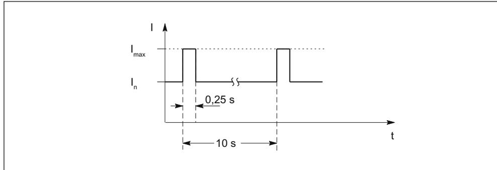
Figure 5-68 Duty cycle with initial load (for servo drives)
