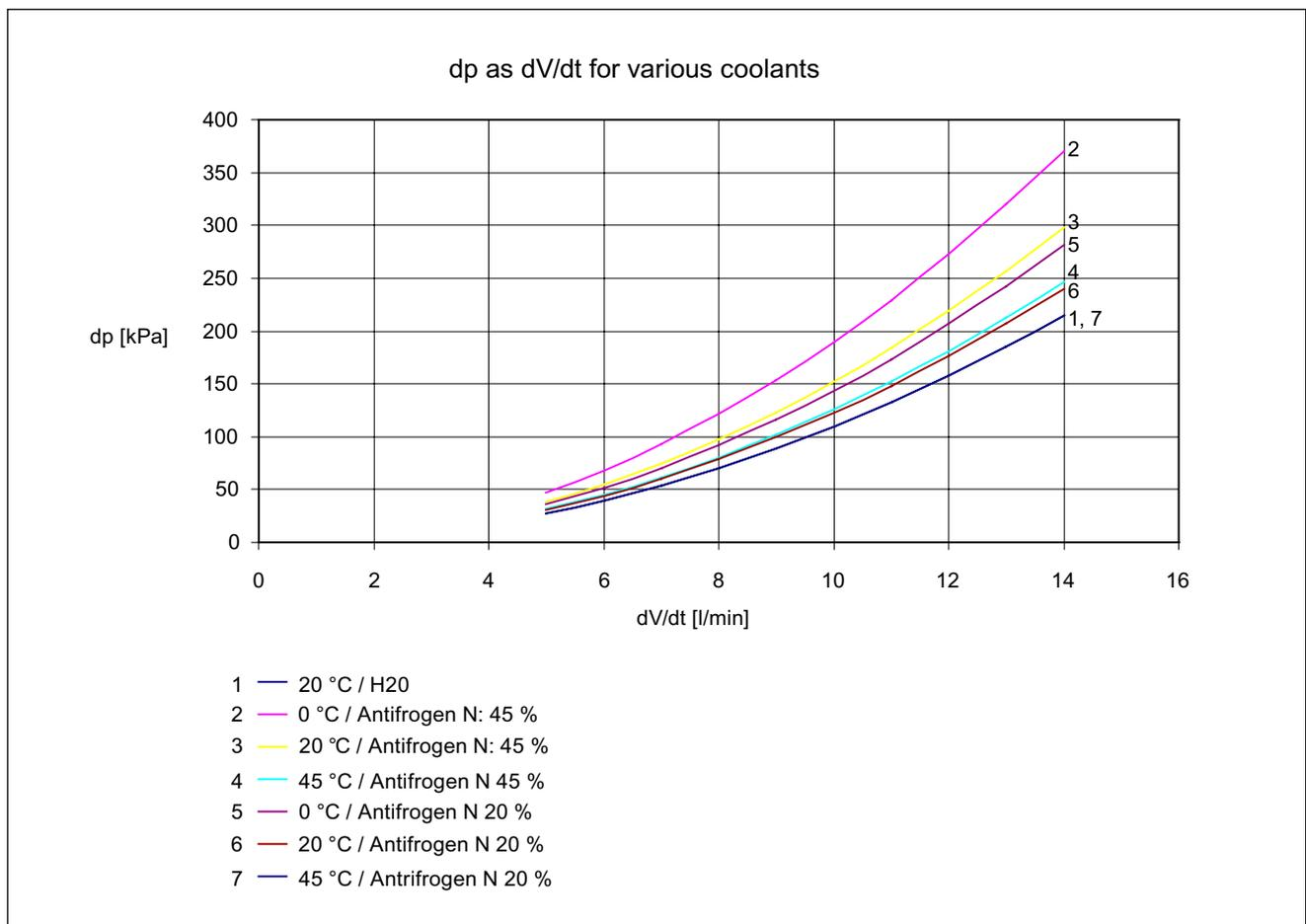
Figure 12-3 Pressure difference as a function of volumetric flow
