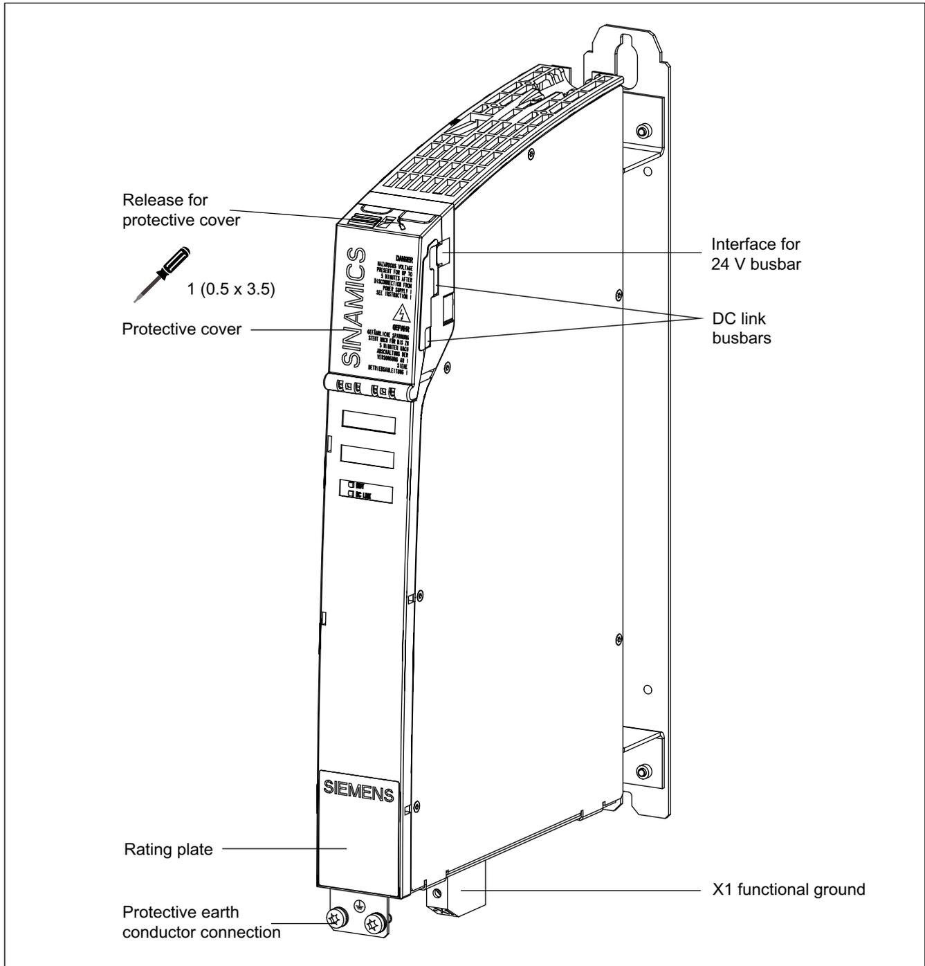
Figure 8-14 Interface description: Voltage Clamping Module
