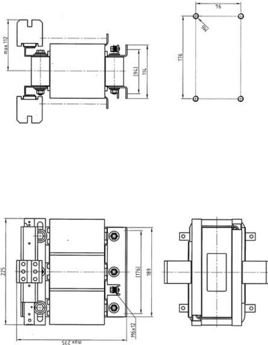
Figure 2-62 Dimension drawing of the line reactor for the Smart Line Module 36 kW
