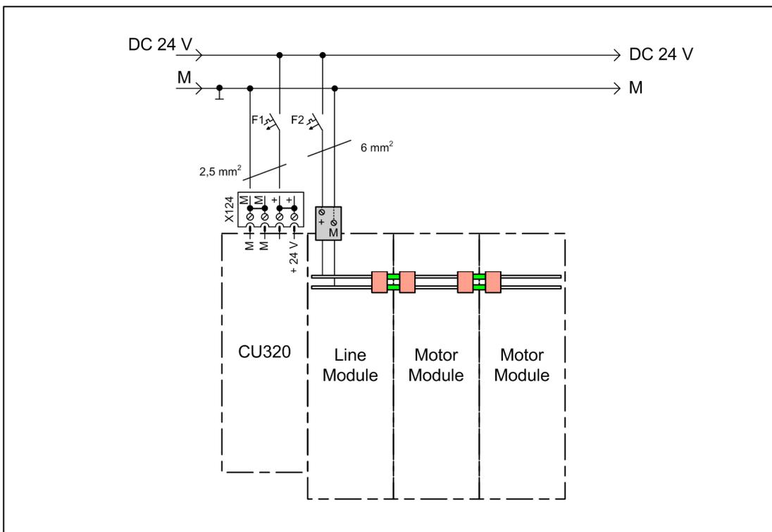
Figure 11-5 Example of 24 VDC fuse protection
