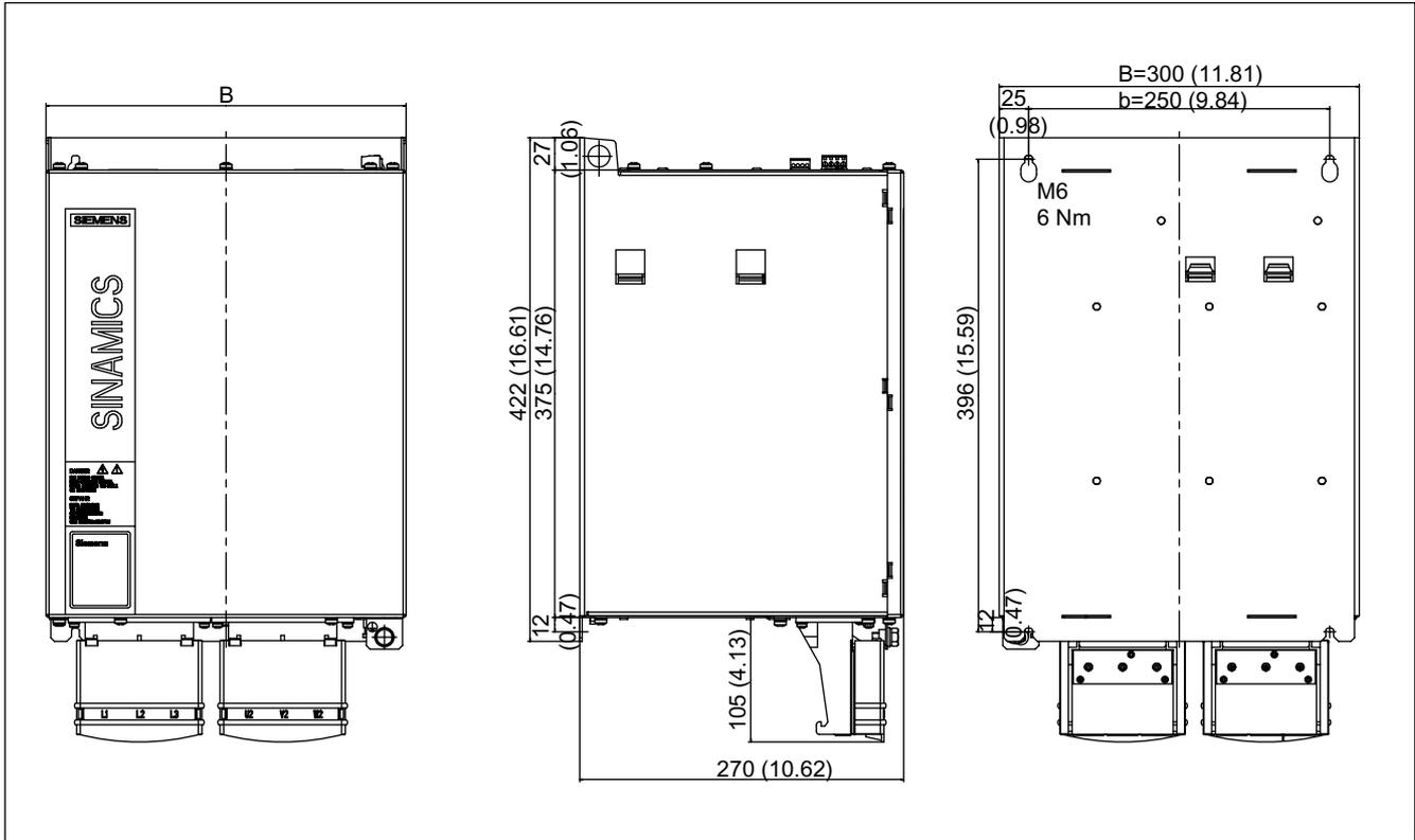
Figure 2-38 Dimension drawing of Active Interface Module 80 kW and 120 kW, all dimensions in mm and (inches)
