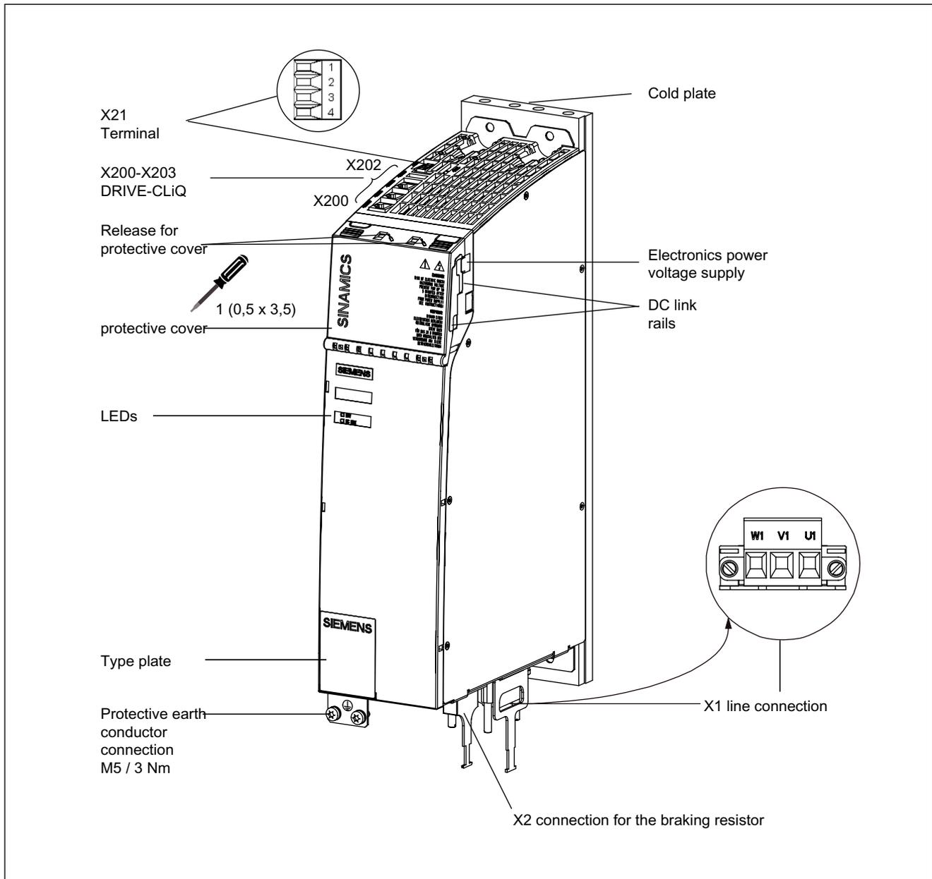
Figure 3-71 Basic Line Module with cold plate (20 kW)
