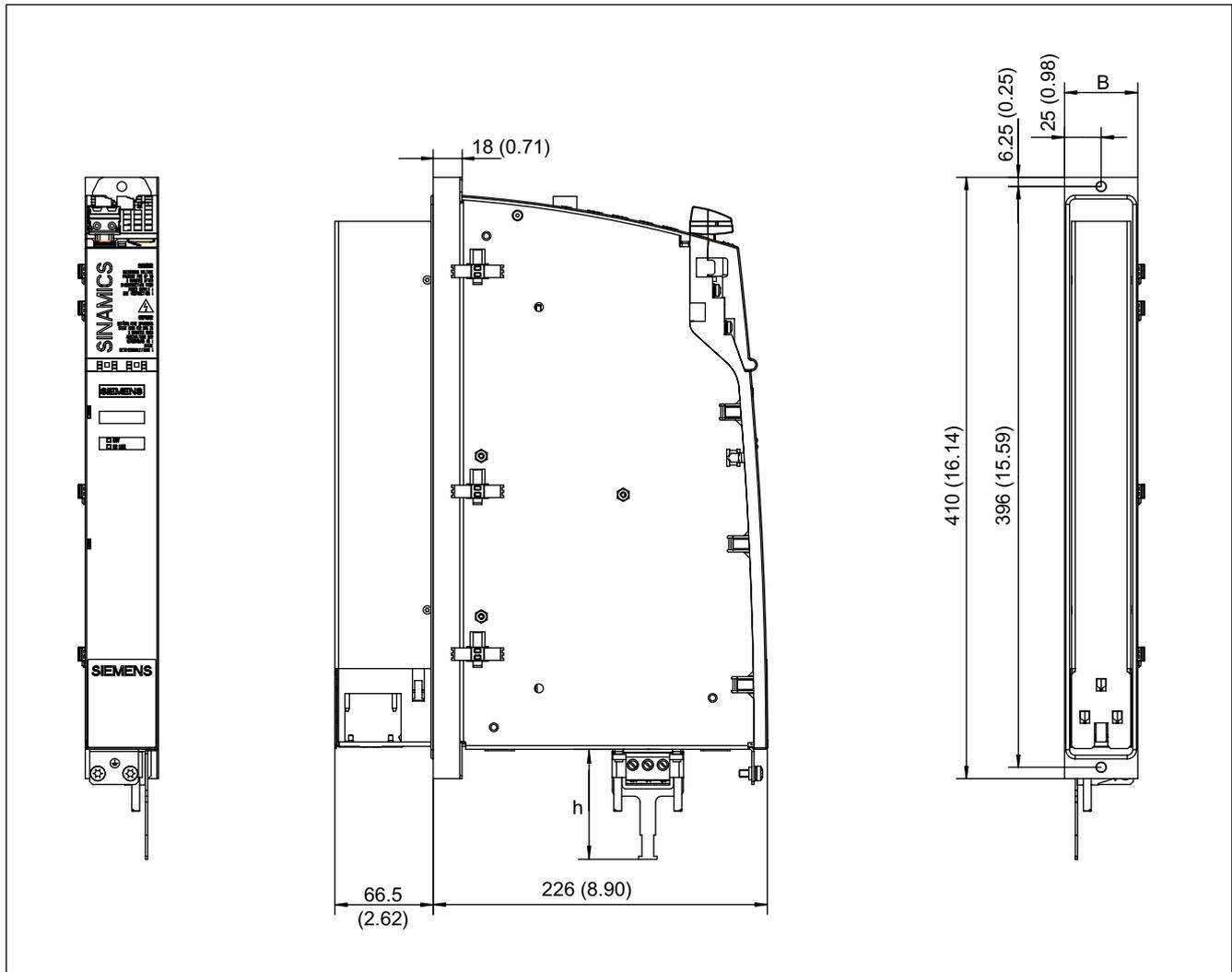
Figure 3-104 Dimension drawing of Smart Line Modules 5 kW and 10 kW with external air cooling, all data in mm and (inches)
