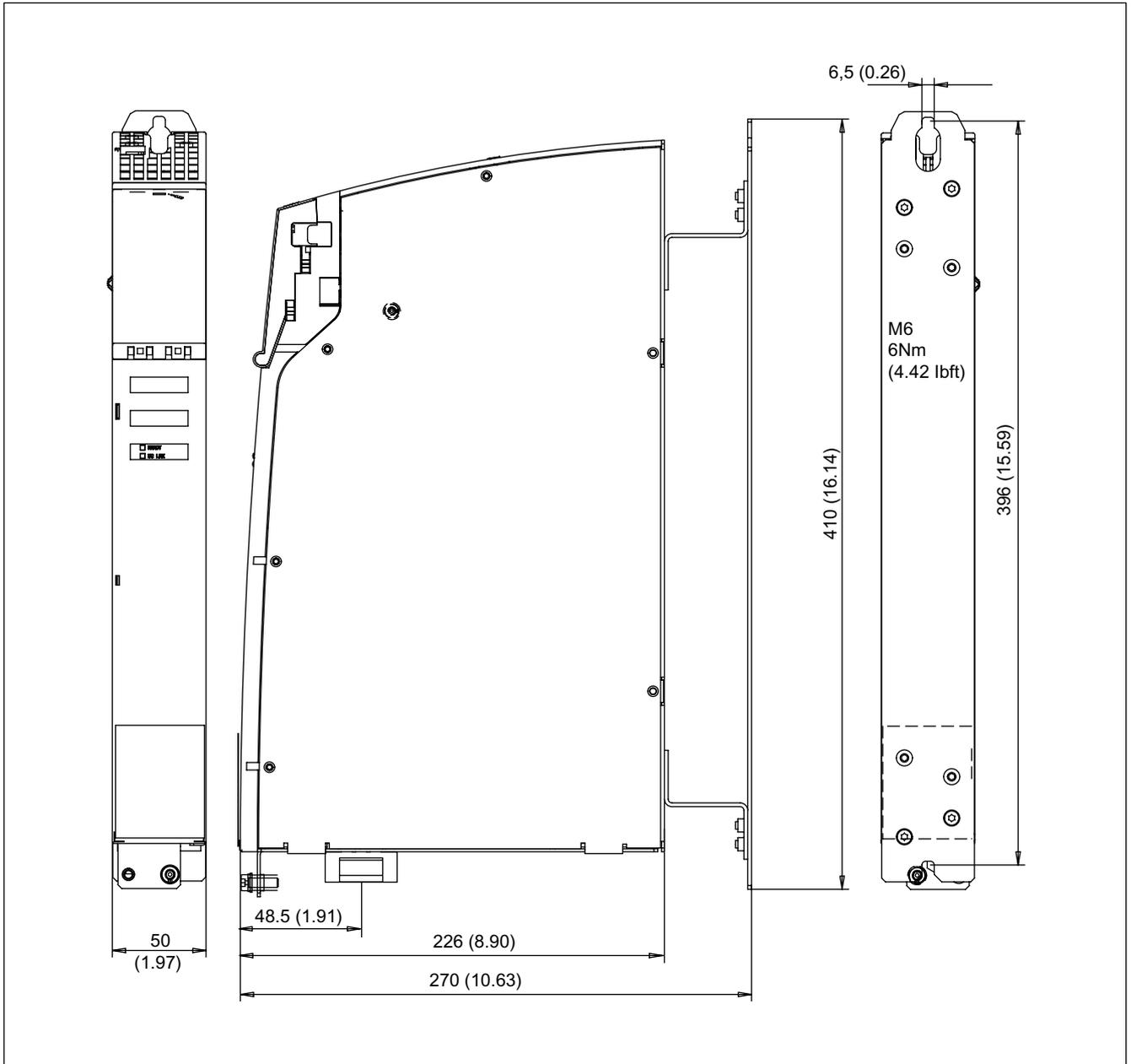
Figure 8-13 Dimension Control Supply Module, all dimensions in mm and (inches)
