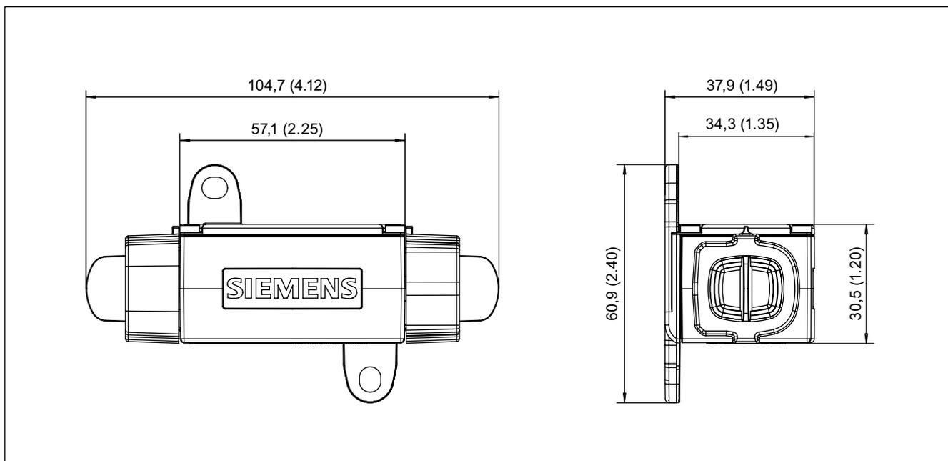
Figure 10-32 Dimension drawing of the DRIVE-CLiQ coupling, all dimensions in mm and (inches)
