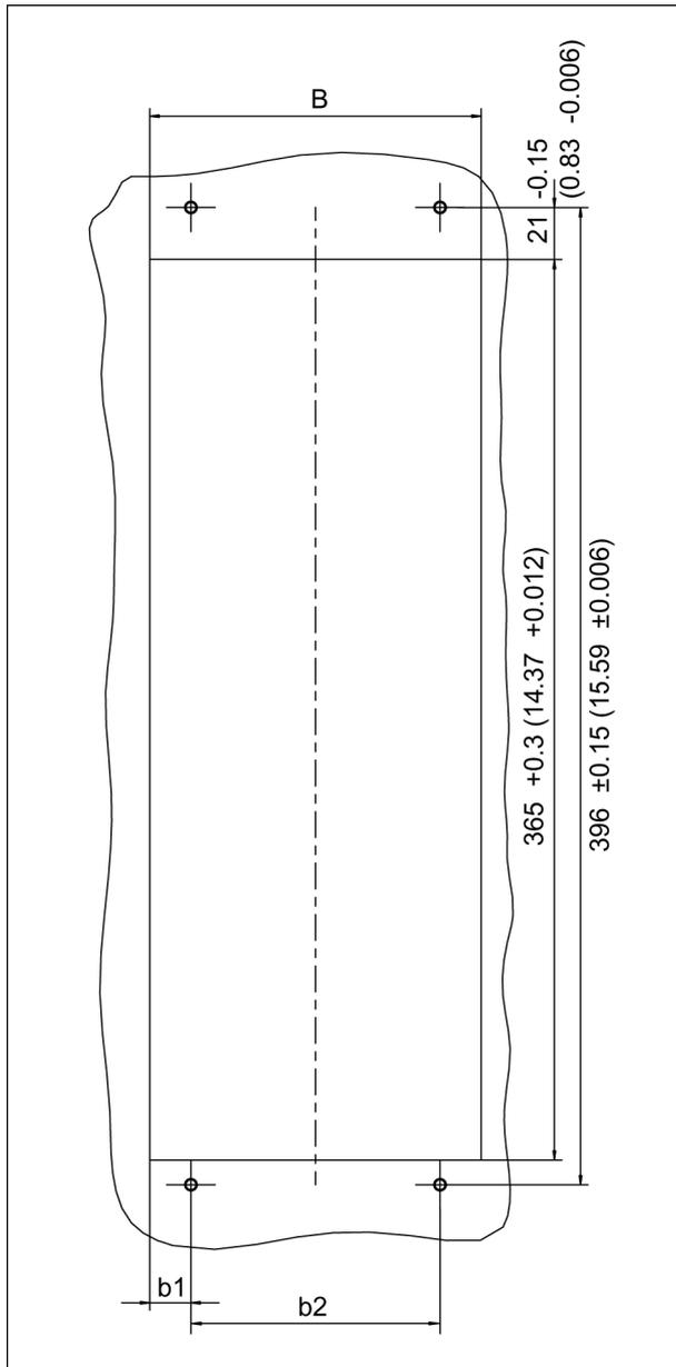
Figure 5-29 Installation openings for the power unit with external air cooling, 50 mm to 200 mm
