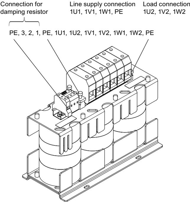
Figure 2-47 HFD line reactor 55 kW
