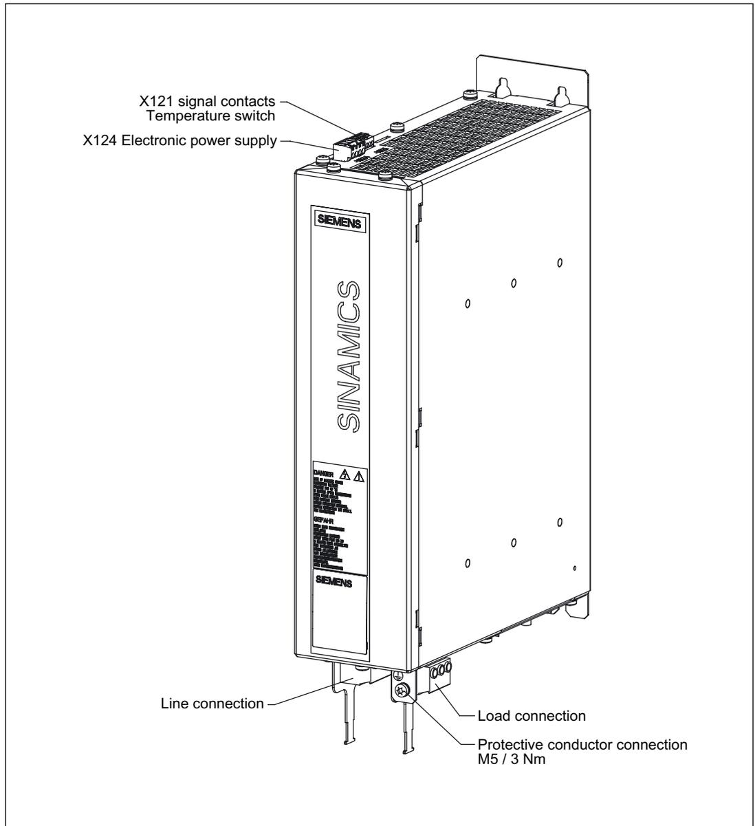
Figure 2-30 Interface description: Active Interface Module 16 kW
