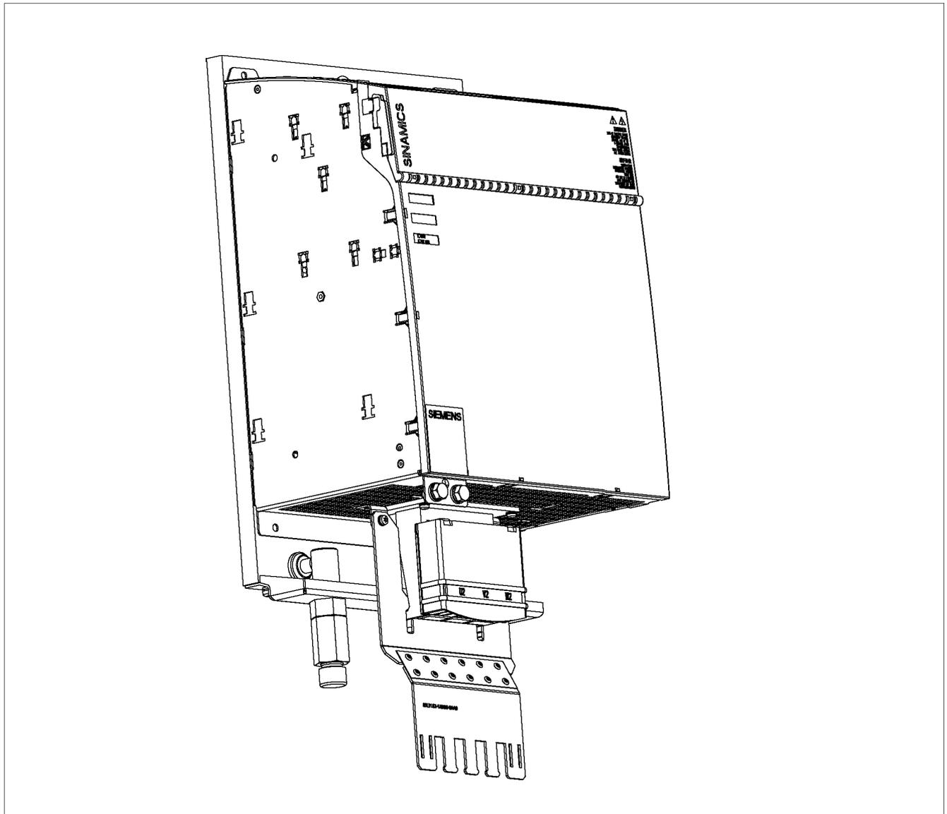
Figure 10-4 Shield connecting plate on a 300 mm Liquid Cooled module
