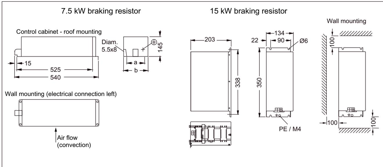
Figure 3-87 Dimension and installation drawing for braking resistor 7.5 kW and 15 kW, all dimensions in mm
