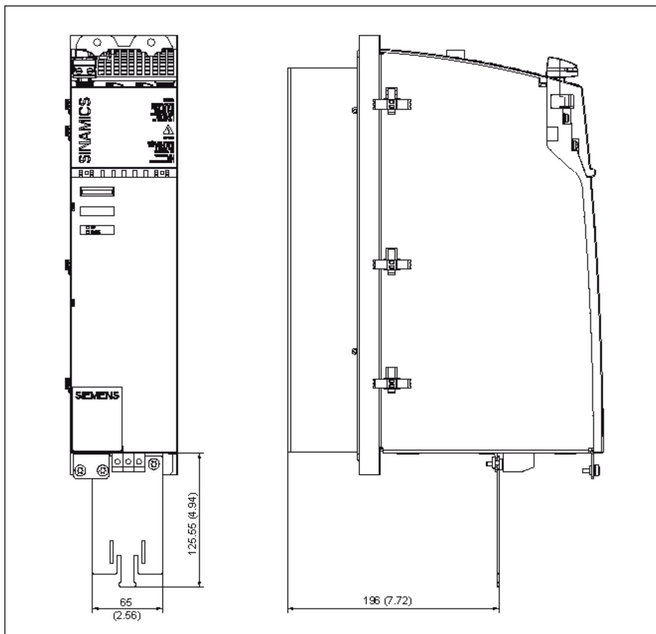
Figure 10-9 Dimension drawing of shield connecting plate on a 100 mm component with external air cooling, all dimensions in mm and (inches)
