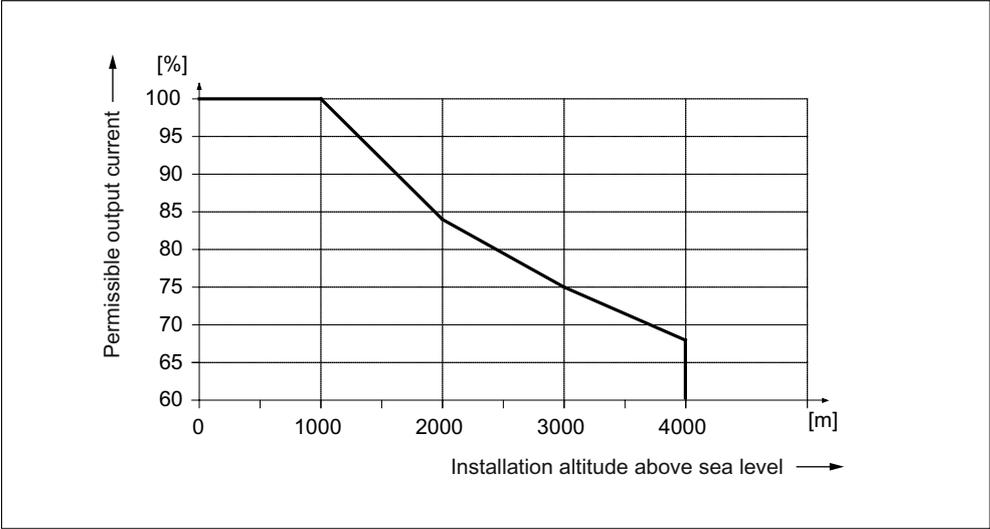
Figure 3-85 Output current as a function of the installation altitude
