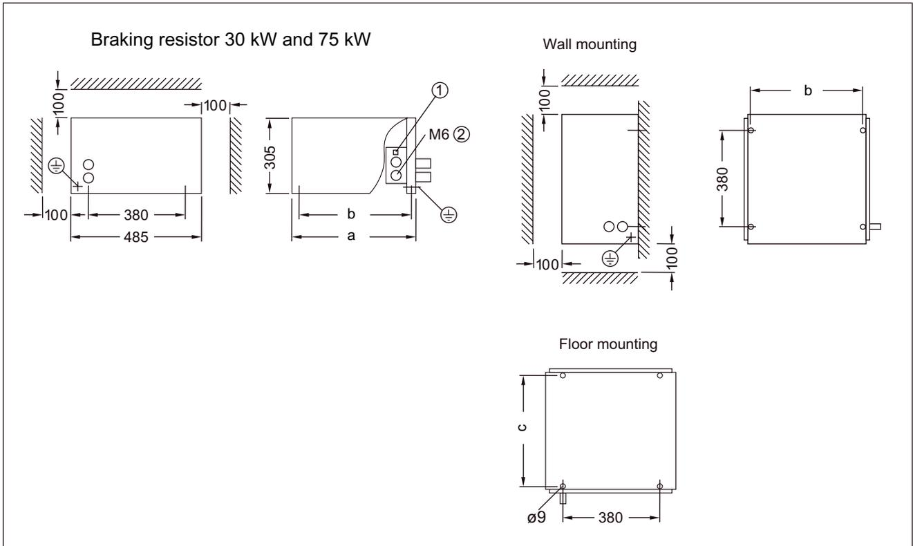
Figure 3-88 Dimension and installation drawing for braking resistor 30 kW and 75 kW, all dimensions in mm
