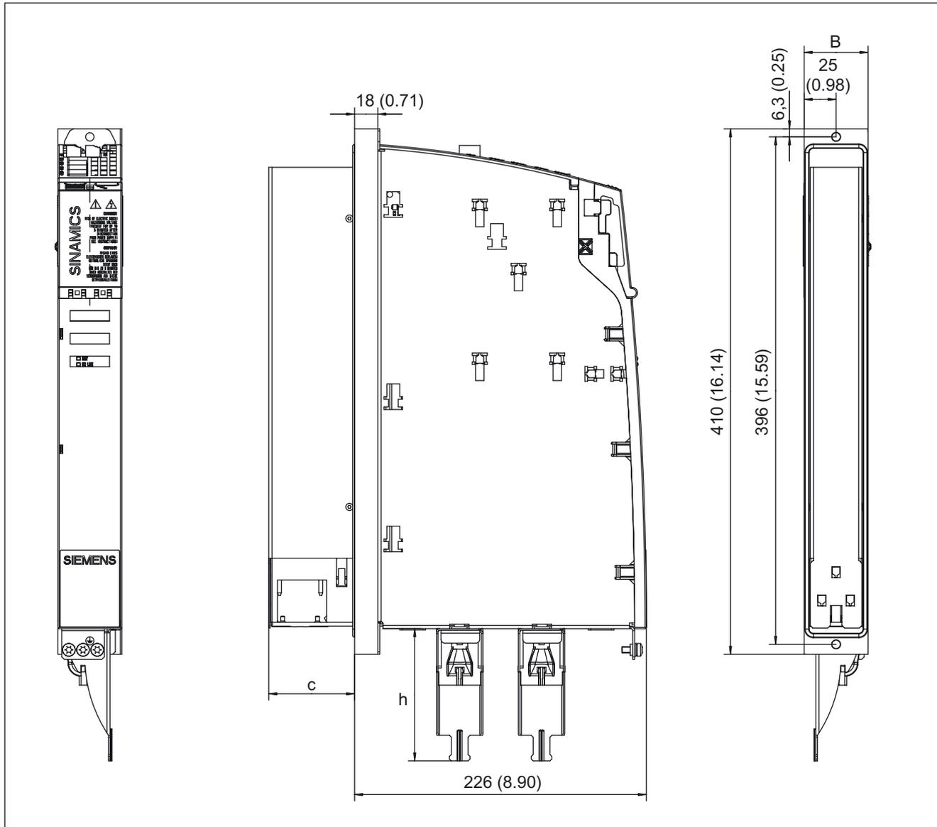
Figure 5-23 Dimension drawing of Motor Modules with external air cooling 3 A to 18 A and 2 x 3 A to 2 x 9 A, all dimensions in mm and (inches)
