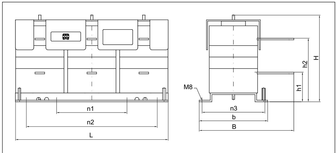
Figure 2-44 Dimension drawing of HF line reactor for Active Line Modules over 80 kW
