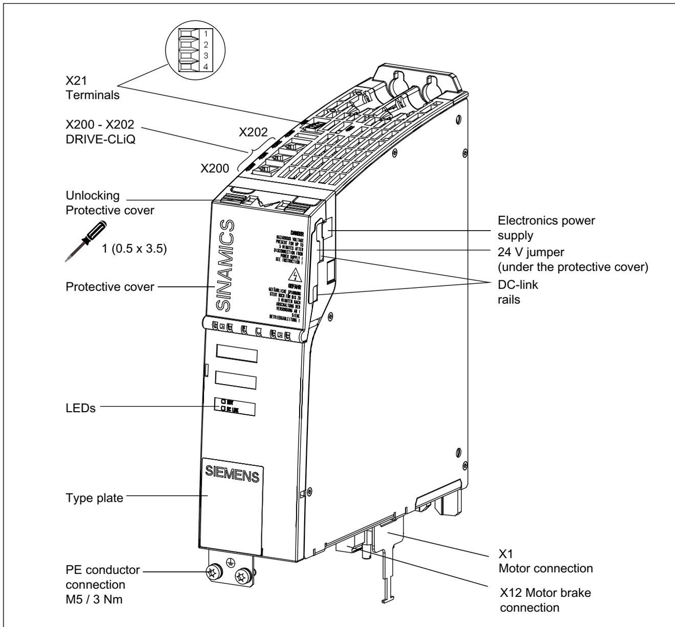
Figure 6-2 Example: Motor Module Booksize Compact format 18 A
