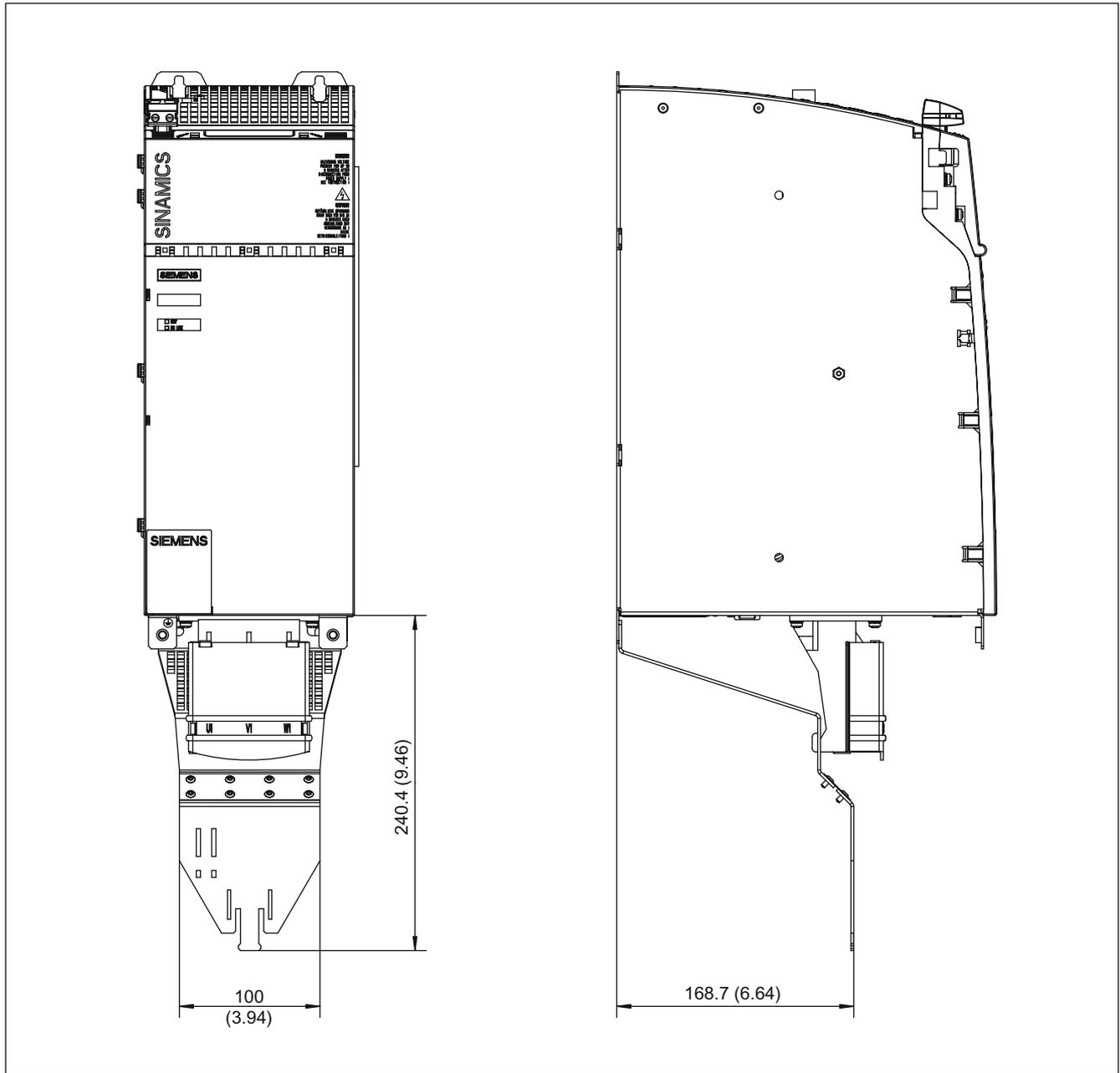
Figure 10-6 Dimension drawing of shield connecting plate on a 150 mm component with internal air cooling, all dimensions in mm and (inches)
