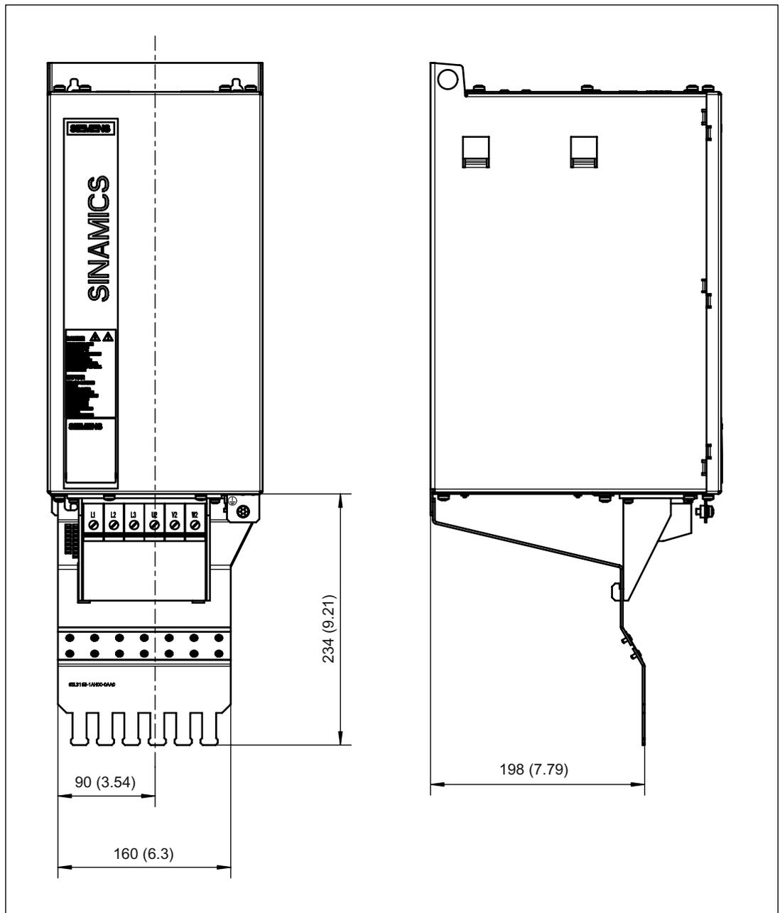
Figure 10-18 Dimension drawing of shield connecting plate on the 55 kW Active Interface Module, all dimensions in mm and (inches)
