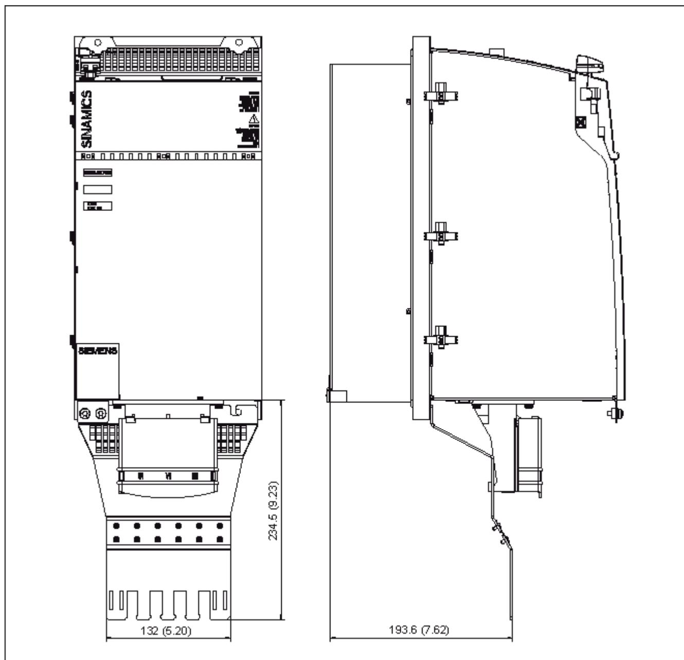
Figure 10-11 Dimension drawing of shield connecting plate on a 200 mm component with external air cooling, all dimensions in mm and (inches)
