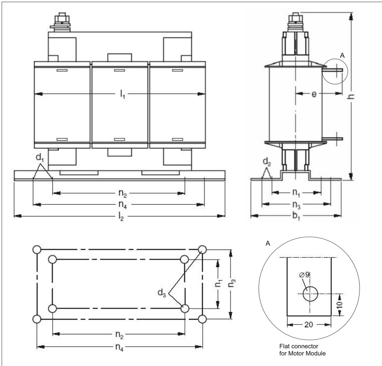
Figure 9-4 Dimension drawing and mounting hole of motor reactor 60 A (6SL3000-2BE26-0AA0)
