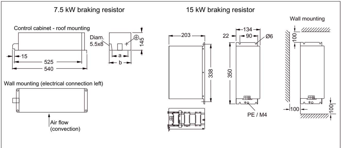
Figure 3-65 Dimension and installation drawing for braking resistor 7.5 kW and 15 kW, all dimensions in mm
