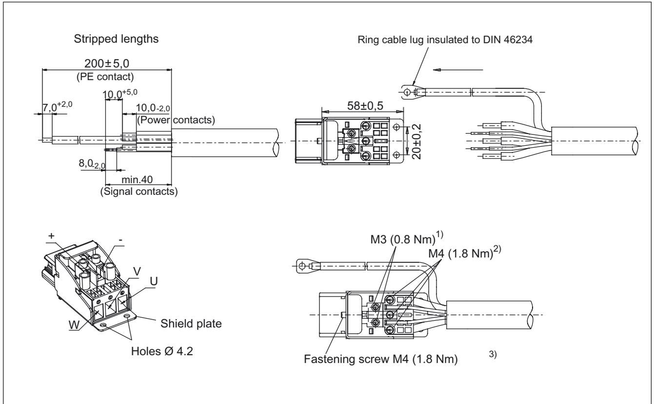
Figure 11-25 Design and installation of the power connector (X1/X2)
