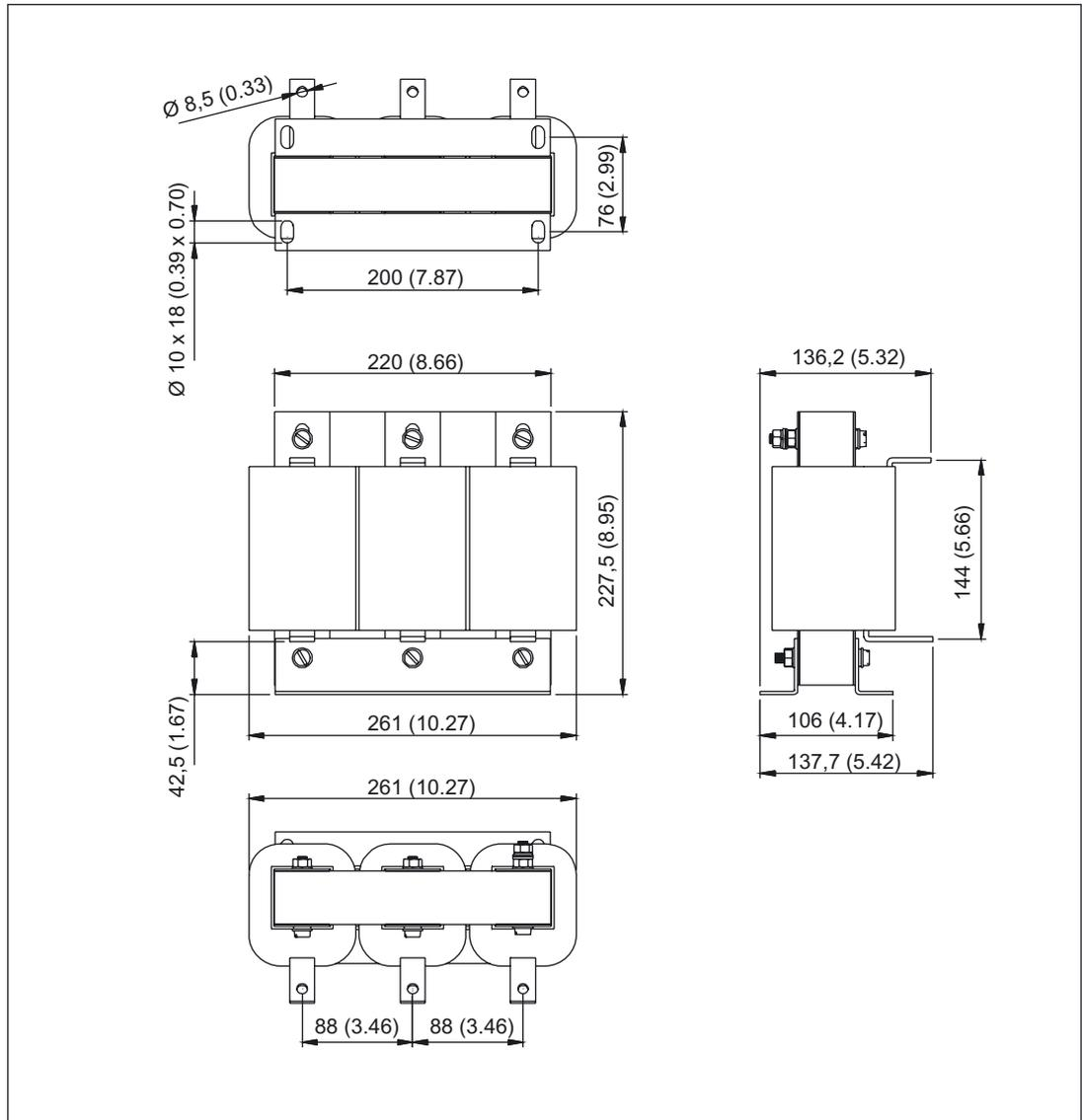
Figure 2-68 Dimension drawing of line reactor for Basic Line Module 100 kW, all dimensions in mm and (inches)
