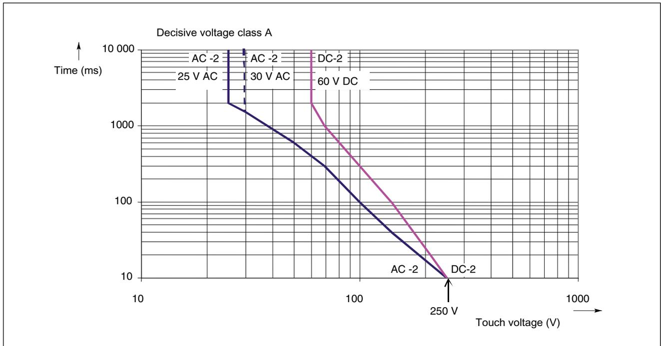
Figure 11-1 Permissible tripping time of fuses
