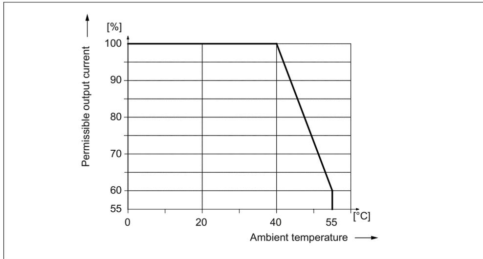
Figure 3-46 Output current as a function of the ambient temperature
