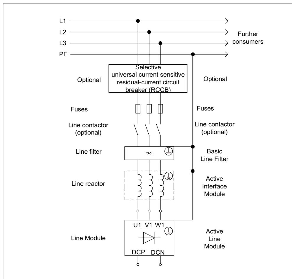
Figure 11-2 Connecting a residual-current operated circuit breaker
