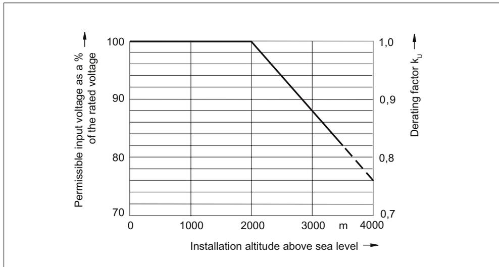
Figure 5-44 Voltage derating as a function of the installation altitude
