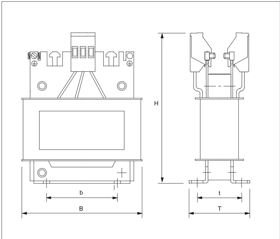
Figure 2-60 Dimension drawing: line reactor for Smart Line Modules (5 and 10 kW)
