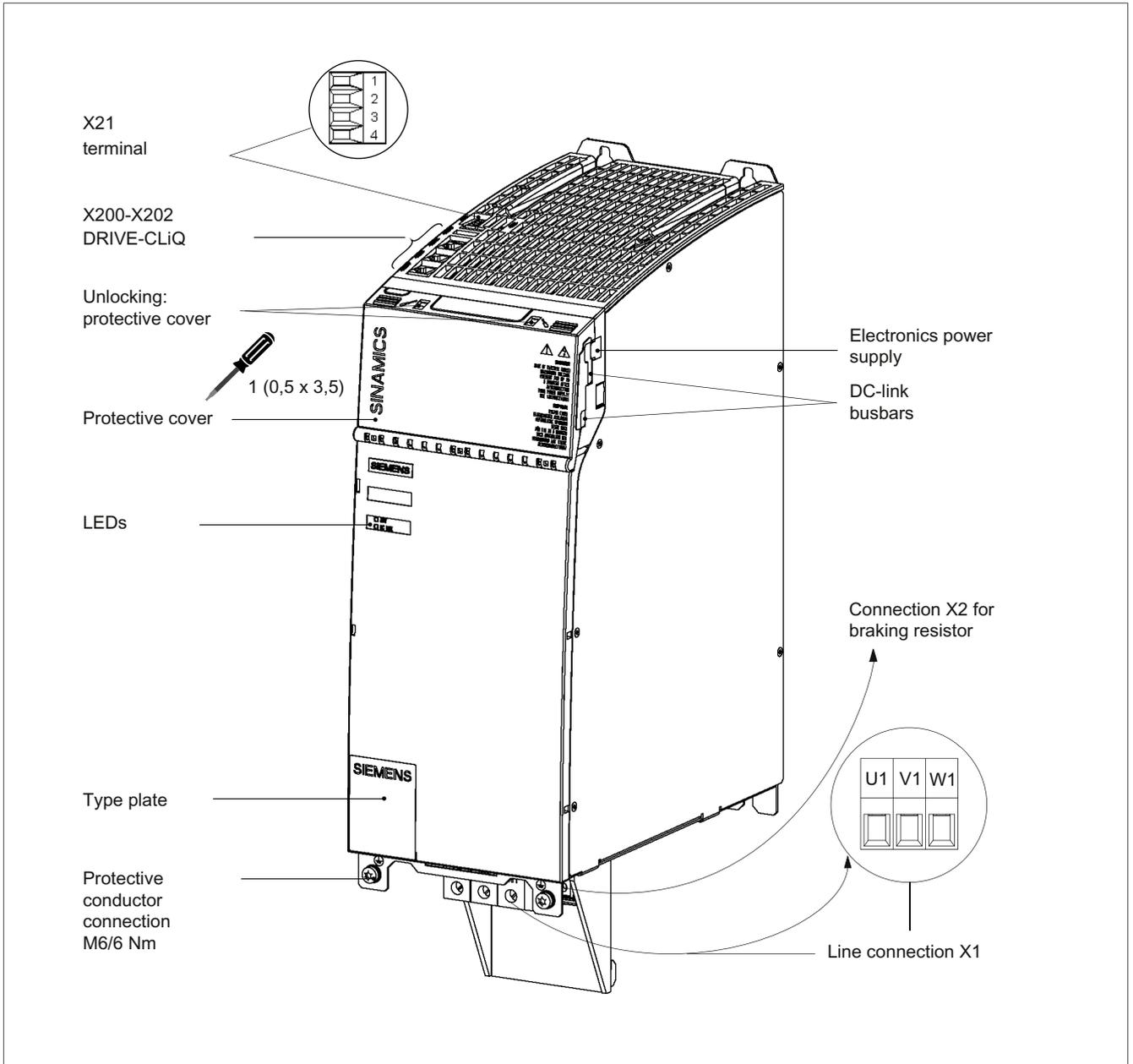
Figure 3-51 Basic Line Module with internal air cooling (40 kW)
