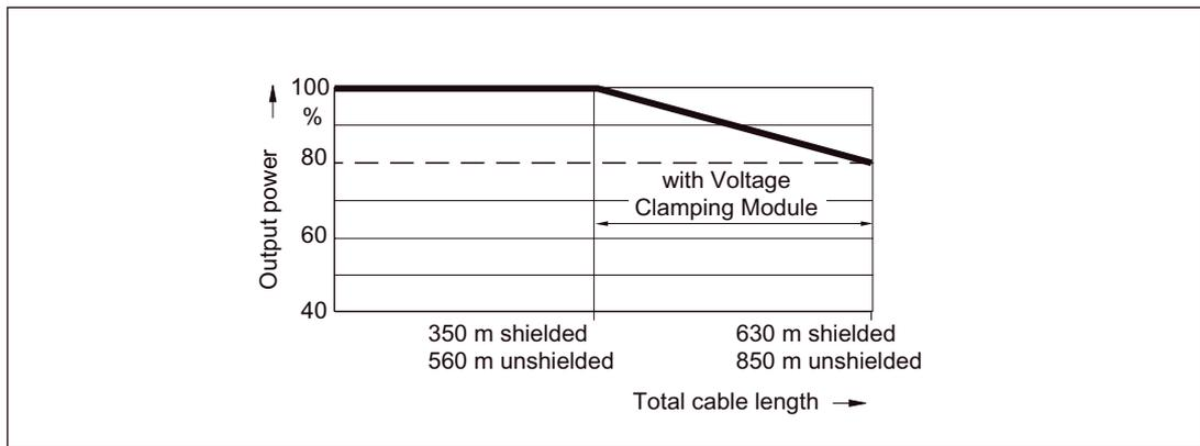
Figure 8-17 Output power as a function of the total cable length
