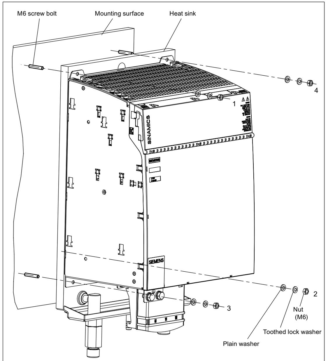
Figure 3-44 Installation of liquid-cooled power unit
