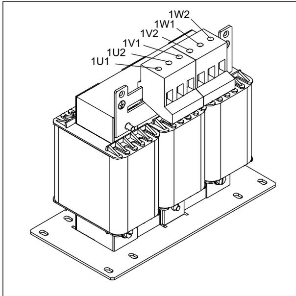
Figure 2-63 Line reactor for Basic Line Module (20 kW)
