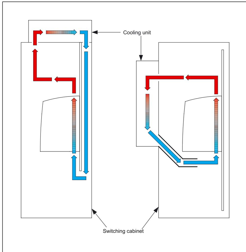
Figure 11-37 Examples of cabinet ventilation
