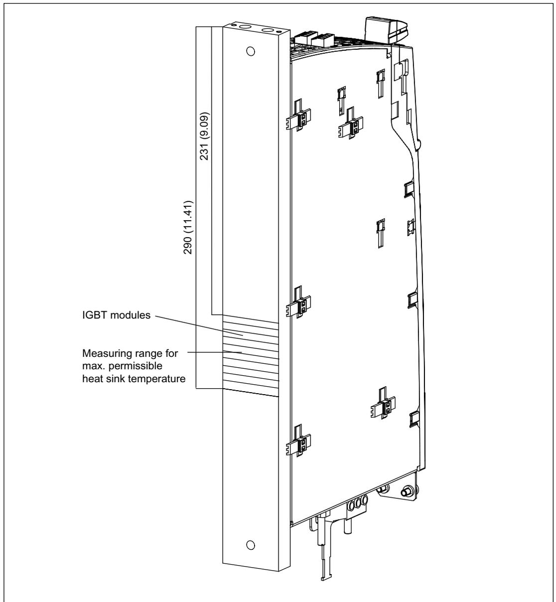
Figure 3-122 Measuring range for max. permissible heat-sink temperature for a Smart Line Module
