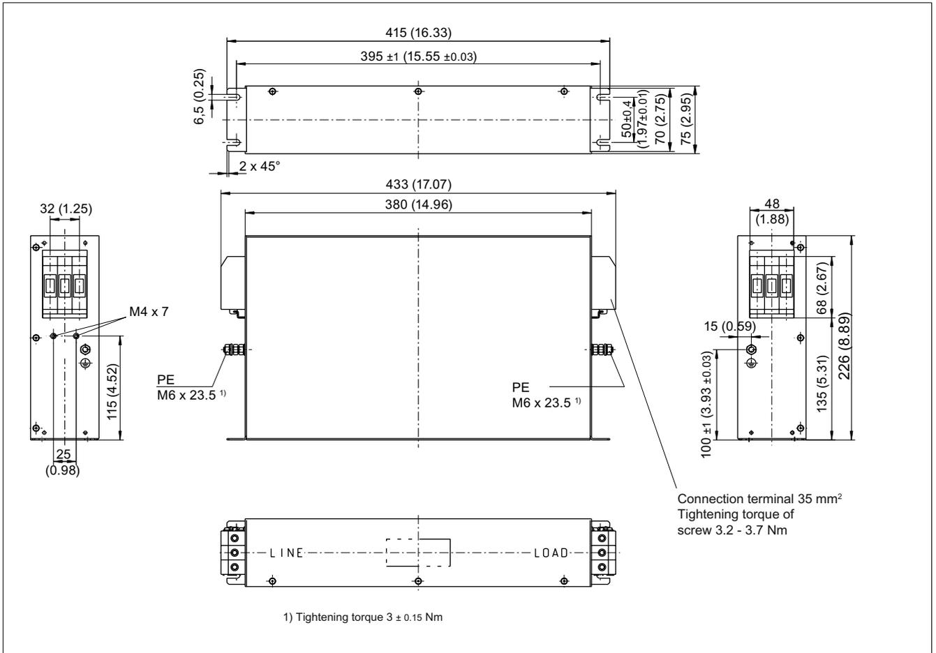
Figure 2-29 Dimension drawing of Basic Line Filter for Smart Line Modules 36 kW, order number 6SL3000-0BE23-6DA1, all dimensions in mm and (inches)
