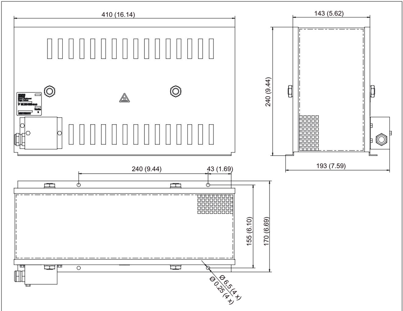
Figure 8-6 Dimension drawing of braking resistor 1.5 kW/100 kW, all dimensions in mm and (inches)
