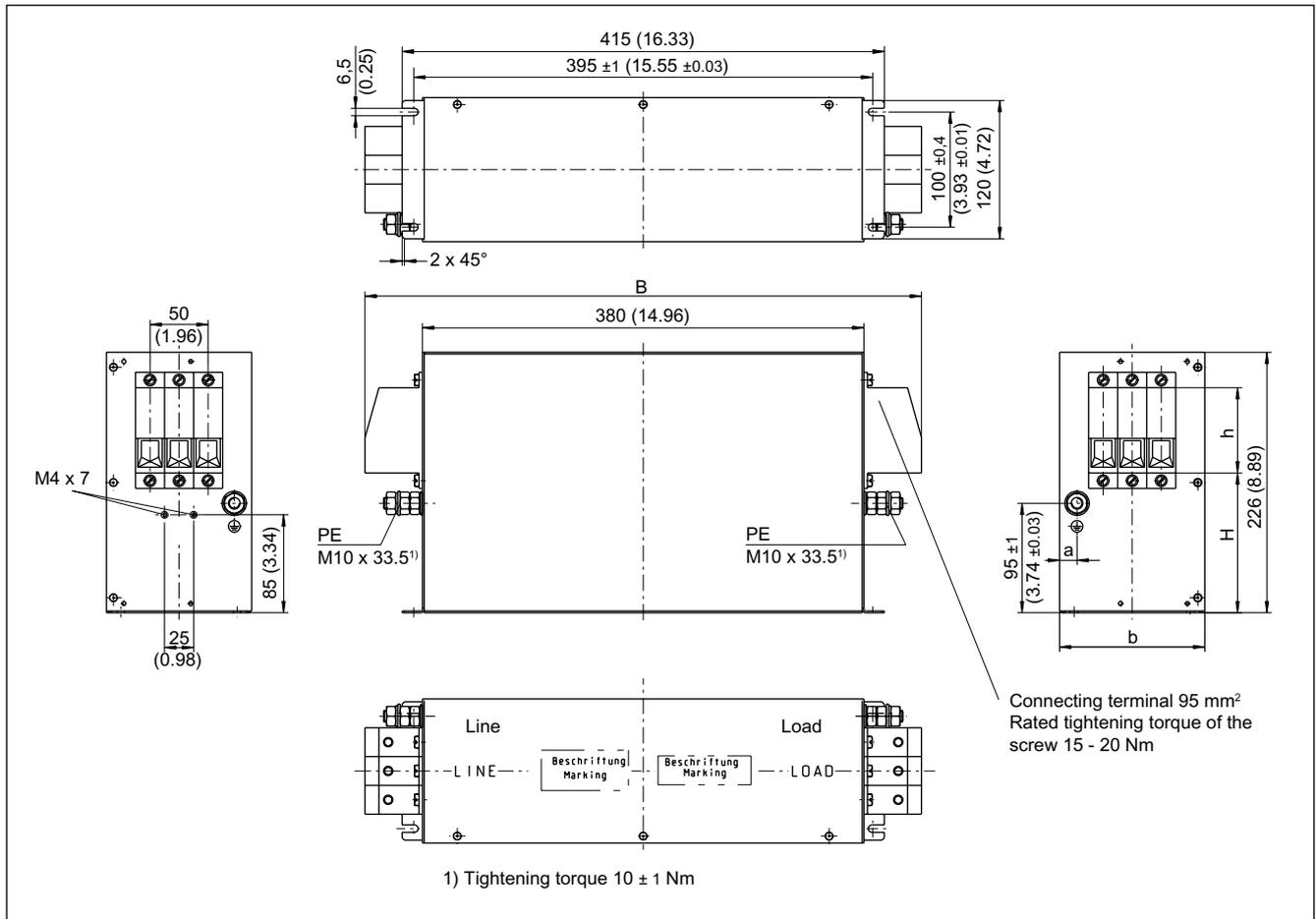
Figure 2-15 Dimension drawing of Basic Line Filter 80 kW and 120 kW, all dimensions in mm and (inches)
