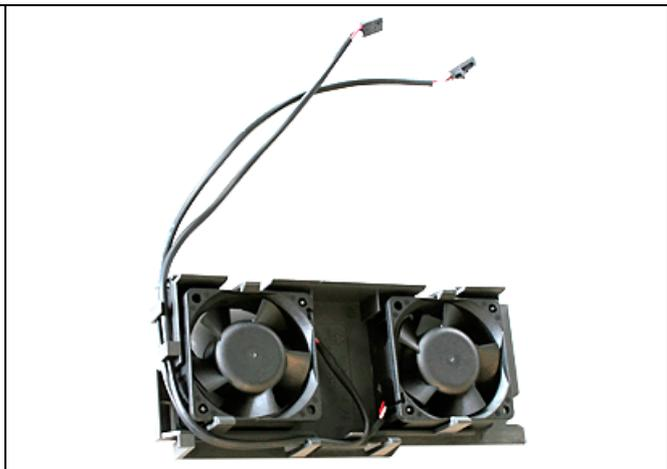
Observe the air flow direction markings when inserting the new fan
