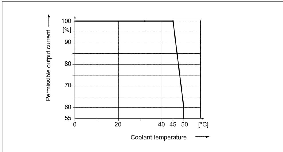
Figure 3-47 Output current as a function of the coolant temperature
