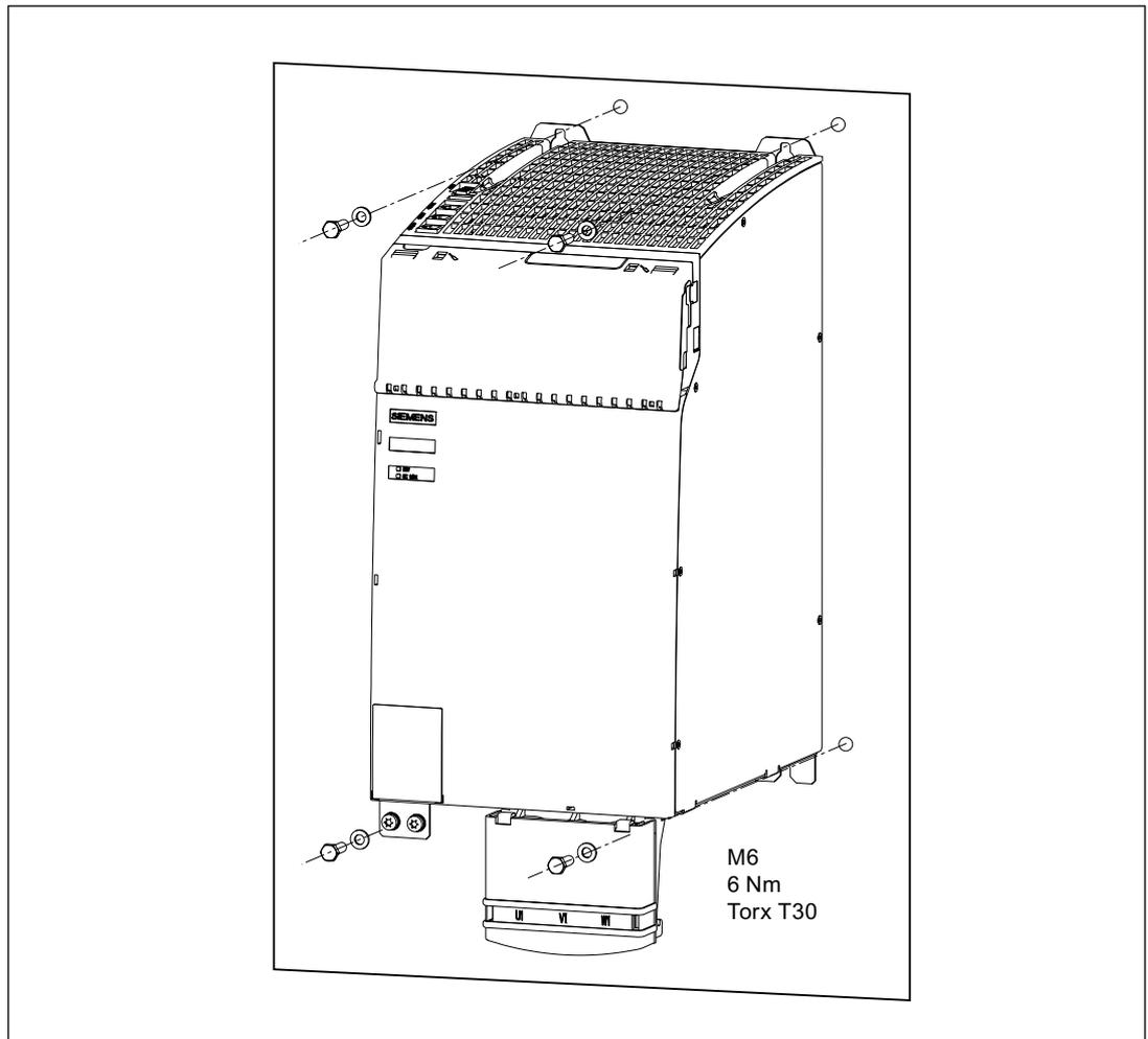
Figure 3-58 Installation: Basic Line Module 100 kW
