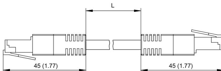
Figure 11-15 DRIVE-CLiQ signal cable without 24 V DC conductors
