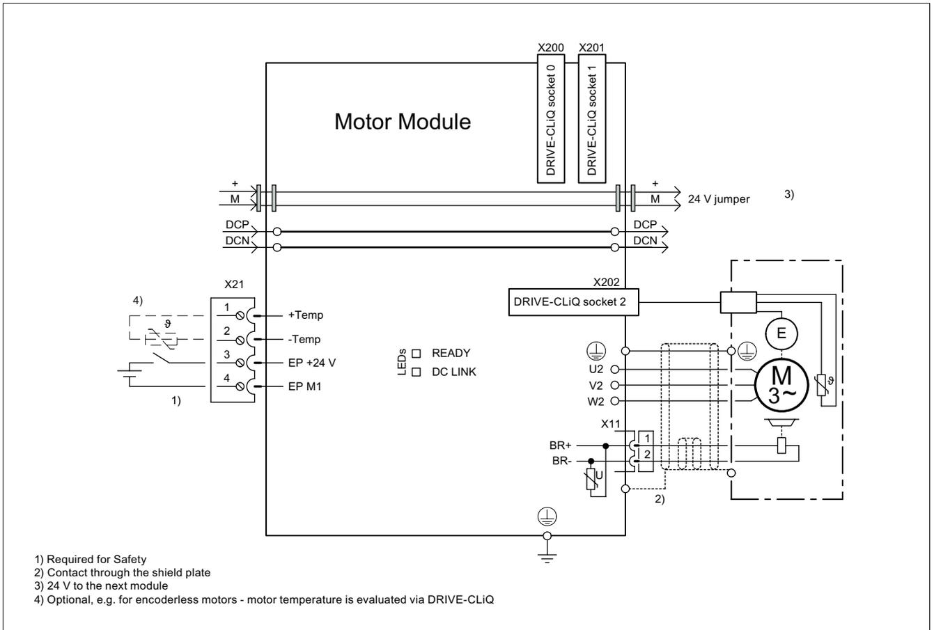
Figure 5-65 Connection example for Motor Module Liquid Cooled (200 A)
