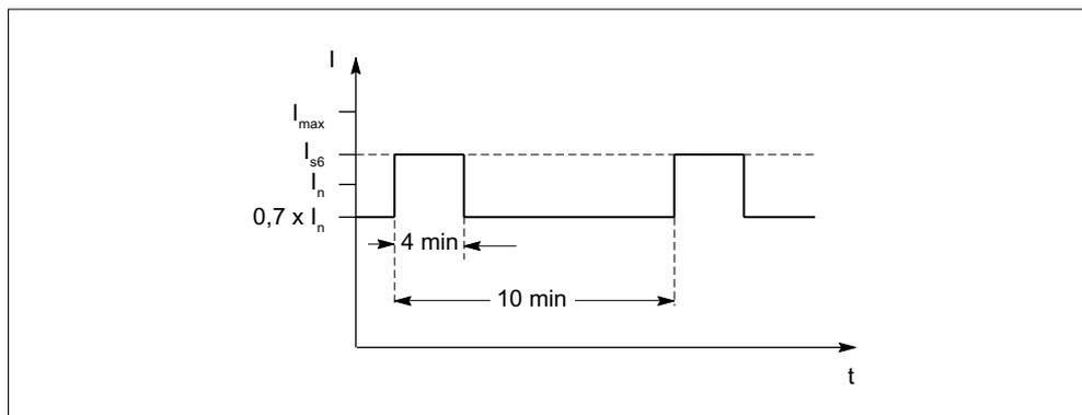
Figure 6-12 S6 duty cycle with initial load with a duty cycle duration of 600 s
