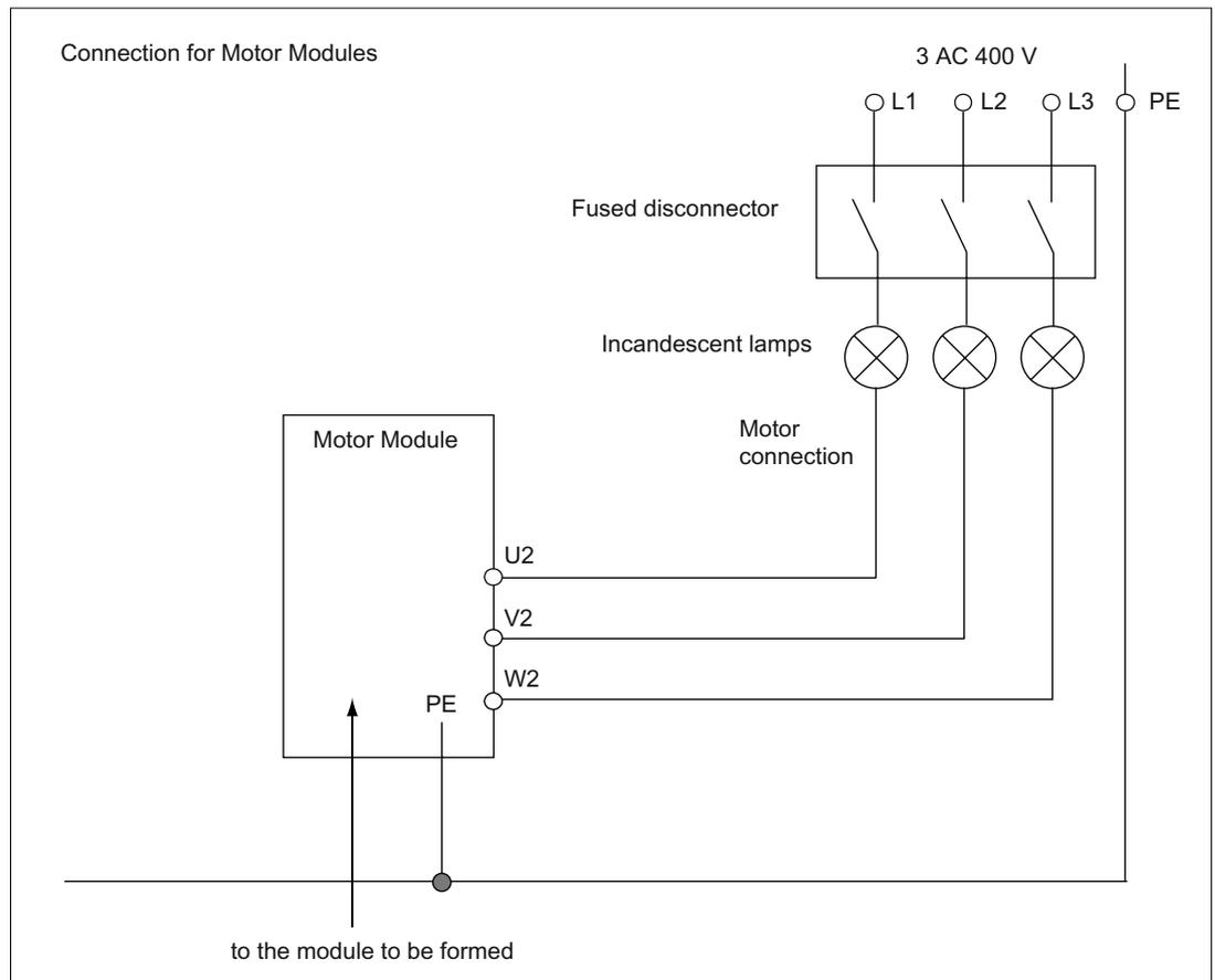
Figure 13-3 Forming circuit for Motor Modules with incandescent lamps
