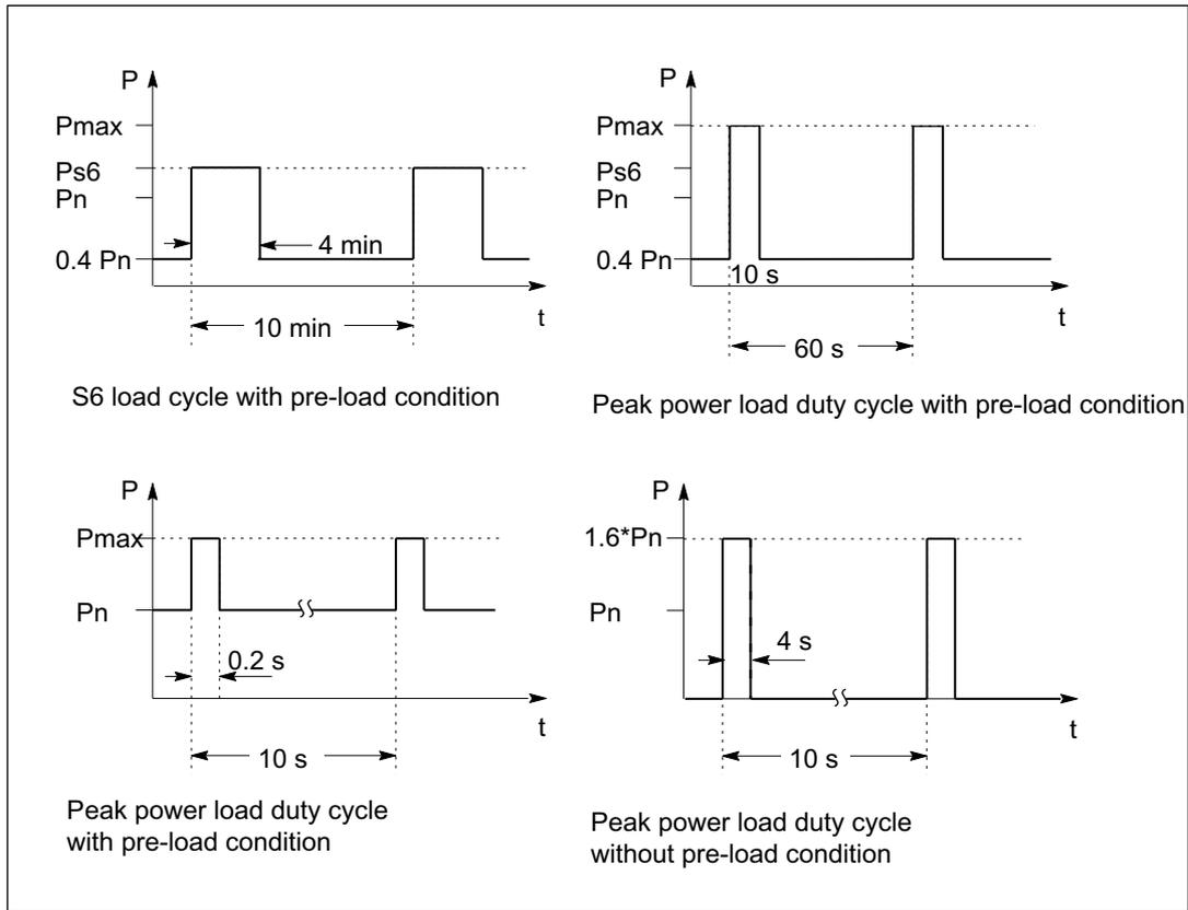
Figure 3-45 Rated duty cycles of Active Line Modules
