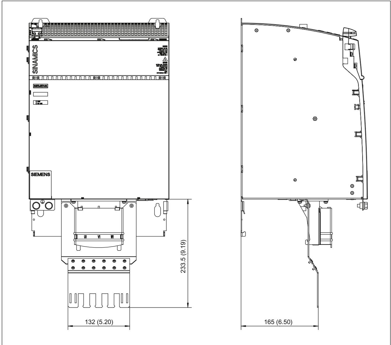
Figure 10-8 Dimension drawing of shield connecting plate on a 300 mm component with internal air cooling, all dimensions in mm and (inches)
