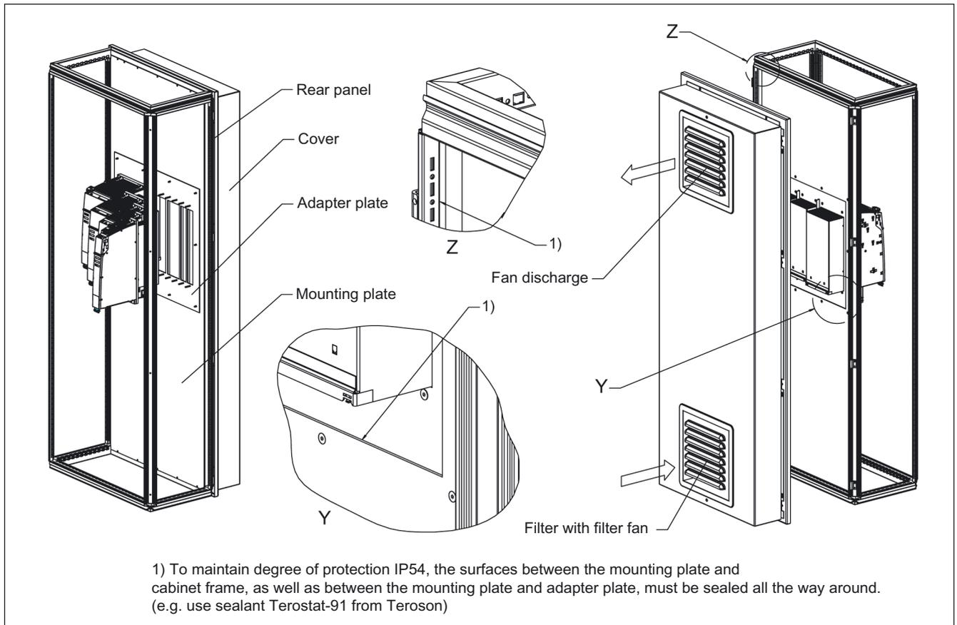
Figure 3-109 Example 2: installation in cabinet with mounting plate
