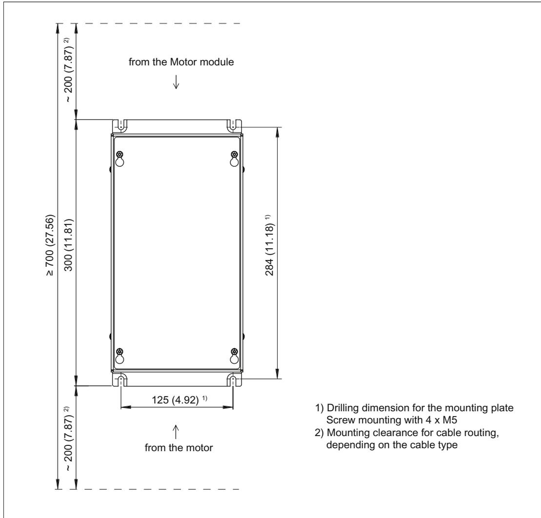
Figure 9-13 Mounting dimension for a Voltage Protection Module VPM120
