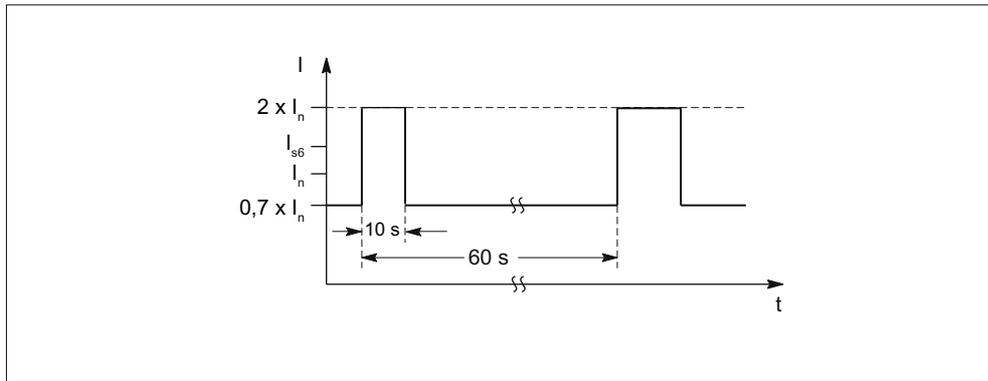
Figure 6-13 S6 duty cycle with initial load with a duty cycle duration of 60 s
