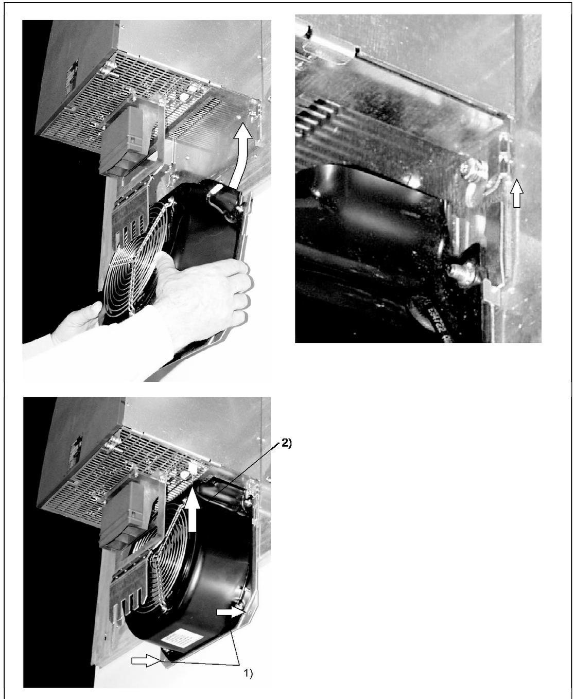
Figure 5-8 Installing the fan for 300 mm modules
