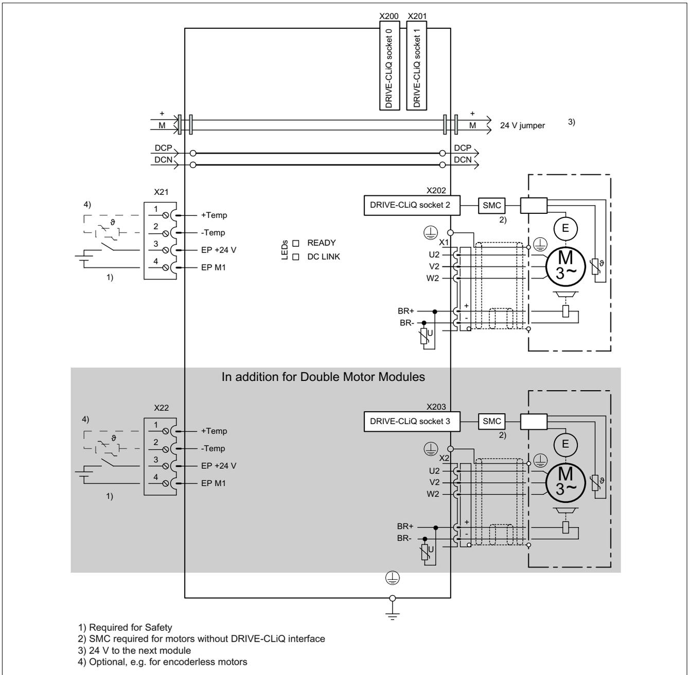
Figure 5-2 Connection example of Motor Modules 3 A to 30 A and Double Motor Modules 3 A to 18 A
