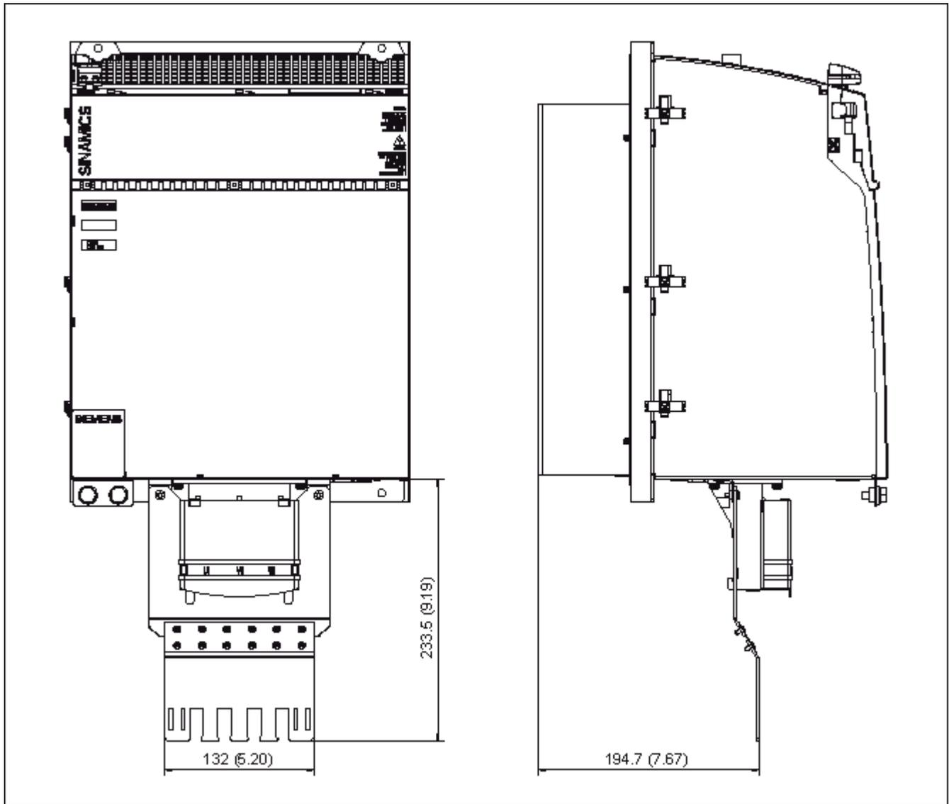
Figure 10-12 Dimension drawing of shield connecting plate on a 300 mm component with external air cooling, all dimensions in mm and (inches)
