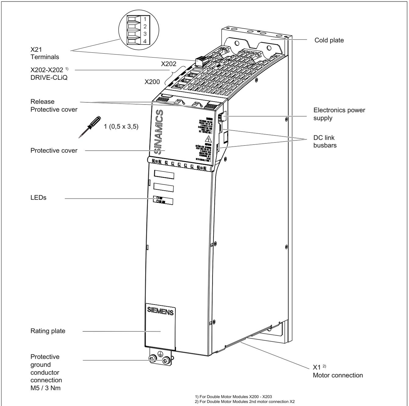
Figure 5-45 Single motor module with cold plate (example 30 A)
