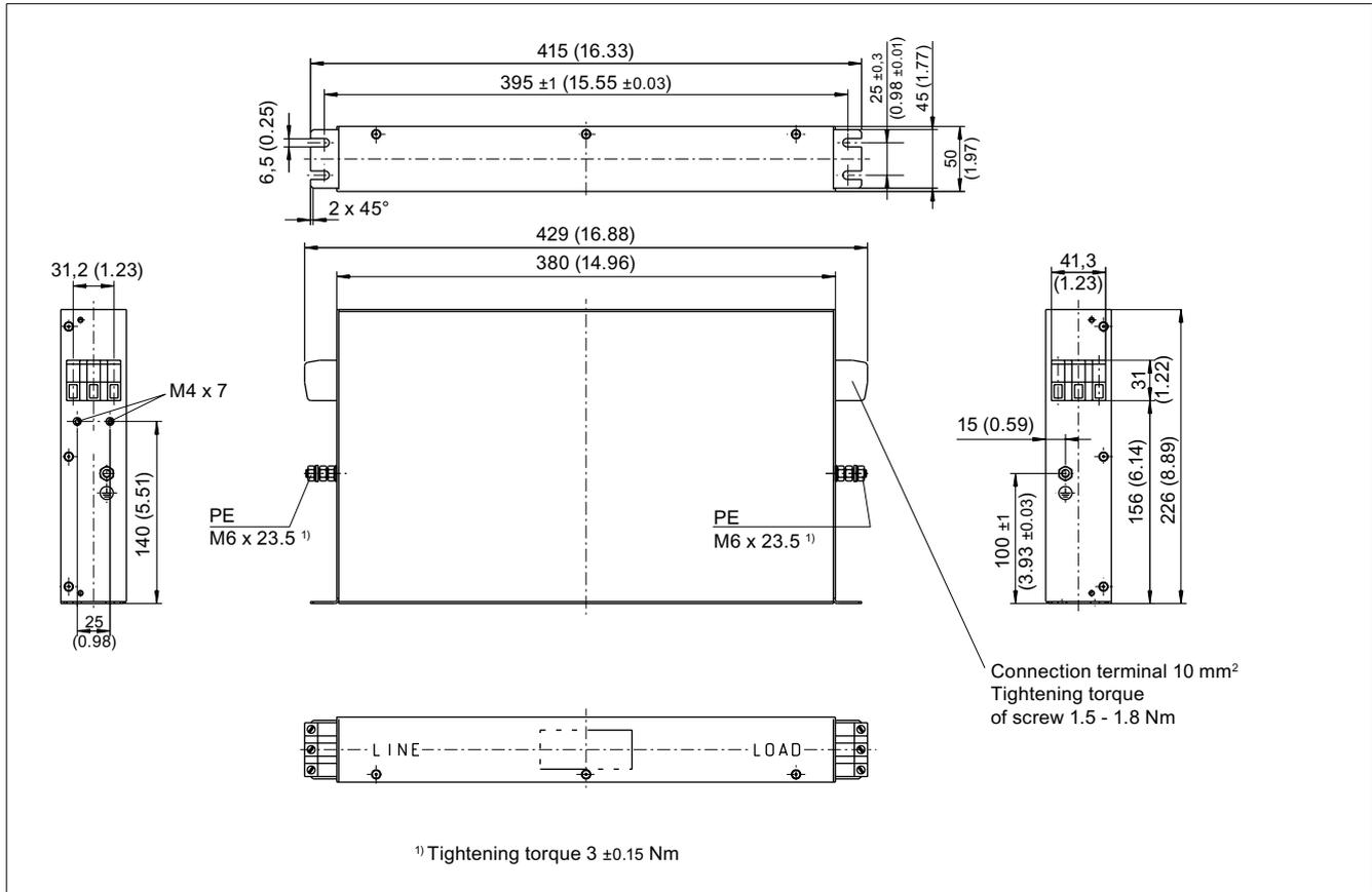
Figure 2-23 Dimension drawing of Basic Line Filter for Basic Line Modules 20 kW, order number 6SL3000-0BE21-6DAX, all dimensions in mm and (inches)
