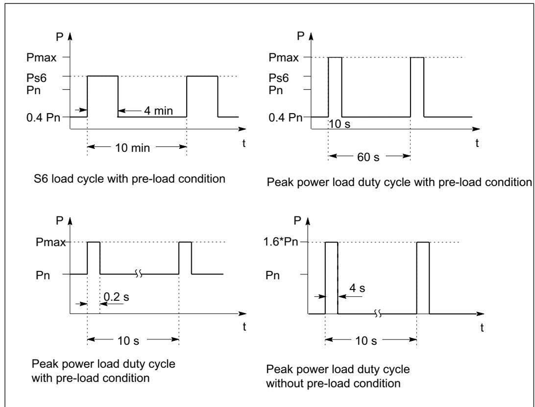
Figure 3-8 Rated duty cycles of Active Line Modules (**exception:** not applicable for 55 kW Active Line Module with Active Interface Module)
