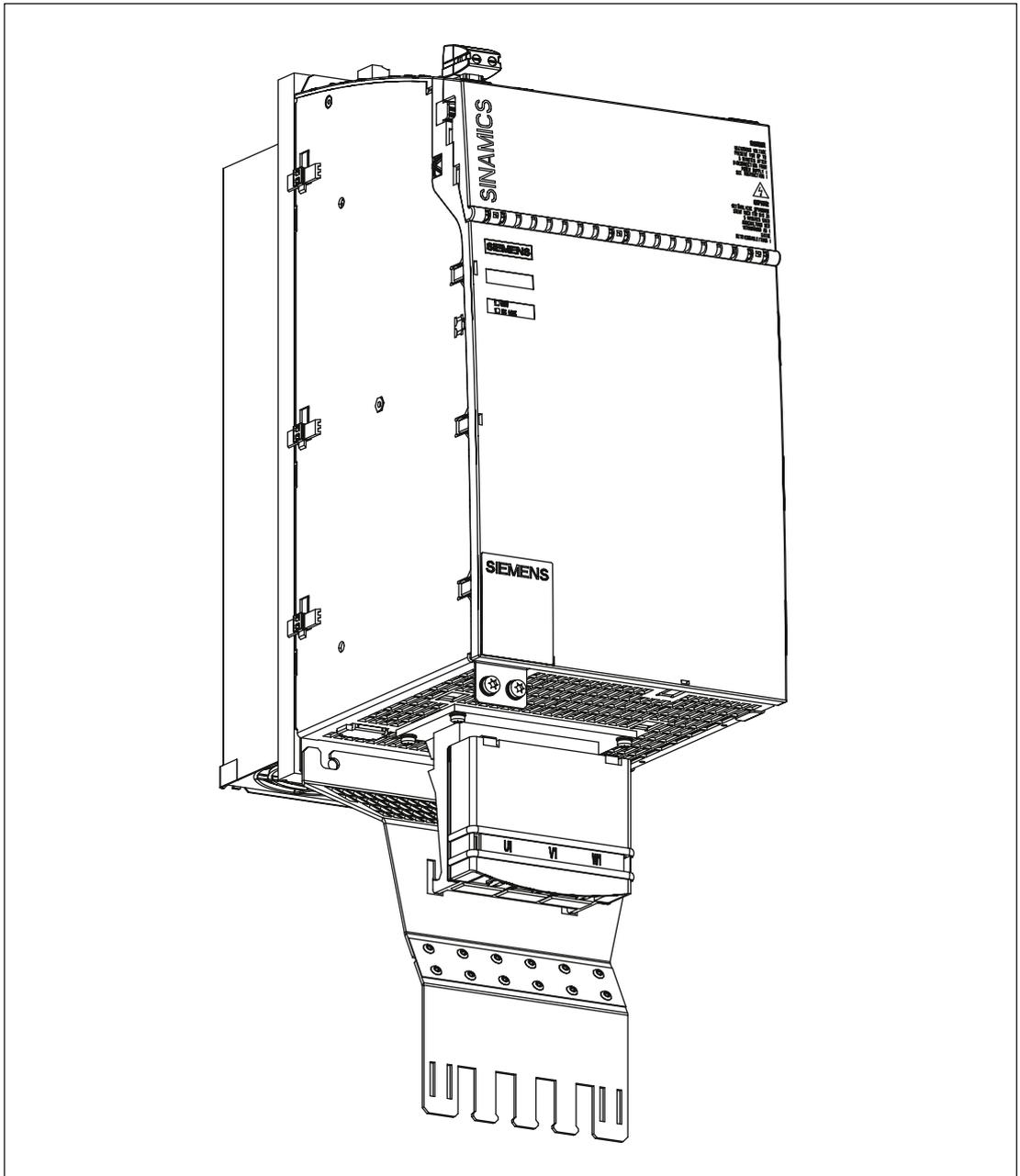
Figure 10-2 Shield connecting plate for a 200 mm module with external air cooling
