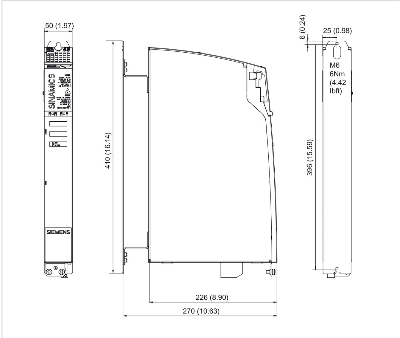
Figure 8-16 Dimension drawing of Voltage Clamping Module, all dimensions in mm and (inches)
