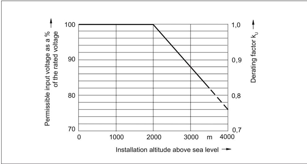
Figure 3-101 Voltage derating as a function of the installation altitude
