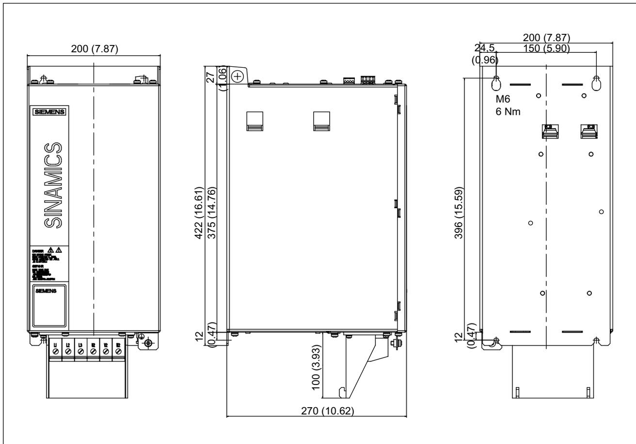
Figure 2-37 Dimension drawing of Active Interface Module 55 kW, all dimensions in mm and (inches)
