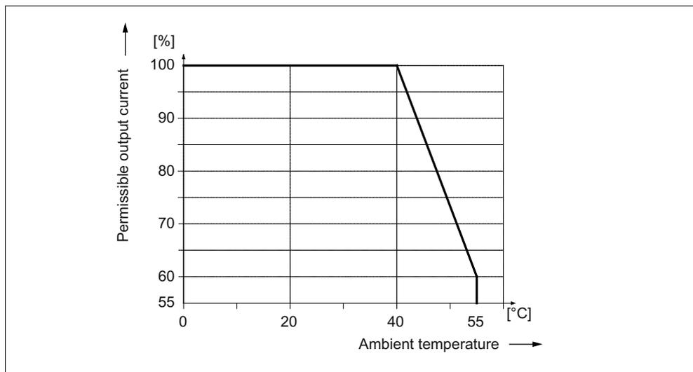
Figure 6-17 Output current as a function of the ambient temperature
