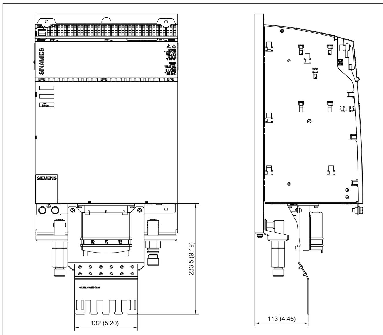
Figure 10-16 Dimension drawing of shield connecting plate on a 300 mm Liquid Cooled component, all dimensions in mm and (inches)
