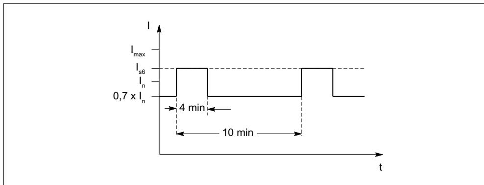
Figure 5-36 S6 duty cycle with initial load with a duty cycle duration of 600 s (for servo drives)
