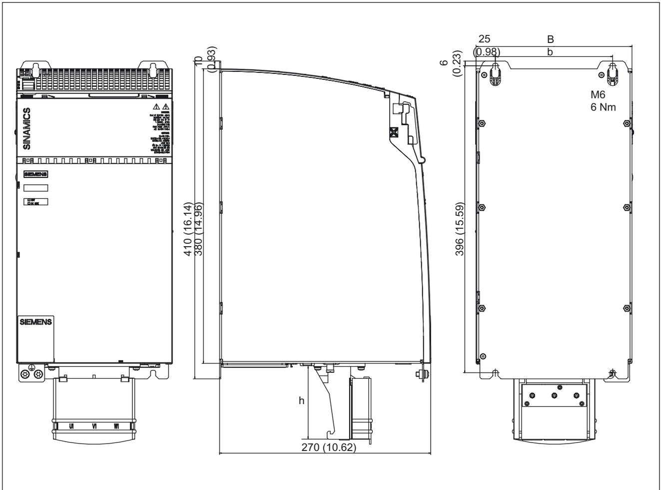
Figure 3-4 Dimension drawing of Active Line Module 36 kW and 55 kW with internal air cooling, all data in mm and (inches)
