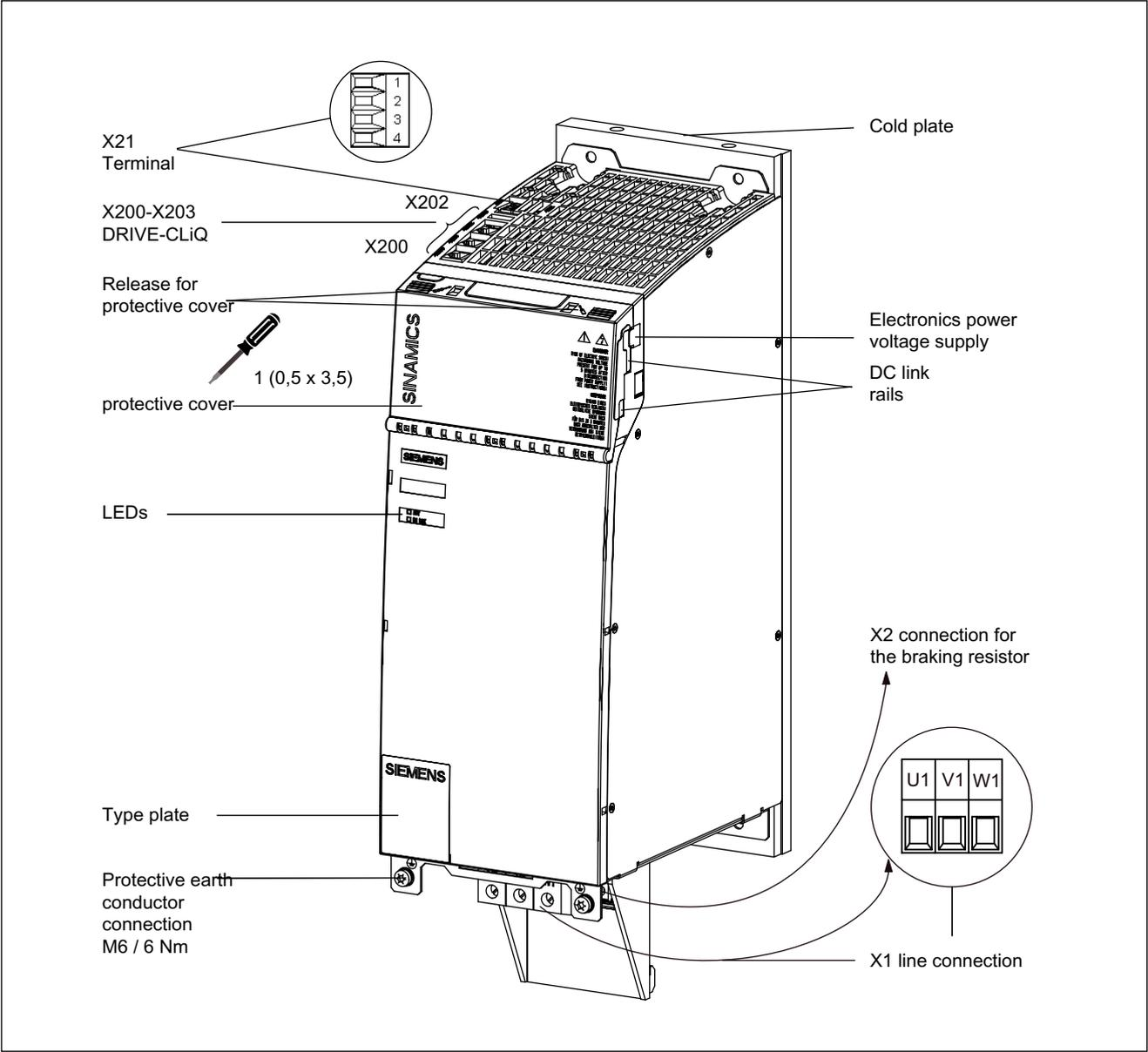
Figure 3-72 Basic Line Module with cold plate (40 kW)
