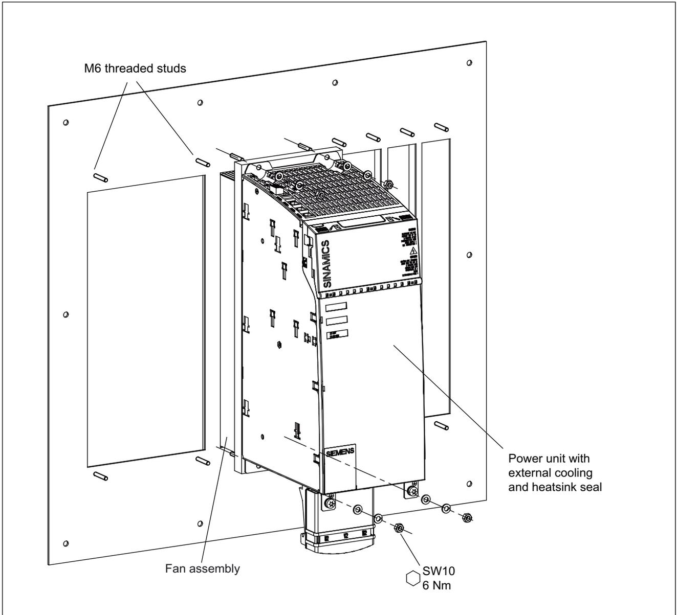
Figure 5-28 Example: Installation of the power unit with external air cooling
