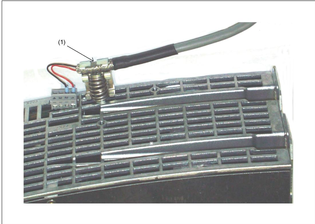
Figure 7-3 Shield connection terminals for shield support
