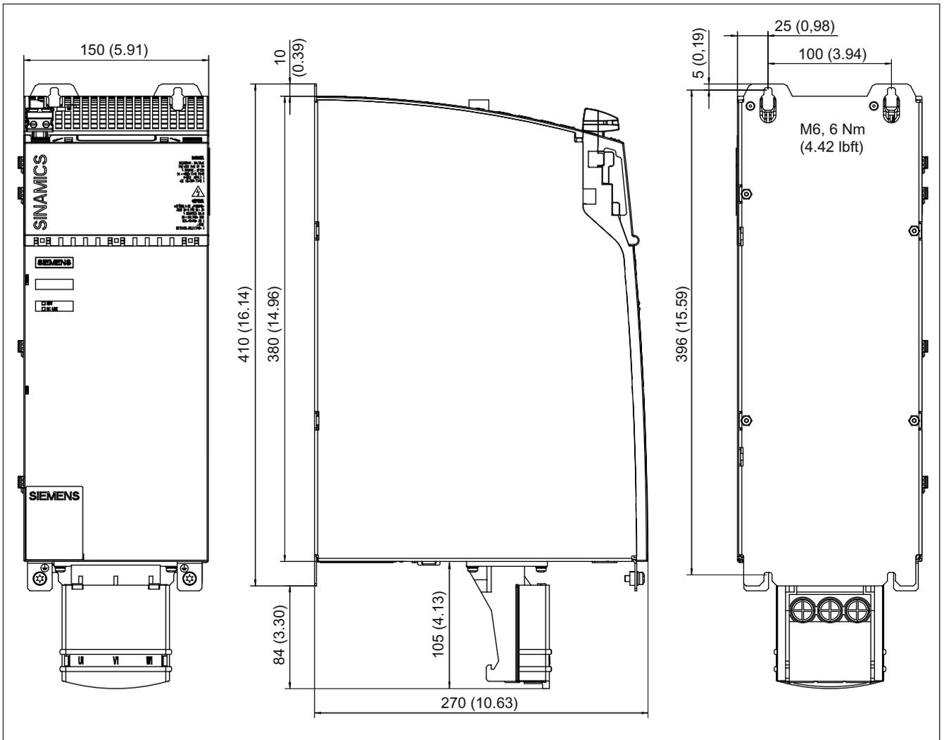
Figure 3-97 Dimension drawing of Smart Line Module with internal air cooling (36 kW), all dimensions in mm and (inches)
