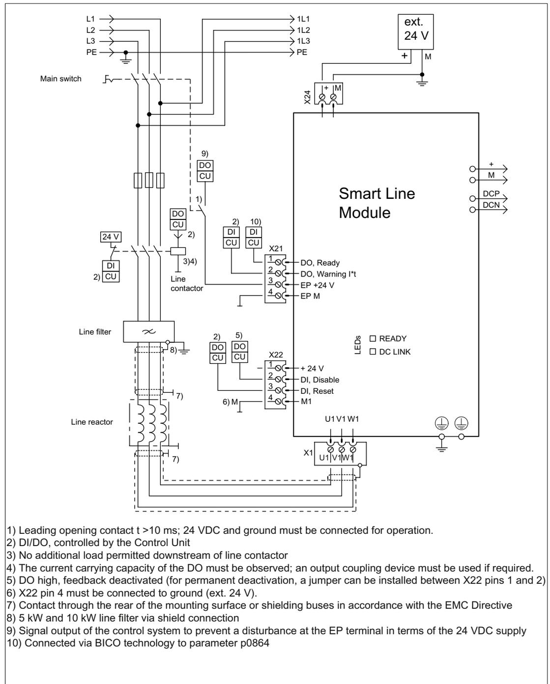
Figure 3-93 Connection example for 5 kW and 10 kW Smart Line Modules
