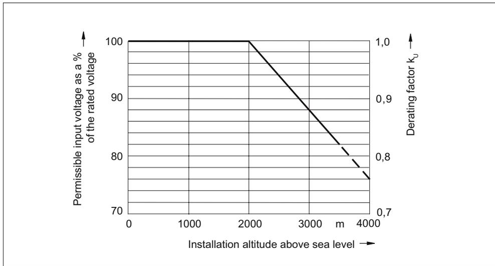
Figure 3-13 Voltage derating as a function of the installation altitude
