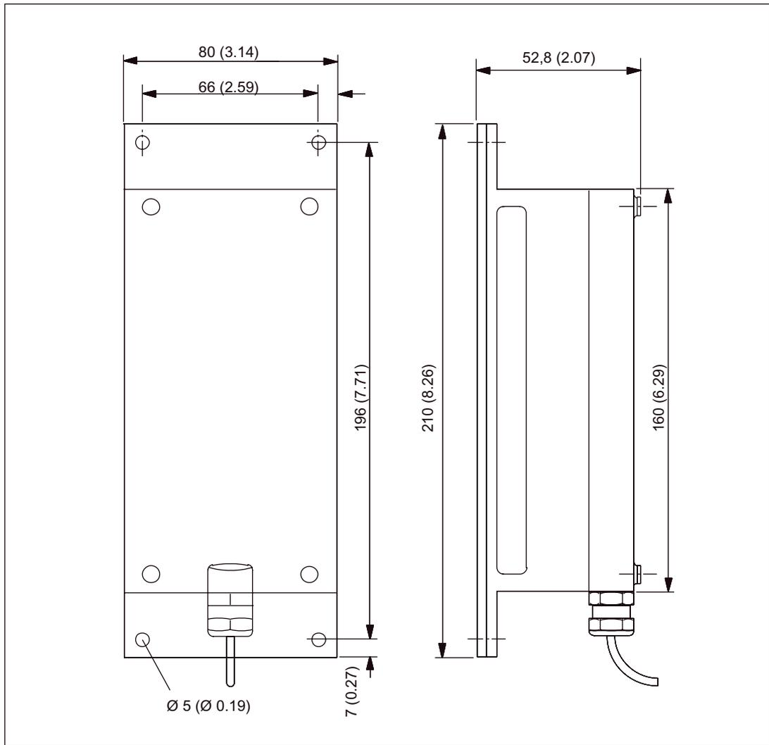
Figure 8-5 Dimension drawing of braking resistor 0.3 kW/25 kW, all dimensions in mm and (inches)
