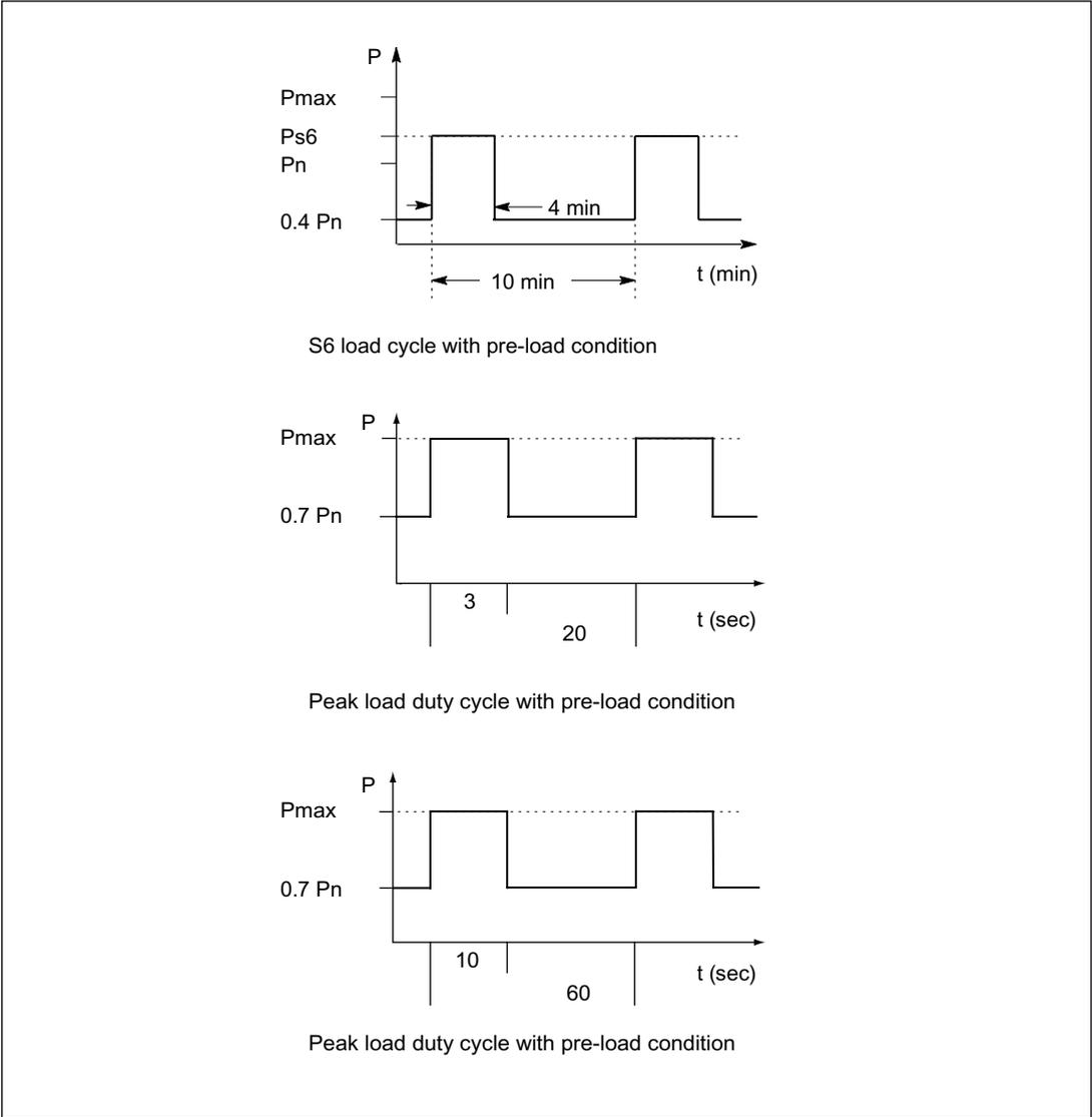
Figure 3-82 Rated duty cycles of 100 kW Basic Line Module
