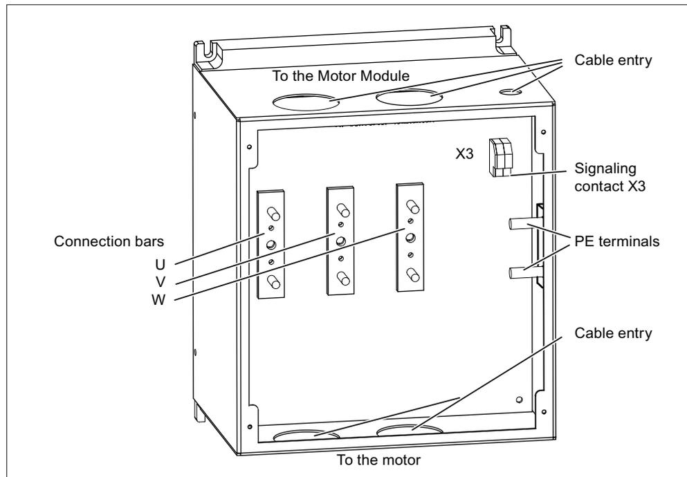
Figure 9-6 Voltage Protection Modules VPM 200 (without cover)
