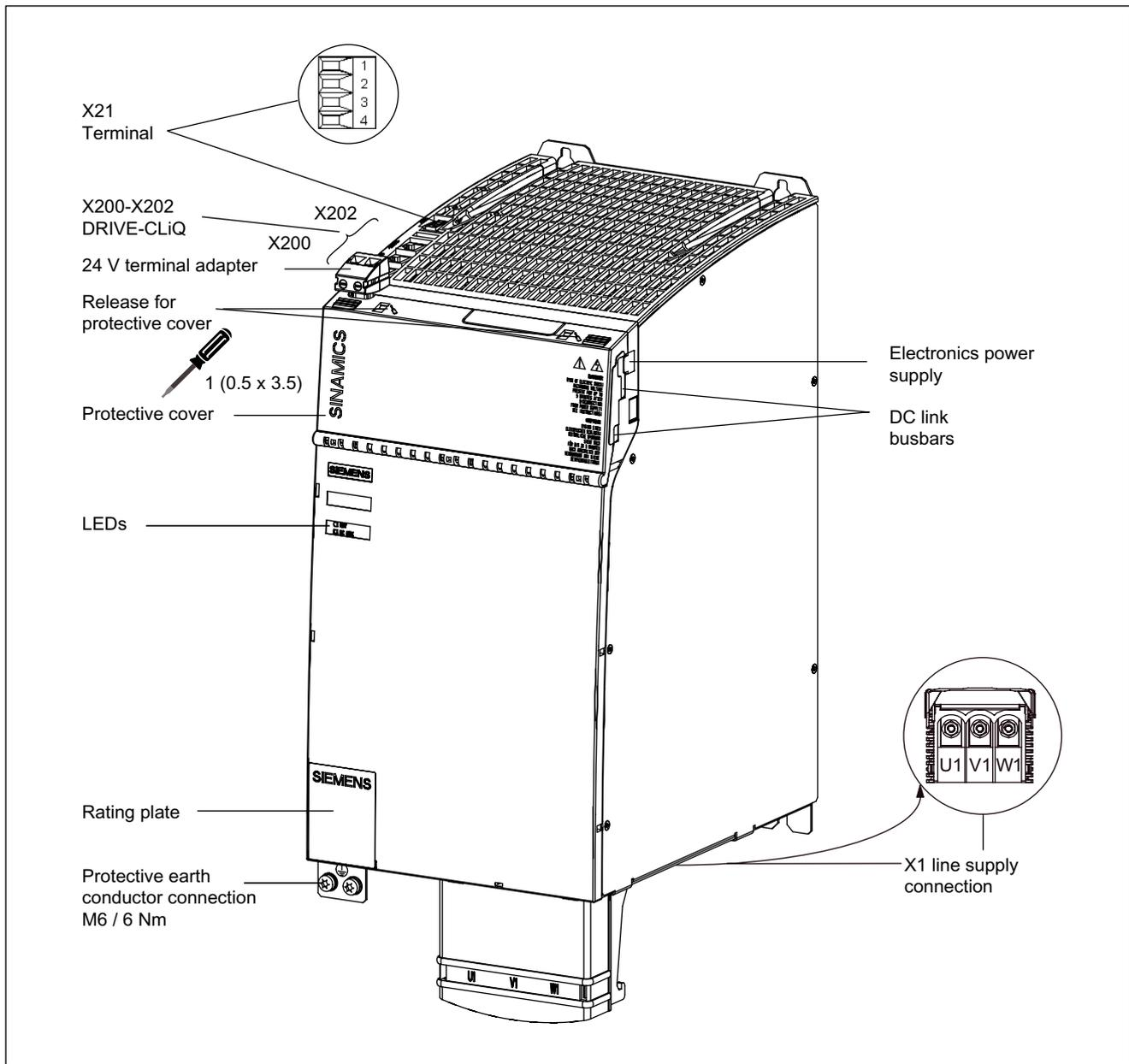
Figure 3-52 Basic Line Module with internal air cooling (100 kW)
