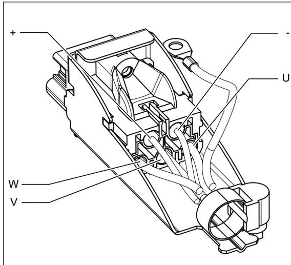
Figure 11-20 Motor connection plug with screwed joint
