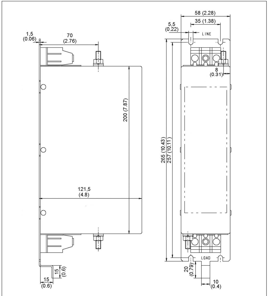
Figure 2-27 Dimension drawing of Basic Line Filter for Smart Line Modules 5 and 10 kW, all dimensions in mm and (inches)
