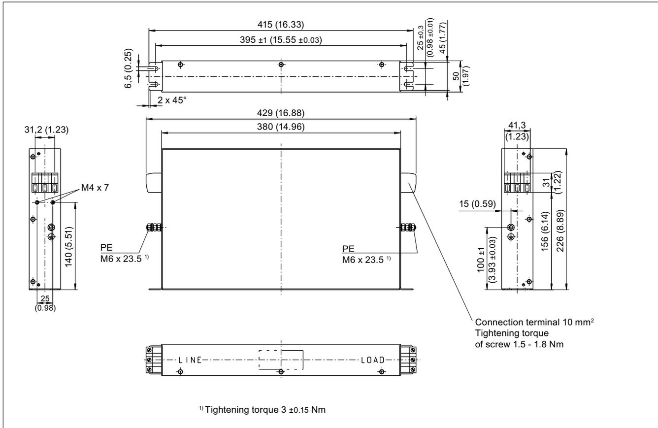
Figure 2-28 Dimension drawing of Basic Line Filter for Smart Line Modules 16 kW, order number 6SL3000-0BE21-6DAx, all dimensions in mm and (inches)
