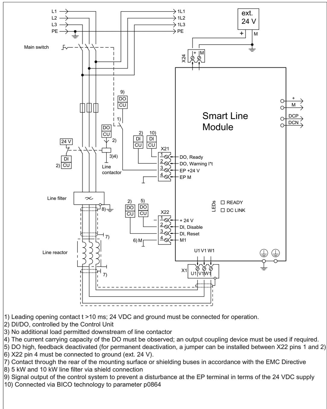
Figure 3-115 Connection example for 5 kW and 10 kW Smart Line Modules
