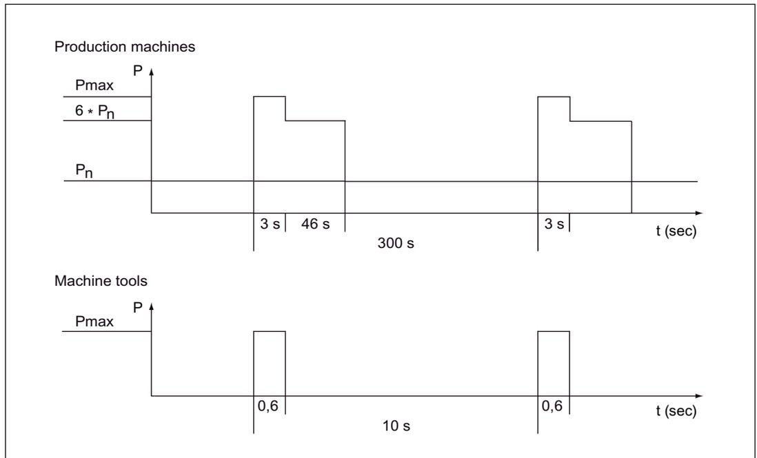
Figure 3-61 Braking duty cycle for Basic Line Modules
