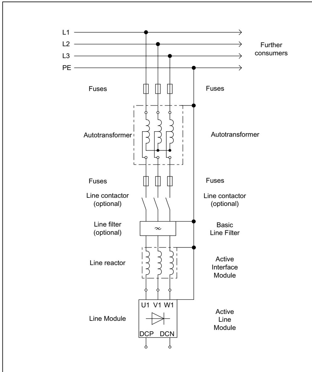
Figure 2-71 Autotransformer
