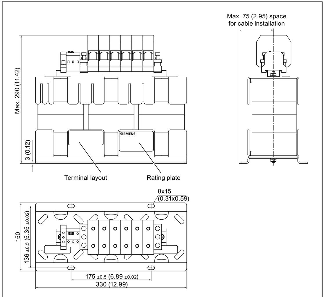
Figure 2-52 Dimension drawing of HFD line reactor 55 kW, all dimensions in mm and (inches)
