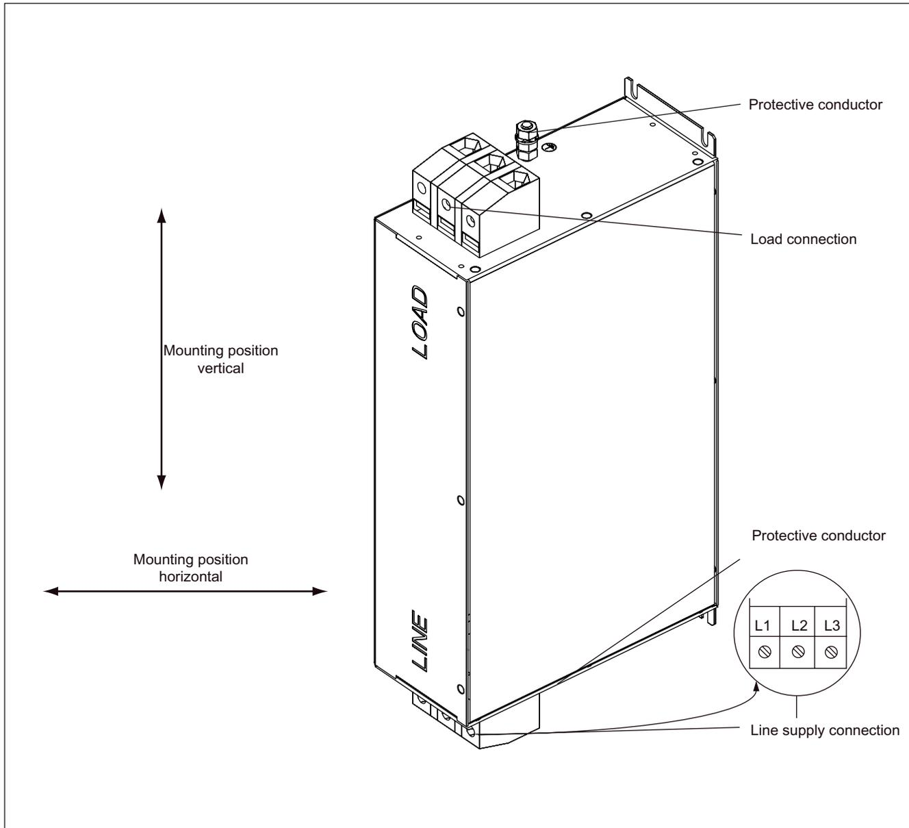
Figure 2-10 Basic Line Filter for Active Line Modules with Active Interface Module 55 kW
