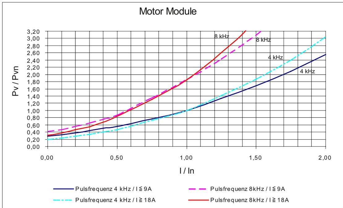
Figure 11-40 Losses in the partial load range for Motor Modules
