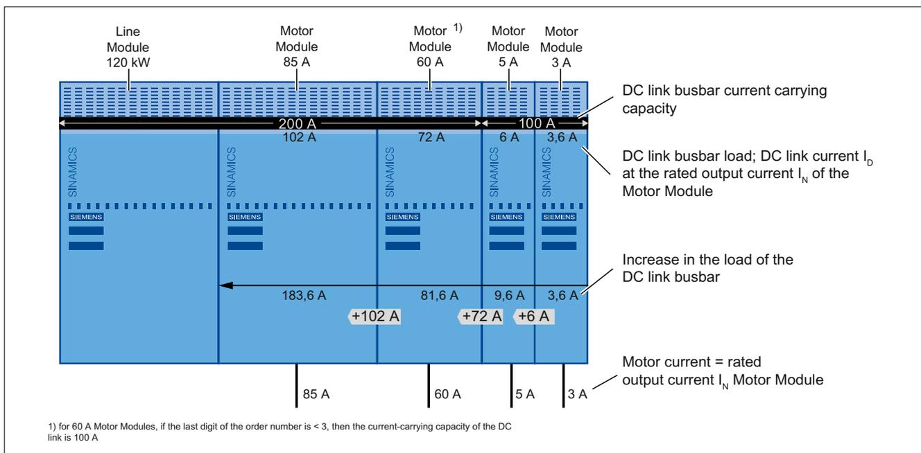
Figure 11-7 Regular arrangement; DC link busbar not overloaded
