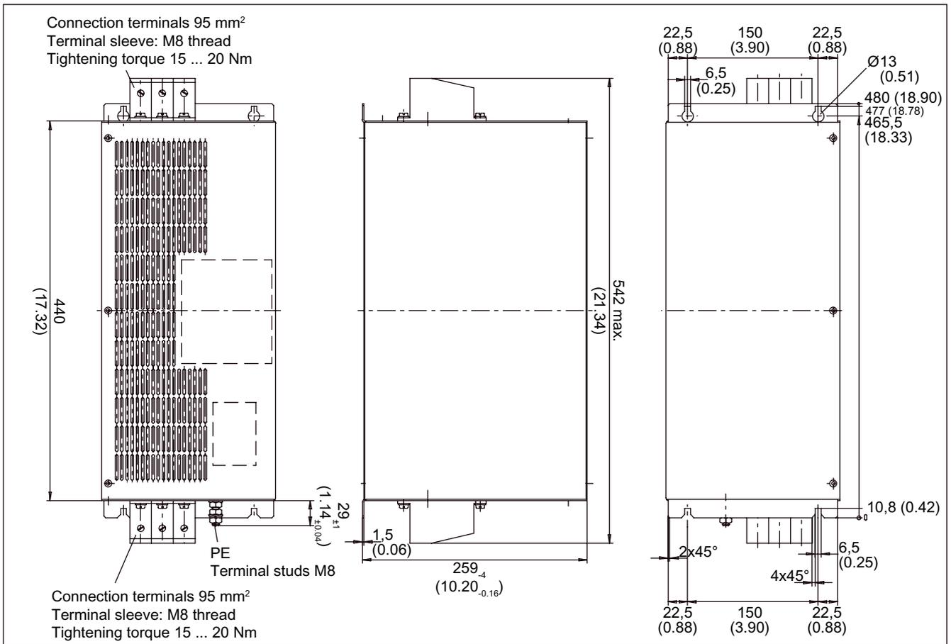
Figure 2-20 Dimension drawing of Wideband Line Filter 80 kW for Active Lines Modules, all dimensions in mm and (inches)
