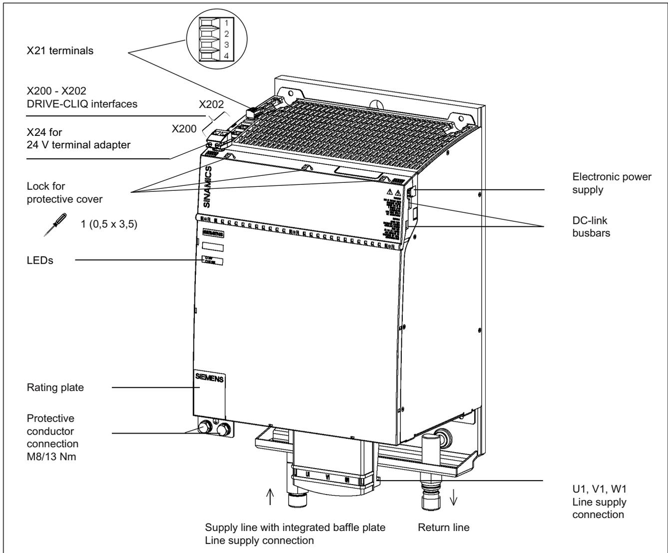
Figure 3-41 Active Line Module Liquid Cooled (120 kW)
