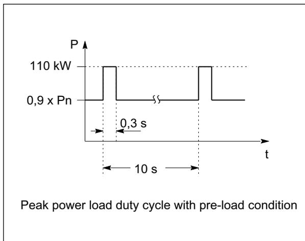
Figure 3-26 Rated duty cycle of 55 kW Active Line Modules with Active Interface Module
