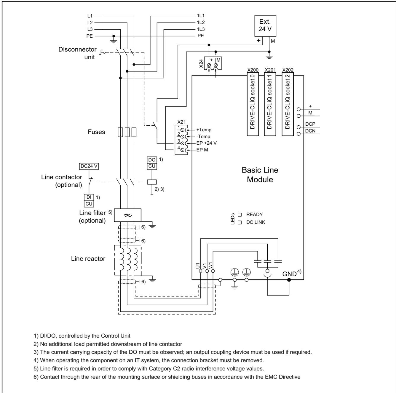
Figure 3-75 Connection example: Basic Line Module (100 kW)
