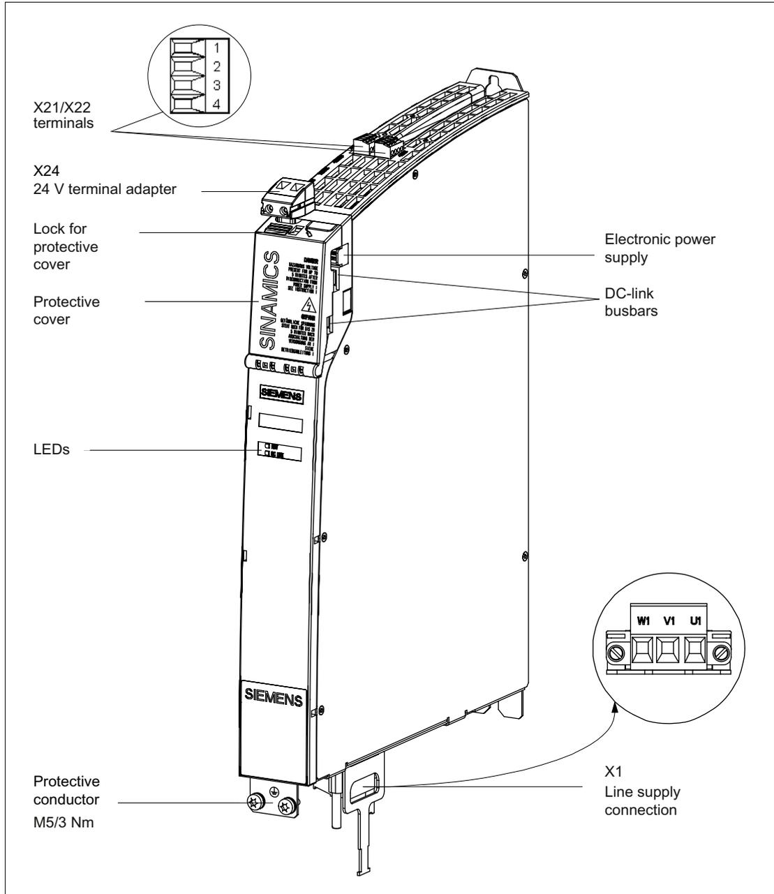
Figure 3-90 Smart Line Modules 5 kW and 10 kW with internal air cooling (example 5 kW)
