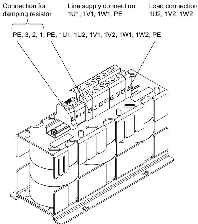
Figure 2-46 HFD line reactor 36 kW
