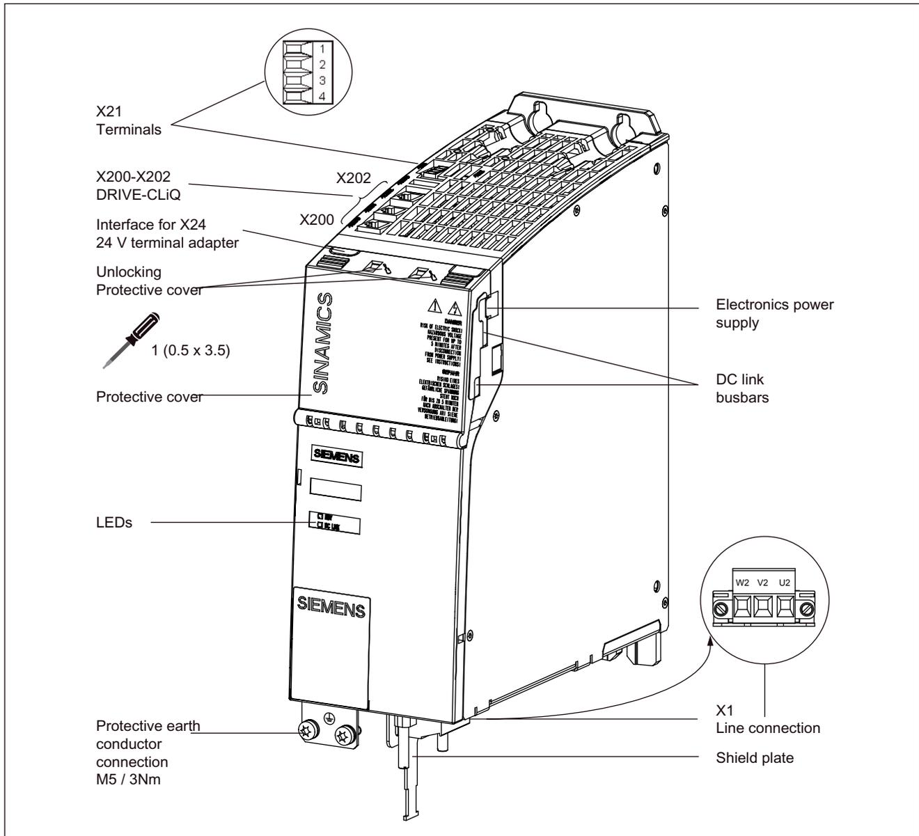
Figure 4-1 Smart Line Module in Booksize Compact format (16 kW)
