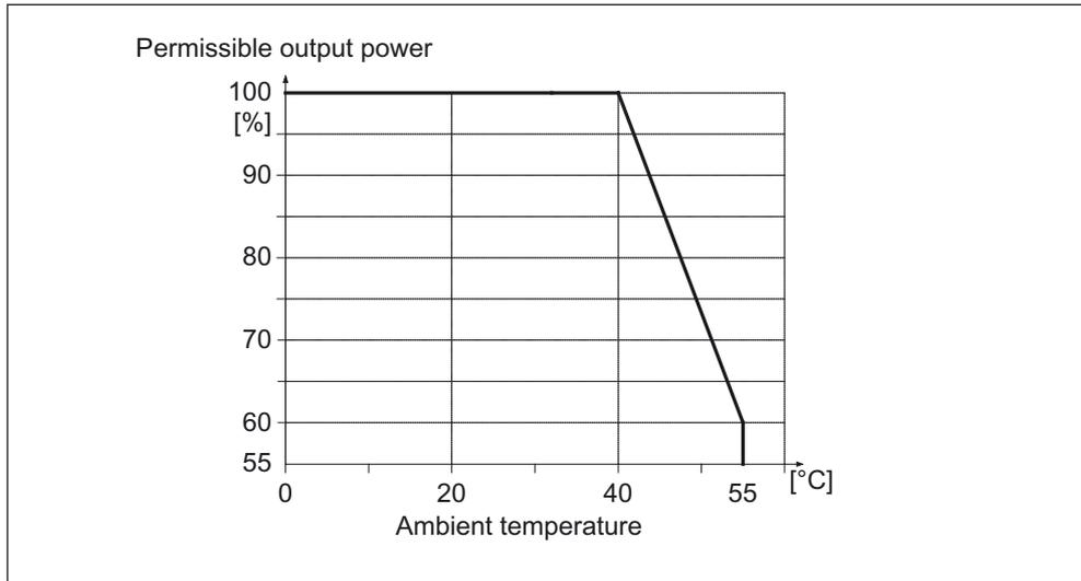
Figure 3-111 Output power as a function of the ambient temperature
