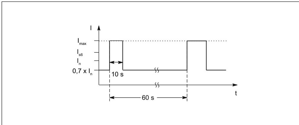
Figure 5-12 S6 duty cycle with initial load with a duty cycle duration of 60 s (for servo drives)
