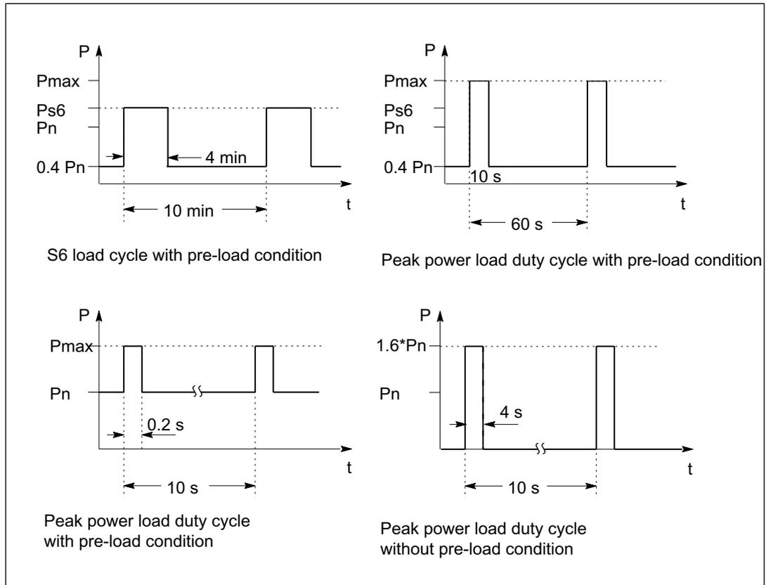
Figure 4-6 Rated duty cycles of Smart Line Modules
