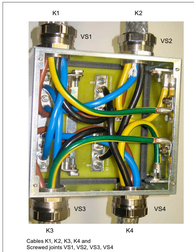
Figure 9-17 Wired Voltage Protection Module VPM 200 Dynamik with short designations
