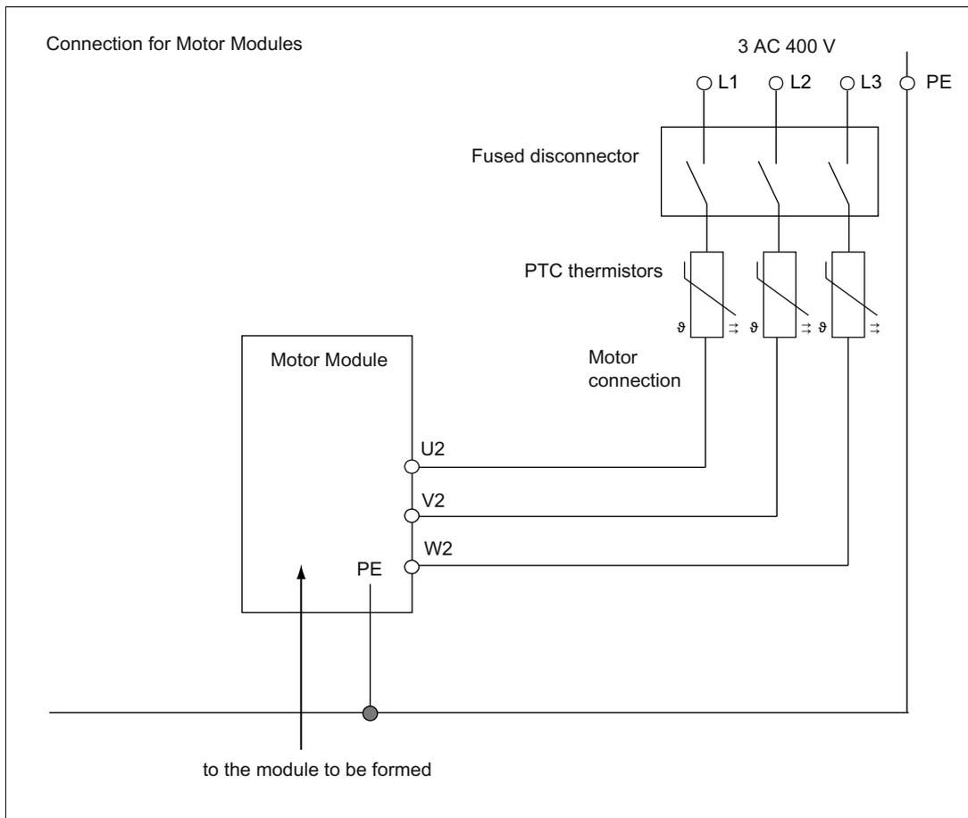
Figure 13-4 Forming circuit for Motor Modules with PTC resistors
