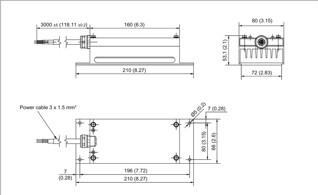
Figure 2-55 300 W damping resistor for HFD line reactors, all dimensions in mm and (inches)
