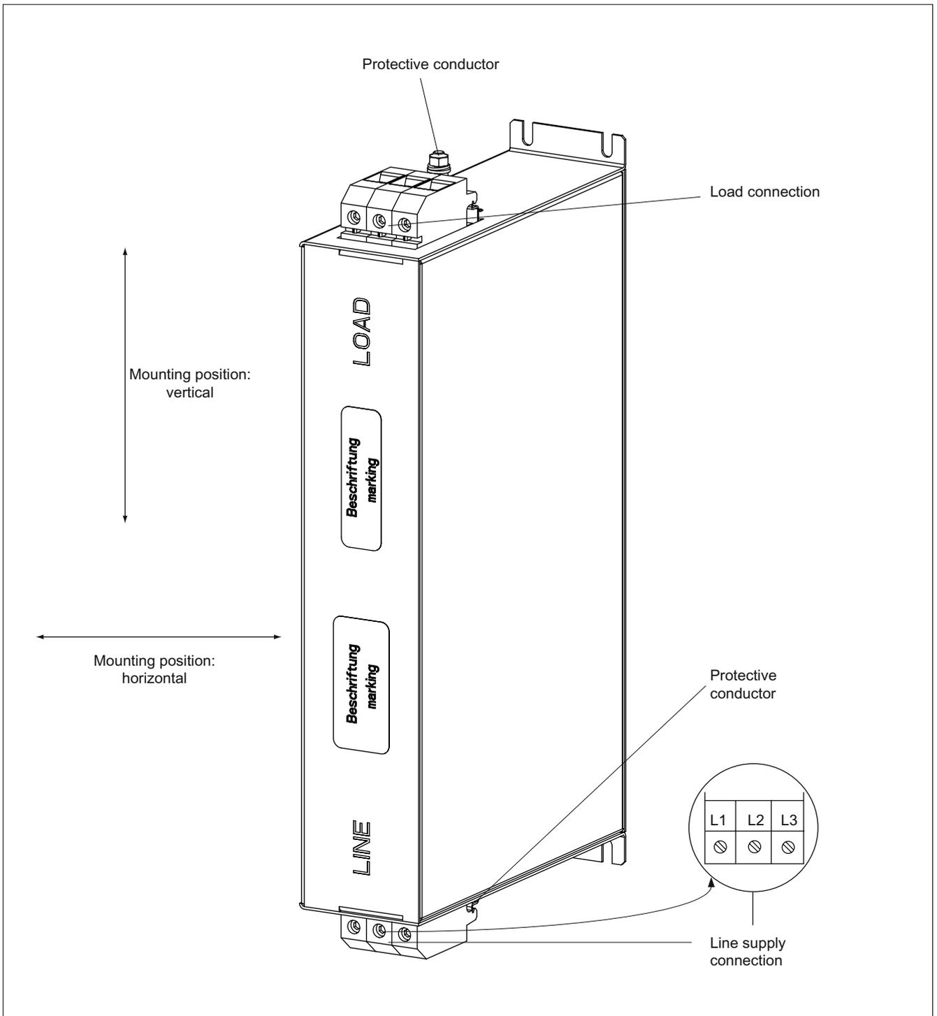
Figure 2-9 Basic Line Filter for Active Line Modules with Active Interface Module 36 kW
