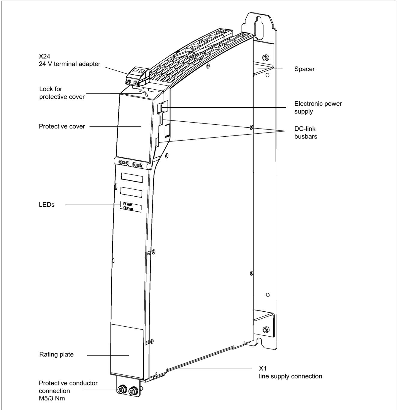
Figure 8-11 Interface description: control supply module
