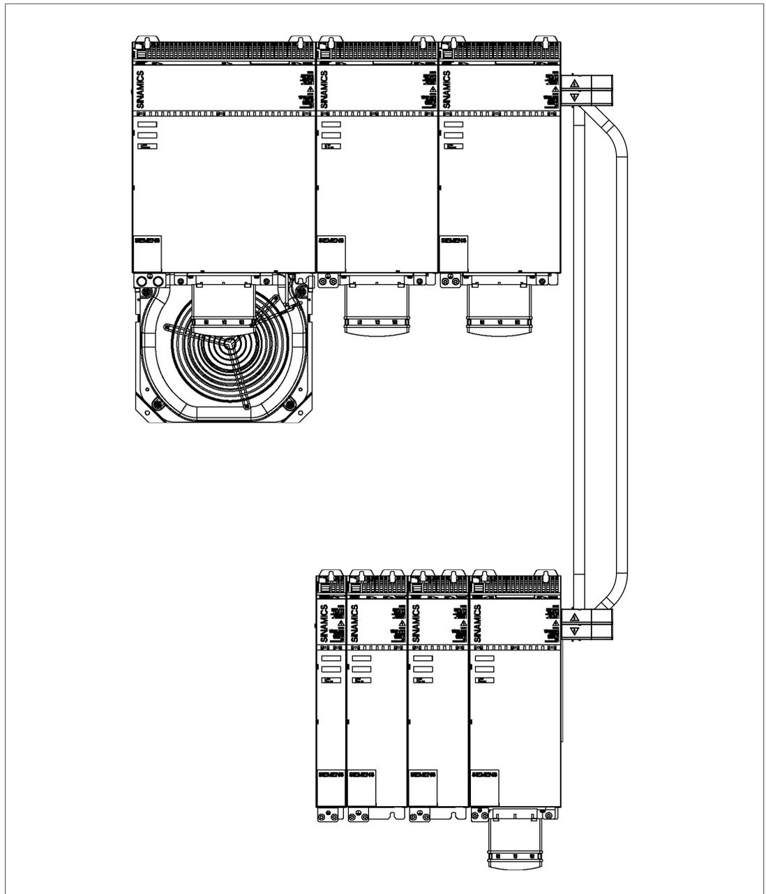
Figure 11-12 Example of a two-tier configuration with components between 150 and 300 mm wide
