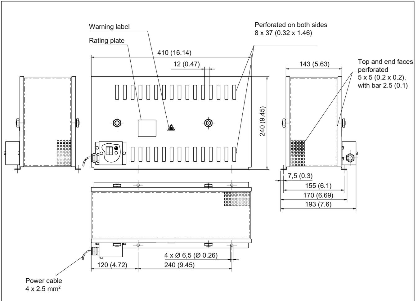
Figure 2-57 1500 W damping resistor for HFD line reactors, all dimensions in mm and (inches)
