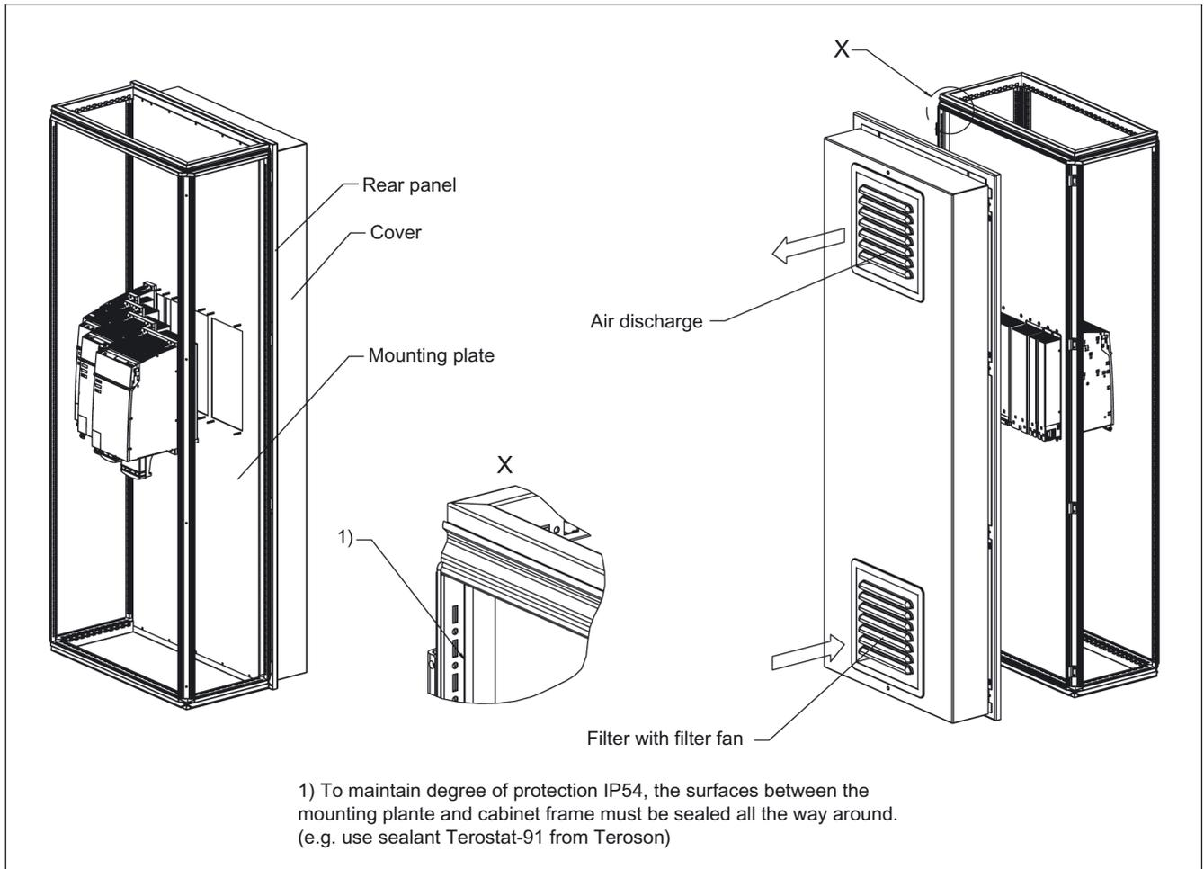
Figure 3-22 Example 1: installation in cabinet with mounting plate
