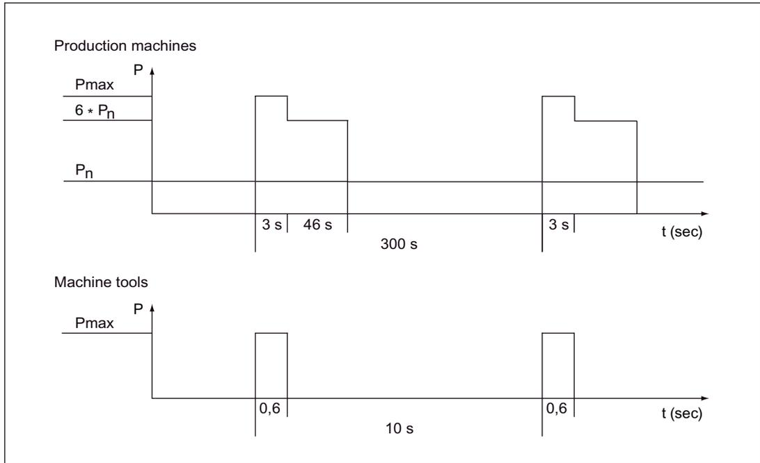
Figure 3-83 Braking duty cycle for Basic Line Modules
