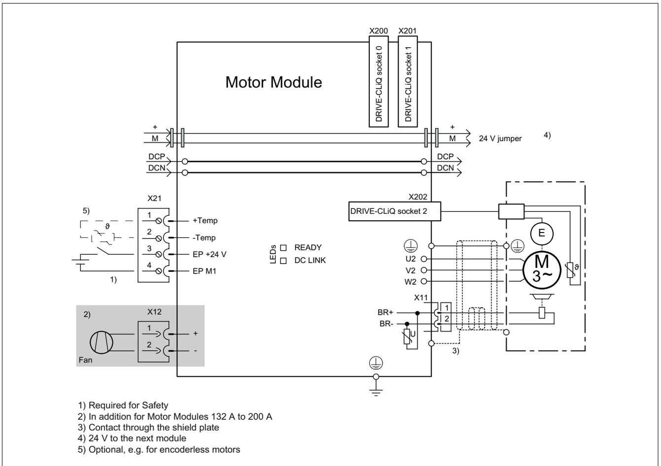
Figure 5-47 Example connection of Single Motor Modules 45 A to 200 A
