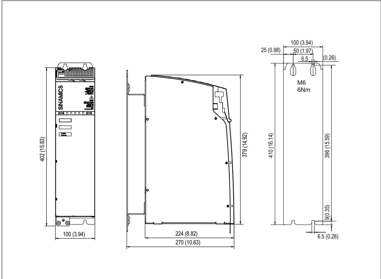
Figure 8-9 Dimension drawing of Capacitor Module, all dimensions in mm and (inches)
