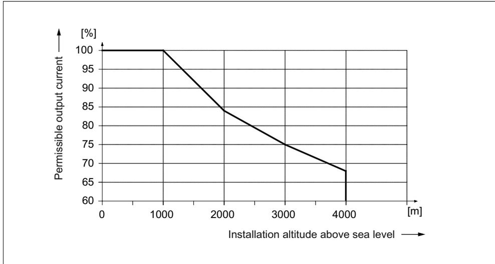
Figure 3-48 Output current as a function of the installation altitude
