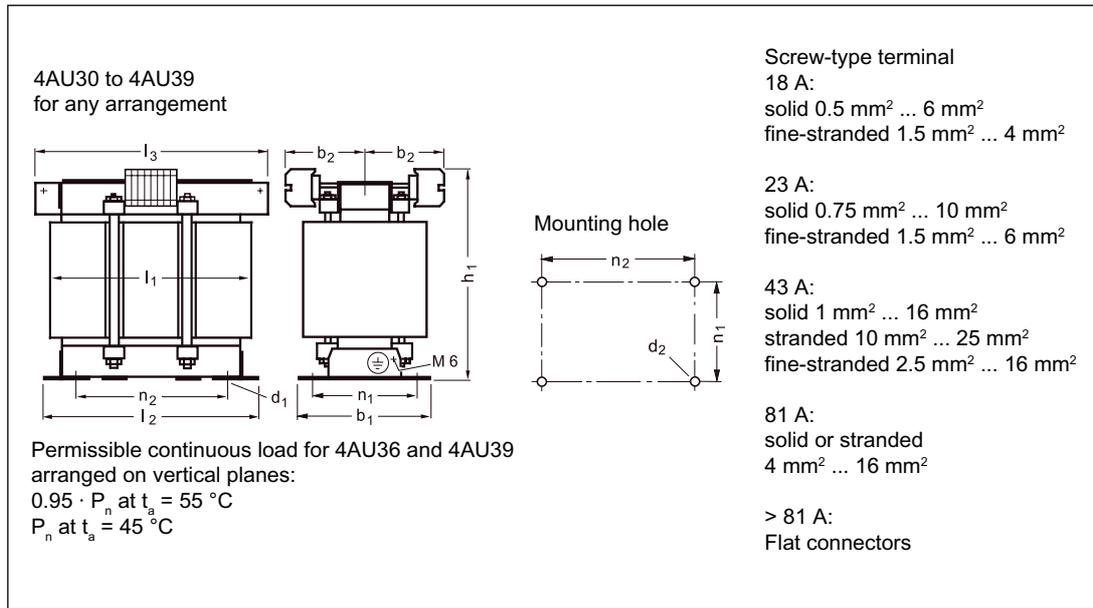
Figure 2-74 Dimension drawing: 4AU30 to 4AU39
