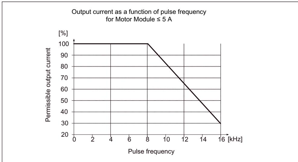
Figure 6-18 Output current as a function of the pulse frequency for the Motor Module  $\leq 5$  A
