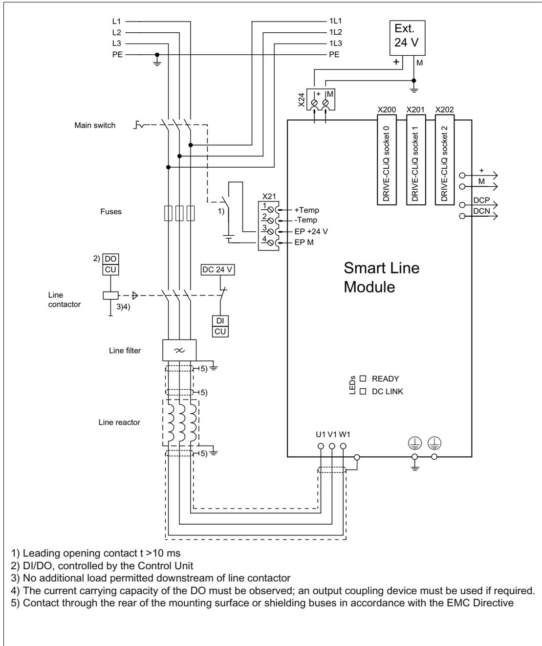
Figure 3-94 Connection example for 16 kW and 36 kW Smart Line Modules
