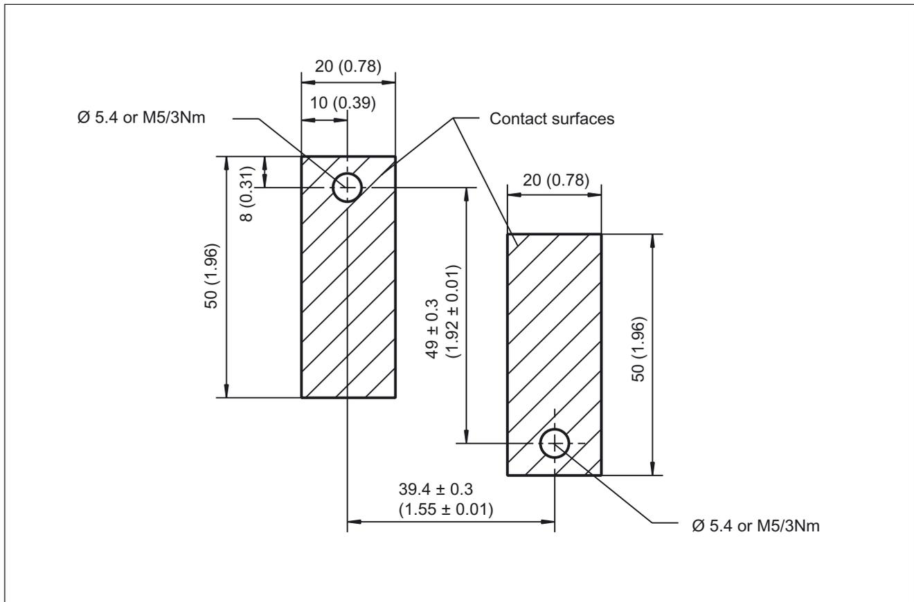
Figure 10-33 Hole drilling pattern for installation
