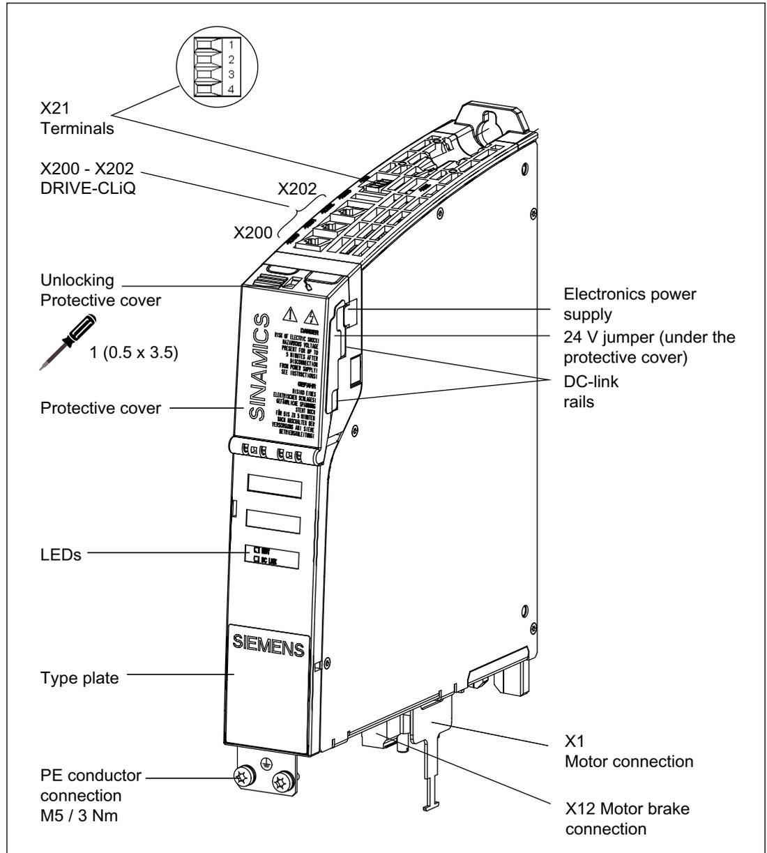
Figure 6-1 Example: Motor Module Booksize Compact format 3 A, 5 A, and 9 A
