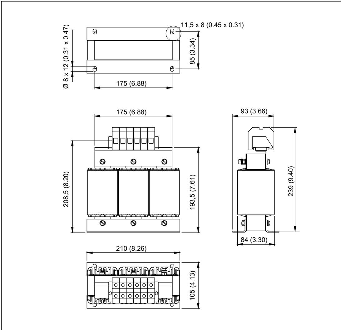
Figure 2-67 Dimension drawing of line reactor for Basic Line Module 40 kW, all dimensions in mm and (inches)
