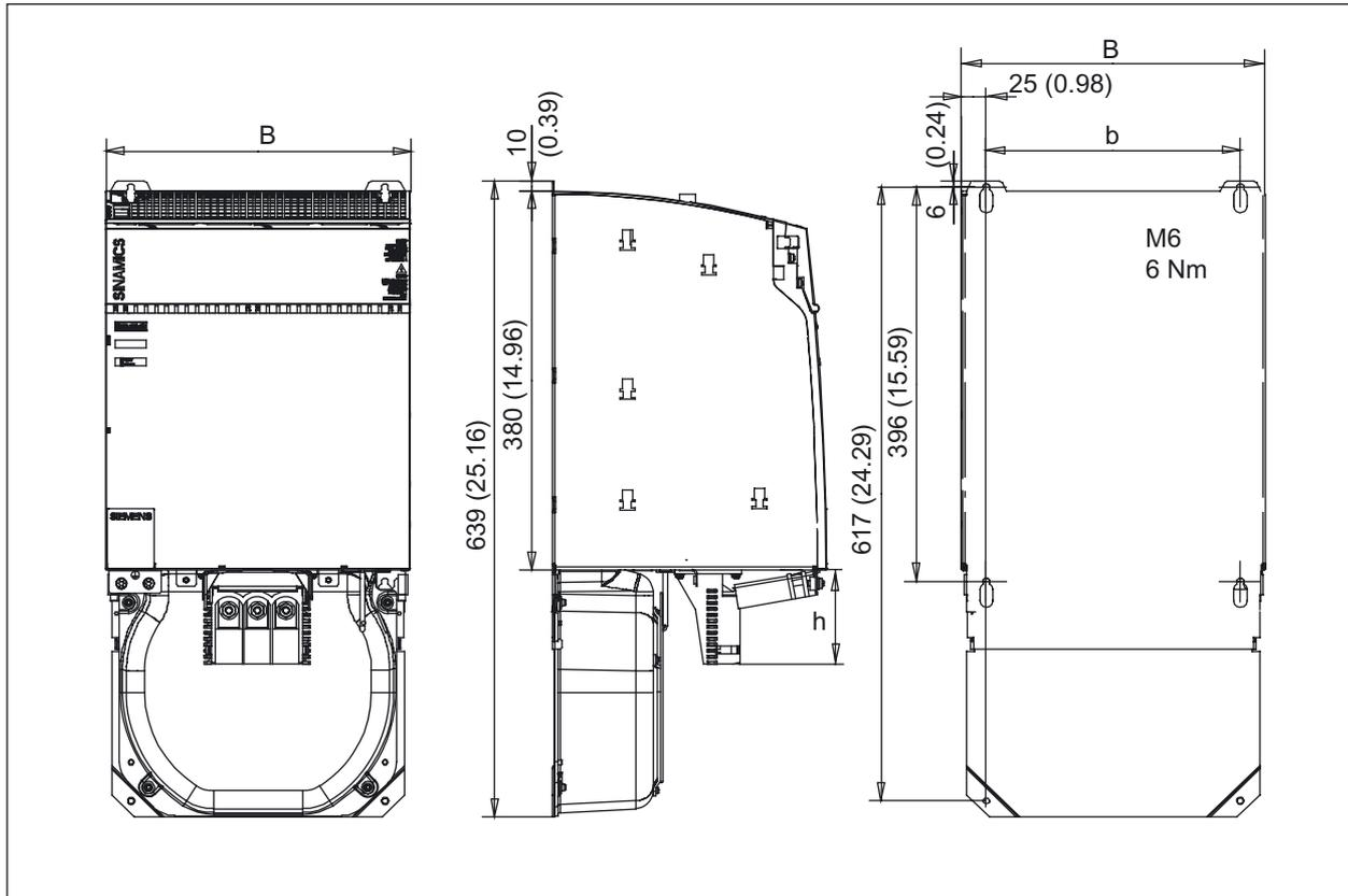
Figure 3-5 Dimension drawing of Active Line Modules 80 kW and 120 kW with internal air cooling, all data in mm and (inches)
