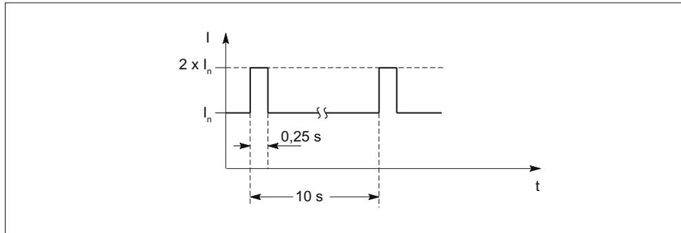
Figure 6-10 Duty cycle with initial load
