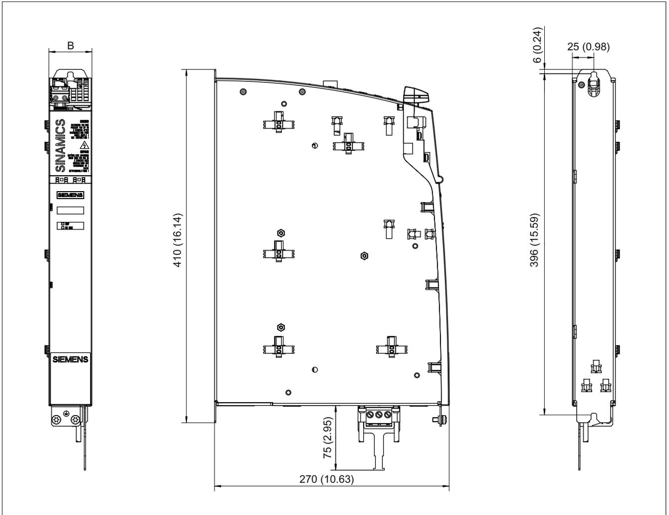
Figure 3-95 Dimension drawing of Smart Line Module with internal air cooling (5 kW and 10 kW), all dimensions in mm and (inches)
