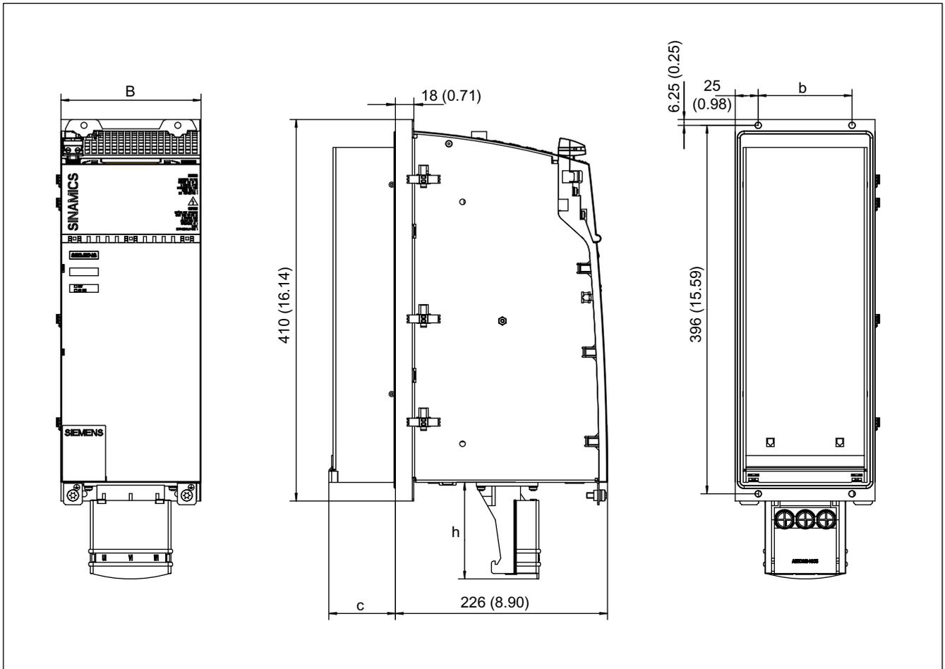
Figure 3-17 Dimension drawing of Active Line with external air cooling 36 kW, 55 kW, 80 kW, and 120 kW, all data in mm and (inches)
