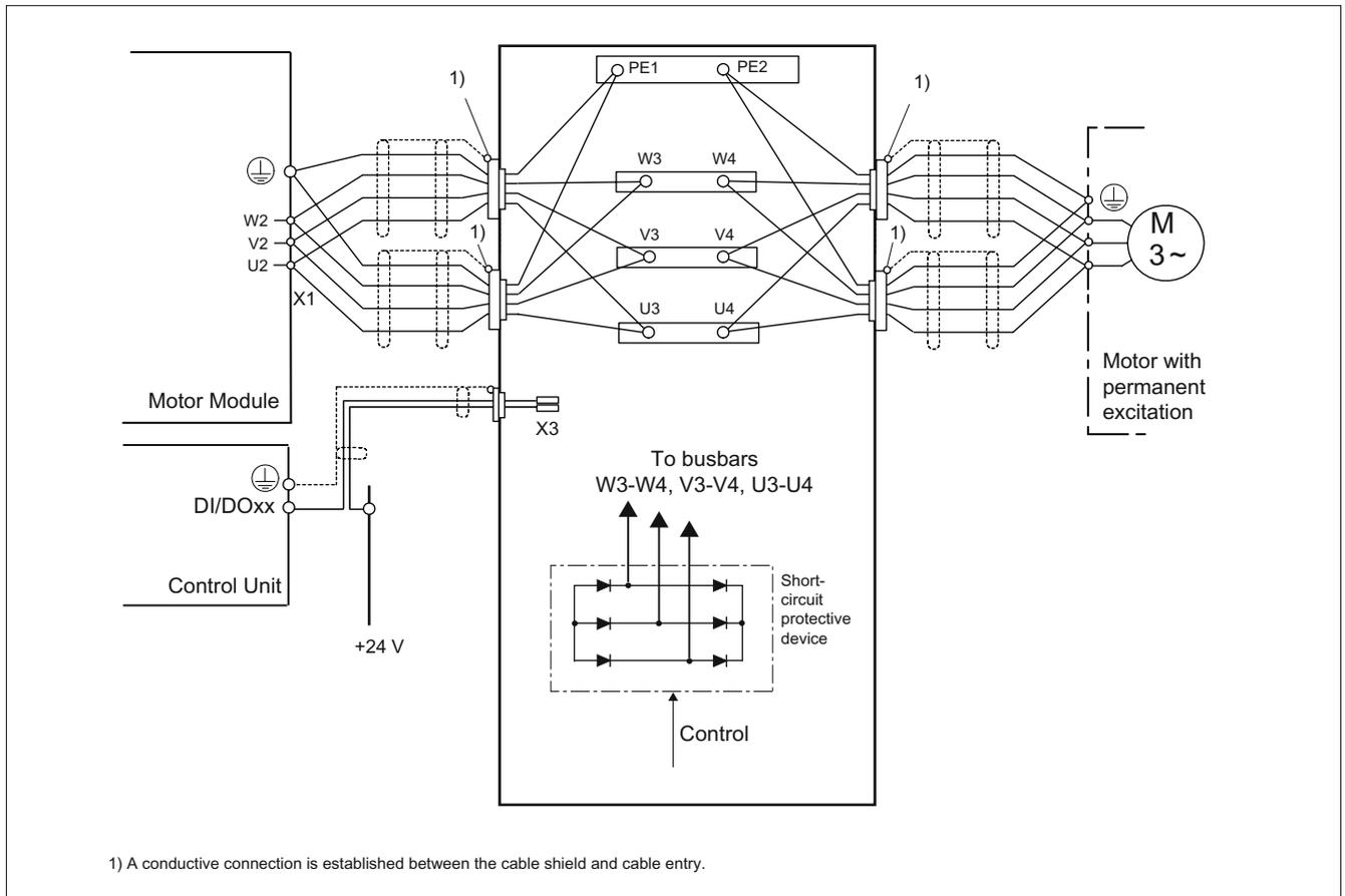
Figure 9-9 Connection example for Voltage Protection Module VPM 200
