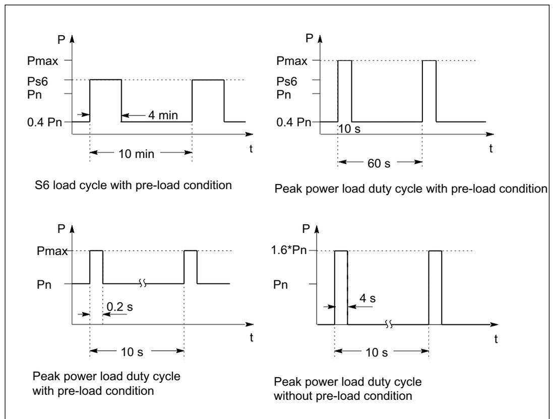
Figure 3-110 Rated duty cycles of Smart Line Modules
