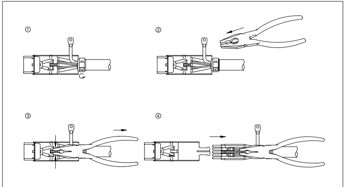
Figure 11-22 Removing the motor connection plug with screwed joint
