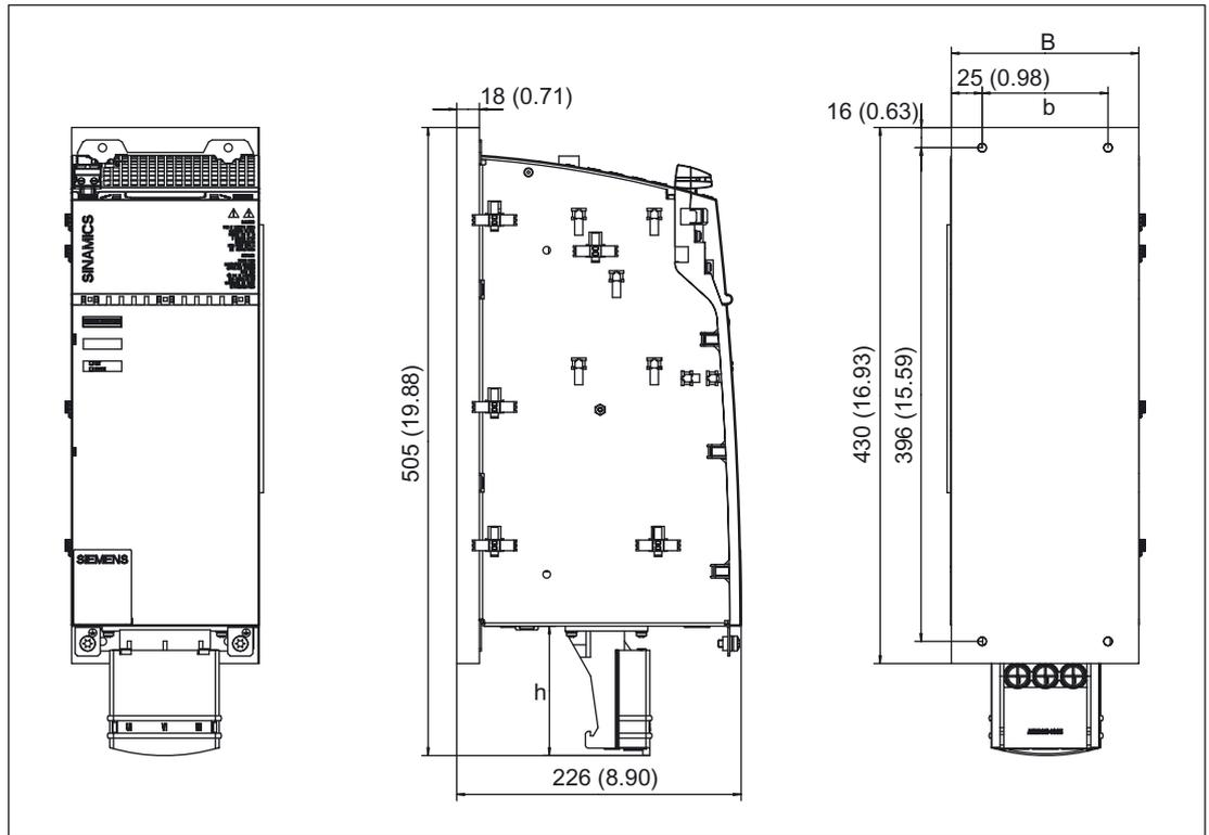
Figure 3-33 Dimension drawing of Active Line Module with cold plate (36 kW, 55 kW, 80 kW, and 120 kW), all dimensions in mm and (inches)
