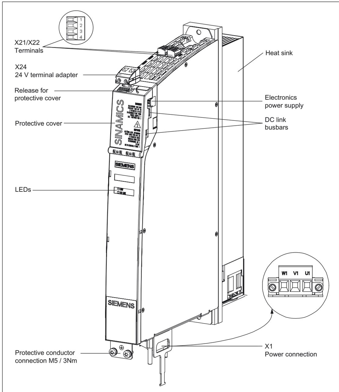
Figure 3-102 Smart Line Module with external air cooling (example 5 kW)
