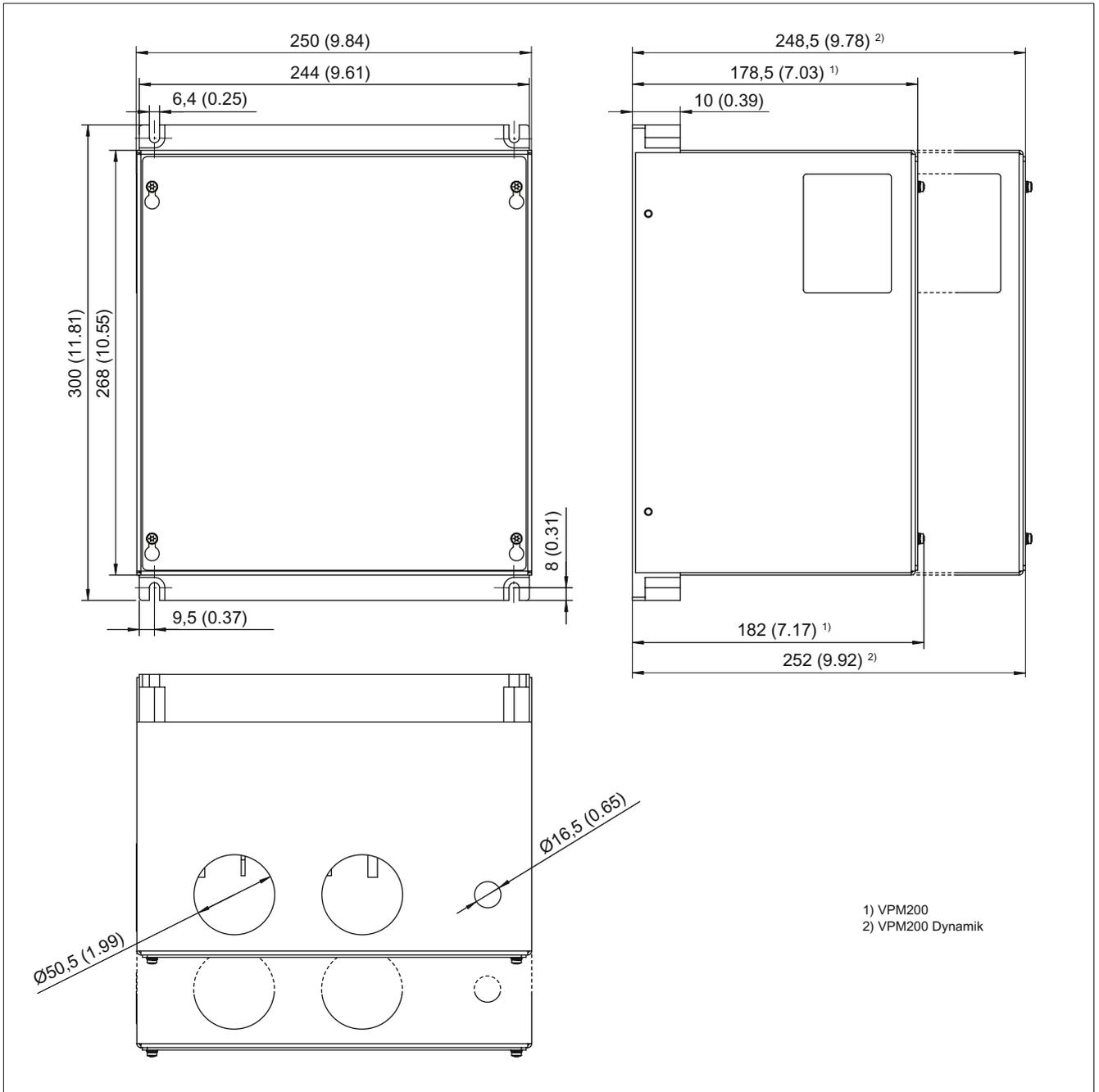
Figure 9-12 Dimension drawing of the Voltage Protection Module VPM200 and VPM200 Dynamic, all data in mm and (inches)
