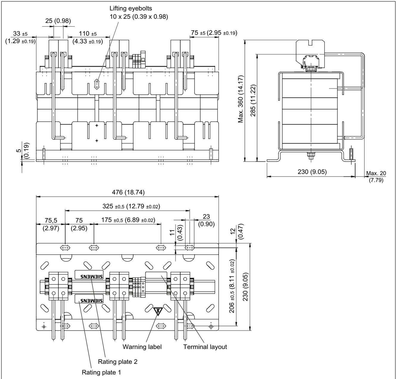
Figure 2-54 Dimension drawing of HFD line reactor 120 kW, all dimensions in mm and (inches)
