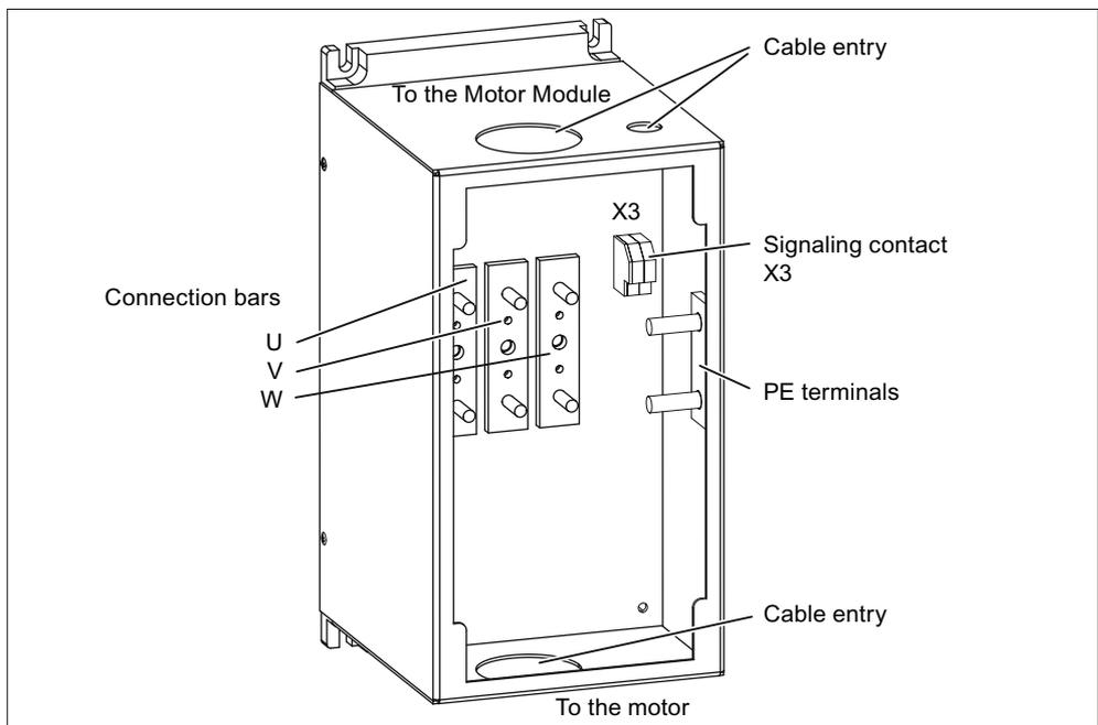
Figure 9-5 Voltage Protection Modules VPM 120 (without cover)
