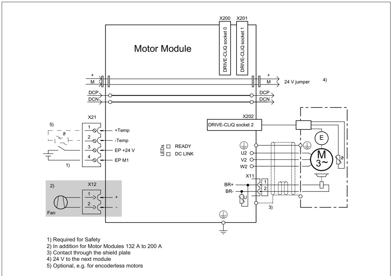
Figure 5-3 Example connection of Single Motor Modules 45 A to 200 A
