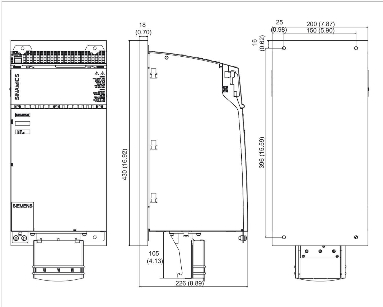
Figure 3-78 Dimension drawing of Basic Line Module with cold plate (100 kW), all dimensions in mm and (inches)
