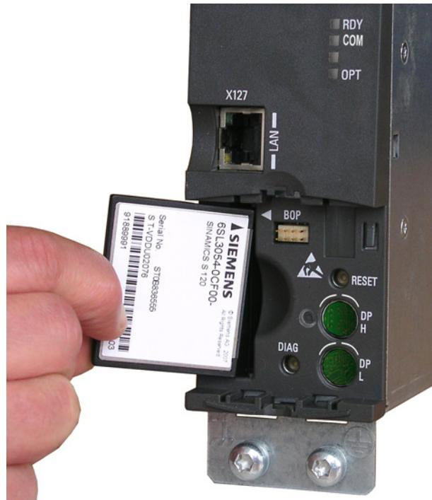
Figure 3-7 Slot for memory card
